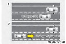
The BSD (Blind spot detection) system uses a radar sensor to alert the driver while driving.
