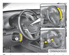
To change the steering wheel angle, pull down the lock-release lever (1), adjust the steering wheel to the desired angle (2) and height (3, if equipped) then pull up the lock-release lever to lock the steering wheel in place. Be sure to adjust the steering wheel to the desired position before driving.
