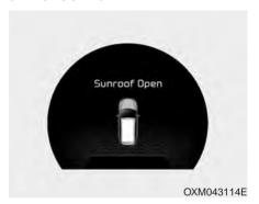
If the driver removes the ignition key (smart key: turns off the engine) and opens the driver-side door when the sunroof is not fully closed, the warning chime will sound for a few seconds and a message "Sunroof Open" will appear on the LCD display.
