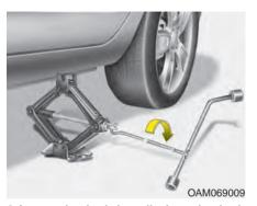
8.Insert the jack handle into the jack and turn it clockwise, raising the vehicle until the tire just clears the ground. This measurement is approximately 30 mm (1 in.).
