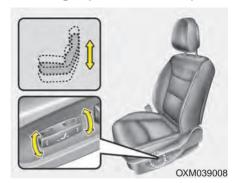
Pull the front portion of the control switch up to raise or press down to lower the front part of the seat cushion. Pull the rear portion of the control switch up to raise or press down to lower the rear part of the seat cushion. Release the switch once the seat reaches the desired position.
