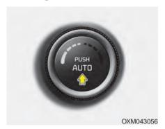
Press the AUTO button. The modes, fan speeds, air intake and air-conditioning will be controlled automatically by setting the temperature.
