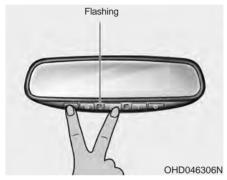
1. When programming the buttons for the first time, press and hold the left and center buttons (① ① ① 10) simultaneously until the indicator light begins to flash after approximately 20 seconds. (This procedure erases the factory-set default codes. Do not perform this step when programming the additional HomeLink buttons.)
