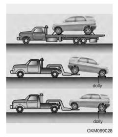
If emergency towing is necessary, we recommend having it done by an authorized Kia dealer or a commercial tow-truck service. Proper lifting and towing procedures are necessary to prevent damage to the vehicle. The use of wheel dollies or flatbed is recommended
