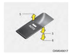
Pressing the power window switch momentarily to the second detent position (6) completely lowers the driver's window even when the switch is released. To stop the window at the desired position while the window is in operation, momentarily pull the switch in the direction opposite of the window's movement.
