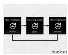
When the steering mode button is pressed, the selected steering mode will appear on the LCD display.
