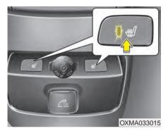
The seat warmer is provided to warm the rear seats during cold weather. With the ignition switch in the ON position, push either of the switches to warm rear seats.
