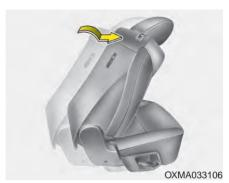
Fold the 2nd row seatback and push the seat to the farthest forward position.
