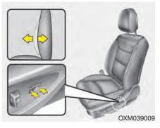
The lumbar support can be adjusted by pressing the button.
