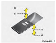
Pressing or pulling up the power window switch momentarily to the second detent position (6) completely lowers or raises the window even when the switch is released. To stop the window at the desired position while the window is in operation, pull up or press down and release the switch.
