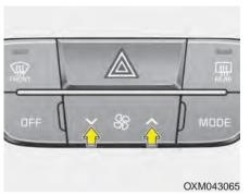
The fan speed can be set to the desired speed by operating the fan speed control switch.
