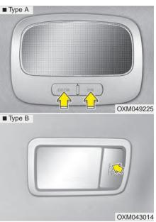
The light will turn on and off as below if the switch is pressed. The light will turn off if the button is pressed again.
