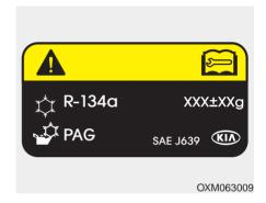
\* The actual Air Conditioning refrigerant label in the vehicle may differ from the illustration. Each symbols and specification on air conditioning refrigerant label means as below :
