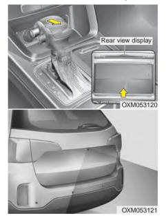
The rearview camera will activate with the ignition switch ON and the shift lever in the R (Reverse) position. This system is a supplemental system that shows behind the vehicle through the rearview display mirror while backing up unless equipped with a navigation system, then will display on the screen.
