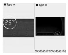
The current outside temperature is displayed in 1°C (1°F) increments. The temperature range is between -40°C  $\sim 60$ °C (40°F  $\sim 140$ °F).
