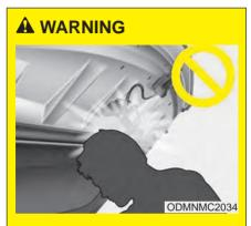
When you check the engine compartment, Take caution to avoid contacting your head with the safety hook which is located inside of the hood.
