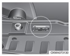
The refrigerant label is located at the front of the engine room.
