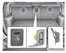
Child restraint hook holders are located on the back of the rear seat-backs.
