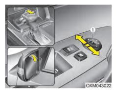
When you shift the shift lever to the R (Reverse) position, the outside rearview mirror(s) will move downward to aid reverse parking. According to the position of the outside rearview mirror switch (1), the outside rearview mirror(s) will operate as follows:
