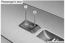
Operate by pressing the central door lock switch.
