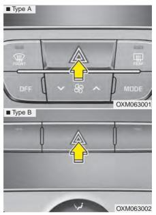
The hazard warning flasher should be used whenever you find it necessary to stop the vehicle in a hazardous location. When you must make such an emergency stop, always pull off the road as far as possible.
