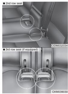
The rear seat belt buckles can be stowed in the pocket between the rear seatback and cushion when not in use.
