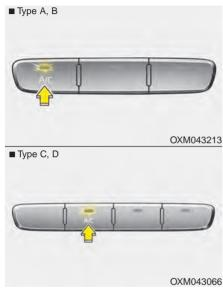
Press the A/C button to turn the air conditioning system on (indicator light will illuminate).
