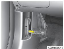
Check whether the stroke is within specification when the parking brake pedal is depressed with 30 kg (66 lb, 294 N) of force. Also, the parking brake alone should securely hold the vehicle on a fairly steep grade. If the stroke is more or less than specified, have the parking brake adjusted by an authorized Kia dealer.
