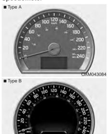
The speedometer indicates the speed of the vehicle and is calibrated in kilometers per hour (km/h) and/or miles per hour (mph).
