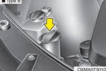
The reservoir is translucent so that you can check the level with a quick visual inspection.
