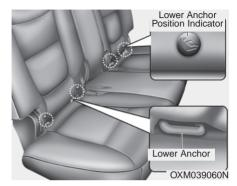
Child restraint symbols are located on the left and right 2nd row seat backs to indicate the position of the lower anchors for child restraints.
