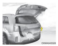
During power opening and closing if the power tailgate is blocked by an object or part of the body, the power tailgate will detect the resistance.
