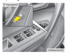
The fuel filler lid must be opened from inside the vehicle by pressing the fuel filler lid opener button on the driver's door. (if equipped)
