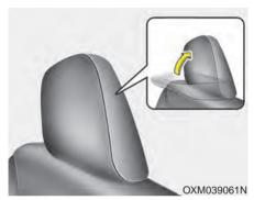
The headrest will fold down automatically when the seatback folding.
