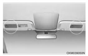
Air bag warning labels, some required by the Canada Motor Vehicle Safety Standards (CMVSS), are attached to the sunvisor to alert the driver and passengers of potential risks of the air bag system.
