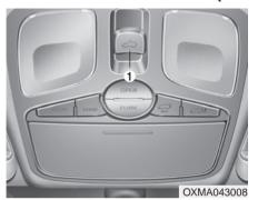
If your vehicle is equipped with a sunroof, you can slide or tilt your sunroof with the sunroof control lever located on the overhead console (1).
