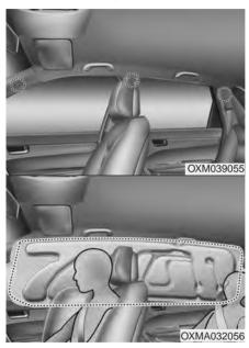
Curtain air bags are located along both sides of the roof rails above the front and rear doors.
