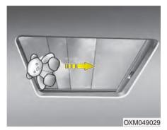
If an object or part of the body is detected while the sunroof is closing automatically, it will reverse the direction, and then stop.
