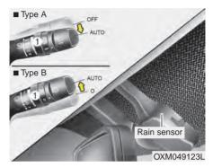
The rain sensor located on the upper end of the windshield glass senses the amount of rainfall and controls the wiping cycle for the proper interval. The more it rains, the faster the wiper operates. When the rain stops, the wipers stop. To vary the speed setting, turn the speed control knob (1).
