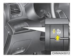
With the ignition switch in the ON position, pressing the heated steering wheel button warms the steering wheel. The indicator on the button will illuminate and notify you on the LCD display.
