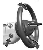
To adjust the steering wheel, if equipped:
