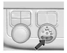
If equipped, the button for the front fog lights is on the headlight control, to the left of the steering column.
