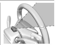
Sunglasses, hats, or other types of clothing that change the shape of the head may interfere with camera performance. To improve camera performance, raise or lower the steering wheel, wear lighter tinted glasses, or change the seat position.
