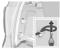
Remove the flat tire secure strap from the glove box and place the loop end of the strap through the cargo tie-down. Place the hook end of the strap through the loop and pull it until the strap is fastened securely to the tie-down.
