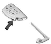
The mechanical key inside the remote key can be used for all locks.
