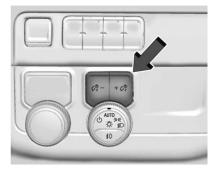
These buttons adjust the brightness of all illuminated controls. The instrument panel illumination control is above the exterior light control.
