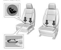
Executive seating lower anchors are in the crease between the seatback and the seat cushion. Push the seatback trim up at the crease to access the lower anchor.
