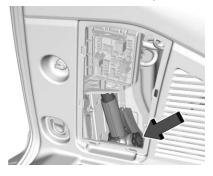
Turn the jack knob counterclockwise to release the jack and wheel blocks from the bracket. If equipped, remove the wheel blocks from the jack and place the wheel blocks on both sides of the tire at the opposite corner of the tire being changed.
