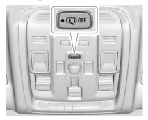
Dome lights provide overhead interior lighting, plus lighting in the rear cargo compartment.
