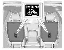
For non-executive seats, the top tether anchors are on the rear of the seatback for each seating position in the second row. Be sure to use an anchor located directly behind the seating position where the child restraint will be placed.
