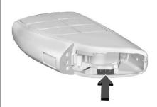
2. Use the mechanical key blade in the slot to remove the battery cover by hand.
