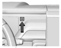
Press the A button to make the front and rear turn signal lights flash on and off. This warns others that you are having trouble. Press again to turn the flashers off.
