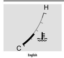
This gauge shows the engine coolant temperature.
