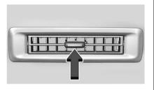
Move the slider knob on rectangular vents and rotate the outlet barrel left to right to change the direction of the air flow and to shut off the air flow
