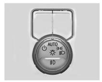
The headlight controls are on the instrument panel to the left of the steering wheel.
