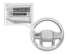
Press to turn cruise control on or off. When ACC is the selected cruise control mode, the ACC light is lit white on the instrument cluster. +RES: Press the button up briefly to resume the previous set speed or use to increase vehicle speed if ACC is already activated. To increase speed by about 1 km/h (1 mph), briefly press the button up to +RES and release it. To increase speed to the next 5 km/h (5 mph) mark on the speedometer, press up to +RES and hold.
