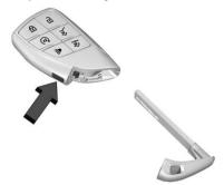
Press the button on the side of the remote key and pull the mechanical key out.
