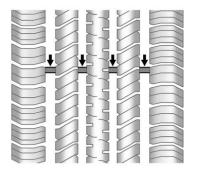
Treadwear indicators are one way to tell when it is time for new tires. Treadwear indicators appear when the tires have only 1.6 mm (1/16 in) or less of tread remaining. See *Tire Inspection* ♀ 337 and *Tire Rotation* ♀ 338.
