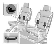
For non-executive seats, the lower anchors are located in the crease between the seatback and seat cushion.
