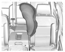
If the vehicle has a front center airbag, it is in the inboard side of the driver seatback.
