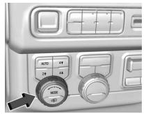
Turn the knob left or right to select the desired ride height in the menu. To finalize the selection, either press the Ride Height button again or wait three seconds for the menu to timeout. Ride Heights that are unavailable are greyed out in the menu.
