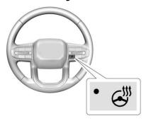
**!** : If equipped, press to turn the heated steering wheel on or off. An indicator next to the button is lit when the feature is turned on.
