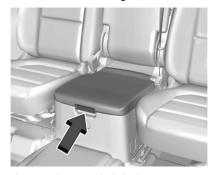
If equipped, you can lock the front center seat storage with the mechanical key inside the remote key. See *Keys* ⇔ 7.
