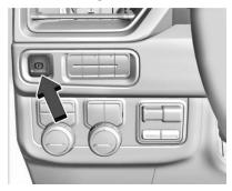
The Electric Parking Brake (EPB) can be applied when the vehicle is off. If there is not enough electrical power, the EPB cannot be applied or released. To prevent draining the battery, avoid unnecessary repeated cycles of the EPB.
