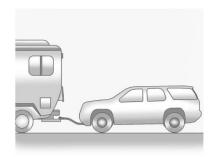
Only dinghy tow four-wheel-drive vehicles with a two speed transfer case that has an N (Neutral) and a 44 setting.
