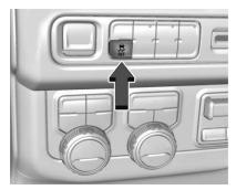
The button for the Traction Control System and the StabiliTrak/Electronic Stability Control system is on the instrument panel to the left of the steering wheel.
