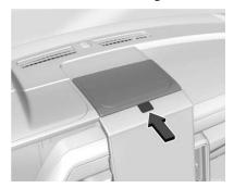
There is storage on the instrument panel. To open, if the storage is covered, press the button and the cover will lift open. To close, pull the storage cover down until it latches and makes an audible click.
