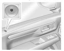
The light, on the driver door near the window, indicates the status of the sustem.
