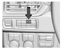
The Auto Stop/Start feature can be disabled and enabled by pressing (A). Stop/Start is enabled each time you start the vehicle.
