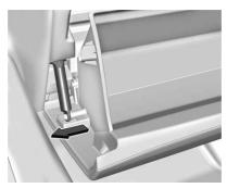
3. Unsnap dampener by pushing outwards to fully remove the glove box bin.
