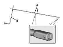
2. Assemble the jack handle extensions (4) and wheel wrench (5), as shown.
