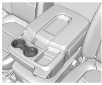
The cupholders are in front of the center console storage area when the armrest is down. See *Center Console Storage* ▷ 100.
