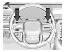
Electronic Range Select, or Manual Mode, allows for the selection of the range of gear positions. Use this mode when driving downhill or towing a trailer to limit the top gear and vehicle speed. The shift position indicator within the Driver Information Center will display a number next to the L indicating the highest available gear.
