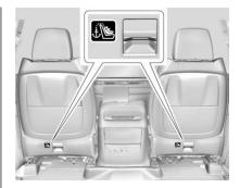
Executive seating top tether anchors are on the lower structure of seat back behind a fabric slit. Slide the seat forward to access the anchor. Be sure to use an anchor located directly behind the seating position where the child restraint will be placed. See Second Row Seats \$\dip\$ 47.
