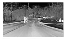
With the Front Pedestrian Braking system turned on, Night Vision provides a red Head-Up Display (HUD) alert, if equipped, when the system detects that the vehicle is approaching a pedestrian or large animal ahead too quickly. In addition, an alert beeps or the Safety Alert Seat pulses, if equipped. See Front Pedestrian Braking (FPB) System ▷ 270.
