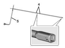
3. Assemble the jack handle extensions (4) and wheel wrench (5).
