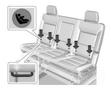
The lower anchors are located in the crease between the seatback and seat cushion.
