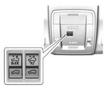
If equipped, the sunroof operates when the ignition is in ACC/ACCESSORY or ON/RUN, or when Retained Accessory Power (RAP) is active. See Retained Accessory Power (RAP) on page 9-28.
