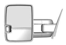
If equipped, adjust trailer-tow mirrors for a clear view of the area behind you. Manually pull out the mirror head to extend it for better visibility when towing a trailer. The lower portion of the mirror is convex. A convex mirror's surface is curved to see more from the driver seat. The convex mirror can be adjusted manually to the driver preferred position for better vision.
