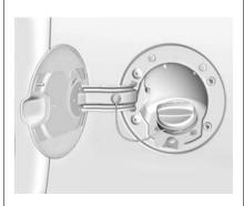
The fuel cap is behind a hinged fuel door on the driver side of the vehicle. Vehicles that have a FlexFuel badge and a yellow fuel cap can use either unleaded gasoline or ethanol fuel containing up to 85% ethanol (E85). See *E85* or FlexFuel on page 9-66.
