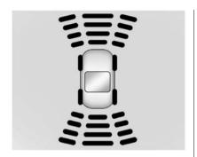
The instrument cluster may have a parking assist display with bars that show "distance to object" and object location information for RPA, and on some vehicles, for FPA. As the object gets closer, more bars light up and the bars change color from yellow to amber to red.
