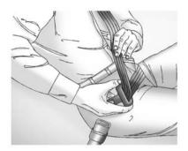
For the driver and front outboard seating positions on light duty vehicles and the center seating position (if equipped) on crew cab and double cab models, if the webbing locks in the latch plate before it reaches the buckle, tilt the latch plate flat to unlock
