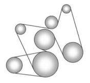
**6.0L V8 Engines**If the vehicle has a diesel engine, see the Duramax diesel supplement.
