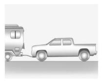
Only dinghy tow four-wheel-drive vehicles with a two-speed transfer case that have an N (Neutral) and a Four-Wheel Drive Low (4 (\$\d\dagger\$) setting.
