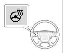
(Heated Steering Wheel, If Equipped): Press to turn it on or off. A light next to the button displays when the feature is turned on.
