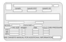
A vehicle-specific Certification/ Tire label is label is attached to the center pillar (B-pillar). The label shows the size of the vehicle's original tires and the inflation pressures needed to obtain the gross weight capacity of the vehicle. This is called Gross Vehicle Weight Rating (GVWR). The GVWR includes the weight of the vehicle, all occupants, fuel, and cargo.
