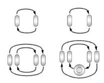
Use this rotation pattern when rotating the tires if the vehicle has polished forged aluminum dual rear wheels. The spare wheel can be used in any position and can be rotated with the rear inner wheels.
