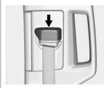
Push down on the release button to move the height adjuster to the desired position.
