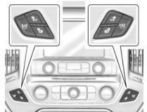
Heated and Cooled Seat Buttons Shown, Heated Seat Buttons Similar
