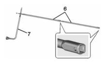
Assemble the wheel wrench (7) and the two jack handle extensions (6), as shown.
