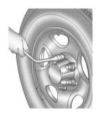
If the vehicle has wheel nut caps, loosen them by turning the wheel wrench counterclockwise. If the vehicle has a center cap with wheel nut caps, the wheel nut caps are designed to stay with the center cap after they are loosened. Remove the entire center cap.
