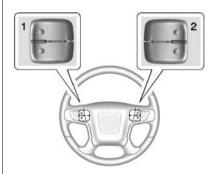
The favorite and volume switches are on the back of the steering wheel.
