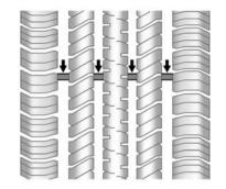
Treadwear indicators are one way to tell when it is time for new tires. Treadwear indicators appear when the tires have only 1.6 mm (1/16 in) or less of tread remaining. Some commercial truck tires may not have treadwear indicators. See *Tire Inspection on page 10-68* and *Tire Rotation on page 10-68* for additional information.
