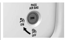
To turn the front outboard passenger frontal airbag on again, insert the ignition key into the switch, push in, and move the switch to the on position.
