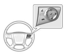
If equipped, some audio controls can be adjusted at the steering wheel.
