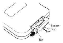
2. Remove the old battery and install a new one with the plus pole pointed up.
