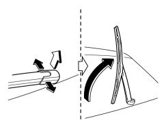
2. Firmly rotate the wiper blade to the right until it unlocks, then remove the blade
