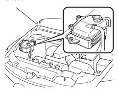
If it's at or near L, add enough coolant to the coolant reservoir to provide freezing and corrosion protection and to bring the level to F.
