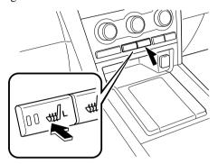
Press the seat warmer switch to illuminate the indicator light while the ignition is switched ON. The mode changes as follow each time the seat warmer switch is pressed.
