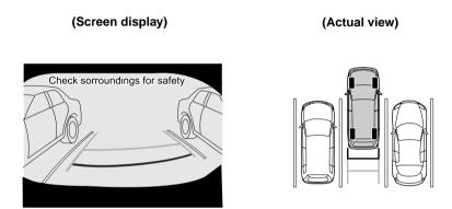
6. When the shift lever is shifted from R to another shift lever position, the screen returns to the previous display.
