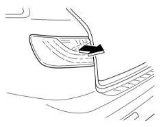
3. Turn the socket and bulb assembly counterclockwise and remove it.
