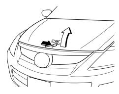
Grasp the support rod in the padded area and secure it in the stay hole indicated by the arrow to hold the hood open.
