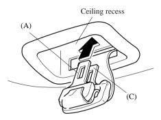
To pull out the seat belt, press the area indicated in the figure upward with your finger and slide the belt forward. Then slowly pull out the seat belt from the ceiling recess.
