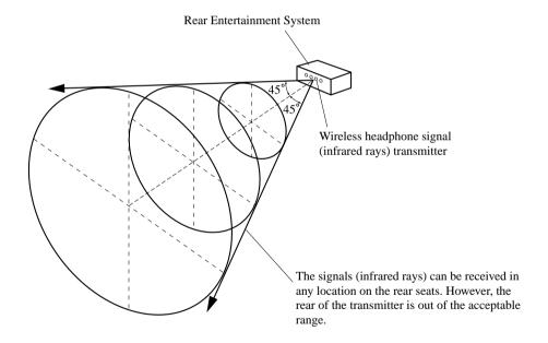
A wireless headphone can be used in any position on the rear seats, however, the sound may skip under the following conditions because the acceptable range varies or the signals are blocked.
