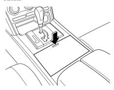
To fit small items in the cup holder, remove the flexible divider.
