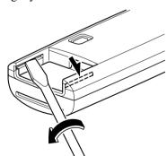
Insert the flathead screwdriver into the gap between the cover and the transmitter, and then rotate the screwdriver to detach the cover.
