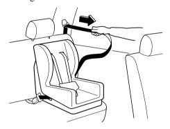
7. Push the child-restraint system firmly into the vehicle seat. Be sure the belt retracts as snugly as possible. A clicking noise from the retractor will be heard during retraction if the system is in the automatic locking mode. If the belt does not lock the seat down tight, repeat this step.
