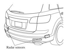
Always keep the bumper surface near the radar sensor area clean so that the BSM system operates normally. Refer to the Exterior Care (page 8-56).
