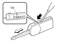
3. Insert a screwdriver into the slot and gently pry open the transmitter.
