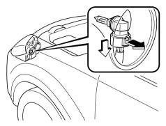
6. Turn the socket and bulb assembly to remove it. Carefully remove the bulb from its socket in the reflector by gently pulling it straight backward out of the socket.
