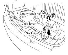
5. Slowly turn the lug wrench counterclockwise until the spare tire reaches the ground and the cable becomes loose.
