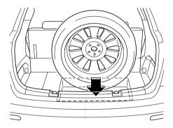
11. Thread the belt through the wheel as shown in the figure, then attach the belt clips to the attachment loop.
