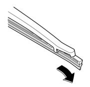
4. Remove the metal stiffeners from each blade rubber and install them in the new blade.
