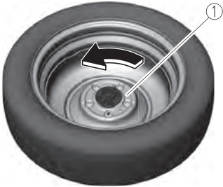
1. Spare tire hold-down bolt
