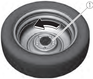
1. Spare tire hold-down bolt
