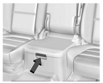
If equipped with front center seat storage, unlock with the mechanical key in the remote key, press the latch, and lift to open. See *Keys* ⇒ 13.
