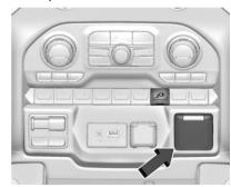
In Cab Power Outlet and DC/AC Switch
