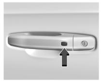
If equipped, the remote key must be within 1 m (3 ft) of the tailgate or door being opened or locked. Press the button on the door handle to open. See "Keyless Access Operation" in Remote Key Operation ▷ 14.
