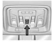
If equipped, the power sliding rear window works when the ignition has been turned on or to accessory mode, or Retained Accessory Power (RAP) must be active. See Retained Accessory Power (RAP) ⇒ 220.
