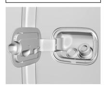
The capless refueling system does not have a fuel cap. Fully insert and latch the fill nozzle, begin fueling.
