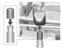
If the vehicle is equipped with a jack lift head adapter (6), fit the adapter over the end of the jack lift head. The adapter should have a snug fit. Check for proper fit between adapter and lift head, then position the jack under the bracket attached to the vehicle's frame, behind the flat tire, as shown.
