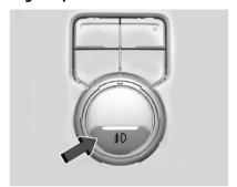
If equipped, the fog lamp control is near the exterior lamp control to the left of the steering column.
