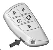
The engine may be started from outside the vehicle using the remote key. Press  $(x_2)$  twice. See *Remote Start*  $\Rightarrow$  20.
