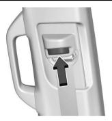
Push the release button to move the height adjuster to the desired position.
