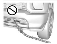
If equipped, there are recovery hooks at the front of the vehicle. Use them if the vehicle is stuck off-road and needs to be pulled some place to continue driving.
