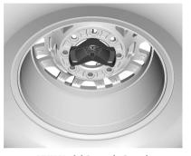
AT4X Model Correctly Stored, Retainer Centered
