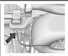
If equipped with a spare tire cable, reattach the clip to the frame attachment bracket. Note that there may be slack in the cable.
