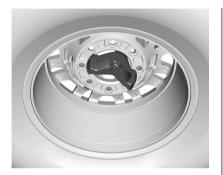
AT4X Model Incorrectly Stored, Retainer Off-Center
