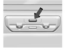
The MultiPro inner tailgate may be equipped with an enable/disable feature to prevent the inner tailgate from being opened when a hitch or other equipment is installed that could damage the inner tailgate.
