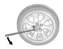
Use the wheel wrench and turn it counterclockwise to loosen the wheel nuts.
