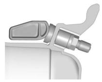
Contact your trailer service center or tire service center to have the pressure sensors installed inside the trailer tires. The technician should insert the sensor stem through the hole in the trailer wheel. When the sensor is correctly positioned, the nut on the sensor stem should be tightened to 8 N•m(6 lb ft). When mounting the trailer tire onto the trailer wheel be careful not to damage the sensor.
