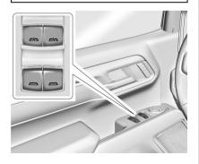
The power windows work when the vehicle is on, in accessory mode, or when Retained Accessory Power (RAP) is active. See *Retained Accessory Power (RAP)* ⇔ 220.
