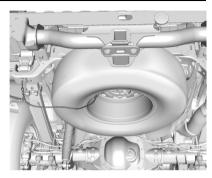
AT4X Model Only Valve Stem Side Up
