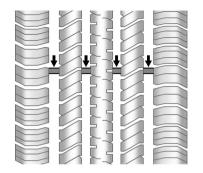
Treadwear indicators are one way to tell when it is time for new tires. Treadwear indicators appear when the tires have only 1.6 mm (1/16 in) or less of tread remaining. See *Tire Inspection* ⇔ 359 and *Tire Rotation* ⇔ 359.
