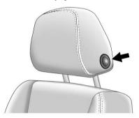
To raise or lower the head restraint, press the button on the side of the head restraint and pull up or push the head restraint down and release the button.
