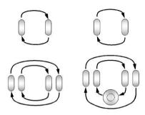
Use this rotation pattern when rotating the tires if the vehicle has polished forged aluminum dual rear wheels. The spare wheel can be used in any position in the event of a flat tire, and can be rotated with the rear inner wheels. After the flat tire is repaired, if the spare is not on one of the inner rear positions, it must be replaced by the correct wheel in the front or rear outer positions.
