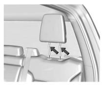
Insert the head restraint or headrest posts into the holes in the top of the seatback. The notches on the posts must face the driver side of the vehicle.
