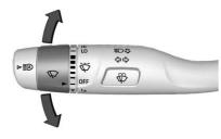
The windshield wiper control is on the turn signal lever.
