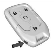
If the vehicle has the Keyless Access system, the transmitter has a button on the side of the transmitter used to remove the key. This key is used for the driver door and glove box.
