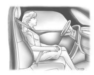
If a person of adult size is sitting in the front outboard passenger seat, but the OFF indicator is lit, it could be because that person is not sitting properly in the seat or that the child restraint locking feature is engaged. Use the following steps to allow the system to detect that person and enable the front outboard passenger frontal airbag:
