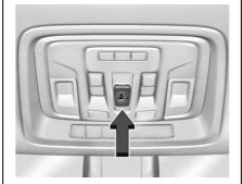
If equipped, the power sliding rear window works when the ignition has been turned on or to ACC/ACCESSORY, or Retained Accessory Power (RAP) must be active. See Retained Accessory Power (RAP) ⇒ 236.
