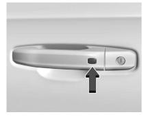
If equipped, the remote key must be within 1 m (3 ft) of the tailgate or door being opened or locked. Press the button on the door handle to open. See "Keyless Access Operation" in Remote Keyless Entry (RKE) System Operation (Key Access) \$\Display\$ 11 or Remote Keyless Entry (RKE) System Operation (Keyless Access) \$\Display\$ 13.
