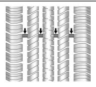
Treadwear indicators are one way to tell when it is time for new tires. Treadwear indicators appear when the tires have only 1.6 mm (1/16 in) or less of tread remaining. See *Tire Inspection* ⇔ 354 and *Tire Rotation* ⇔ 354 for additional information.
