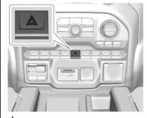
\(\to \): Press this button to make the front and rear turn signal lamps flash on and off. Press again to turn the flashers off.
