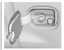
The capless refueling system does not have a fuel cap. Fully insert and latch the fill nozzle, begin fueling.
