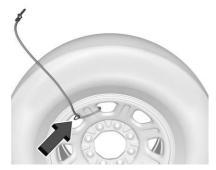
If equipped with a spare tire cable, reinstall the cable to the spare wheel by looping the cable around a wheel vent window then pass the clip end of the
