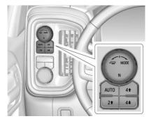
To activate Tow/Haul Mode turn the knob counterclockwise. To activate other drive modes turn the knob clockwise.
