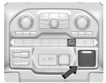
In Cab Power Outlet and DC/AC Switch
