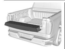
To open the inner tailgate, press the upper touch pad on the tailgate handle after unlocking all doors. Pull the top of the tailgate to open.
