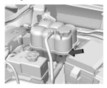
Check to see if coolant is visible in the coolant surge tank. If the coolant inside the coolant surge tank is boiling, wait until it cools down. The coolant level should be at or above the indicated mark. If it is not, there may be a leak in the cooling system.
