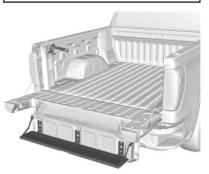
• To lower the tailgate step, press the button at the center of the step. Make sure it lowers to the fully open position. To close the tailgate step, lift it firmly.
