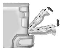
To close the tailgate using the lift-to-close feature, lift the tailgate from the full-open position to at least 10 cm (4 in) and hold it momentarily. Then, the tailgate will start closing automatically. If the tailgate is lifted more than halfway between open and close, then it will not close automaticallu.
