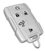
$\Omega$ : Press and release  $\widehat{\Omega}$ , then immediately press and hold  $\Omega$  until the turn signal lamps flash or for at least four seconds. The engine may be started from outside the vehicle using the RKE transmitter. See Remote Vehicle Start  $\Rightarrow$  20.
