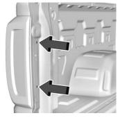
2. Remove the two rear lamp assembly screws.
