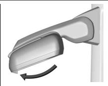
**Manual Extend:** If equipped, grasp the mirror housing firmly and pull back in one motion, arching slightly toward the rear of the vehicle.
