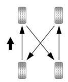
Use this rotation pattern when rotating the tires if the vehicle has single rear wheels.
