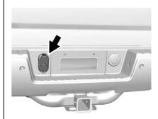
For vehicles equipped with heavy-duty trailering, the harness connector is mounted in the bumper.
