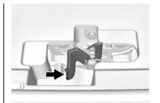
Go to the front of the vehicle to find the secondary hood release. The handle is under the front edge of the hood near the center. Push the handle to the right and at the same time raise the hood.
