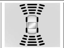
The instrument cluster may have a parking assist display with bars that show "distance to object" and object location information for the Parking Assist system. As the object gets closer, more bars light up and the bars change color from yellow to amber to red.
