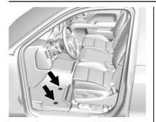
Reinstall by lining up the floor mat retainer openings over the carpet retainers and snapping into position.
