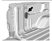
For vehicles with the fifth wheel/ gooseneck trailer package, the harness connector is mounted on the inside of the pickup bed behind the rear wheel.
