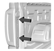
2. Remove the two rear lamp assembly screws.
