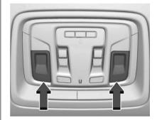
Press the lamp lenses to turn the front reading lamps on or off.
