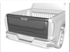
Switches in the inner tailgate prevent the primary tailgate from being opened when the inner tailgate is not fully closed.
