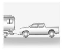
Only dinghy tow four-wheel-drive vehicles with a two-speed transfer case that have an N (Neutral) and a 4 \( \dagger (Four-Wheel Drive Low) setting.
