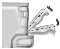
To close the tailgate using the lift-to-close feature, lift the tailgate from the full-open position to at least 10 cm (4 in) and hold it momentarily. Then, the tailgate will start closing automatically. If the tailgate is lifted more than halfway between open and close, then it will not close automatically.
