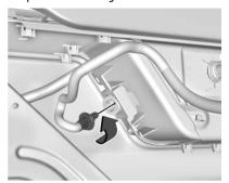
3. Replace the bulb and reverse Step 2 to reinstall.
