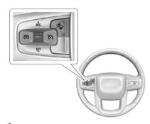
\*©: Press to turn the system on or off. The indicator turns white on the instrument cluster when ACC is turned on.
