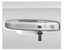
If equipped, the remote key must be within 1 m (3 ft) of the tailgate or door being opened or locked. Press the button on the door handle to open. See "Keyless Access Operation" in Remote Key Operation
