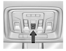
If equipped, the power sliding rear window works when the ignition has been turned on or to accessory mode, or Retained Accessory Power (RAP) must be active. See Retained Accessory Power (RAP) ⇒ 222.
