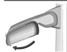
If equipped, grasp the mirror housing firmly and pull back in one motion, arching slightly toward the rear of the vehicle.
