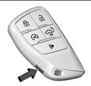
If the vehicle has the Keyless Access system, the remote key has a button on the side of the remote key used to remove the mechanical key.
