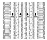
Treadwear indicators are one way to tell when it is time for new tires. Treadwear indicators appear when the tires have only 1.6 mm (1/16 in) or less of tread remaining. See *Tire Inspection* ♀ 392 and *Tire Rotation* ♀ 392.
