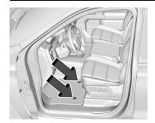
Reinstall by lining up the floor mat/liner retainer openings over the carpet retainers and snapping into position.
