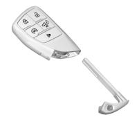
Press the button to remove the mechanical key. Never pull the mechanical key out without pressing the button.
