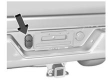
If equipped, the trailer wiring harness, with a seven-pin connector and a four-pin connector, is mounted on the vehicle's rear bumper.
