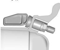
Contact your trailer service center or tire service center to have the pressure sensors installed inside the trailer tires. The technician should insert the sensor stem through the hole in the trailer wheel. When the sensor is correctly positioned, the nut on the sensor stem should be tightened to 8 N•m(6 lb ft). When mounting the trailer tire onto the trailer wheel be careful not to damage the sensor.
