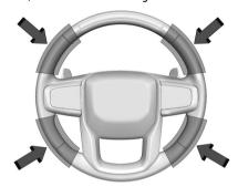
To begin steering manually, hold the steering wheel firmly with both hands using the highlighted regions.
