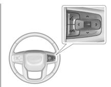
or : Press to move left or right between the interactive display zones in the instrument cluster. Press the thumbwheel to select.
