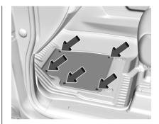
Reinstall by lining up the floor liner insert button clips over the liner retainers and snapping into position.
