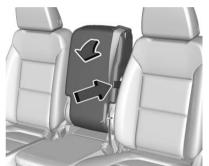
Pull the strap on the side of the center seatback to fold the center seatback. Do not use the center seatback as a seating position when the seatback is folded down.
