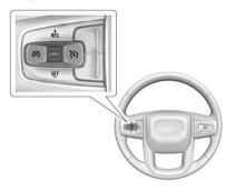
: Press to turn cruise control on or off. A white indicator light comes on in the instrument cluster when cruise control is turned on.
