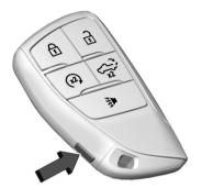
Press and release , then immediately press and hold until the turn signal lamps flash or for at least four seconds. The engine may be started from outside the vehicle using the remote key. See *Remote Start* 20.
