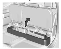
There may be storage under the rear passenger seat. Lift up on the seat bench to access. Push the seat bench toward the floor to close.
