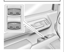
The power windows work when the vehicle is on, in accessory mode, or when Retained Accessory Power (RAP) is active. See *Retained Accessory Power (RAP)* ⇔ 222.
