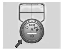
The exterior lamp controls are on the instrument panel to the left of the steering wheel.
