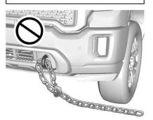
If the vehicle has recovery hooks at the front of the vehicle, use them if the vehicle is stuck off-road and needs to be pulled some place to continue driving.
