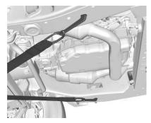
The vehicle is equipped with specific attachment points to be used to pull the vehicle onto a flatbed car carrier from a flat
