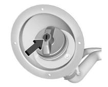
Use the fuel cap key to unlock the fuel cap then turn the fuel cap counterclockwise to remove. Fully insert and latch the fill nozzle, begin fueling.
