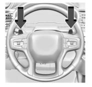
Electronic Range Select (ERS), or Manual Mode, allows for the selection of the range of gear positions. Use this mode when driving downhill or towing a trailer to limit the top gear and vehicle speed. The shift position indicator within the Driver
