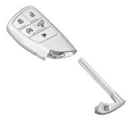
Remove the key by pressing the button on the side of the remote key near the bottom and pull the key out. Never pull the key out without pressing the button. See your dealer if a new remote key is needed.
