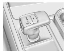
The shift pattern is displayed on the top of the shift lever. The selected gear position illuminates red on the shift lever, while all others will be displayed in white. If the shift is not immediate, as in very cold conditions, the indicator on the shift switch may blink until it is fully engaged. The shift lever always starts from a center position, represented by an up/down arrow on the shift pattern. After releasing the shift lever, it will return to the center position.
