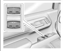
The power windows work when the ignition is on, in accessory mode, or when Retained Accessory Power (RAP) is active. See Retained Accessory Power (RAP) ⇒ 219.
