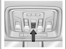
If equipped, the power sliding rear window works when the ignition has been turned on or to accessory mode, or Retained Accessory Power (RAP) must be active. See Retained Accessory Power (RAP) ⇒ 219.
