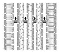
Treadwear indicators are one way to tell when it is time for new tires. Treadwear indicators appear when the tires have only 1.6 mm (1/16 in) or less of tread remaining. See *Tire Inspection* ⇔ 384 and *Tire Rotation* ⇔ 385.
