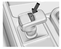
**P**: This position locks the rear wheels. Use P (Park) when starting the engine to prevent the vehicle from moving easily.
