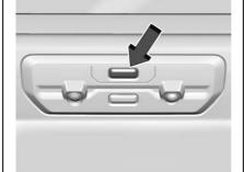
The MultiPro inner tailgate may be equipped with an enable/disable feature to prevent the inner tailgate from being opened when a hitch or other equipment is installed that could damage the inner tailgate.
