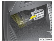
To engage the parking brake, first apply the foot brake and then depress the parking brake pedal down as far as possible.
