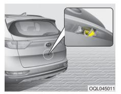
Press the liftgate handle switch carrying the smart key with you.
