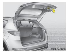
To close the liftgate, lower and push down the liftgate firmly. Make sure that the liftgate is securely latched. Make sure your hands, feet and other parts of your body are safely out of the way before closing the liftgate.
