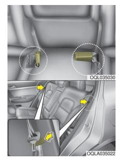
Insert the rear seat belt buckle in the pocket between the rear seatback and cushion, and insert the rear seat belt webbing in the guide to prevent the seat belt from being damaged.
