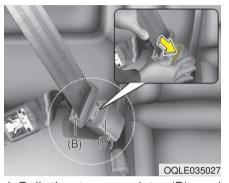
Pull the tongue plate (B) and insert it into the buckle (B') until an audible "click" is heard, indicating the latch is locked. Make sure the belt is not twisted.
