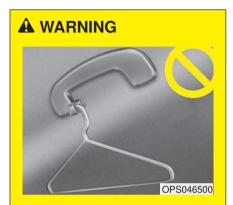
Do not hang other objects such as hangers or hard objects except clothes. Also, do not put heavy, sharp or breakable objects in the clothe pockets. In an accident or when the curtain air bag is inflated, it may cause vehicle damage or personal injury.
