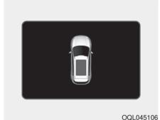
· The warning message illuminates if you turn off the engine and then open the driver's door when the sunroof is open.
