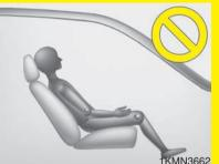
The driver must advise the passengers to keep the seatback in an upright position whenever the vehicle is in motion. If a seat is reclined during an accident, the restraint system's ability to restrain will be greatly reduced.
