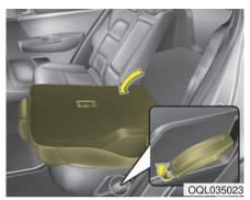
4. Lift up the front portion of the seatback folding lever, then fold the seat toward the front of the vehicle. When you return the seatback to its upright position, always be sure it has locked into position by pushing on the top of the seatback.
