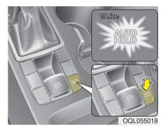
1. Depress the brake pedal, start the engine and then press the Auto Hold button. The white AUTO HOLD indicator will come on indicating the system is in standby. Before the Auto Hold will engage, the driver's door, engine hood must be closed and the driver's seat belt must be fastened.
