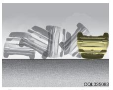
Front air bags may not inflate in all rollover accidents where the SRSCM indicates that the front air bag deployment would not provide additional occupant protection.
