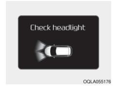
This warning message illuminates if there is a malfunction (burned-out bulb except LED lamp or circuit malfunction) with the headlamp. In this case, have your vehicle inspected by
