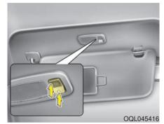
Push the switch to turn the light on or off.
