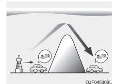
AM broadcasts can be received at greater distances than FM broadcasts. This is because AM radio waves are transmitted at low frequencies. These long distance,low frequency radio waves can follow the curvature of the earth rather than travelling straight. In addition, they curve around obstructions resulting
