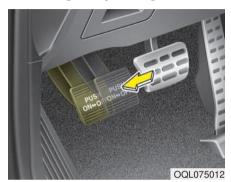
Check whether the stroke is within specification when the parking brake pedal is depressed with 20 kg (44 lbs, 196 N) of force. Also, the parking brake alone should securely hold the vehicle on a fairly steep grade. If the stroke is more or less than specified, have the parking brake adjusted by an authorized Kia dealer.
