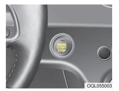
Whenever the front door is opened, the ENGINE START/STOP button will illuminate for your convenience. The light will go off after about 30 seconds when the door is closed.
