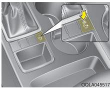
This system will activate when the indicator on the rear parking assist OFF button is not illuminated. If you desire to deactivate the rear parking assist system, press the rear parking assist OFF button again. (The indicator on the button will illuminate.) To turn the system on, press the button again. (The indicator on the button will go off.) If the vehicle is moving at a speed over 5 km/h (3 mph), the system may not be activated correctly.
