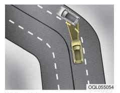
While driving on a curve, the AEB may recognize the vehicle in front in the next lane and it produces the warning message and activates as a result. Exercise caution, and, if necessary, depress the brake pedal.
