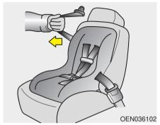
3. Pull the shoulder portion of the seat belt all the way out. When the shoulder portion of the seat belt is fully extended, it will shift the retractor to the "Automatic Locking" (child restraint) mode.
