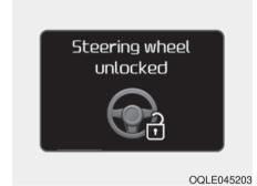
This warning message illuminates if the steering wheel does not lock when the Engine Start/Stop Button changes to the OFF position.
