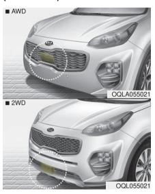
The sensor is to maintain a certain distance from the vehicle in front. However, the smudged sensor or sensor cover with foreign substances, such as snow and rain, adversely affects the sensing performance.
