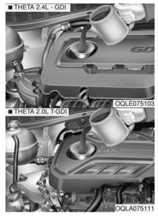
If it is near or at L, add enough oil to bring the level to F. **Do not overfill.**
