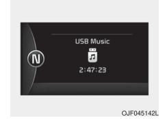
This mode displays the state of the A/V system.
