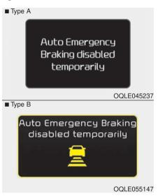
When the sensor is covered or the sensor is dirty with foreign substances, such as snow or rain, the AEB operation may temporarily stop. In this case, a warning message will appear to notify the driver.
