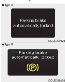
If the EPB is applied while Auto Hold is activated because of ESC (Electronic Stability Control) signal, a warning will sound and a message will appear.
