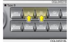
The fan speed can be set to the desired speed by operating the fan speed control button.
