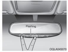
1. When programming the buttons for the first time, press and hold the left and center buttons (中, 1) simultaneously until the indicator light begins to flash after approximately 20 seconds. (This procedure erases the factory-set default codes. Do not perform this step when programming the additional HomeLink buttons.)
