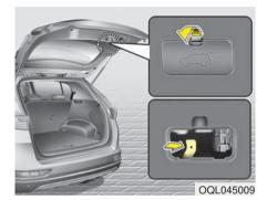
Your vehicle is equipped with an emergency liftgate safety release lever located on the bottom of the liftgate. When someone is inadvertently locked in the cargo area, the liftgate can be opened by pushing the release lever and pushing open the liftgate.
