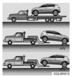
If emergency towing is necessary, we recommend having it done by an authorized Kia dealer or a commercial tow-truck service. Proper lifting and towing procedures are necessary to prevent damage to the vehicle. The use of wheel dollies or flatbed is recommended.
