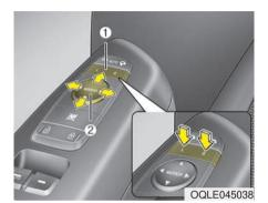
The electric remote control mirror switch allows you to adjust the position of the left and right outside rearview mirrors. To adjust the position of either mirror, press the R or L button (1) to select the right side mirror or the left side mirror, then press a corresponding point (▲) on the mirror adjustment control to position the selected mirror up, down, left or right.
