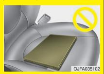
Do not put an electronic device (ex. Laptop computer, after market DMB, navigation, satellite audio, video game machine, MP3, AC inverter, etc.) in the front passenger seatback pocket or on the front passenger seat.
