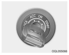
The ignition key can be removed only in the LOCK position.
