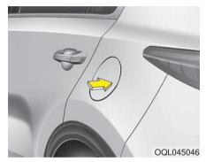
To open the fuel filler lid, press the 3 o`clock position edge of the fuel filler lid.
