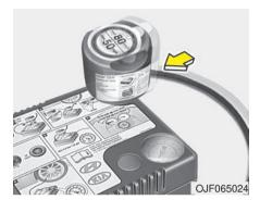
5. Insert the sealant bottle into the housing of the compressor (5) so that the bottle is upright.
