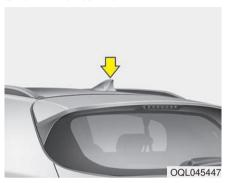
The shark fin antenna will receive the AM, FM broadcast signals and transmit data.
