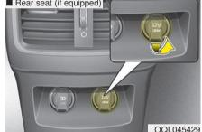
The power outlet is designed to provide power for mobile telephones or other devices designed to operate with vehicle electrical systems. The devices should draw less than 10 amps with the engine running.
