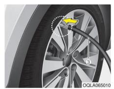
4. Unscrew the valve stem cap from the flat tire and screw the filling hose (3) of the sealant bottle onto the valve stem.
