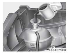
If the coolant level is low, add enough specified coolant to provide protection against freezing and corrosion. Bring the level to MAX, but do not overfill. If frequent additions are required, see an authorized Kia dealer for a cooling system inspection.
