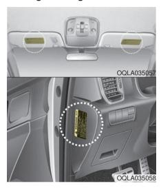
Air bag warning labels, some required by the Canada Motor Vehicle Safety Standards (CMVSS), are attached to the sunvisor to alert the driver and passengers of potential risks of the air bag system.
