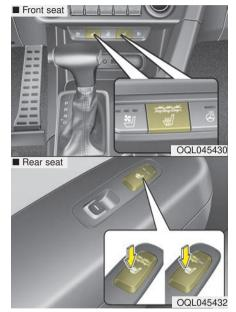
The seat warmer is provided to warm the front seats during cold weather. With the ignition switch in the ON position, push either of the switches to warm the driver's seat or the front passenger's seat.
