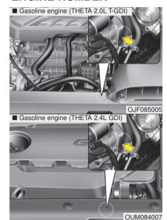
The engine number is stamped on the engine block as shown in the drawing.
