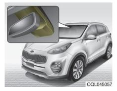
Auto defogging reduces the probability of fogging up the inside of the windshield by automatically sensing the moisture of inside the windshield. The auto defogging system operates when the heater or air conditioning is on.
