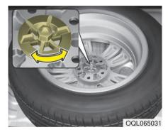
Turn the tire hold-down wing bolt counterclockwise.
