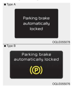
Parking brake automatically locked When the EPB is applied from Auto Hold, a warning will sound and a message will appear.
