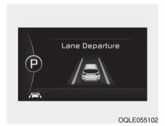
If the system detects that your vehicle is leaving the lane when the LDWS is operating and vehicle speed exceeds 64 km/h (40 mph), the warning operates as follows:
