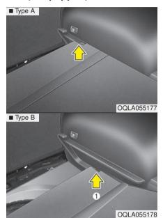
If the vehicle is equipped with a TMK (Tire Mobility Kit) or a temporary tire, you can make the luggage board to flat (Type A) or lower (Type B) for more luggage storage.
