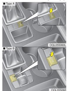
Engine power can be delivered to all front and rear wheels for maximum traction. AWD is useful when extra traction is required on road, such as, when driving on slippery, muddy, wet, or snow-covered roads. These vehicles are not designed for challenging off-road use.
