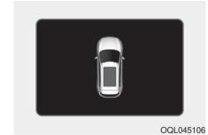
If the driver removes the ignition key (smart key: turns off the engine) when the sunroof is not fully closed, the warning chime will sound for a few seconds and a message will appear on the LCD display or the warning indicator will illuminate.
