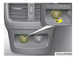
The USB charger is designed to recharge batteries of small size electrical devices using a USB cable. The electrical devices can be recharged when the Engine Start/Stop button is in ACC/ON/START position.
