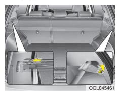
Use the cargo security screen to hide items stored in the cargo area. To use the cargo security screen, pull the handle backward and insert the edges into the slots.
