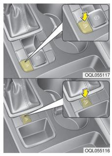
The Downhill Brake Control (DBC) supports the driver come down a steep hill without depressing the brake pedal.
