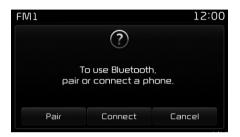
If Bluetooth® Wireless Technology devices are paired but none are currently connected, pressing the [PHONE] button or the [CALL] button on the steering wheel controls displays the following screen. Press the [Pair] button to pair a new device or press the [Connect] to connect a previously paired device.
