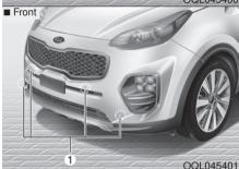
The parking assist system assists the driver during movement of the vehicle by chiming if any object is sensed within the distance of 100 cm (39 in.) in front and 120 cm (47 in.) behind the vehicle
