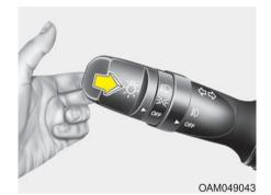
To flash the headlights, pull the lever towards you. It will return to the normal (low beam) position when released. The headlight switch does not need to be on to use this flashing feature.
