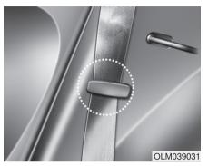
Routing the seat belt webbing through the rear seat belt guides will help keep the belts from being trapped behind or under the seats.
