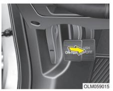
Releasing the parking brake Foot type
