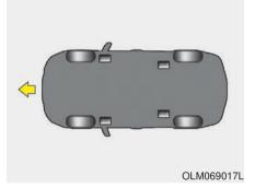
Tie-down hook (for flatbed towing, if equipped)
