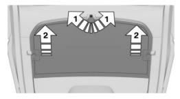
2. Pull the cargo cover up and out of the brackets, arrows 2.
