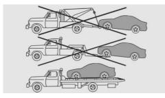
The vehicle should only be transported on a loading platform.
