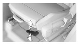
Pull the lever up or press it down as often as needed until the seat has reached the desired. inclination.
