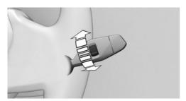
Turn the thumbwheel on the wiper lever.
