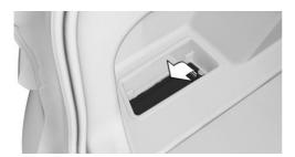
The onboard vehicle tool kit is located in the left storage compartment of the cargo area under a cover.
