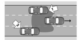
Radar sensors monitor the area behind and next to the vehicle when traveling faster than a minimum speed.
