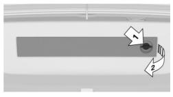
2. Push the warning triangle sideways to the left and remove it.
