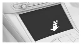
2. A socket is located between the cup holders. Detach the cover.
