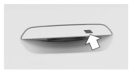
Touch the grooved surface on the external door handle of a closed door with your finger
