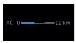
The shaded area indicates a limitation in the charging capacity that can occur, for instance due to the connected charging infrastructure.
