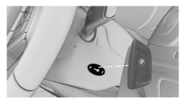
It is not possible to switch on the drive-ready state if the vehicle key has not been detected.
