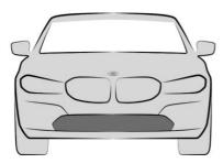
The front radar sensor is located in the front bumper.
