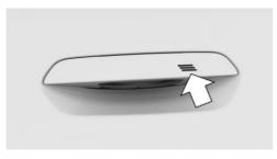
Touch the grooved surface on the external door handle of a closed door with your finger and hold it there without grasping the recessed grip.
