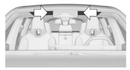
With climate comfort windshield: the marked area is not covered with heat-reflective coatina.
