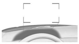
Head-up display views are projected onto the windshield using protective glass. The protective glass is located between the steering wheel and windshield.
