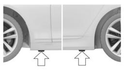
The jacking points are located at the indicated positions.
