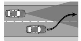
If a vehicle driving ahead of you suddenly merges into your lane, the system may not be able to automatically restore the selected distance. It may not be possible to restore the selected distance in certain situations, including if you are driving significantly faster than vehicles driving ahead of you, for instance when rapidly
