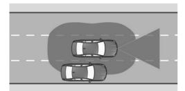
Radar sensors monitor the space next to the vehicle when traveling faster than a minimum speed and up to approx. 130 mph/210 km/h.
