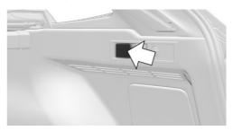
Depending on vehicle equipment, there is a socket in the cargo area on the right side. Unfold the cover.
