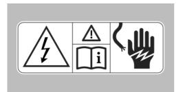
These icons found on parts of the vehicle indicate that incorrect use of high-voltage technology or of orange-colored high-voltage components poses a risk of life-threatening injury by electric shock.
