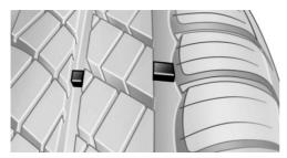
The tire manufacturer's wear indicators are distributed over the tire circumference. These indicators have a height of min. 0.06 in/1.6 mm and serve as an indicator for tire tread wear.
