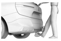
Moving a foot again will stop the opening proccedure. The subsequent foot movement will close the cargo area again.
