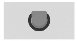
There are several lashing eyes in the cargo area for securing cargo. Attach auxiliary materials to secure the cargo such as lashing straps, tensioning straps, draw straps, or cargo nets to the lashing eyes.
