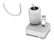
Let the compressor run for a maximum of 10 minutes to fill in the tire sealant and reach a tire pressure of approx. 2 bar/29 psi.
