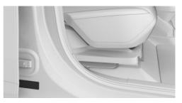
The vehicle identification number can be found on the nameplate, on the right-hand side of the vehicle.
