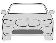
The radar sensor is located in the area shown.
