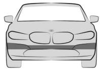
The ultrasonic sensors of the parking assistance systems are located in the area shown.
