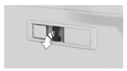
Fold down the multifunction hook until it noticeably engages in the lower position.
