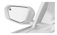
The light in the exterior mirror flashes if vehicles are detected by the rear sensors and your own vehicle is moving in reverse.
