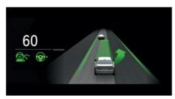
An example with active Driver Assistance: the indicator and warning lights for the distance control and the Automatic Lane Change Assistant indicate a lane change to the next lane. At the same time, the lane change to the next lane is shown with animation in the Assisted View.
