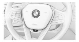
Button for steering wheel heating
