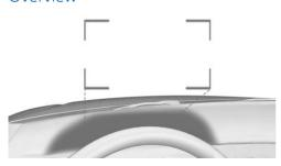
The protective glass of the Head-up display is located between the steering wheel and the windshield.
