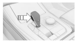
3. Push the selector lever in the desired direction, past a resistance point, if needed. The selector lever automatically returns to the center position when released.
