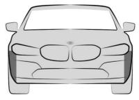
The radar sensors are located in the areas shown.
