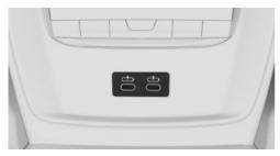
Depending on the equipment, there are two USB ports in the center console in the rear. Properties:
