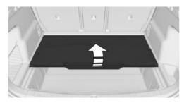
To move the cargo area floor into the foldedup position, fold up the cargo area floor that was folded down at the front.
