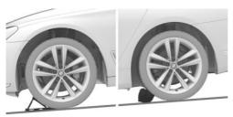
If you need to change a wheel on a slight downhill grade, place chocks and other suitable objects, for instance rocks, under the proper side of the wheels of both the front and rear axles to block the car from rolling downhill.
