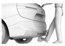
Before the cargo area opens, the hazard warning system flashes.
