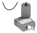
2. Switch off the compressor when you reach a tire pressure of 2.5 bar/36 psi.
