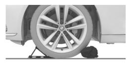
Place wheel chocks or other suitable objects in front and behind the wheel that is diagonal to the wheel being changed.
