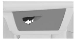
Pull the handle on the glove compartment.
