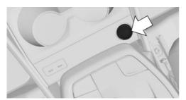
A socket is provided on the front center console under a cover. Pull off the cover before using the socket.
