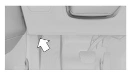
The diagnostic socket for reading out vehicle data is located on the driver's side.
