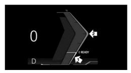
Needle in lower range of arrow 1: display for energy recovery such as while decelerating, CHARGE.
