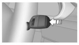
Press the button on the wiper lever.
