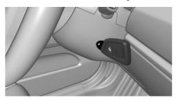
It is not possible to start the engine if the vehicle key has not been detected.
