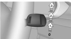
To activate: press the lever up once from its standard position, arrow 1.
