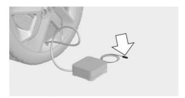
5. With the ignition switched on or the engine running, switch on the compressor.
