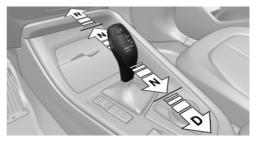
The selector lever positions R, N, and D are selected by tapping the selector lever forward or back. The selector lever automatically returns to the center position when released.
