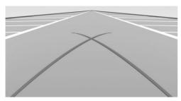
Turning radius lines can only be superimposed on the rearview camera image together with lanes.
