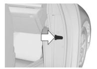
Side door lock for manually locking the doors.
