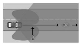
The sensors detect the traffic situation in their detection range on a straight road.
