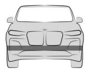
The ultrasonic sensors are located in the front bumper.
