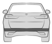
The ultrasonic sensors are located in the rear bumper.
