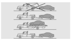
The vehicle should be transported with a tow truck with a so-called spectacle lift or on a loading platform.
