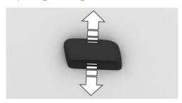
To adjust the seat height, press the seat height switch up or down.
