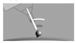
Two static circle segments are displayed in the camera image. These circle segments help to estimate the distance of the trailer to the trailer hitch.
