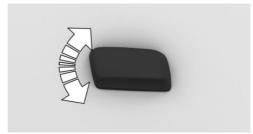
To adjust the seat tilt, flip the seat tilt switch up or down.
