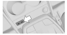
Two USB ports are located on the front center console.
