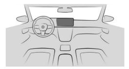
The control display is located on the instrument panel above the center console.
