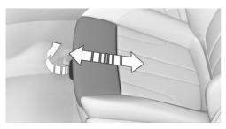
To adjust the thigh support, pull the thigh support lever at the front of the seat then push the thigh support forward or backward.
