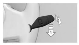
To turn off the wiper system, push the wiper lever down until it reaches position 0, arrow 1.
