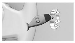
To turn on the rear wiper, rotate the outer switch on the wiper lever upward.
