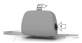
Press the button and fold the head restraint back, arrow 1.
