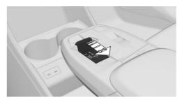
To activate the Sport program, pull the selector lever from selector lever position D to D/S.
