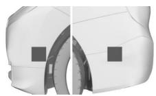
The ultrasonic sensors are located on the sides of the front and rear bumpers.
