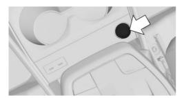
A socket is provided on the front center console under a cover. Pull off the cover before using the socket.
