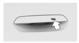
To close the glass sunroof using the door handle of a closed front door, place a finger on the grooved surface of the door handle and hold it there without reaching into the recessed grip.
