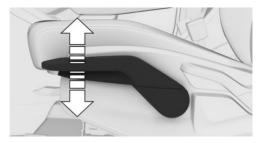
To adjust the height: On the side of the seat, push the front seat height lever up or down as many times as necessary for the seat to reach the desired height.
