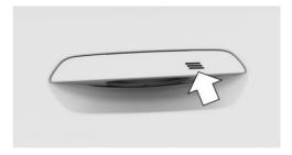
To close a window using the door handle of a closed front door, place a finger on the grooved surface of the door handle and hold it there without reaching into the recessed grip.
