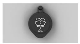
The washer fluid reservoir is located in the engine compartment on the right side of vehicle.
