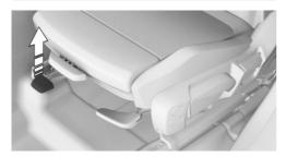
To adjust the longitudinal direction, pull up the longitudinal direction lever at the front of the seat and push the seat in the desired direction.
