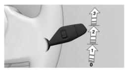
To activate the rain sensor: Push the wiper lever upward from position 0, arrow 1, once. Wiping operation is started.
