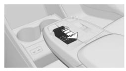
To activate LOW mode, pull the selector lever from selector lever position D to D/L.
