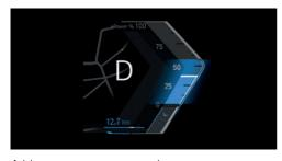
A blue range appears on the power gauge, indicating reduced consumption while driving.
