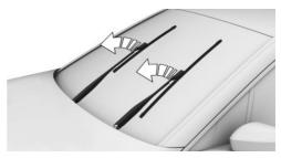
3. Press the button on the wiper, arrow 1, turn the wiper blade clockwise slightly, then pull it forward and out, arrow 2.
