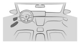
The central locking buttons are located on the front door.
