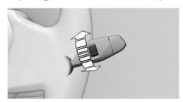
To adjust the sensitivity of the rain sensor, turn the thumbwheel on the wiper lever.
