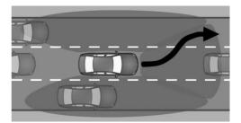
The sensors monitor and detect the clearance in front of the vehicle. Depending on the vehicle equipment, the areas next to the vehicle are also monitored.
