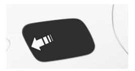
2. Open the fuel filler cap counterclockwise.
