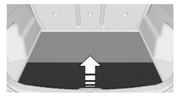
To open the storage compartment, grasp the rear edge of the cargo area floor and fold it forward.
