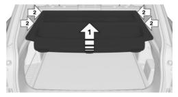
3. Firmly pull the cover backward out of the brackets, arrows 2.
