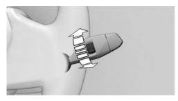
To adjust the sensitivity of the rain sensor, turn the thumbwheel on the wiper lever as follows:
