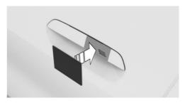
Hold the activated Service Card directly over the middle of the driver's door handle.
