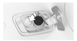
3. Place the fuel filler cap in the bracket on the fuel filler flap.
