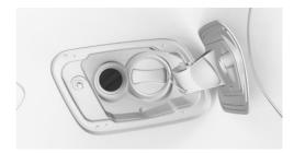
The fuel cap for diesel exhaust fluids is next to the fuel cap for the fuel tank.
