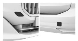
Press on the mark on the edge of the cover to push it out.
