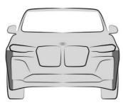
The radar sensors are located to the side in the front bumper.
