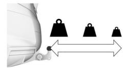
The permitted gross weight of the loaded rearmounted luggage rack depends on how far its center of gravity is from the ball head.
