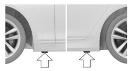
The jacking points are located at the indicated positions.
