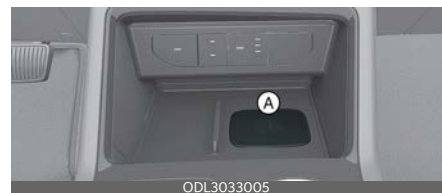
A: Charging pad
