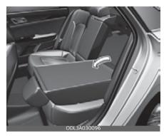
To use the rear seat, lift and pull the seatback rearward. Pull the seatback firmly until it clicks into place. Make sure the seatback is locked in place.
