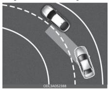
Blind-Spot Collision-Avoidance Assist may not operate properly when driving on a curved road. The function may not recognize a vehicle in the same lane.
