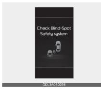
When Safe Exit Assist is not working properly, the 'Check Blind-Spot Safety system' warning message will appear on the cluster, and Safe Exit Assist will turn off automatically or it will be limited. In this case, have your vehicle inspected by an authorized Kia dealer.
