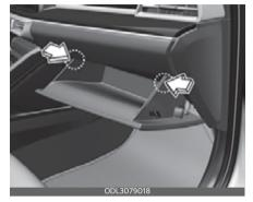
Remove the climate control air filter cover by pulling out right side of the cover.
