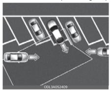
Rear Cross-Traffic Collision-Avoidance Assist may be limited, and may not detect the vehicle approaching from the left or right. If this occurs, the function may not warn the driver, or control the brakes when necessary. Always check your surroundings while backing up. Always check your surroundings while backing up.
