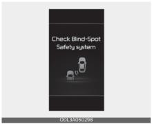
When Blind-Spot Collision-Avoidance Assist is not working properly, the 'Check Blind-Spot Safety system' warning message will appear on the cluster, and Blind-Spot Collision-Avoidance Assist will turn off automatically or Blind-Spot Collision-Avoidance Assist will be limited. In this case, have your vehicle inspected by an authorized Kia dealer.
