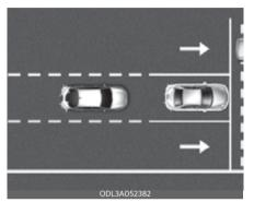
Forward Collision-Avoidance Assist is designed to help detect and monitor the vehicle ahead or help detect a pedestrian or cyclist in the roadway and warn the driver that a collision is imminent with a warning message and an audible warning, and if necessary, apply emergency braking.
