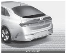
The wide-rear view camera (1) is used as a detecting sensor to detect pedestrians. If the camera lens is covered with foreign material, such as snow or rain, it may adversely affect camera performance and Reverse Parking Collision-Avoidance Assist may not operate normally. Always keep the camera lens clean.
