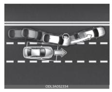
When changing lanes by detecting the lane ahead, if Blind-Spot Collision-Avoidance Assist judges that there is a collision risk with an approaching vehicle in the blind spot, it can help avoid collision by applying the brake.
