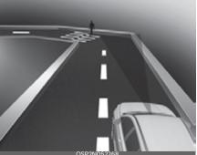
Forward Collision-Avoidance Assist may not detect other vehicle, pedestrian in front of you on curved roads adversely affecting the performance of the sensors. This may result in no warning or braking assist when necessary.
