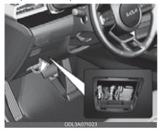
3. Pull the suspected fuse straight out.
