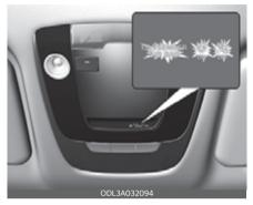
The ODS is designed to detect the presence of a properly-seated front passenger and determine if the passenger's front air bag should be enabled (may inflate) or not. Only the front passenger front air bag is controlled by the ODS. Do not put anything in front of the passenger air bag "\*\* indicator.
