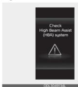
When High Beam Assist is not working properly, the 'Check High Beam Assist (HBA) system' warning message will appear and \(\bigai\) warning light will appear on the cluster. In this case, have the function inspected by an authorized Kia dealer.
