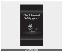
When Forward Collision-Avoidance Assist is not working properly, the 'Check Forward Safety system' warning message will appear, and the and and
