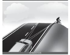
Forward Collision-Avoidance Assist may not detect other vehicle, pedestrian or cyclist in front of you while driving uphill or downhill adversely affecting the performance of the sensors.
