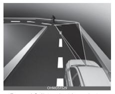
Forward Collision-Avoidance Assist may not detect other vehicle, pedestrian or cyclist in front of you on curved roads adversely affecting the performance of the sensors. This may result in no warning or braking assist when necessary.
