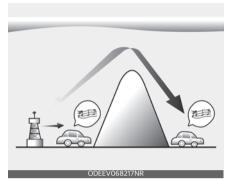
AM broadcasts can be received at greater distances than FM broadcasts. This is because AM radio waves are transmitted at low frequencies. These long distance, low frequency radio waves can follow the curvature of the earth rather than traveling straight. In addition, they curve around obstructions resulting in better signal coverage.
