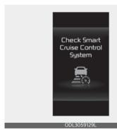
When Smart Cruise Control is not working properly, the 'Check Smart Cruise Control system' warning message will appear, and the / warning light will appear on the cluster. In this case, have your vehicle inspected by an authorized Kia dealer.
