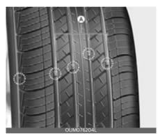
This shows there is less than 1/16 inches (1.6 mm) of tread left on the tire. Replace the tire when this happens.
