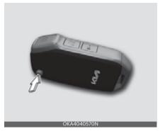
To unfold the key, press the release button then the key will unfold automatically.
