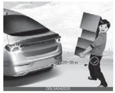
If you are positioned in the detecting area (20~39 inches (50~100 cm)) behind the vehicle carrying a smart key, the hazard warning lights will blink and chime will sound to alert you the smart key has been detected and the trunk will open.
