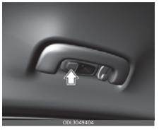
Press the switch to turn the room lamp on and off.
