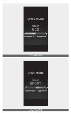
With the standard driving style in the center, the left side of the gauge is 'Econ.' and right side is 'Dynamic' style.
