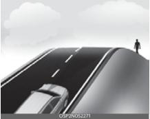
Forward Collision-Avoidance Assist may not detect other vehicle, pedestrian in front of you while driving uphill or downhill adversely affecting the performance of the sensors.
