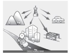
FM broadcasts are transmitted at high frequencies and do not bend to follow the earth's surface. Because of this, FM broadcasts generally begin to fade within short distances from the station. Also, FM signals are easily affected by buildings, mountains, and obstructions.
