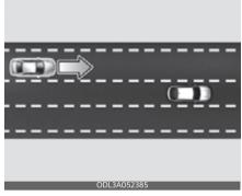
Blind-Spot Collision-Avoidance Assist help detect and informs the driver that a vehicle is approaching at high speed from the blind spot area.
