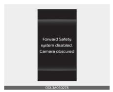
When the front windshield where the front view camera is located, is covered
