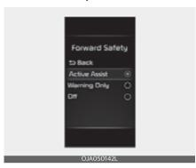
With the ENGINE START/STOP button in the ON position, select or deselect 'Driver Assistance → Forward Safety' from the Settings menu to set whether or not to use each function.
