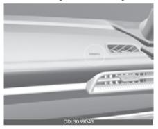
The indication of the system's presence are the letters "AIR BAG" located on the air bag pad cover and driver's knee area on the steering wheel and the passenger's side front panel pad above the glove box.
