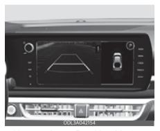
You can change Rear View Monitor settings by pressing the setup icon on the screen while the function is operating, or select 'Driver Assistance 6
