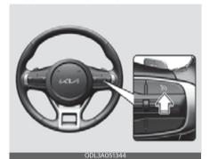
2. Release the accelerator pedal. The desired speed will automatically be maintained.
