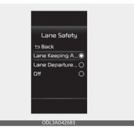
With the ENGINE START/STOP button in the ON position, select or deselect 'Driver Assistance → Lane Safety' from the Settings menu to set whether or not to use each function.
