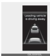
When the front vehicle departs from a stop, Leading Vehicle Departure Alert will inform the driver by displaying the 'Leading vehicle is driving away' message on the cluster and an audible warning will sound.
