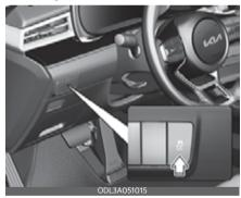
ESC applies the brakes on individual wheels and intervenes with the vehicle management system to stabilize the vehicle.
