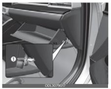
3. Push in both sides of the glove box as shown. This will ensure that the glove box stopper pins will get released from its holding location allowing the glove box to hang.
