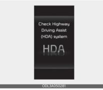
When Highway Driving Assist is not working properly, the 'Check Highway Driving Assist (HDA) system' warning message will appear, and the warning light will appear on the cluster. In this case, have your vehicle inspected by an authorized Kia dealer.
