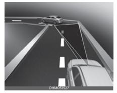
On curves, Smart Cruise Control may not detect a vehicle in the same lane, and may accelerate to the set speed. Also, vehicle speed may rapidly decrease when the vehicle ahead is detected suddenly.
