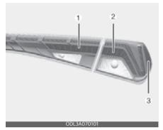
If the tail lamp (1), tail & stop lamp (2) and side marker lamp (3) does not operate, have the vehicle checked by an authorized Kia dealer.
