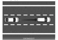
Highway Driving Assist is designed to help detect vehicles and lanes ahead, and help maintain distance from the vehicle ahead, maintain the set speed, and keep the vehicle between lanes while driving on the highway (or motorway).
