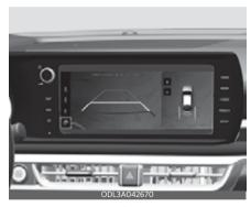
You can change Surround View Monitor settings by pressing the setup icon (♠) on the screen while the function is operating, or select "Setup → Vehicle (Infotainment System screen) → Driver Assistance → Parking Safety → Camera Settings' from the Settings menu in the Settings in the Infotainment System screen while the ENGINE START/STOP button is in the ON position.
