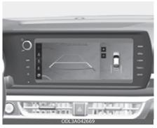
Surround View Monitor can assist with parking by allowing the driver to see around the vehicle.
