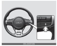
Each time the button is pressed, the Vehicle Distance changes as follows:
