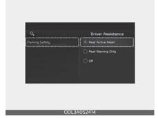
With the ENGINE START/STOP button in the ON position, select or deselect 'Driver Assistance → Parking Safety' from the Settings menu to set whether or not to use the function.
