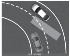
Blind-Spot Collision-Avoidance Assist may not operate properly when driving on a curved road. Blind-Spot Collision-Avoidance Assist may not detect the vehicle in the next lane.
