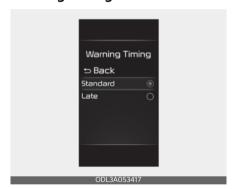
With the ENGINE START/STOP button in the ON position, select 'Driver Assistance → Warning Timing' from the Settings menu to change the initial warning activation time for Driver Attention Warning. When the vehicle is first delivered, Warning Timing is set to 'Standard'. If you change the Warning Timing, the warning time of other Driver Assistance systems may change.
