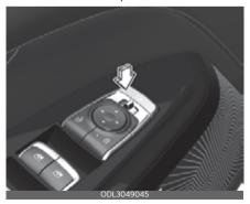
To fold the outside rear view mirror depress the button. • To unfold it, depress the button again.
