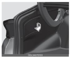
Remove the socket from the assembly by pressing it in and rotating it counterclockwise.
