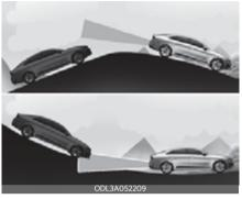
Blind-Spot Collision-Avoidance Assist may not operate properly when driving on a slope. Blind-Spot Collision-Avoidance Assist may not detect the vehicle in the next lane or may incorrectly detect the ground or structure. Always pay attention to road and driving conditions while driving.
