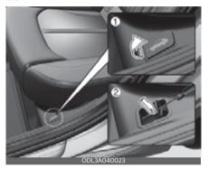
Open the cable cover(1) under the rear seat with a mechanical key and pull the cable (2) for unlocking the trunk. The cable is fixed firmly so it may hard to pull. Therefore, please use auxiliary equipment such as a screwdriver to grab the loop and pull it comfortably.
