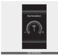
If the brightness reaches to the maximum or minimum level, an alarm will sound.
