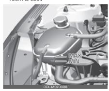
If the coolant level is low, add enough specified coolant to provide protection against freezing and corrosion. Bring the level to MAX, but do not overfill.
