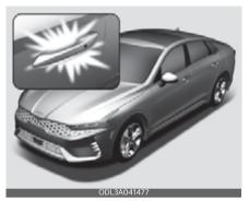
When all the doors (and trunk) are closed and locked, the door handle lamp will come on for about 15 seconds if any of the below is performed.
