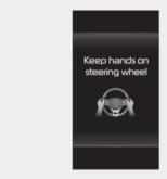
If the driver takes their hands off the steering wheel for several seconds, the 'Keep hands on the steering wheel' warning message will appear on the cluster, and an audible warning will sound in stages.
