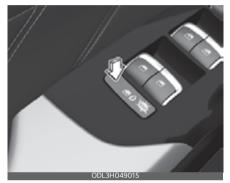
To cancel the electronic child safety lock system, push the electronic child safety lock system switch one more time and then the indicator turns off.
