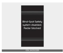
When the rear bumper around the rearside radar or sensor is covered with foreign matters, such as snow or rain, or installing a trailer or carrier, it can reduce the detecting performance and temporarily limit or disable Safe Exit Assist. If this occurs, the 'Blind-Spot Safety system disabled. Radar blocked' warning message will appear on the cluster.
