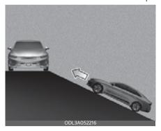
Rear Cross-Traffic Collision-Avoidance Assist may be limited when the vehicle is on, or near, a uphill or downhill slope, and may not detect the vehicle approaching from the left or right. If this occurs, the function may not warn the driver or control the brakes when necessary.
