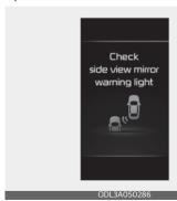
When the side view mirror warning light is not working properly, the 'Check side view mirror warning light' warning message will appear on the cluster. In this
