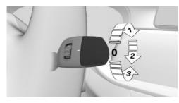
Turn the outer switch upward.
