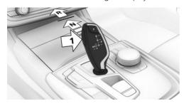
4. Release Start/Stop button and selector lever.
