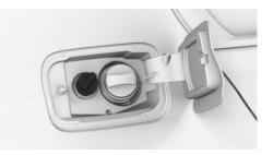
The fuel cap for diesel exhaust fluids is next to the fuel cap for the fuel tank.
