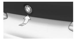
▶ Unlock the vehicle and then press the button on the outside of the tailgate.
