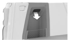
5. Loosen the screw and remove the holder.
