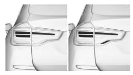
During normal brake application, the outer brake lights light up.
