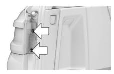
4. Open the cover on the side trim in the cargo area, arrow, and remove the warning triangle, refer to page 344.
