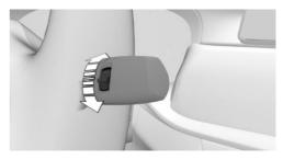
Turn the thumbwheel on the wiper lever.
