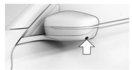
One camera is located at the bottom of each exterior mirror housina.
