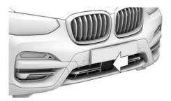
The radar sensor is located in the front bumper. Always keep radar sensor clean and unob-
