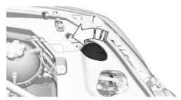
3. Pull the bulb holder out past the spring resistance point.
