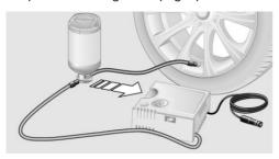
Screw the filling hose of the sealant container onto the tire valve of the defective wheel.
