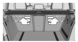
Reach under the cover and turn it upward, arrows. Pull the cover back horizontally.
