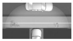
Side View provides an early look at cross traffic at blind driveways and intersections. Road users concealed by obstacles to the left and right of the vehicle can only be detected relatively late from the driver's seat. To improve the viewing, each camera, front and rear on the vehicle, detects the traffic area on the side.
