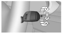
Turn the switch from idle position 0 upward, arrow 1: interval mode. When reverse gear is
