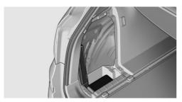
The tow fitting is located in the onboard vehicle tool kit behind the left folding cover in the trunk.
