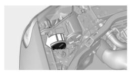
The upper bulb is the low beam and the lower bulb is the parking lamp.
