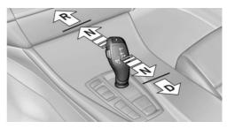
Briefly push the selector lever in the desired direction, beyond a resistance point if needed.
