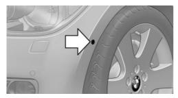
The ultrasound sensors for measuring parking spaces are located on the side of the vehicle.
