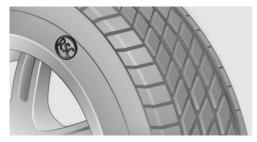
RSC label on the tire sidewall.
