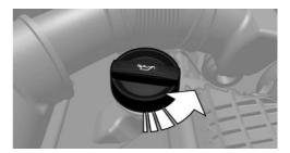
Only add engine oil when the message is displayed in the instrument cluster. The quantity to be added is indicated in the message displayed in the instrument cluster.
