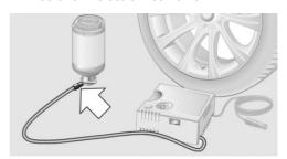
Insert the sealant container on the compressor housing in an upright position.
