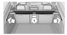
Pull out the cargo cover, arrow 1, and hook both sides into the brackets, arrow 2.
