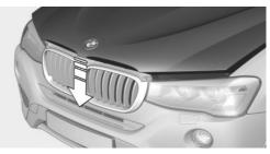
Let the hood drop from a height of approx. 16 in/40 cm and push down on it to lock it fully. Make sure you hear the hood engage.
