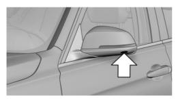
The lenses of the Top View cameras are located at the bottom of the exterior mirror housings. The image quality may be impaired by dirt.
