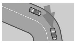
If the desired speed is too high for a curve, the speed is reduced slightly, although curves cannot be anticipated in advance. Therefore, drive into a curve at an appropriate speed.
