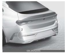
[1]: Front view camera[2]: Rear corner radarRefer to the picture for the detailed location of the detecting sensors.
