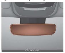
The sensor mounted in the mirror senses the light level around the vehicle. and automatically controls the headlight glare from the vehicles behind you.
