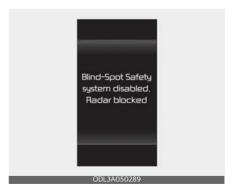
When the rear bumper around the rearside radar or sensor is covered with foreign matters, such as snow or rain, or installing a trailer or carrier, it can reduce the detecting performance and temporarily limit or disable Safe Exit Assist.
