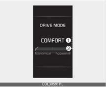
The drive mode selected by the driver (1) and the driving style gauge (2) showing the driver's driving style are displayed on the screen.
