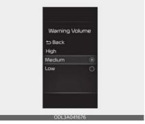
With the ENGINE START/STOP button in the ON position, select 'Driver Assistance → Warning Volume' from the Settings menu to change the warning volume to 'High', 'Medium' or 'Low' for Reverse Parking Distance Warning.
