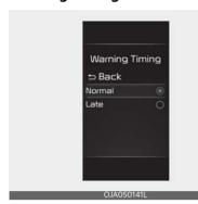
With the ENGINE START/STOP button in the ON position, select 'Driver Assistance → Warning Timing' from the Settings menu to change the initial warning activation time for Blind-Spot Collision-Avoidance Assist.
