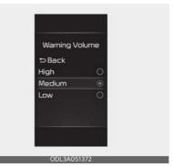
With the ENGINE START/STOP button in the ON position, and select 'Driver Assistance → Warning Volume' to change the warning volume to 'High', 'Medium' or 'Low' for Safe Exit Warning.
