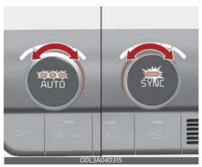
The temperature will increase to the maximum (HI) by rotating the knob clockwise direction.
