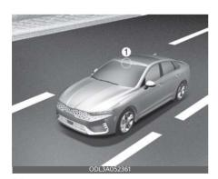
[1]: Front view camera Refer to the picture for the detailed location of the detecting sensors.
