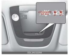
The ODS is designed to detect the presence of a properly-seated front passenger and determine if the passenger's front air bag should be enabled (may inflate) or not. Only the front passenger front air bag is controlled by the ODS. Do not put anything in front of the passenger air bag "XXXIIII indicator.
