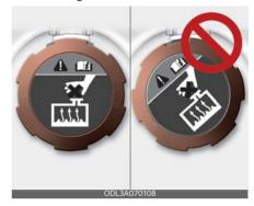
Maker sure that the tiny protrusions inside the coolant cap are securely interlocked.
