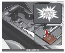
Before the AUTO HOLD will engage, the driver's door and engine hood must be closed.
