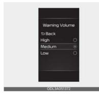
With the ENGINE START/STOP button in the ON position, select 'Driver Assistance → Warning Volume' from the Settings menu to change the Warning Volume to 'High', 'Medium' or 'Low' for Forward Collision-Avoidance Assist.
