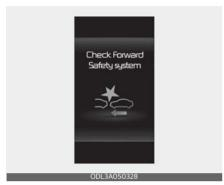
When Forward Collision-Avoidance Assist is not working properly, the 'Check Forward Safety system' warning message will appear, and the
