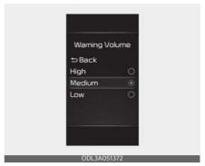
With the ENGINE START/STOP button in the ON position, select 'Driver Assistance → Warning Volume' from the Settings menu to change the Warning Volume 'High', 'Medium' or 'Low' for Smart Cruise Control.
