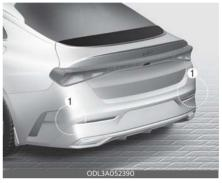
[1]: Rear corner radar Refer to the picture for the detailed location of the detecting sensor.
