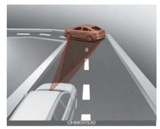
Your driving speed can be reduced due to a vehicle in the adjacent lane. Apply the accelerator pedal and select the appropriate set speed. Check to be sure that the road conditions permit safe operation of Smart Cruise Control.
