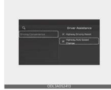
With the ENGINE START/STOP button in the ON position, select 'Driver Assistance → Driving Convenience → Highway Auto Speed Change' from the Settings menu to turn on Navigation-based Smart Cruise Control and deselect to turn off the function.
