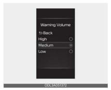
With the ENGINE START/STOP button in the ON position, select 'Driver Assistance → Warning Volume' from the Settings menu to change the Warning Volume to 'High', 'Medium' or 'Low' for Lane Keeping Assist.
