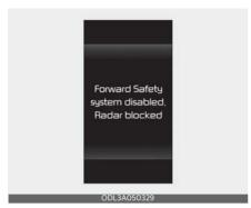
When the front windshield where the front view camera is located, front radar cover, bumper or sensor is covered with foreign material, such as snow or rain, it can reduce the detecting performance and temporarily limit or disable Forward Collision-Avoidance Assist.
