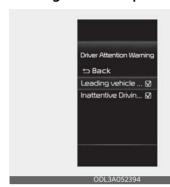
• If 'Leading Vehicle Departure Alert' is selected, the function will inform the driver when the front vehicle departs from a stop.
