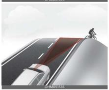
Forward Collision-Avoidance Assist may not detect other vehicle, pedestrian or cyclist in front of you while driving uphill or downhill adversely affecting the performance of the sensors.
