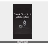
When Safe Exit Assist is not working properly, the 'Check Blind-Spot Safety system' warning message will appear on the cluster, and Safe Exit Assist will turn off automatically or it will be limited. In this case, have your vehicle inspected by an authorized Kia dealer.
