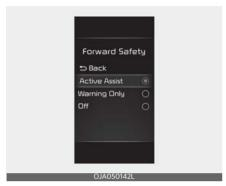
With the ENGINE START/STOP button in the ON position, select or deselect 'Driver Assistance → Forward Safety' from the Settings menu to set whether or not to use each function.
