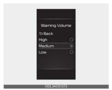
With the ENGINE START/STOP button in the ON position, select 'Driver Assistance → Warning Volume' from the Settings menu to change the Warning Volume to 'High', 'Medium' or 'Low' for Highway Driving Assist.
