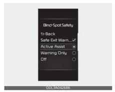
With the ENGINE START/STOP button in the ON position, select or deselect 'Driver Assistance → Blind-Spot Safety' from the Settings menu to set whether or not to use each function.
