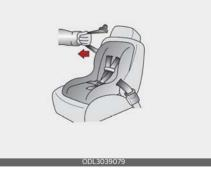
4. Slowly allow the shoulder portion of the seat belt to retract and listen for an audible "clicking" or "ratcheting" sound. This indicates that the retractor is in the "automatic locking" mode.
