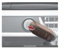
When the stop lamp fuse is blown, you cannot start the engine normally. Replace the fuse with a new one. If it is not possible, you can start the engine by pressing the ENGINE START/STOP button for 10 seconds while it is in the ACC position. The engine can start without pressing the brake pedal. But for your safety, always press the brake pedal before starting the engine.
