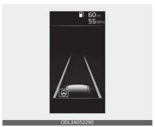
If the vehicle ahead and/or both lane markings are detected and your driving speed is below 110 mph (180 km/h), the green [ juice and indicator light will illumi-
