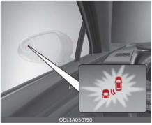
To warn the driver a vehicle is detected, the warning light on the side view mirror and head-up display (if equipped) will illuminate.  Blind-Spot Collision-Avoidance Assist will operate when your driving speed is above 12 mph (20 km/h) and the speed of the vehicle in the blind spot area is above 7 mph (10 km/h).
