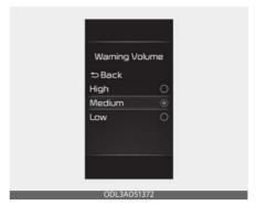
With the ENGINE START/STOP button in the ON position, select 'Driver Assistance → Warning Volume' from the Settings menu to change the Warning Volume 'High', 'Medium' or 'Low' for Safe Exit Assist.
