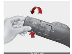
High Beam Assist is a function that automatically adjusts the headlamp range (switches between high beam and low beam) depending on the brightness of detected vehicles and certain road conditions.
