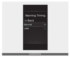
With the ENGINE START/STOP button in the ON position, select 'Driver Assistance → Warning Timing' from the Settings menu to change the initial warning activation time for Reverse Parking Collision-Avoidance Assist.
