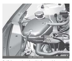
If the coolant level is low, add enough specified coolant to provide protection against freezing and corrosion. Bring the level to MAX, but do not overfill.
