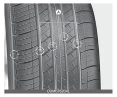
This shows there is less than 1/16 inches (1.6 mm) of tread left on the tire. Replace the tire when this happens.
