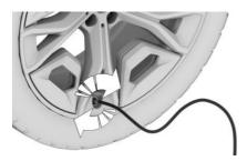
With the compressor switched off, insert the connector into the power socket in the vehicle interior
