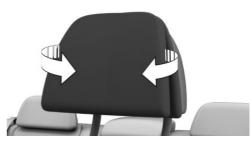
Fold the side extensions on the head restraint forward for increased side support in the resting position.
