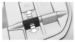
Repeatedly push the rocker switch forward or pull it back until the desired xOFFROAD driving mode is displayed on the instrument cluster.
