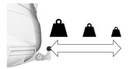
The permissible gross weight of the loaded rear carrier depends on how far its center of gravity is from the ball head.
