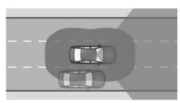
Radar sensors monitor the space next to the vehicle when traveling faster than a minimum speed and up to approx. 130 mph/210 km/h.
