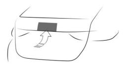
Press the button on the trunk to access the vehicle while in deep sleep mode. Deep sleep mode remains on in this case.
