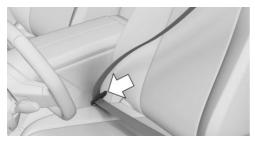
To ease accessibility to the seat belt buckle, an adjustable slider is available on the belt to help position the buckle when not in use.
