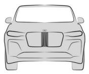
The front camera is located in the radiator grille.
