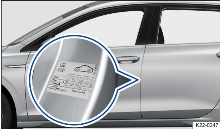
Fig. 1 On the driver door pillar: tyre pressure sticker (alternatively on the inside of the charging socket flap).
