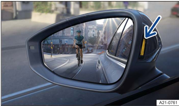
Fig. 1 In the exterior mirror housings: display of the exit warning system (illustration).
