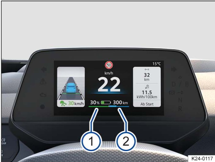
Fig. 1 In the digital instrument cluster: charge level of the high-voltage battery (1) and vehicle range (2) (illustration).
