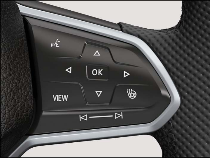
Fig. 1 Right side of the multifunction steering wheel: operating the digital instrument cluster (illustration).
