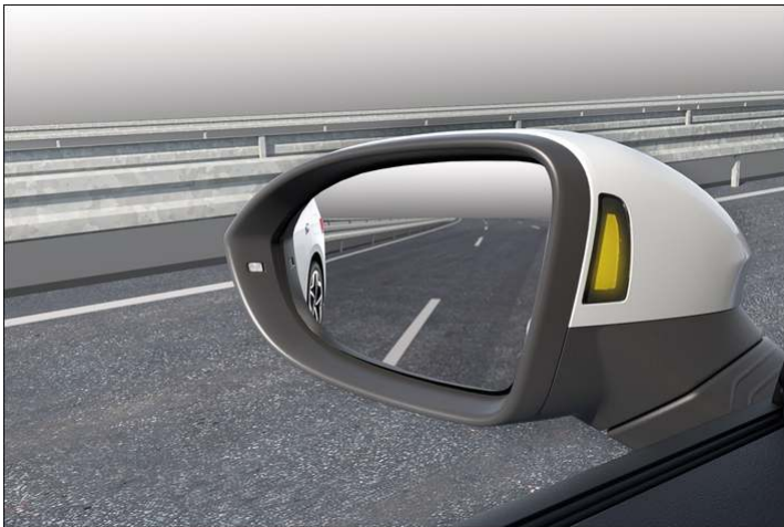
Fig. 1 In the housings of the exterior mirrors: Side Assist displays.
