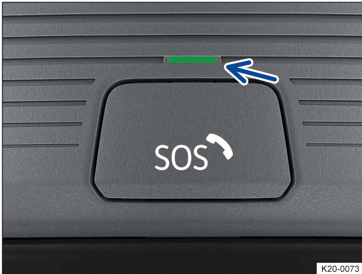
Fig. 1 In the roof console: button for Emergency Call Service (behind button cover) and indicator lamp.
