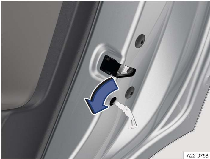
Fig. 1 In the front edge of the rear right-hand door: manually locking the vehicle with the manual key (illustration).
