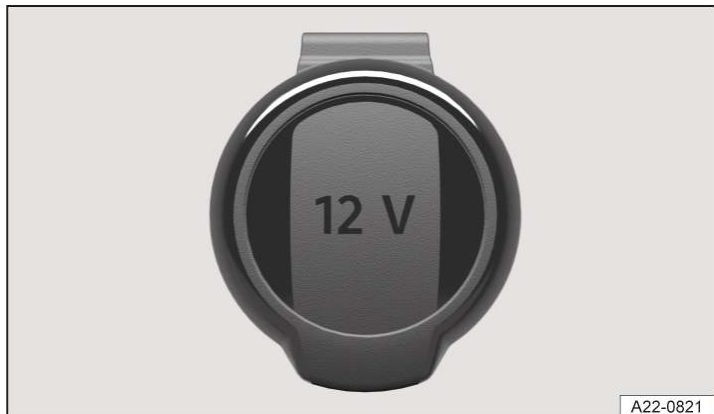
Fig. 1 In the luggage compartment on the left-hand side: fold-open 12-volt socket (illustration).
