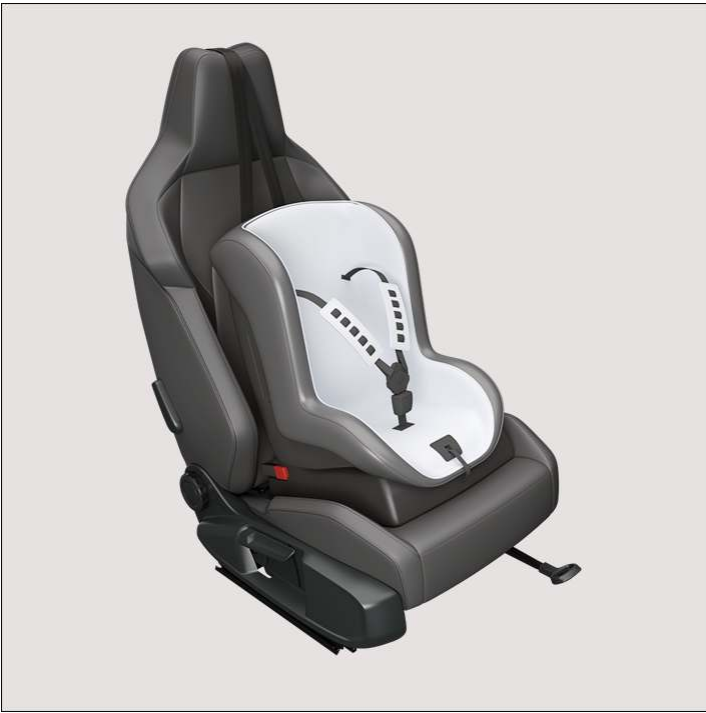
Fig. 5 In the backrest of the premium sport seat (without opening) on the front passenger side: routing for the top tether (illustration).
