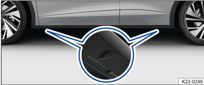
Fig. 1 On the sill: markings for the jacking points.
