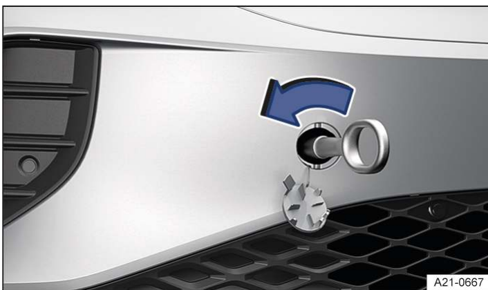
Fig. 2 In the front bumper on the right: screwing in the towing eye.
