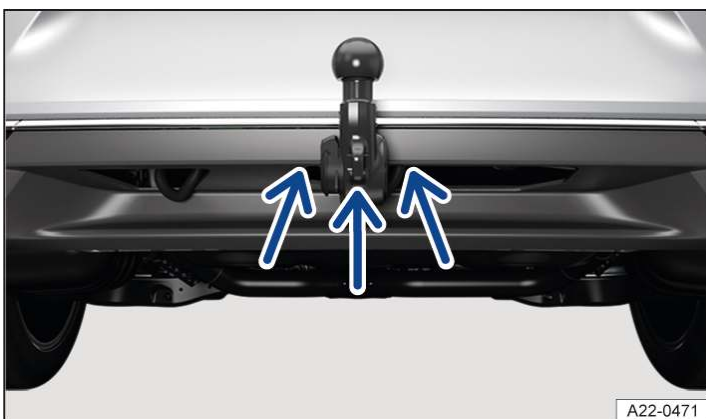
Fig. 1 On the towing bracket: eye for securing the safety or breakaway cable (illustration).
