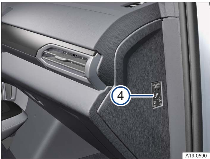
Fig. 2 With open front passenger door (left-hand drive vehicles): key-operated switch in the dash panel (mirrored for right-hand drive vehicles).
