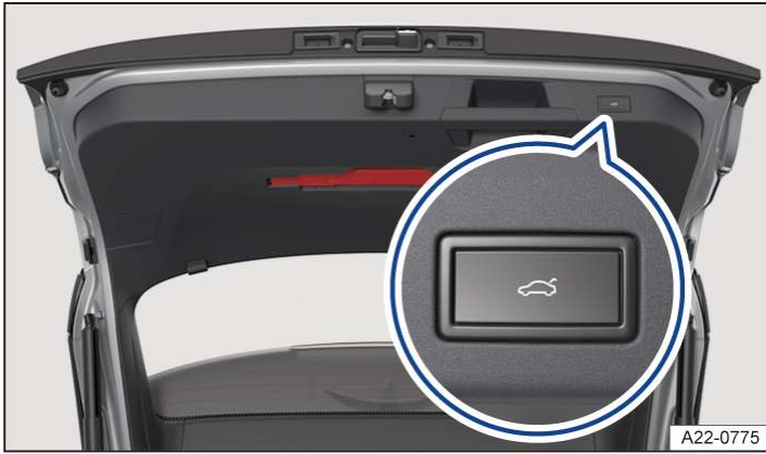
Fig. 1 In the open boot lid: button for electrically closing the boot lid (illustration).
