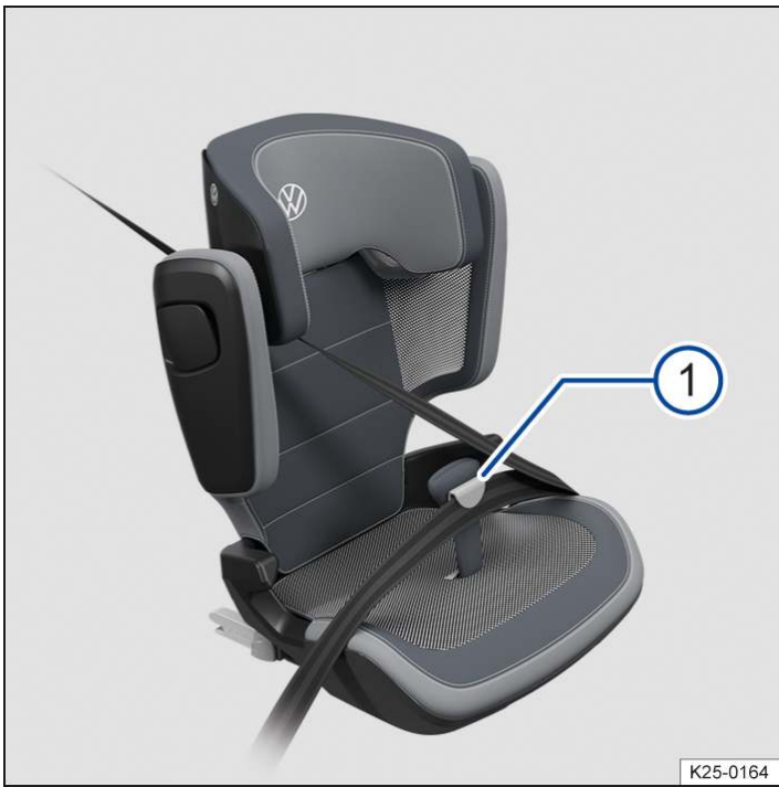
Fig. 2 Child seat with additional belt guide (illustration).
