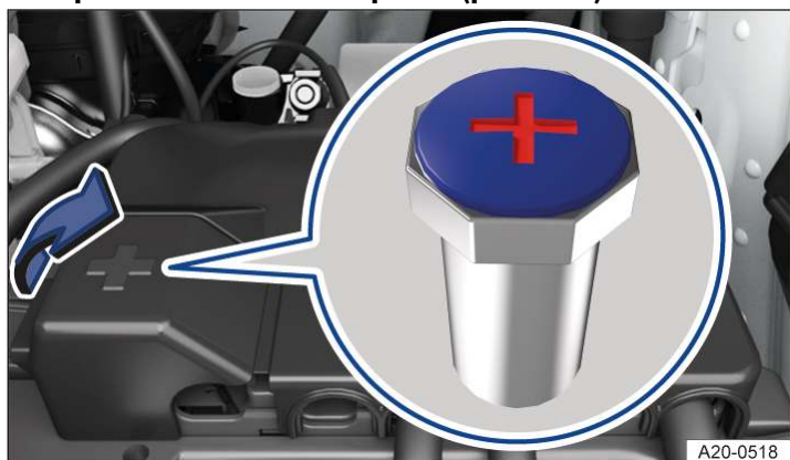
Fig. 1 In the bonnet space underneath a cover: positive jump-start connection point.
