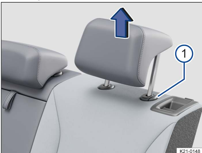
Fig. 2 Removing a rear head restraint (illustration).
