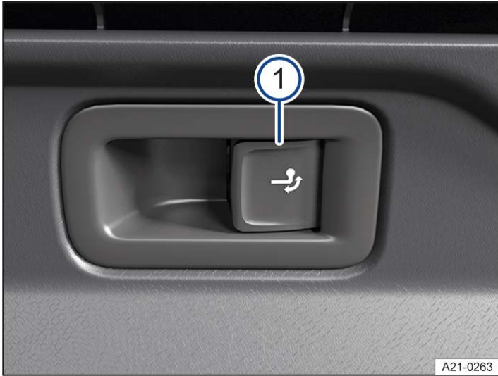
Fig. 1 On the right of the luggage compartment: button for releasing the ball coupling.
