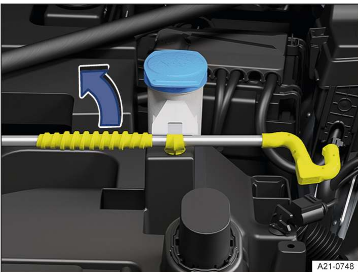
Fig. 3 In the bonnet space: bonnet stay in holder (illustration).
