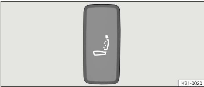
Fig. 1 On the outside of the driver seat: button for the massage function.
