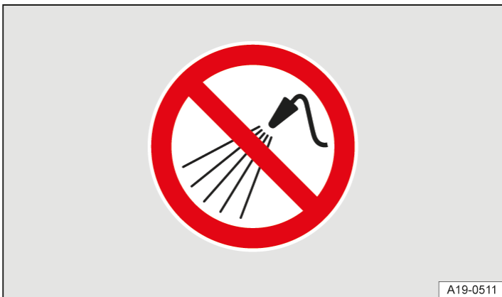
Fig. 1 In the bonnet space: do not use a high-pressure cleaner.
