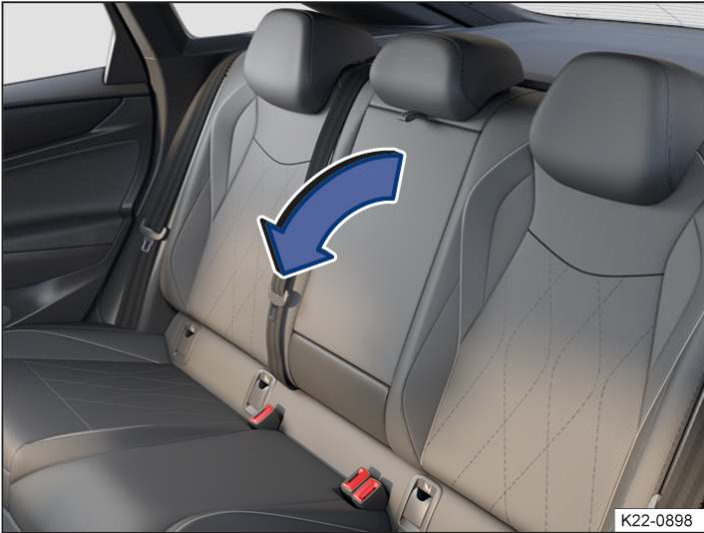
Fig. 1 In the backrest of the middle seat: fold-out rear centre armrest (illustration).
