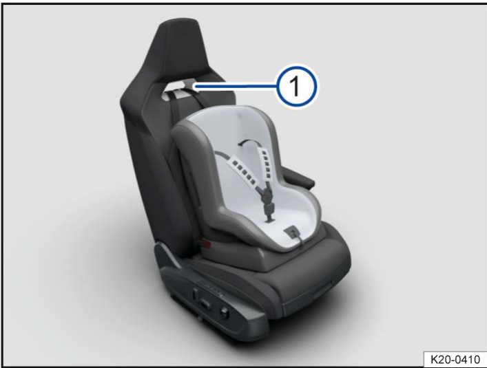
Fig. 4 In the backrest of the premium sport seat (with opening) on the front passenger side: routing for the top tether (illustration).
