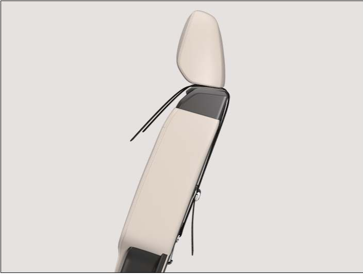
Fig. 3 On the rear of the outer rear seats or front passenger seat: attached top tether.
