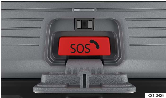
Fig. 2 In the roof console: button for the legally required eCall Emergency System.
