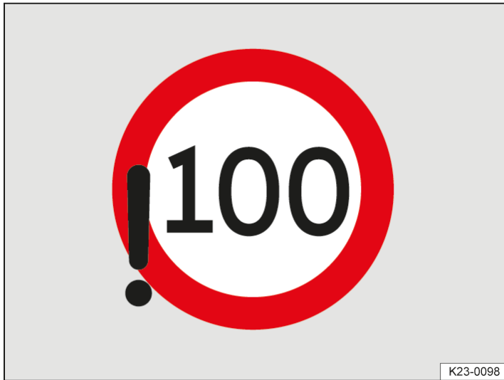
Fig. 1 On the display of the digital instrument cluster: detected violation of maximum permitted speed (illustration).
