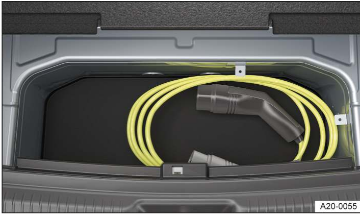
Fig. 1 Under the luggage compartment floor: stowage compartment with stowage space for the charging cable (illustration).
