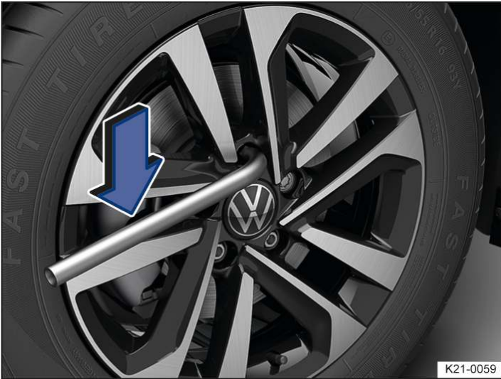
Fig. 1 Loosening wheel bolts.
