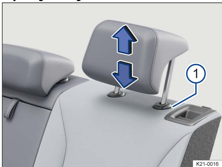
Fig. 2 Adjusting a rear head restraint (illustration).
