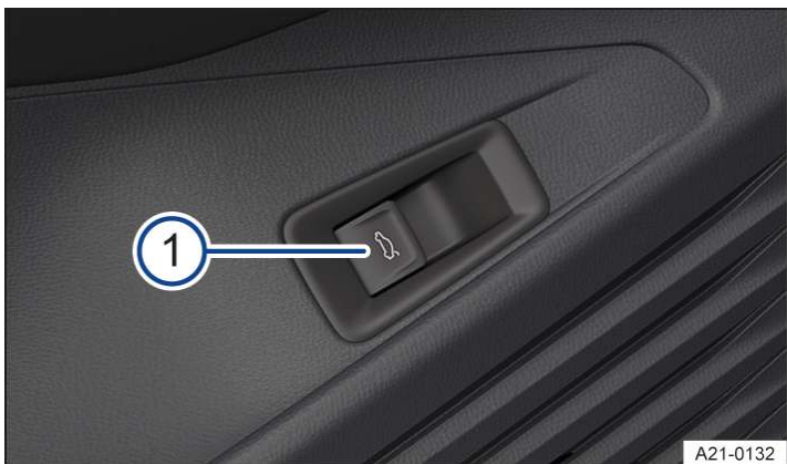
Fig. 2 In the driver door: release button for the boot lid.
