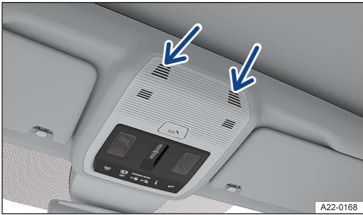
Fig. 1 In the roof console: sensors for the interior monitoring system (arrows).
