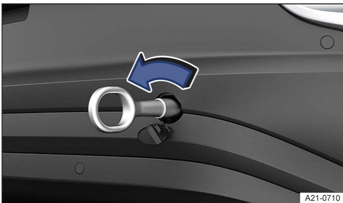
Fig. 2 In the rear bumper on the right: screwing in the towing eye.
