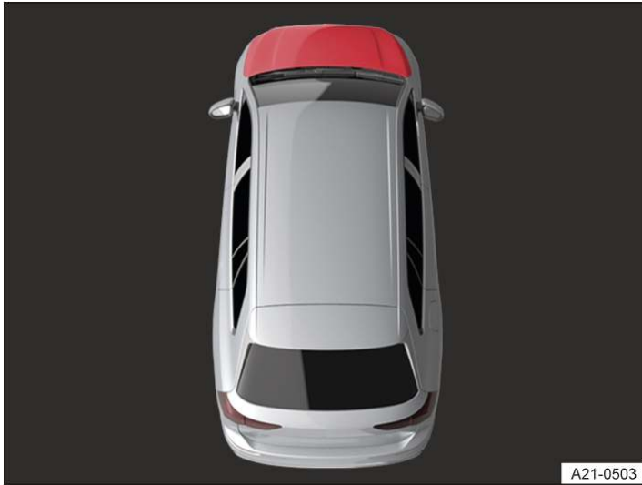
Fig. 5 On the instrument cluster display: the bonnet is open or not closed properly (illustration).
