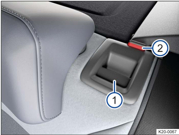
Fig. 1 In the rear seat backrest: release button.
