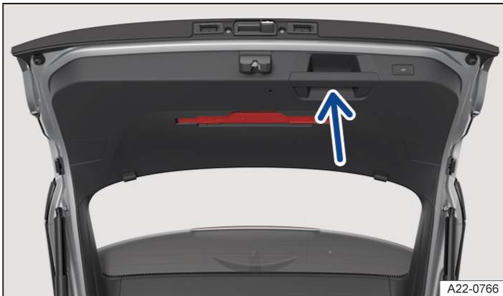
Fig. 2 In the open boot lid: handle for closing the boot lid (illustration).
