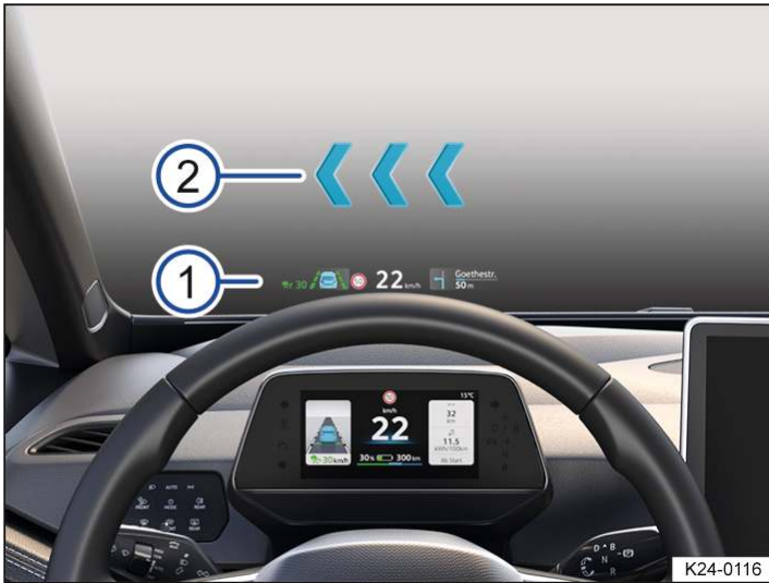
Fig. 1 In the driver's field of vision: displays in the head-up display (illustration).
