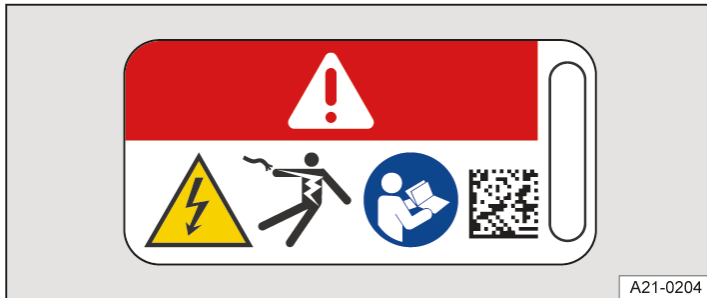
Fig. 1 Warning sign on high-voltage components.
