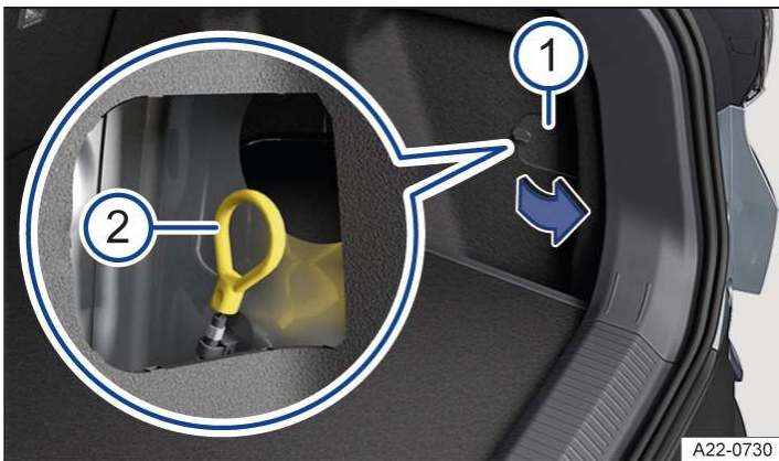
Fig. 2 In the lower right-hand side of the luggage compartment trim: manual release of the charging connector.
