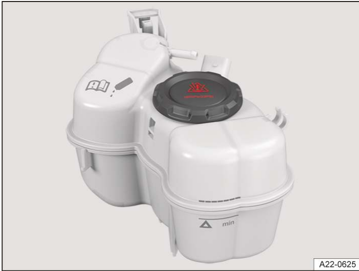
Fig. 2 In the bonnet space: markings on the coolant expansion tank (illustration).
