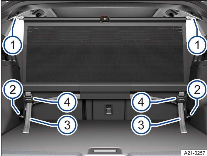
Fig. 1 In the luggage compartment: net partition installed behind the rear bench seat.
