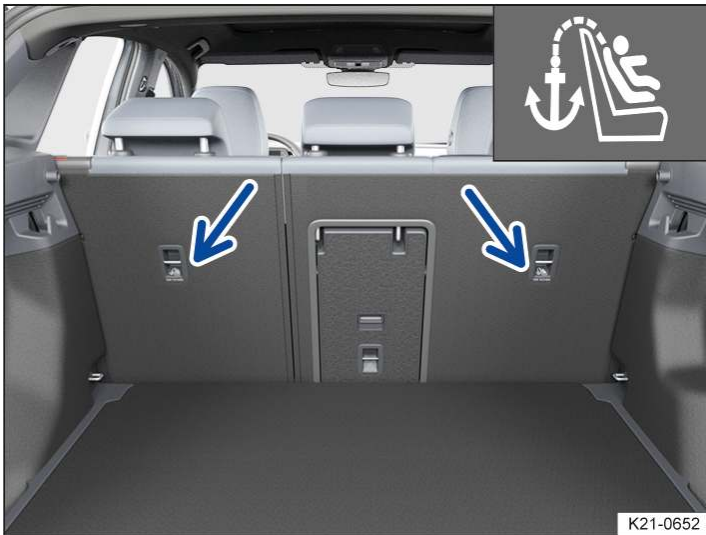
Fig. 1 On the rear of the rear seats: top tether anchor points for top tether.
