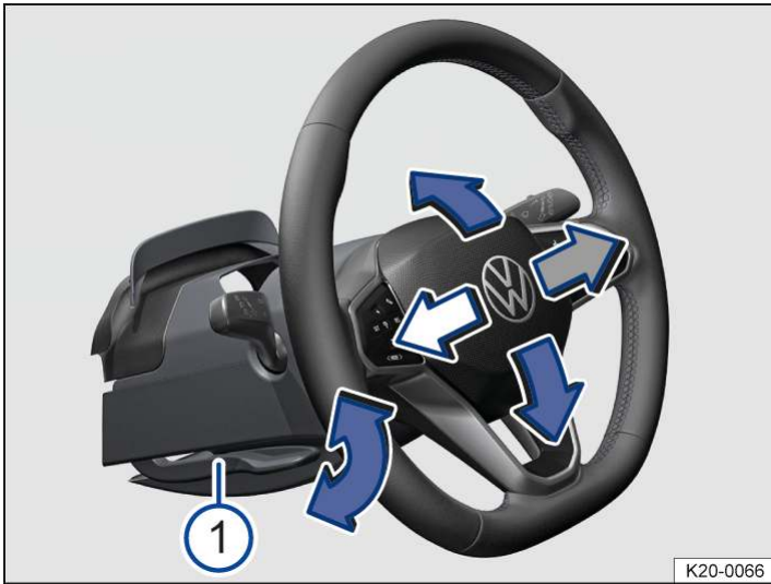
Fig. 1 Below the steering wheel in the steering column trim: lever for mechanical adjustment of the steering wheel position (illustration).
