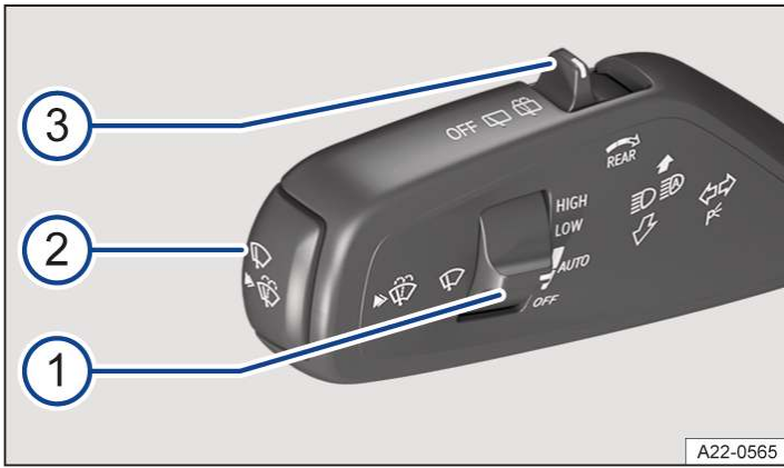
Fig. 1 On the left-hand side of the steering column: lever for turn signal, main beam and wipers.
