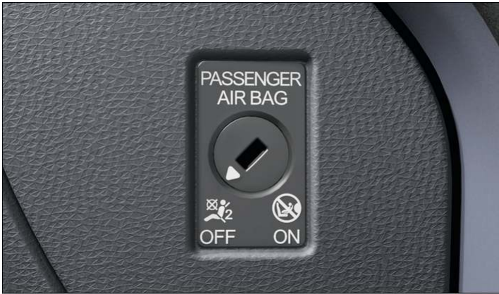
Fig. 1 In the dash panel on the front passenger side: key-operated switch for switching the front passenger front airbag on and off.
