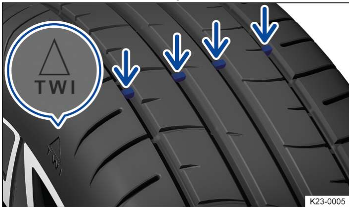
Fig. 1 In the tread grooves: tread wear indicator.
