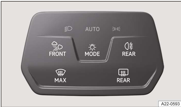
Fig. 1 Next to the steering wheel: touch panel for switching on the exterior lighting.
