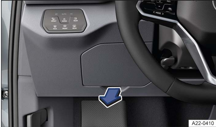
Fig. 1 On the driver side: fuse box cover in the dash panel (left-hand drive vehicle)
