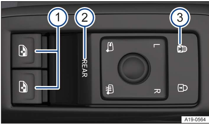
Fig. 1 In the driver door: buttons for the front and rear electric windows (illustration).
