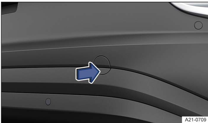
Fig. 1 In the rear bumper on the right: removing the cover.
