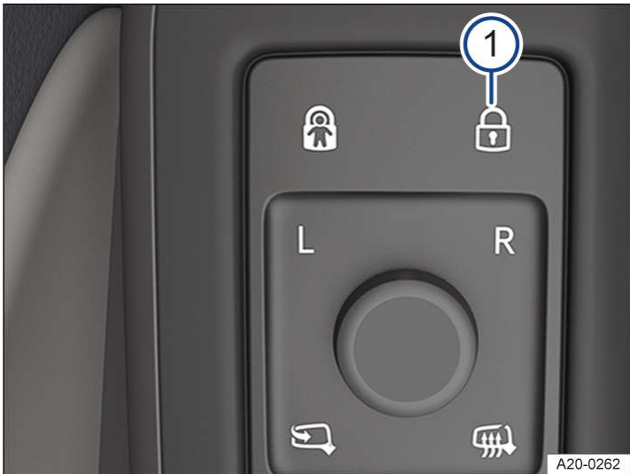
Fig. 1 In the driver door: central locking touch panel.
