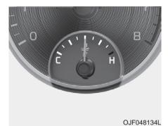
This gauge indicates the temperature of the engine coolant when the ignition switch or Engine Start/Stop button is ON
