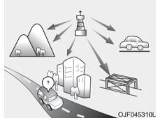
FM broadcasts are transmitted at high frequencies and do not bend to follow the earth's surface. Because of this, FM broadcasts generally begin to fade within short distances from the station. Also, FM signals are easily affected by buildings, mountains, and obstructions. This can lead to undesirable or unpleasant listening conditions which might lead you to believe a problem exists with your radio. The following conditions are normal and do not indicate radio trouble:
