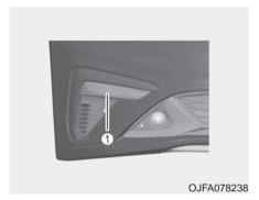
If the front turn signal lamp (1) does not operate, have the vehicle checked by an authorized Kia dealer.
