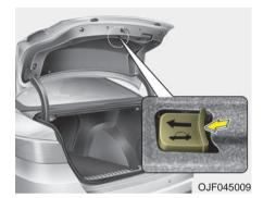
Your vehicle is equipped with an emergency trunk release lever located inside the trunk. If someone is inadvertently locked in the trunk, moving the handle in the direction of the arrow will release the trunk latch mechanism and open the trunk.
