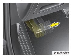
Check whether the stroke is within specification when the parking brake pedal is pressed with 30 kg (66 lb, 294 N) of force. Also, the parking brake alone should securely hold the vehicle on a fairly steep grade. If the stroke is more or less than specified, have the parking brake adjusted by an authorized Kia dealer.
