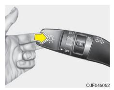
To flash the headlight high beams, pull the lever towards you. It will return to the normal (low beam) position when released. The headlight switch does not need to be on to use this flashing feature.
