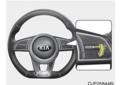
Move the lever down (to SET-), and release it at the desired speed. The SET indicator light in the instrument cluster will illuminate. Release the accelerator at the same time. The desired speed will automatically be maintained.
