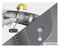
When the light switch is in the AUTO light position, the taillights and headlights will turn ON or OFF automatically depending on the amount of outside light the auto light sensor receives.
