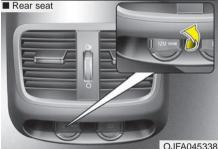
The power outlet is designed to provide power for mobile telephones or other devices designed to operate with vehicle electrical systems. The devices should draw less than 10 amps with the engine running.
