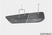
If the stop and tail lamp (LED) does not operate, have the vehicle checked by an authorized Kia dealer. The LED lamp cannot be replaced as a single component because it is an integrated unit. The LED lamp has to be replaced with the unit.
