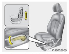
To change the height of the seat, move the lever upwards or downwards.
