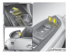
While the vehicle is moving in reverse, the outside rearview mirror(s) will move downward to aid reverse parking. According to the position of the outside rearview mirror switch, the outside rearview mirror(s) will operate as follows:
