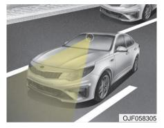
In order for the FCA system to operate properly, always make sure the sensor are clean and free of dirt, snow, and debris.
