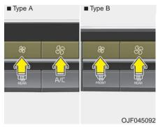
The fan speed can be set to the desired speed by operating the fan speed control buttons.
