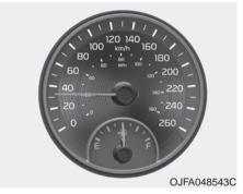
The speedometer indicates the speed of the vehicle and is calibrated in kilometers per hour (km/h) and/or miles per hour (mph).
