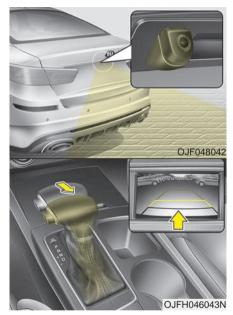
The rear view monitor will activate with the ignition switch ON and the shift lever in the R (Reverse) position. The system is a supplemental sys-
