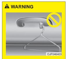
Do not hang other objects such as hangers or hard objects except clothes. Also, do not put heavy, sharp or breakable objects in the clothing pockets. An occupant could be seriously injured from these items if they become projectiles during a collision.
