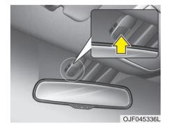
Auto defogging reduces the probability of fogging up the inside of the windshield by automatically sensing the moisture of inside the windshield. The auto defogging system operates
