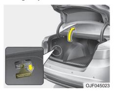
If the fuel filler lid does not open using the fuel filler lid opener button, you can open it manually. Open the trunk and slightly pull the emergency release handle on the left side.
