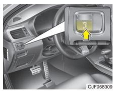
The indicator on the switch will illuminate when the BCW (Blind-Spot Collision Warning) system switch is pressed with the ignition switch ON. If the vehicle speed exceeds 30 km/h (20 mph), the system will activate.
