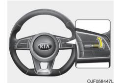
If any method other than the CRUISE ON-OFF switch was used to cancel cruising speed and the system is still activated, the most recent set speed will automatically resume
