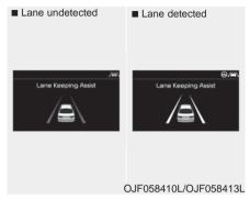
If the speed of the vehicle is over 64 km/h (40 mph) and the system detects lane markers, the color changes from gray to white
