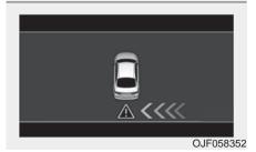
If the vehicle detected by the sensors approaches your vehicle, the warning chime will sound, the warning light on the outside rearview mirror will blink and a message will appear on the LCD display.
