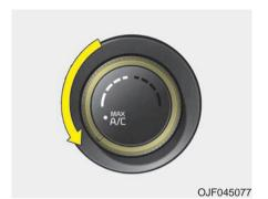
The MAX A/C mode is used to cool the inside of the vehicle faster.
