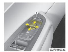
The electric remote control mirror switch allows you to adjust the position of the left and right outside rearview mirrors. To adjust the position of either mirror, press the R or L button (1) to select the right side mirror or the left side mirror, then press a corresponding point (▲) on the mirror adjustment control to position the selected mirror up, down, left or right.
