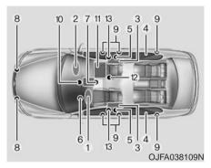
The SRS consists of the following components:
