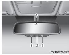
The electric rearview mirror automatically controls the glare from the headlights of the vehicles behind you in nighttime or low light driving conditions. The sensor (4) mounted in the mirror senses the light level around the vehicle, and automatically conrols the headlight glare from the vehicles behind vou.
