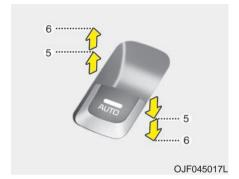
Pressing or pulling up the power window switch momentarily to the second detent position (6) completely lowers or raises the window even when the switch is released. To stop the window at the desired position while the window is in operation, pull up or press down and release the switch.
