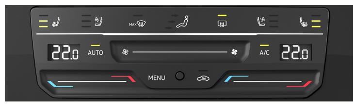
Fig. 81 In the upper section of the center console: Climate control bar for the Climatronic system.
