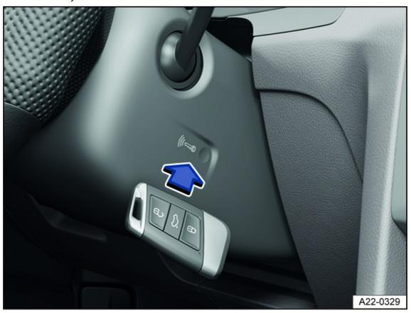
Fig. 86 On the right side of the steering column: emergency start function on vehicles with Keyless Access with push-button start.
