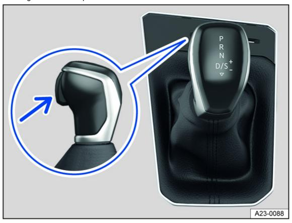
Fig. 88 In the center console: selector lever of the automatic transmission (general example).
