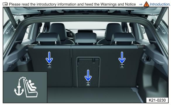
Fig. 33 On the back of the rear seats: top tether anchorages for the top tether safety belt.
