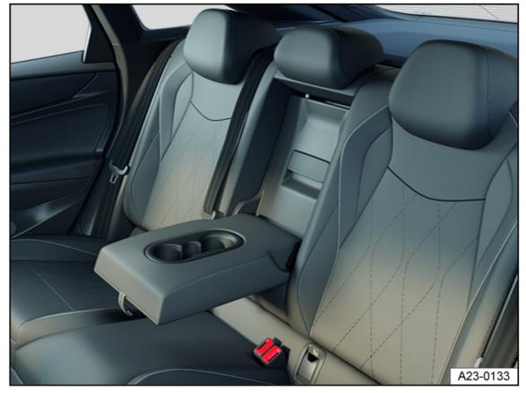
Fig. 119 In the rear center armrest: cup holder (general example).
