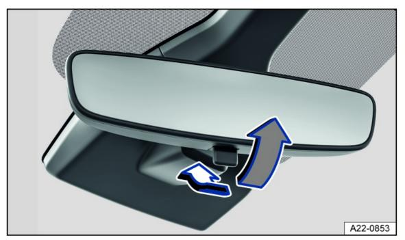
Fig. 77 On the windshield: manual dimming interior rearview mirror.
