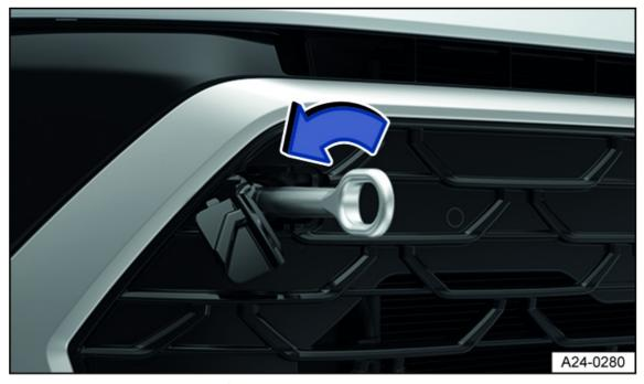
Fig. 151 In the right front bumper: Screw in towing eye.
