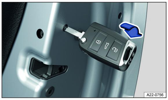
Fig. 49 In the front edge of the rear door: locking of the vehicle in an emergency with the key bit or emergency key (variant 1).
