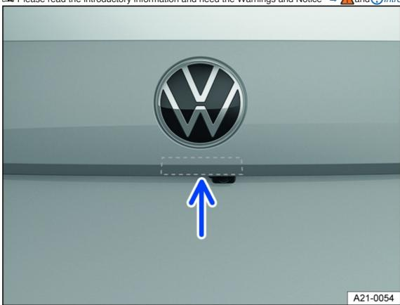
Fig. 52 In the trunk lid: Button to open the trunk lid (general example).
