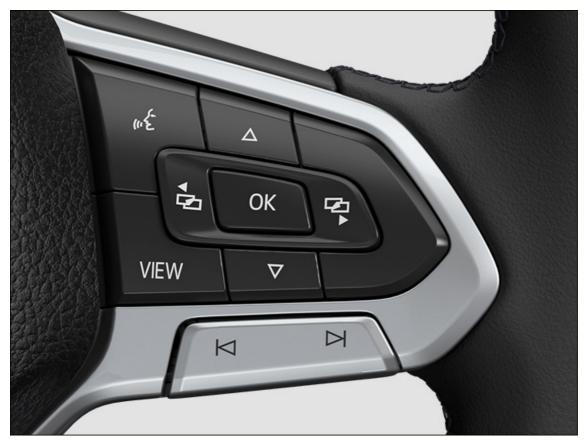
Fig. 10 Right side of the multi-function steering wheel: Operating the Volkswagen Digital Cockpit Pro.
