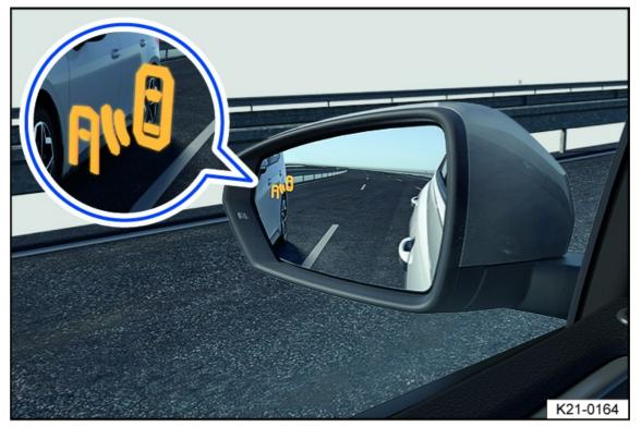
Fig. 107 In the mirror glass of the outside mirrors: Blind Spot Monitor indicator.
