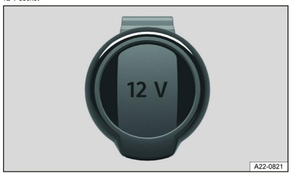
Fig. 120 In the front storage compartment or in the luggage compartment on the left-hand side: Folding 12 V socket (general example).
