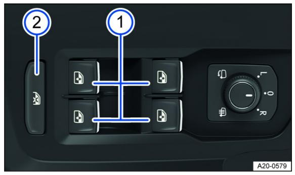
Fig. 54 In the driver door: Power window buttons.
