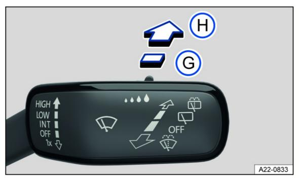
Fig. 74 On the right side of the steering column: operating the rear window wiper.
