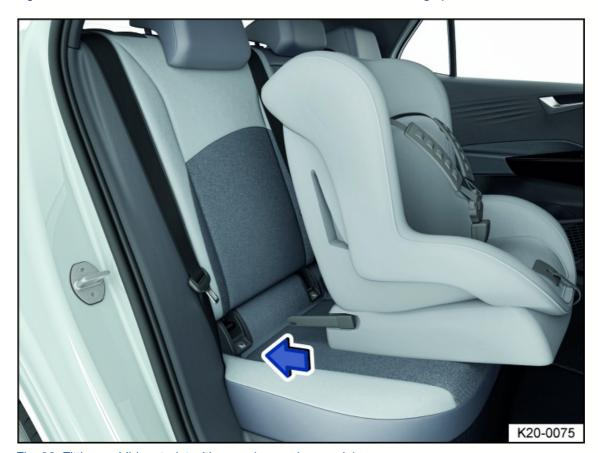
Fig. 32 Fitting a child restraint with arms (general example).
