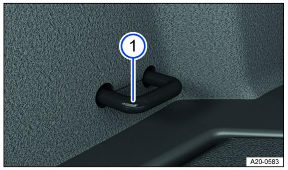
Fig. 127 In the luggage compartment: Tie-down (general example).
