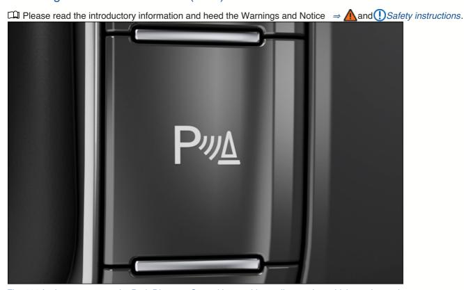
Fig. 111 In the center console: Park Distance Control button (depending on the vehicle equipment).
