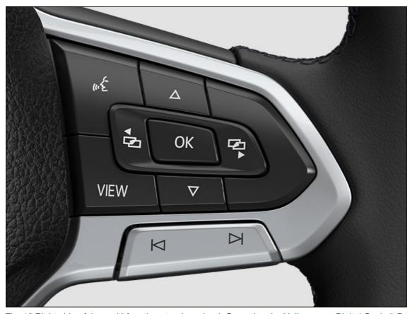
Fig. 12 Right side of the multi-function steering wheel: Operating the Volkswagen Digital Cockpit Basic.
