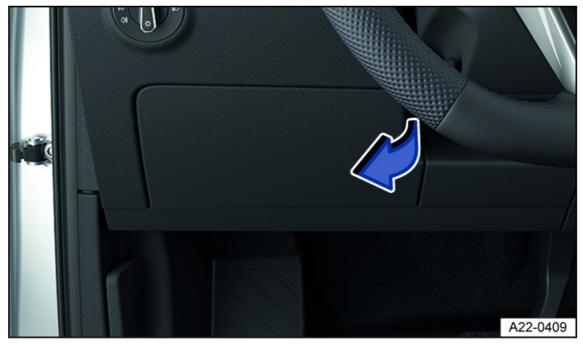
Fig. 143 On the driver side in the instrument panel: fuse box cover (general example).
