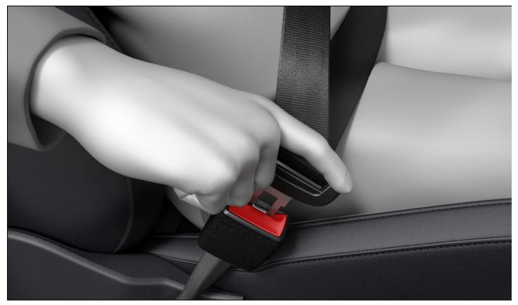
Fig. 22 Inserting the buckle tongue into the safety belt buckle (general example).
