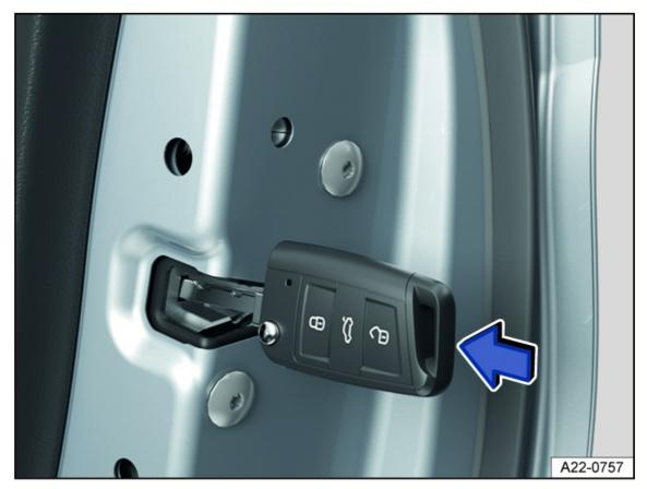
Fig. 50 In the front edge of the rear door: locking of the vehicle in an emergency with the key bit or emergency key (variant 2).
