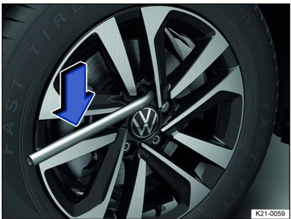
Fig. 180 Removing wheel bolts with the lug wrench.
