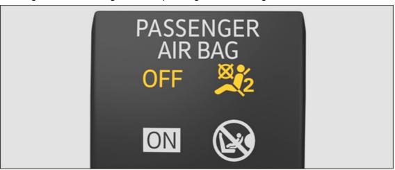
Fig. 27 In the center console: indicator light for the switched off front passenger's front airbag.
