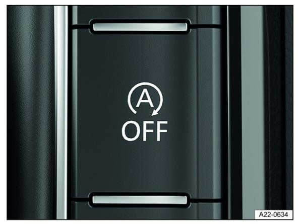
Fig. 87 In the lower section of the center console: Button for the start-stop system.
