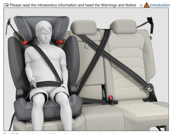
Fig. 36 Correctly fastened child on a booster seat (general example).
