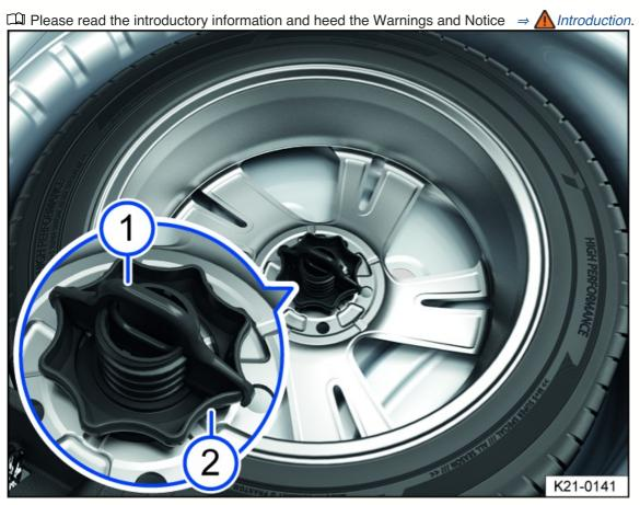
Fig. 172 Under the luggage compartment floor: handwheel to secure the spare wheel or compact spare wheel.
