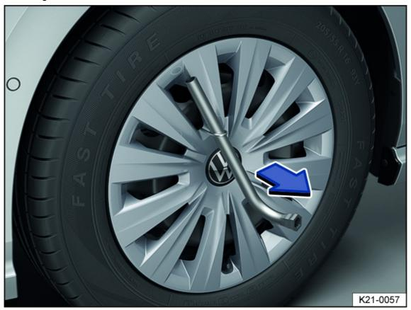
Fig. 174 Remove the wheel hub cover.
