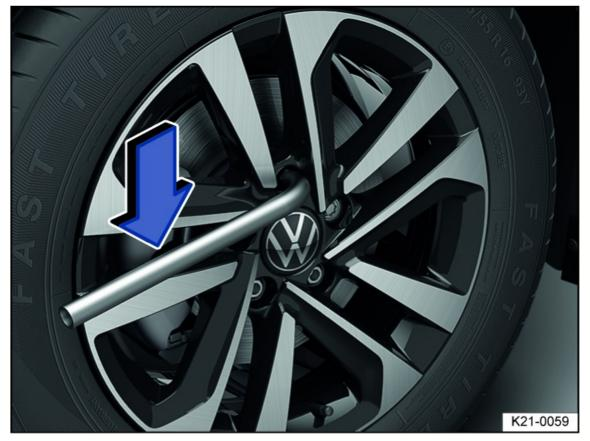
Fig. 176 Loosening wheel bolts.
