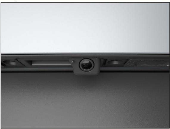
Fig. 184 In the rear of the vehicle: Rear View Camera system on the handle (general example).
