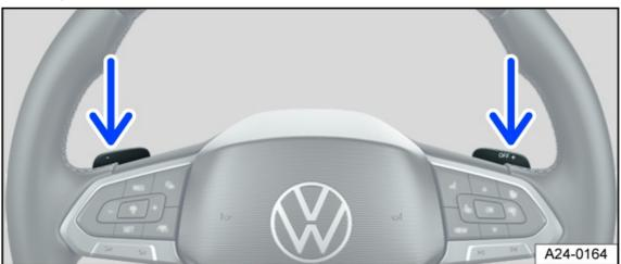
Fig. 90 Behind the steering wheel: shift paddles for the tiptronic (general example).
