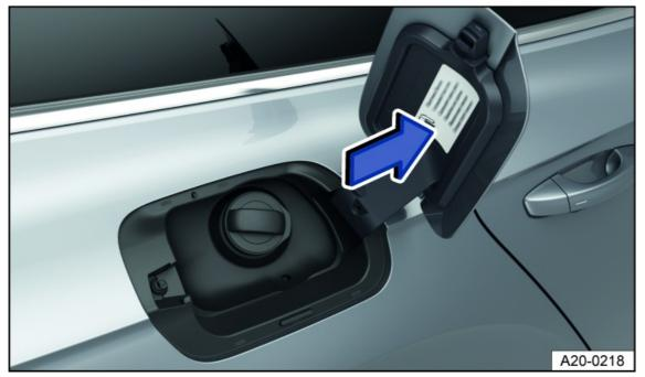
Fig. 131 On the inside of the fuel filler flap: fuel label (general example)
