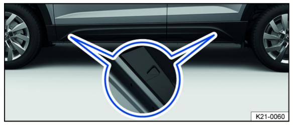
Fig. 177 On the side sill: markings for the jack lift points.
