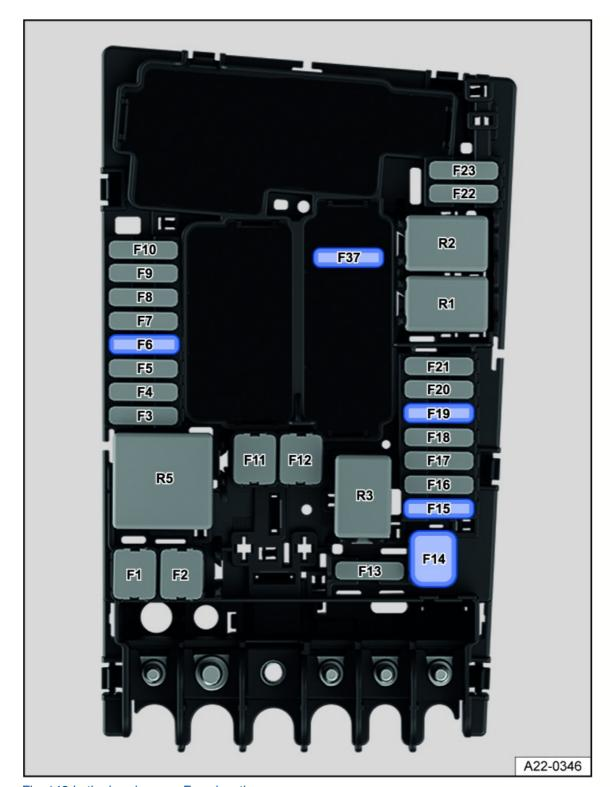
Fig. 142 In the hood space: Fuse locations.
