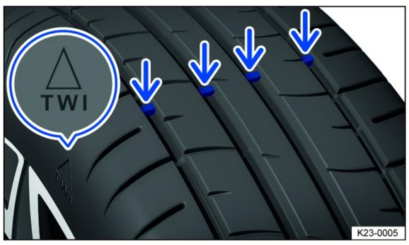
Fig. 169 In the tread grooves: wear indicator.
