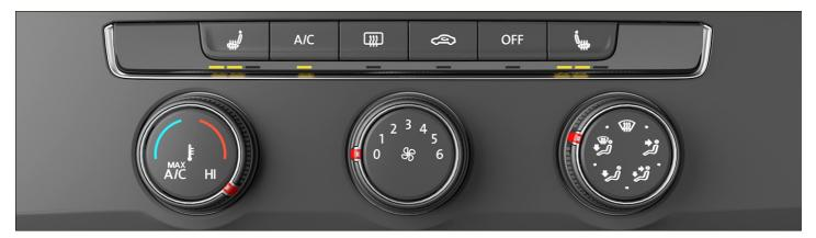
Fig. 82 In the upper section of the center console: Climate control bar for the manual climate control system.
