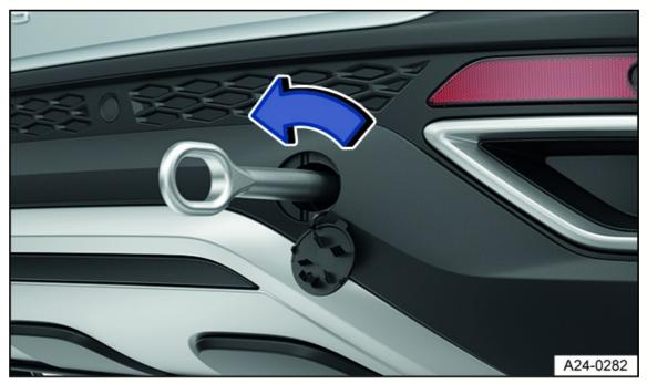
Fig. 153 In the right rear bumper: Screw in towing eye.
