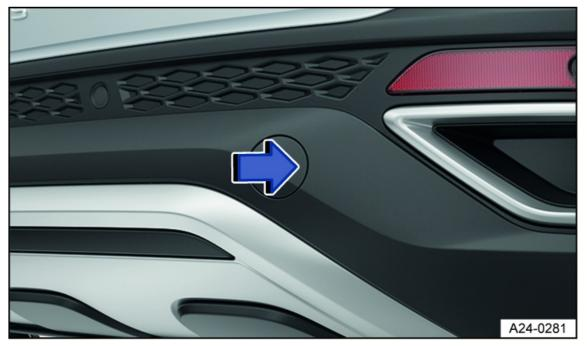
Fig. 152 In the right rear bumper: Remove cover.
