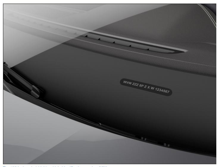
Fig. 185 In the windshield: vehicle identification number (VIN)
