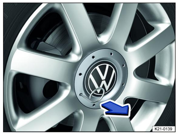
Fig. 173 Remove the hubcap.
