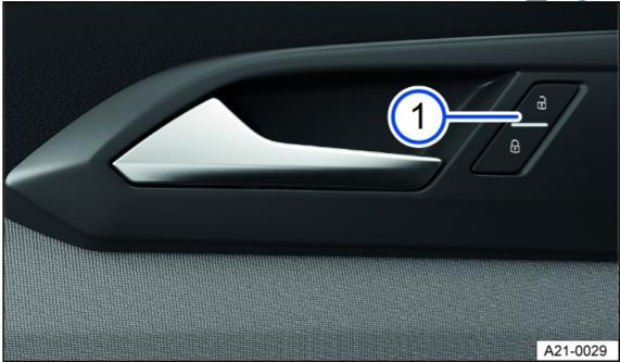
Fig. 47 In the driver's door: Central locking button (general example).
