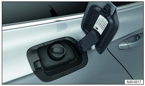
Fig. 132 Behind the fuel filler flap: fuel tank cap (general example)
