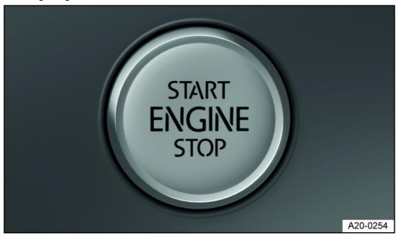
Fig. 85 In the lower section of the center console: starter button.
