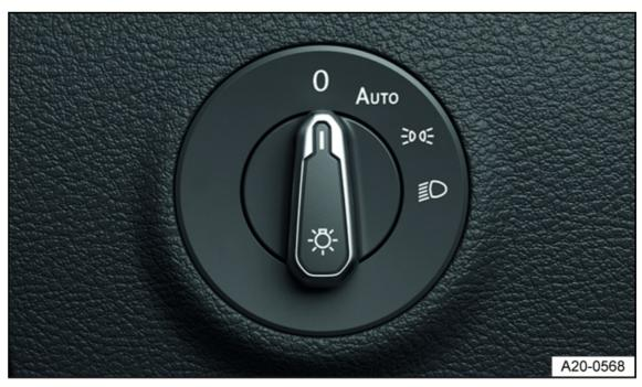
Fig. 70 Next to the steering wheel: light switch (one version).
