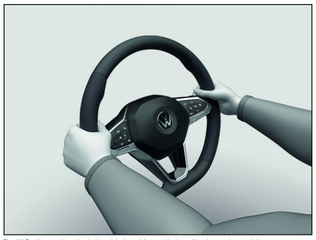
Fig. 57 On the steering wheel: nine o'clock and three o'clock position (general example).
