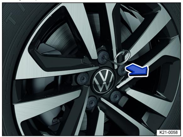
Fig. 175 Remove the caps from the wheel bolts.
