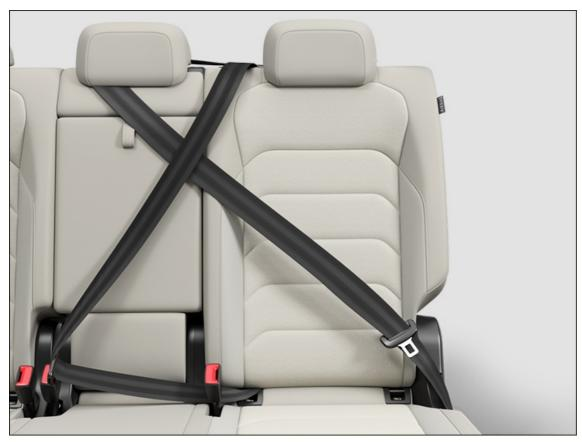
Fig. 35 Securing unused safety belts (general example).
