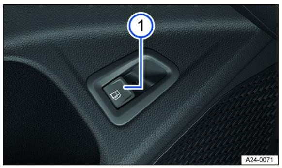
Fig. 133 In the driver door: button for the fuel filler door release (general example).
