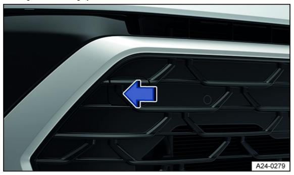
Fig. 150 In the right front bumper: Remove cover.
