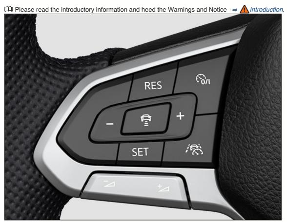
Fig. 106 Left side of the multi-function steering wheel.
