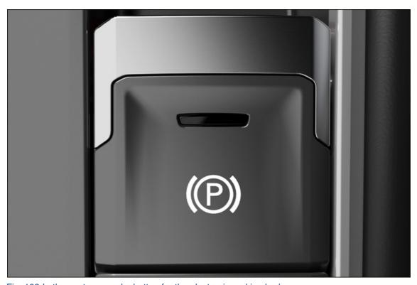
Fig. 108 In the center console: button for the electronic parking brake.
