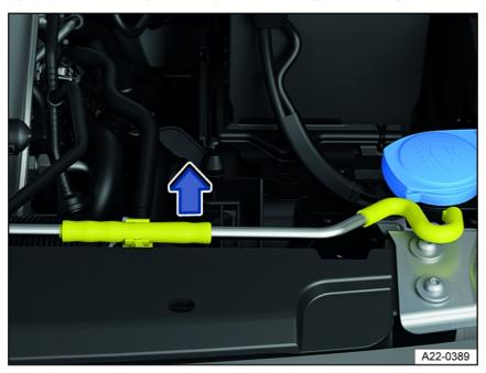
Fig. 161 In the engine compartment: Hood support in the bracket.
