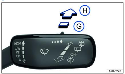
Fig. 80 On the right side of the steering column: operating the rear window wiper.
