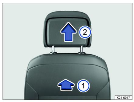
Fig. 71 Removing the front head restraint (general example).
