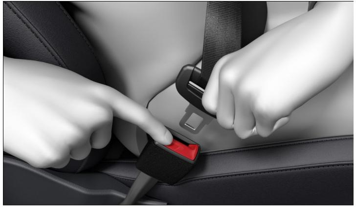
Fig. 24 Releasing the buckle tongue from the safety belt buckle.
