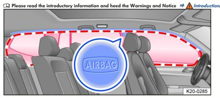
Fig. 34 On the left side of the vehicle: installation location and deployment zone of the Side Curtain Protection®.
