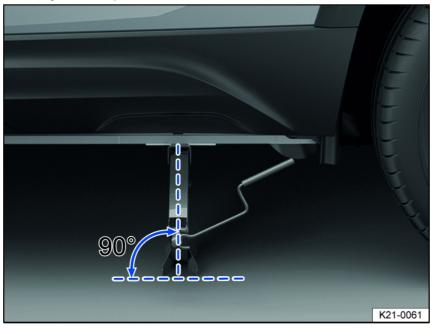
Fig. 181 Correct jack setup.
