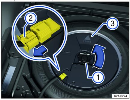
Fig. 174 In the luggage compartment: removing the subwoofer (version 2).
