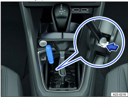
Fig. 97 In the center console: manually release the Automatic Shift Lock (ASL) (variant 1).
