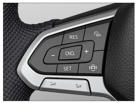
Fig. 109 Left side of the multi-function steering wheel (variant 1).
