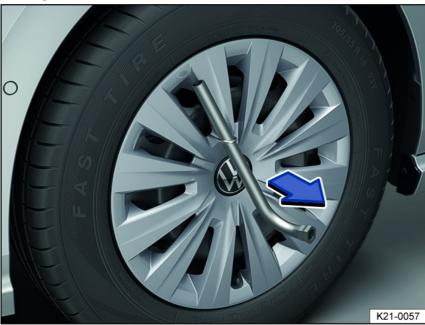
Fig. 177 Remove the wheel hub cover.
