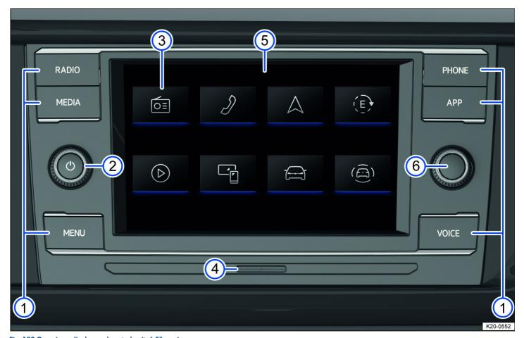
Fig. 132 Overview: display and control unit, 6.5" version.
