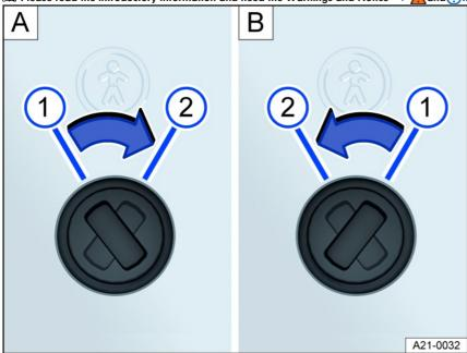
Fig. 56 Child safety lock: A left rear door, B right rear door.
