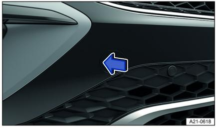
Fig. 155 In the right front bumper: Remove cover.
