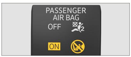
Fig. 29 In the center console: Indicator light (general example) for the activated front passenger's front airbag.
