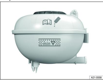
Fig. 167 In the engine compartment: markings on the engine coolant expansion tank.
