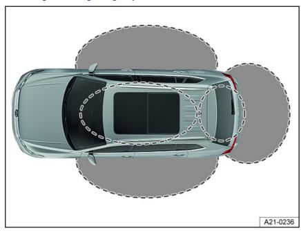
Fig. 50 Keyless Access: Sensor ranges (general example).
