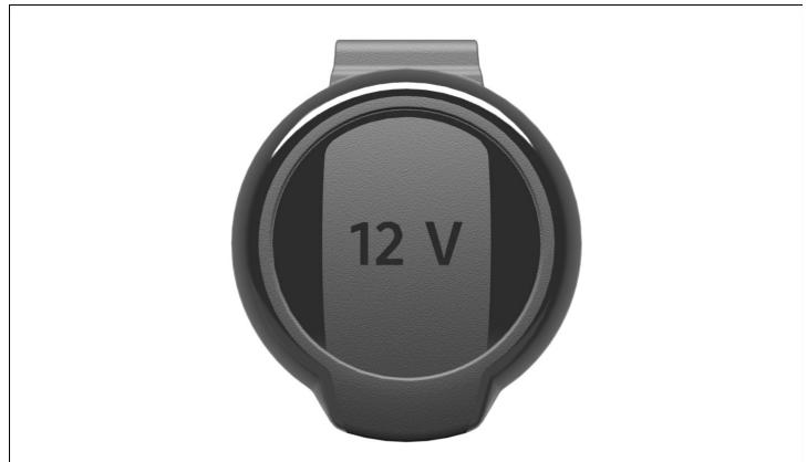
Fig. 128 In the front storage compartment or in the luggage compartment on the left-hand side: Folding 12 V socket (general example).
