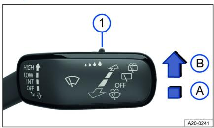
Fig. 81 On the right side of the steering column: windshield wiper lever.
