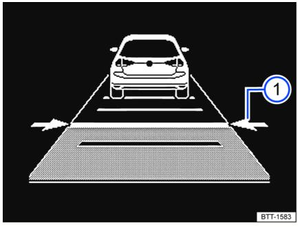
Fig. 114 In the instrument cluster display: set distance 🕦 (general example, ACC is regulating).
