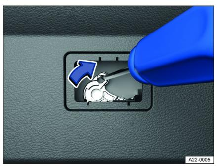
Fig. 60 In the luggage compartment: trunk lid emergency release.
