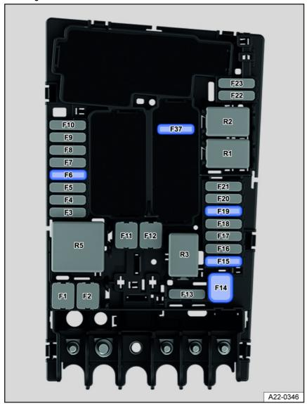
Fig. 148 Fuse locations in the engine compartment.
