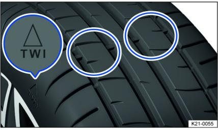
Fig. 172 Tire tread: tread wear indicator.
