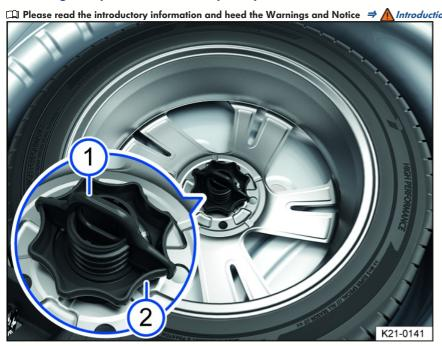
Fig. 175 In the luggage compartment: Handle to secure the spare wheel or compact spare wheel.
