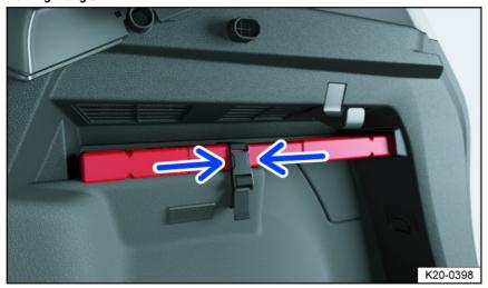
Fig. 42 In the luggage compartment on the right-hand side: Holder for the warning triangle.
