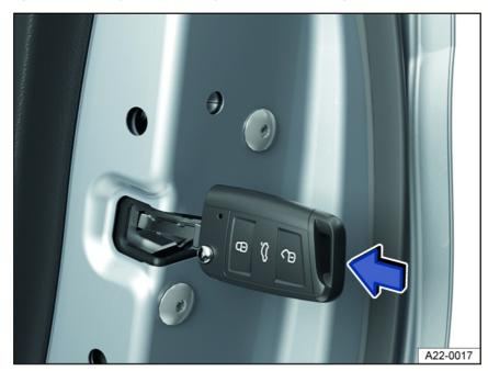
Fig. 55 In the front edge of a door: locking of the vehicle in an emergency with the key bit or emergency key (version 2).
