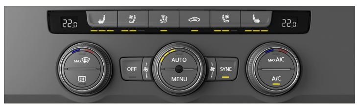
Fig. 87 In the upper section of the center console: Climate control bar for the Climatronic system.
