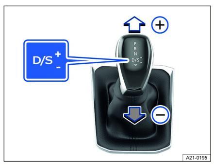
Fig. 95 Selector lever in Tiptronic position.
