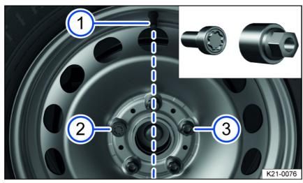
Fig. 184 Changing a tire: tire valve (1) and locations of the anti-theft wheel bolt (2) or (3).
