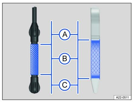
Fig. 165 Engine oil level markings on the oil dipstick (versions).
