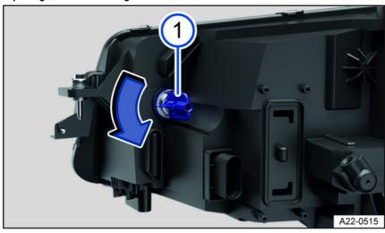
Fig. 146 In the right-side of the engine compartment: Rear side of the headlights.
