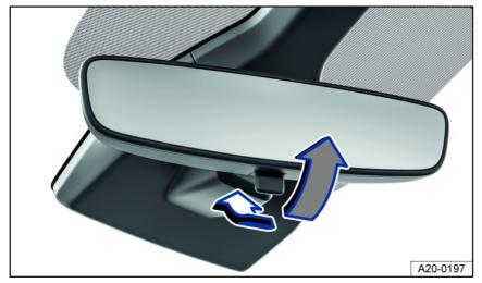
Fig. 83 On the windshield: manual dimming interior rearview mirror.
