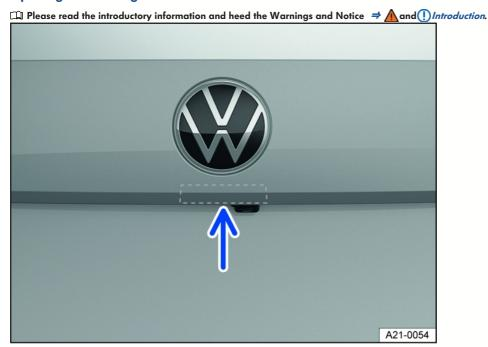
Fig. 57 In the trunk lid: Button to open the trunk lid (general example).
