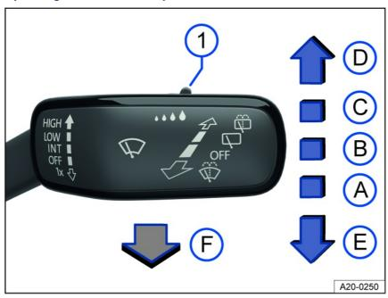
Fig. 79 On the right side of the steering column: operating the windshield wipers.
