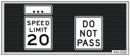
Fig. 20 In the instrument cluster display: Example of detected speed limits.
