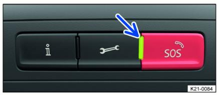
Fig. 43 In the roof console: Controls for call services and indicator light.
