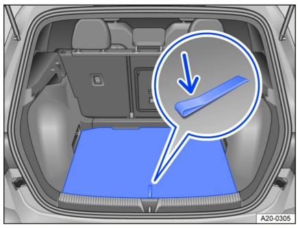
Fig. 134 In the luggage compartment: opening the luggage compartment floor.
