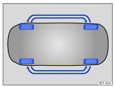
Fig. 171 General example: Diagram for rotating the wheels.
