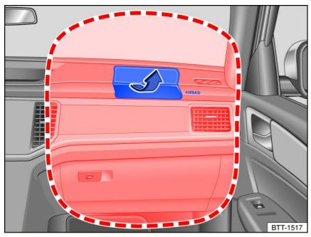
Fig. 31 Installation location and deployment zone of the front passenger's front airbag.
