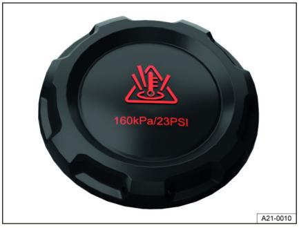
Fig. 166 In the engine compartment: cap on the engine coolant expansion tank.
