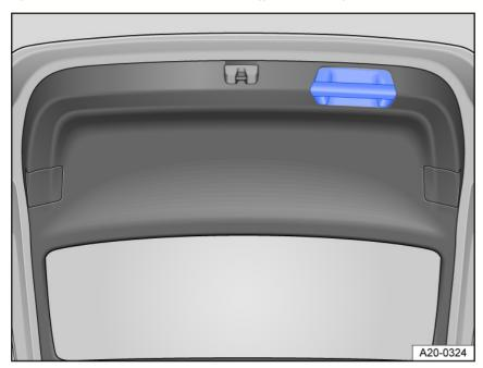
Fig. 58 In the open trunk lid: handle for closing the trunk lid.
