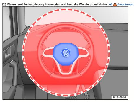
Fig. 30 Installation location and deployment zone of the driver's front airbag.
