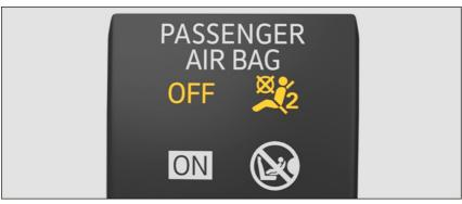
Fig. 28 In the center console: indicator light (general example) for the switched off front passenger's front airbag.
