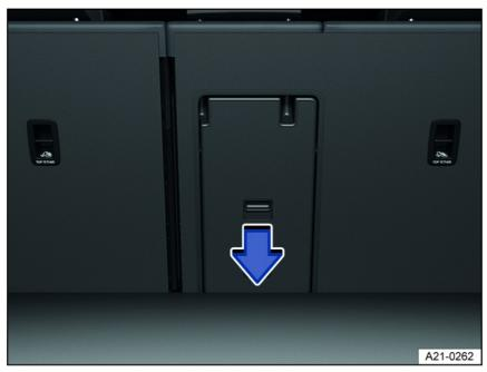
Fig. 138 Pass-through in the luggage compartment.
