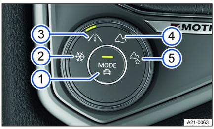
Fig. 100 In the center armrest: 4MOTION Active Control rotary switch.
