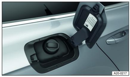
Fig. 140 Behind the fuel filler flap: fuel tank cap (general example)
