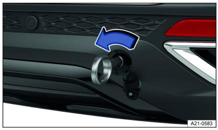
Fig. 158 In the right rear bumper: Screw in towing eye.
