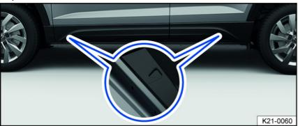
Fig. 180 Mounting points for the vehicle jack.
