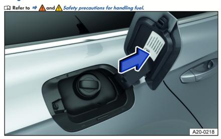
Fig. 139 On the inside of the fuel filler flap: fuel label (general example)
