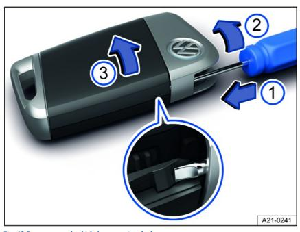
Fig. 48 Remote control vehicle key: opening the battery compartment cover.
