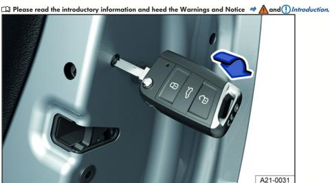
Fig. 54 In the front edge of a door: locking of the vehicle in an emergency with the key bit or emergency key (version 1).
