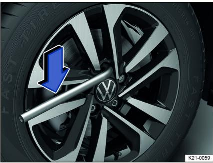
Fig. 183 Wheel change: removing wheel bolts with the lug wrench.
