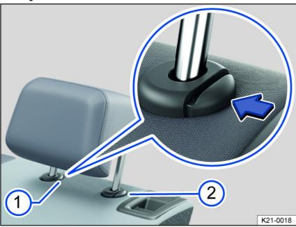
Fig. 72 Removing the rear head restraint (general example).
