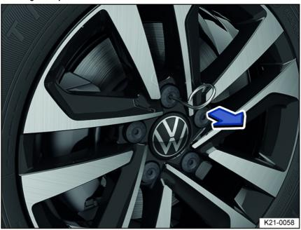
Fig. 178 Remove the caps from the wheel bolts.
