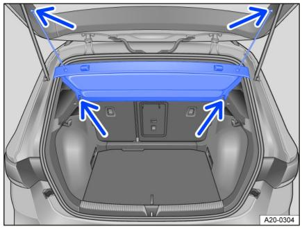
Fig. 133 In the luggage compartment: Installing and removing the luggage compartment cover.
