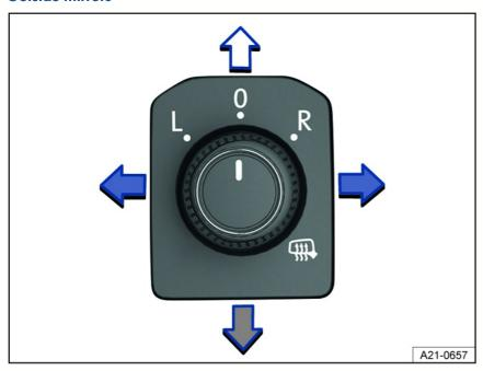
Fig. 84 In the driver door: knob for the outside mirrors.
