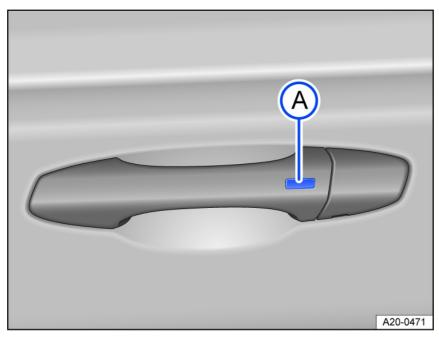
Fig. 51 In door handle: Button to unlock or lock.
