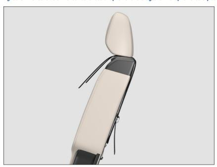
Fig. 39 On the rear side of the rear bench seat: attached top tether safety belt.
