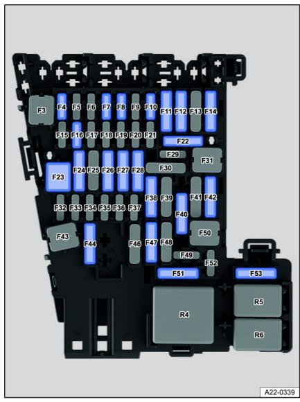
Fig. 150 Fuse assignment in the instrument panel.
