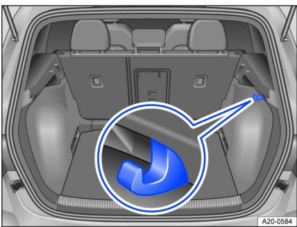
Fig. 136 Shopping bag hooks on the left and right of the luggage compartment.
