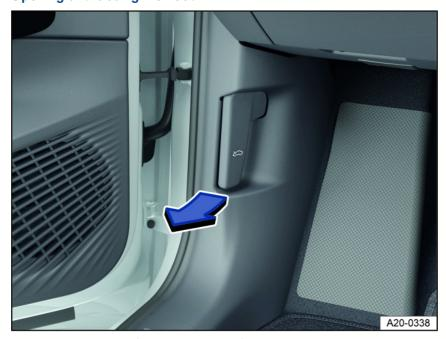
Fig. 159 In the driver's side footwell: Release lever for the hood (general example).
