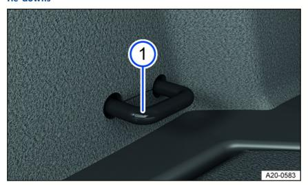
Fig. 135 In the luggage compartment: Tie-down (general example).
