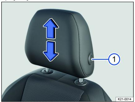
Fig. 69 Adjusting the front head restraint (general example).
