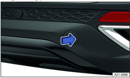
Fig. 157 In the right rear bumper: Remove cover.
