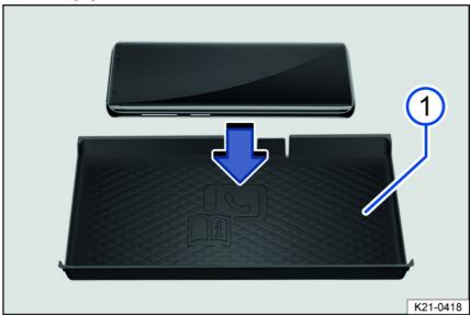
Fig. 129 General example: Storage compartment with a liner pad for wireless charging in the center console.
