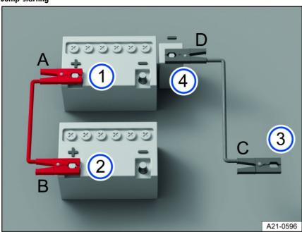
Fig. 154 Diagram for connecting the jumper cables.
