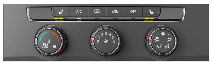
Fig. 88 In the upper section of the center console: Climate control bar for the manual climate control system.
