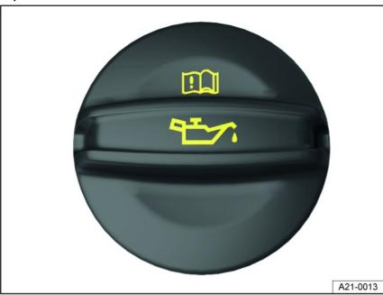
Fig. 164 In the engine compartment: engine oil filler cap (general example).
