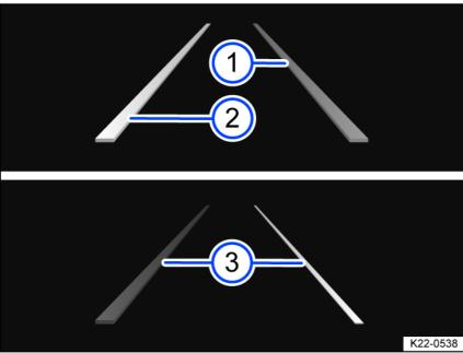
Fig. 115 In the instrument cluster display: displays of Lane Assist
