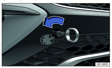
Fig. 156 In the right front bumper: Screw in towing eye.
