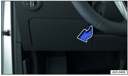
Fig. 149 On the driver side in the instrument panel: fuse box cover (general example).
