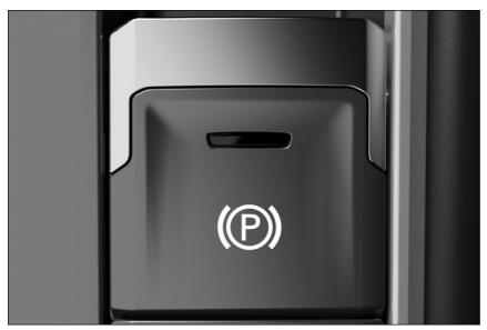
Fig. 120 In the center console: button for the electronic parking brake.
