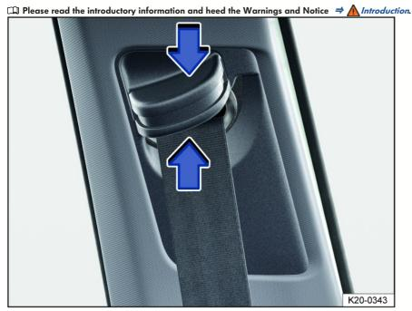
Fig. 27 Next to the front seats: safety belt height adjuster.
