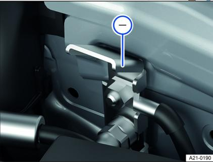
Fig. 153 In the engine compartment: Negative terminal jump-start point.
