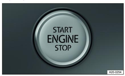
Fig. 91 In the lower area of the center console: starter button for starting the engine.
