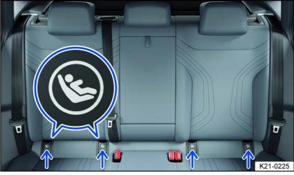
Fig. 36 On the outer seats in the rear bench seat: Designation of the ISOFIX/lower LATCH anchorage points for child restraints.
