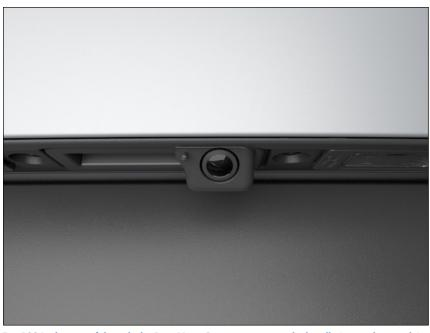
Fig. 188 In the rear of the vehicle: Rear View Camera system on the handle (general example).
