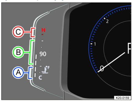
Fig. 17 Coolant temperature gauge in the Volkswagen Digital Cockpit Pro (general example).
