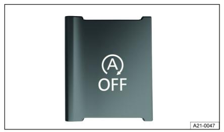
Fig. 93 In the lower section of the center console or, depending on the vehicle equipment, in the Infotainment system: Button for the start-stop system.
