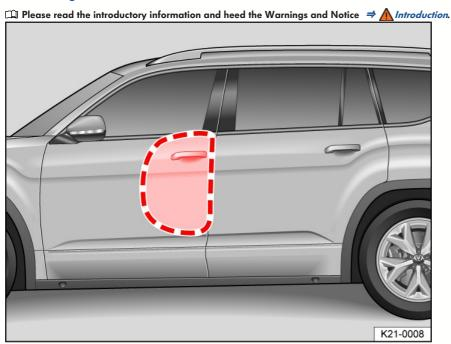
Fig. 32 In the vehicle interior on both sides of the vehicle: Deployment zone of the front side airbag.
