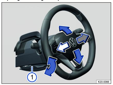
Fig. 63 Under the steering wheel in the steering column trim panel: lever to adjust the steering wheel position manually (general example).
