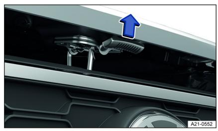
Fig. 160 Above the radiator grille: Opening lever for the hood (general example).
