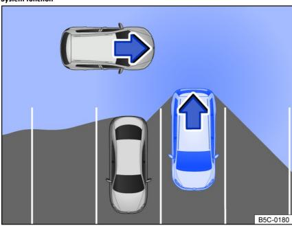
Fig. 126 Rear Traffic Alert, general example: monitored area around the vehicle that is exiting a parking space.
