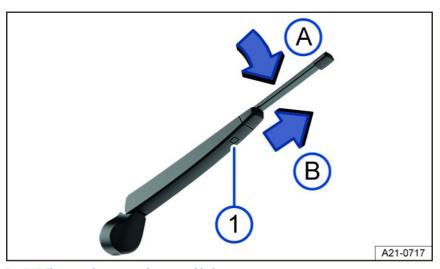
Fig. 145 Changing the rear window wiper blade.
