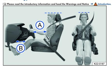
Fig. 21 General example: correct distance between the driver and the steering wheel, correct safety belt routing and correct head restraint adjustment.
