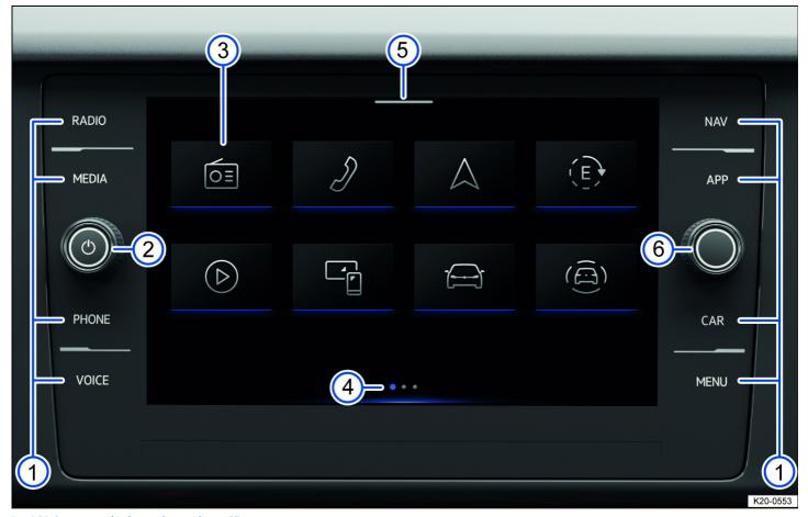
Fig. 131 Overview: display and control unit, 8" version.
