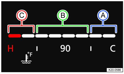
Fig. 18 Coolant temperature gauge in the Volkswagen Digital Cockpit Basic (general example).
