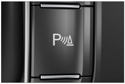
Fig. 122 In the center console: Park Distance Control button (depending on the vehicle equipment).
