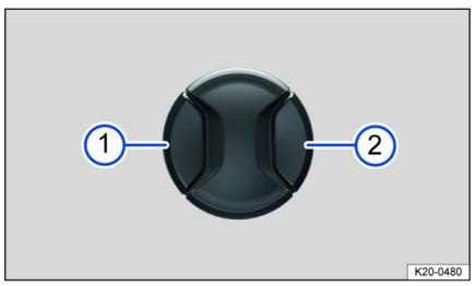
Fig. 67 Switch on the driver seat: Adjusting the lumbar support.
