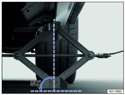
Fig. 182 Jack is positioned on the left side of the vehicle at the rear.
