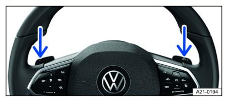
Fig. 96 Steering wheel with shift paddles for Tiptronic.
