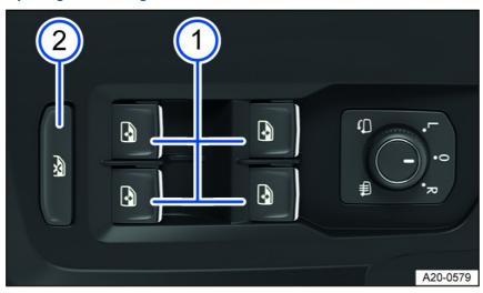
Fig. 61 In the driver door: Power window buttons.
