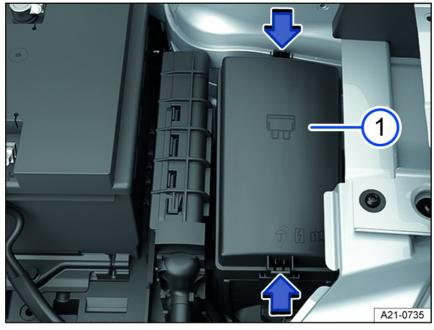
Fig. 147 In the engine compartment: Fuse box.
