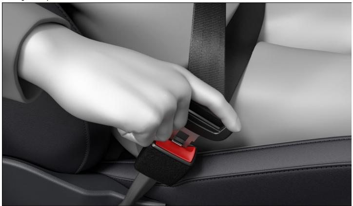
Fig. 23 Inserting the buckle tongue into the safety belt buckle.
