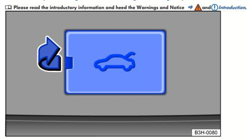
Fig. 59 In the trunk lid: cover for the trunk lid emergency release.
