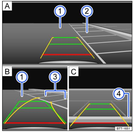
Fig. 124 Infotainment system: Parking perpendicular to the road.
