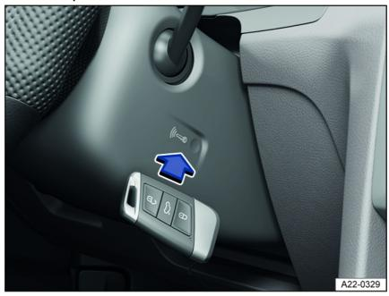
Fig. 92 On the right side of the steering column: emergency start function on vehicles with Keyless Access with push-button start.
