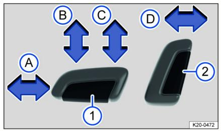
Fig. 66 Switch on the driver seat: Adjusting the front seat forward/back, the height and angle of the seat surface, and the front seat backrest.
