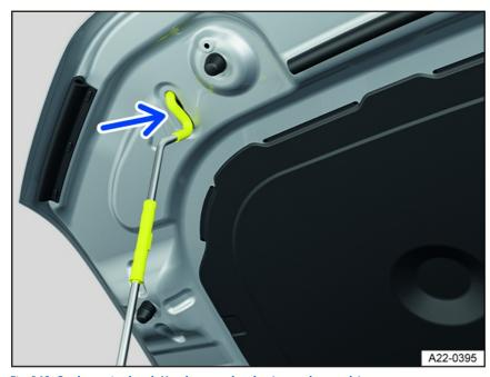
Fig. 162 On the engine hood: Hood support bracket (general example).
