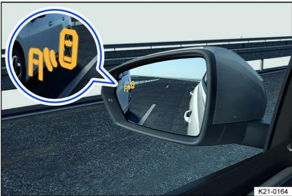
Fig. 119 In the mirror glass of the outside mirrors: Blind Spot Monitor indicator.
