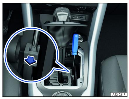
Fig. 98 In the center console: manually release the Automatic Shift Lock (ASL) (variant 2).
