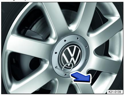
Fig. 176 Remove the hubcap.
