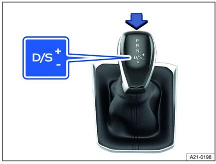
Fig. 94 Selector lever with lock button (arrow) on an automatic transmission.
