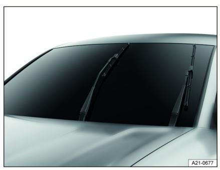
Fig. 143 Windshield wipers in service position (general example).
