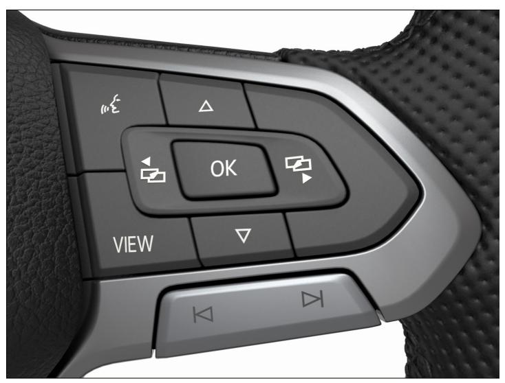
Fig. 10 Right side of the multi-function steering wheel: Operating the Volkswagen Digital Cockpit Pro (variant 1).
