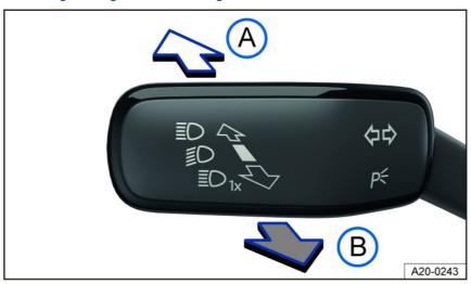
Fig. 78 On the left side of the steering column: turn signal and high beam lever.
