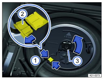
Fig. 173 In the luggage compartment: removing the subwoofer (version 1).
