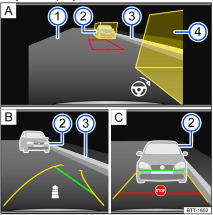
Fig. 125 Infotainment system: Parking parallel to the road.
