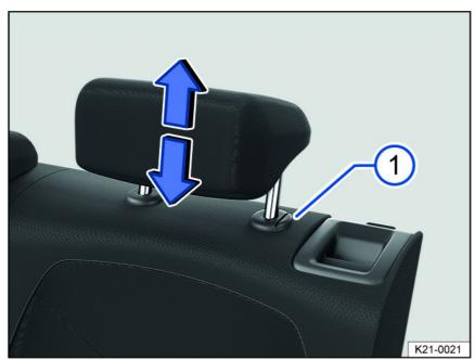
Fig. 70 Adjusting the rear head restraint (general example).
