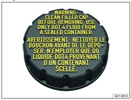
Fig. 168 In the engine compartment: cap on the brake fluid reservoir.
