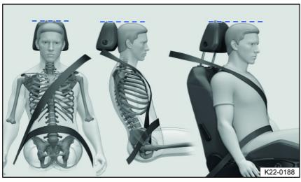
Fig. 25 Correct safety belt positioning and correct head restraint adjustment.
