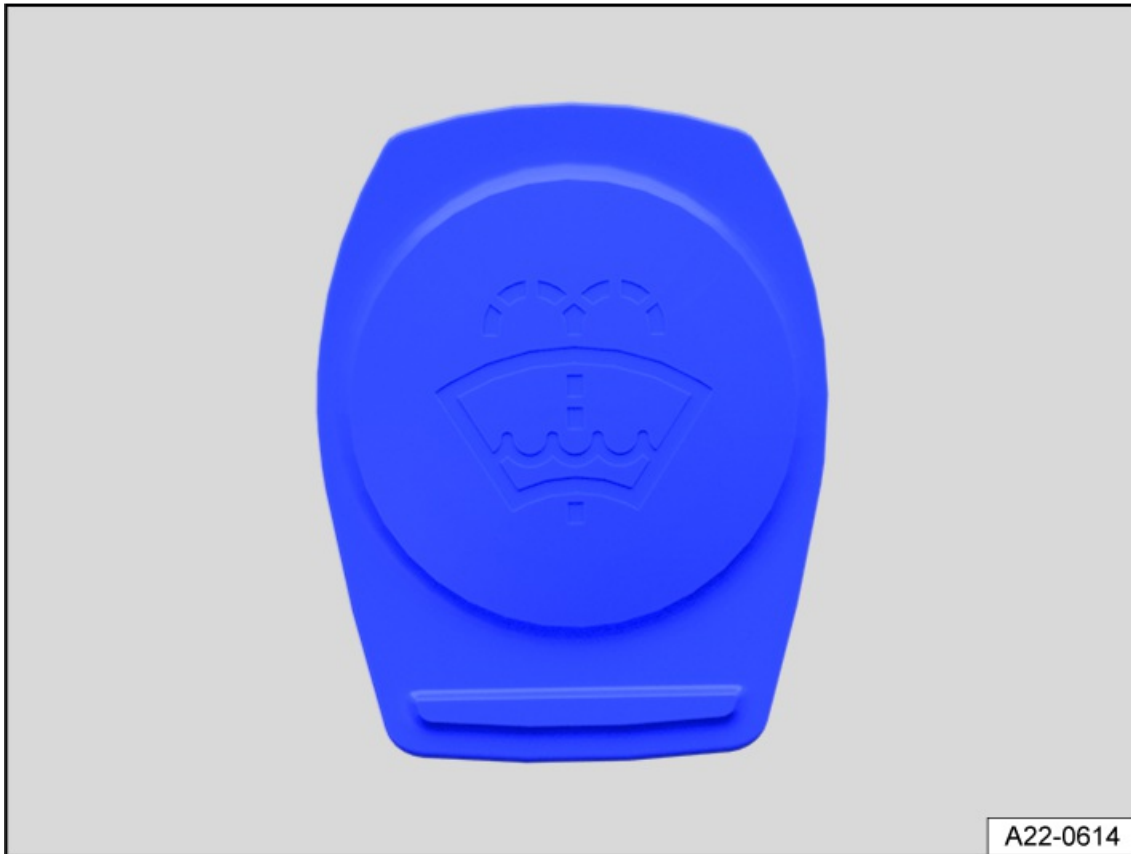
Fig. 170 In the hood space: Cap on the washer fluid reservoir (general example).
