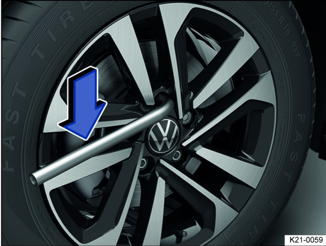
Fig. 187 Loosening wheel bolts.
