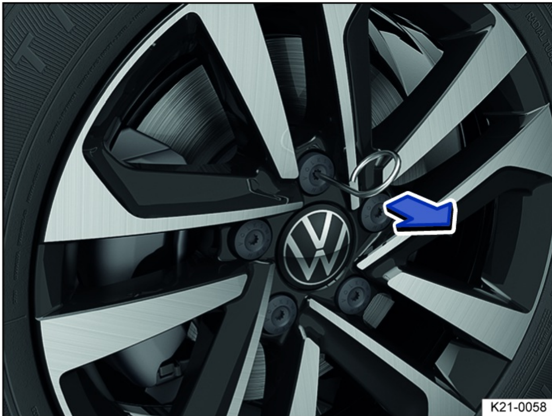
Fig. 186 Remove the caps from the wheel bolts.
