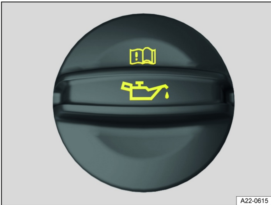
Fig. 173 In the hood space: engine oil filler cap (general example).
