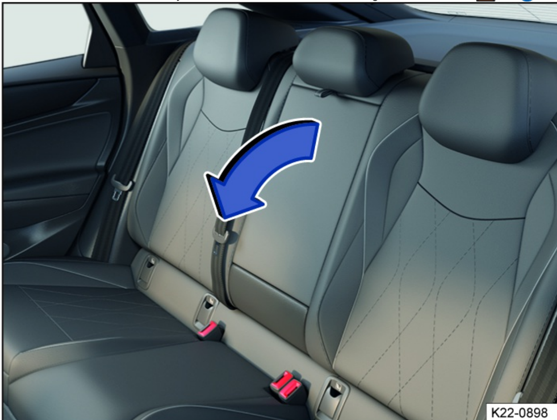
Fig. 123 In the backrest of the center seat: folding rear center armrest (general example).
