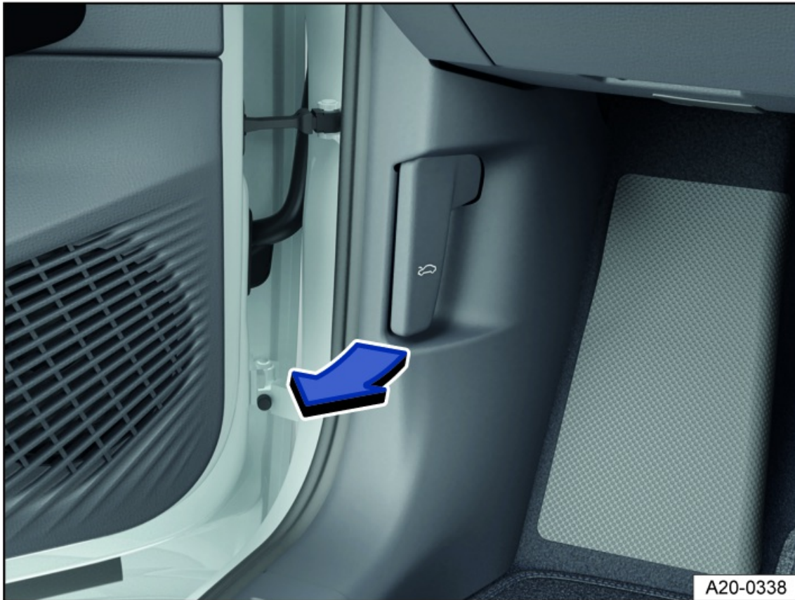
Fig. 167 In the driver's side footwell: Release lever for the hood (general example).
