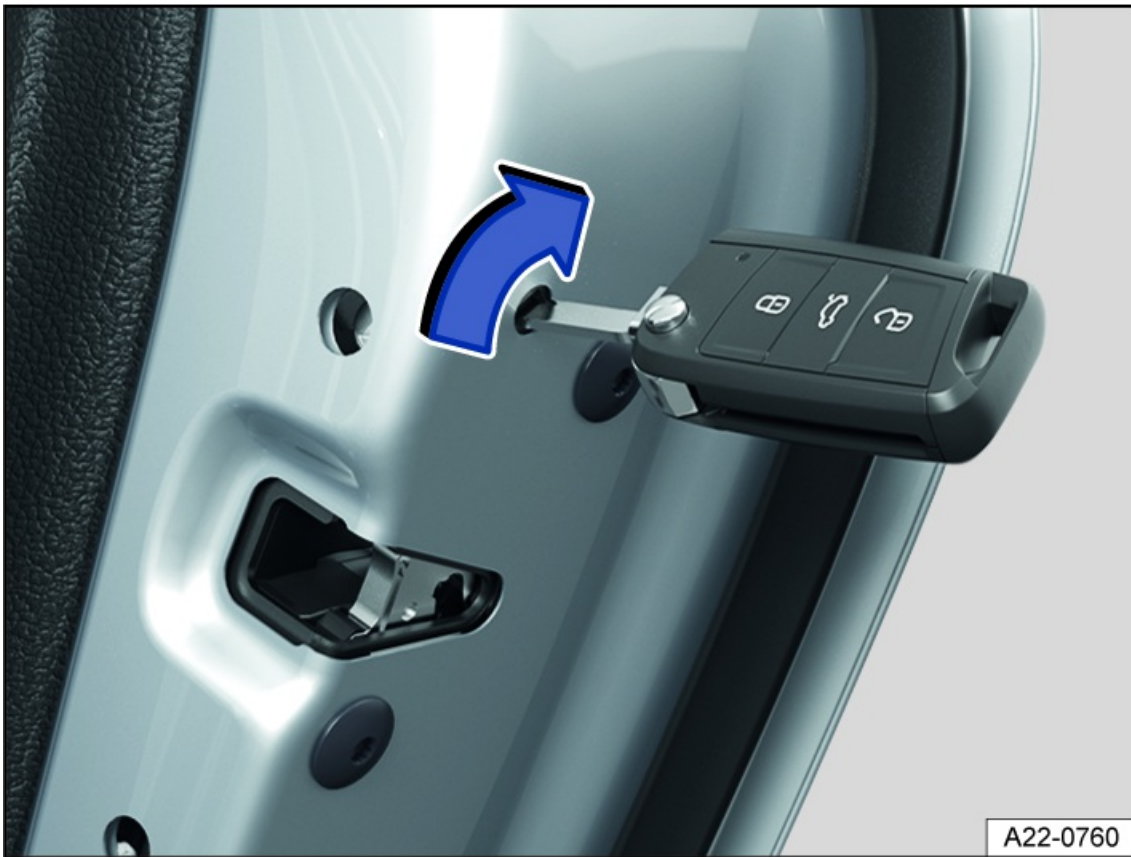
Fig. 47 On the front of the right rear door: emergency locking the vehicle with the vehicle key (general example).
