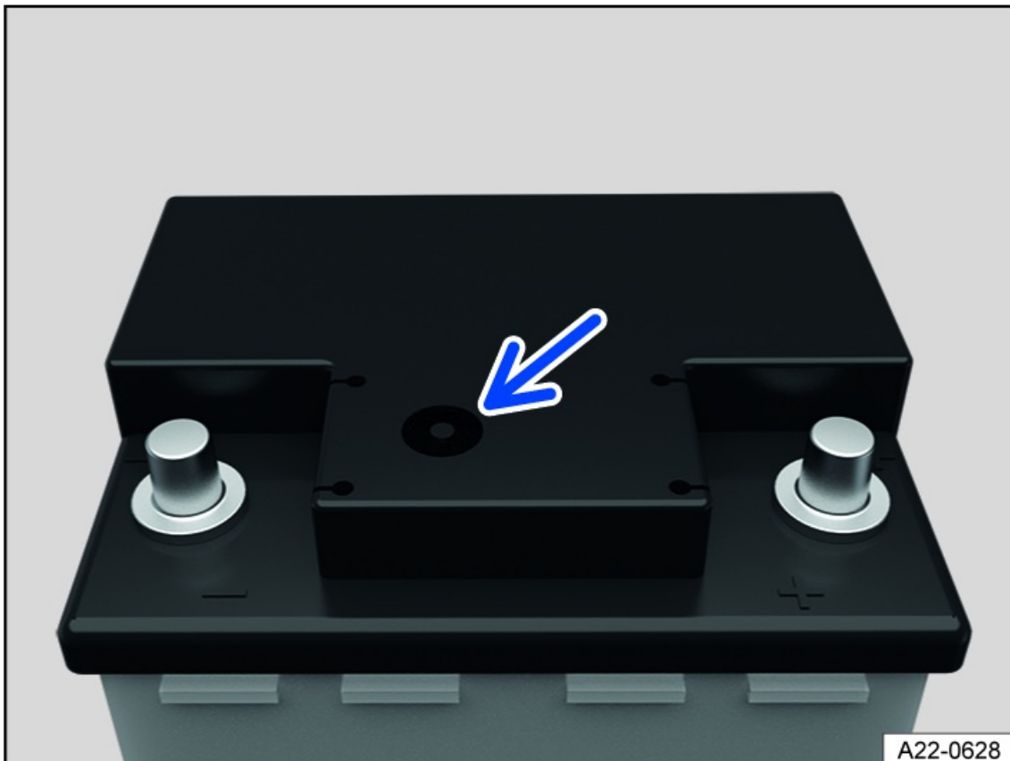
Fig. 178 On the top of the 12 V vehicle battery: Window (general example).
