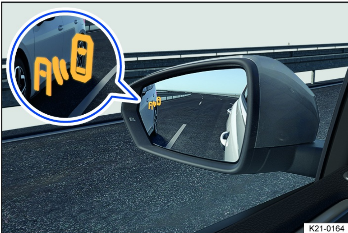
Fig. 110 In the mirror glass of the outside mirrors: indicator of Side Assist.
