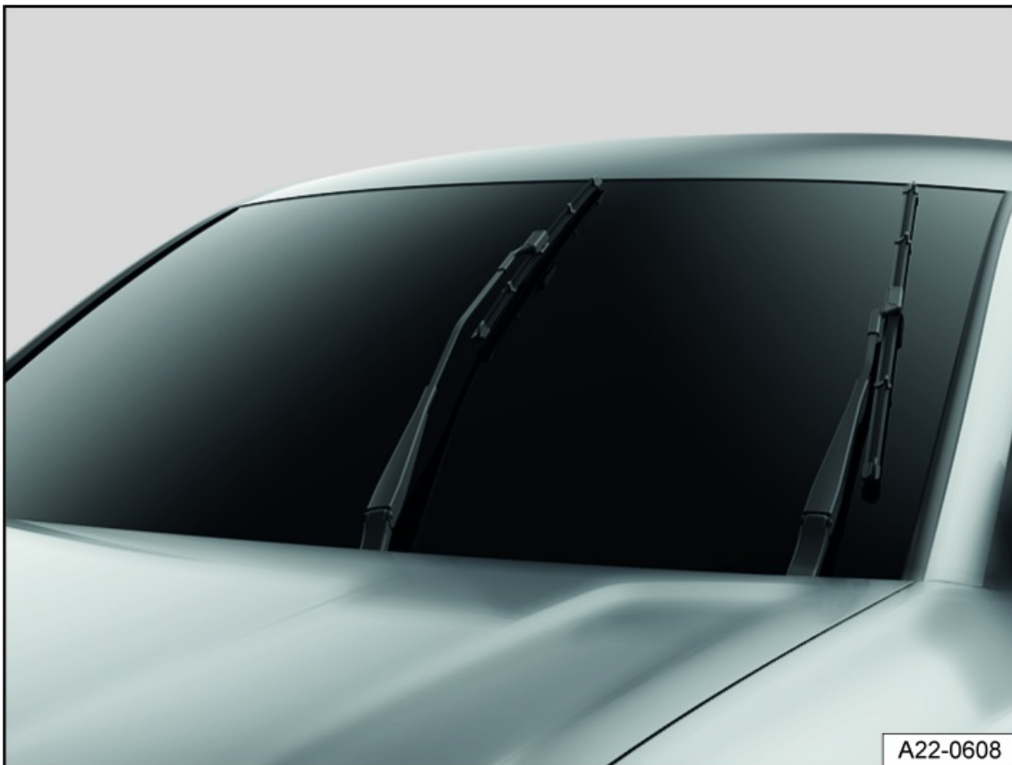
Fig. 149 Windshield wipers in service position (general example).
