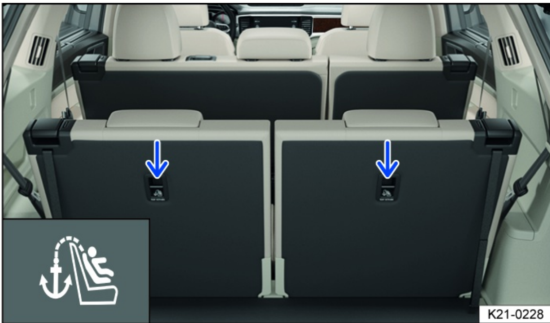
Fig. 28 On the back of the rear seats of the third-row seats: top tether anchorages for the top tether safety belt.
