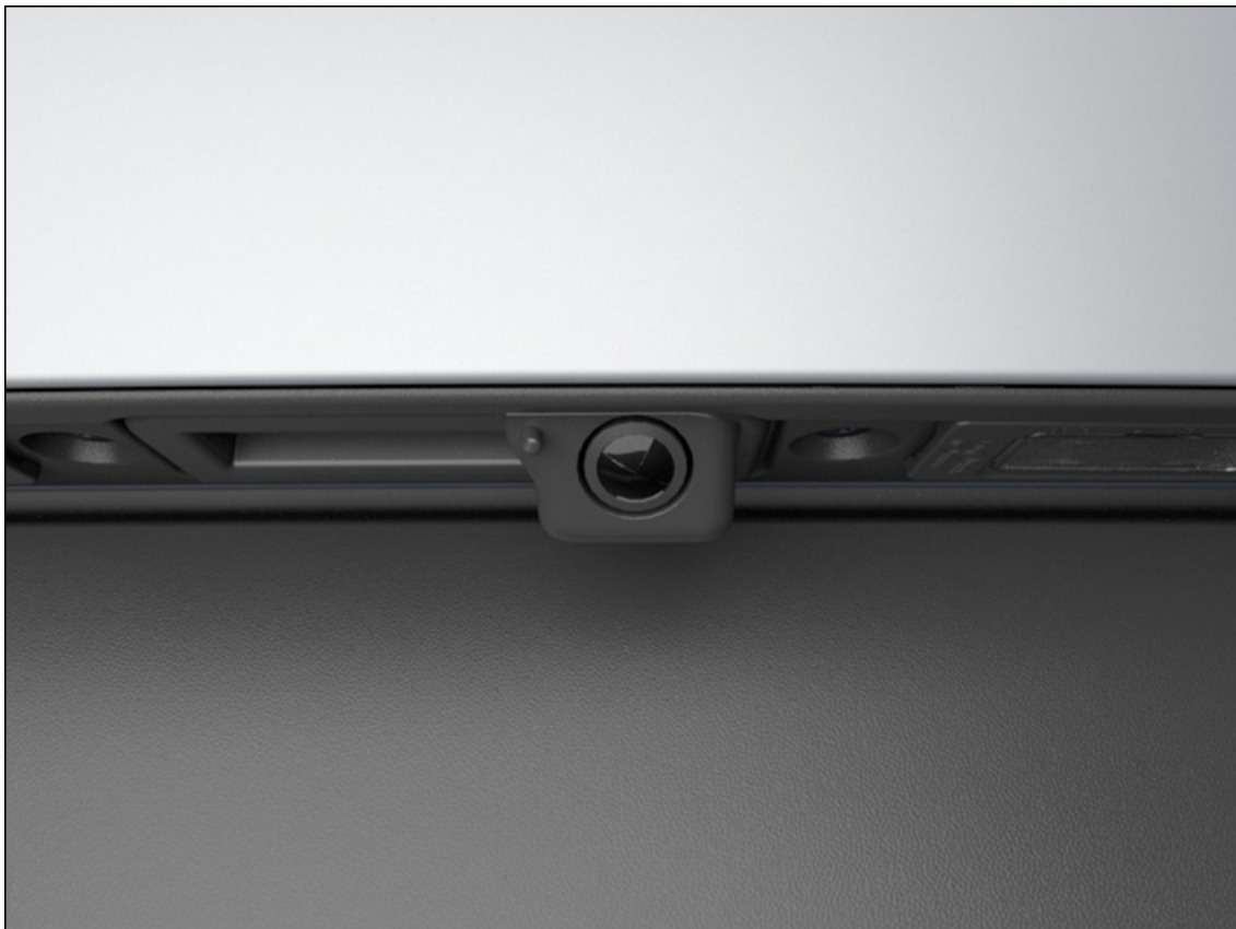
Fig. 195 In the rear of the vehicle: Rear View Camera system on the handle (general example).
