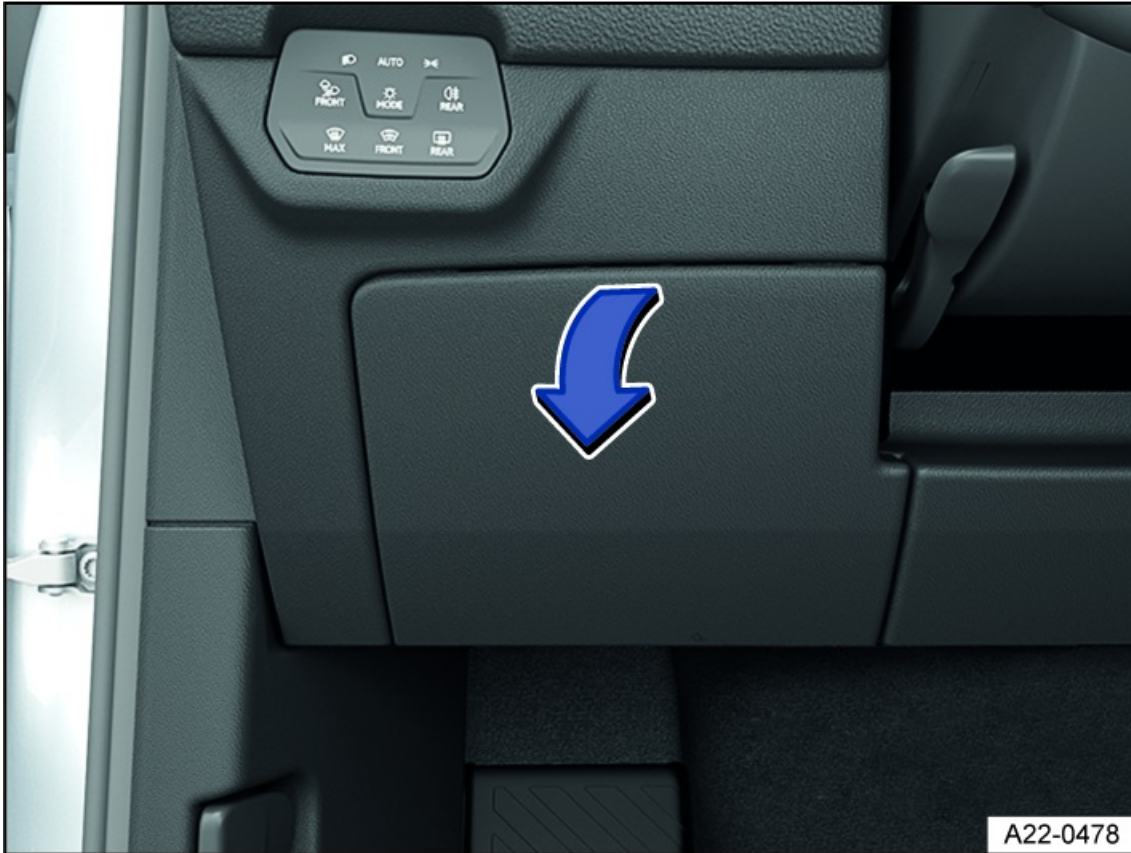
Fig. 154 On the driver side in the instrument panel: fuse box cover.
