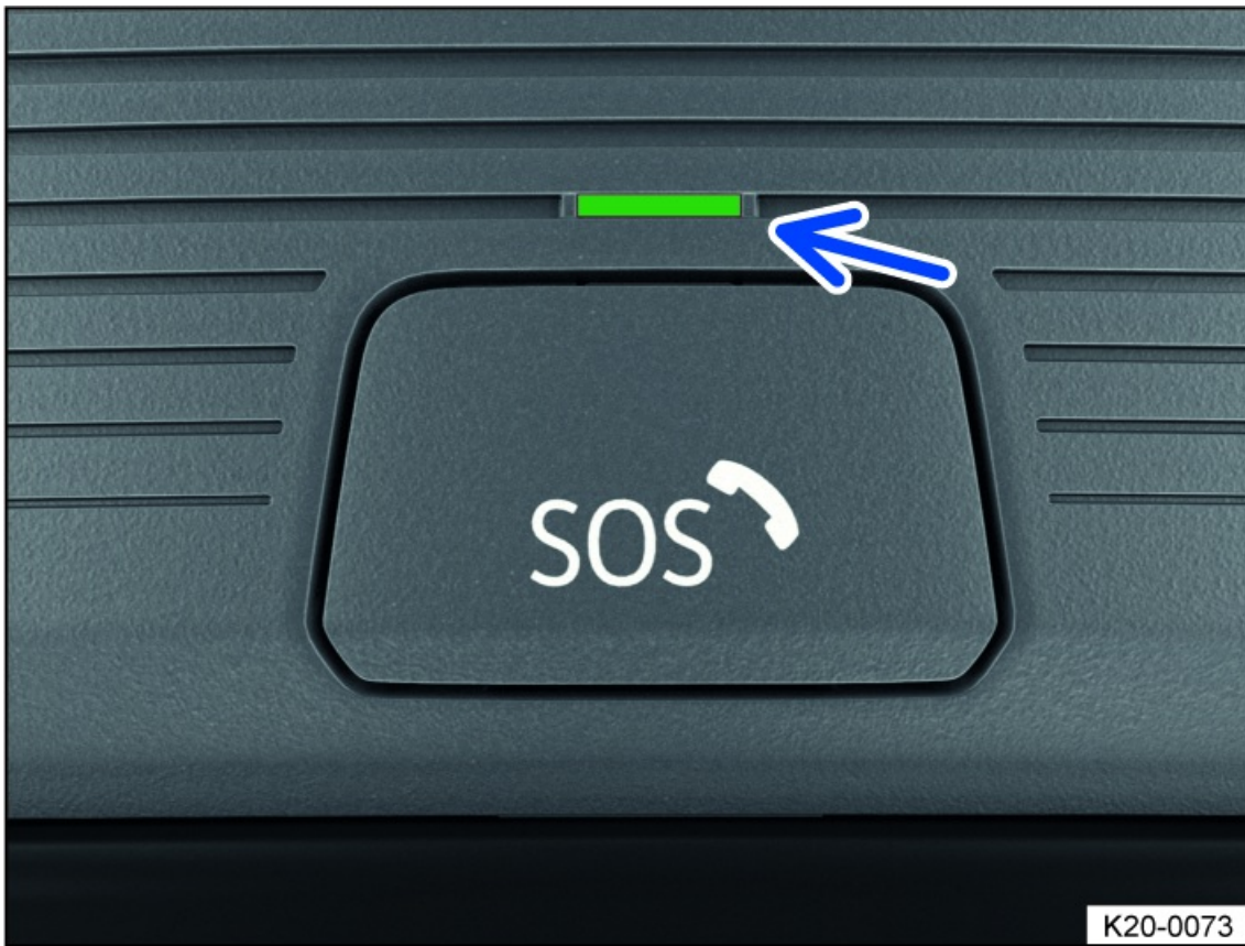
Fig. 34 Located on the roof console: Emergency Call Service button (behind a button cover) and indicator light.
