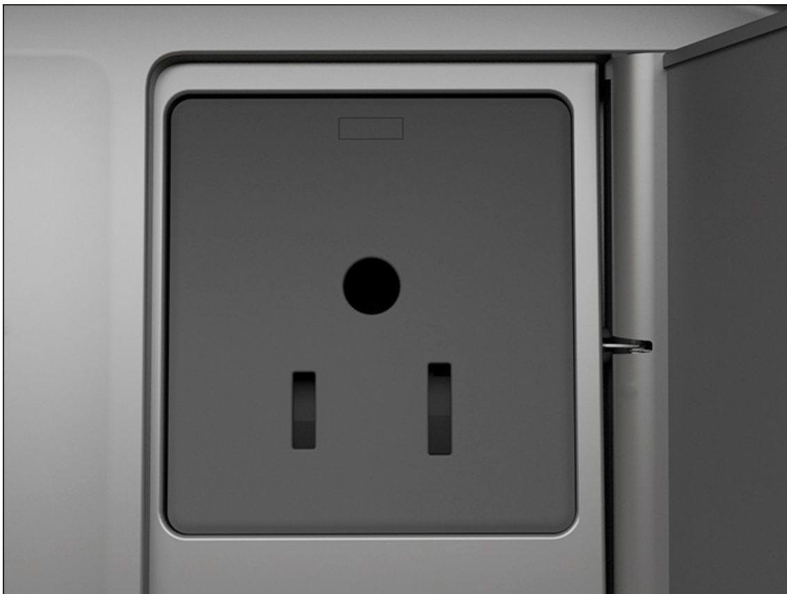
Fig. 126 In the center console at the rear: 115 V socket (depending on the vehicle equipment).
