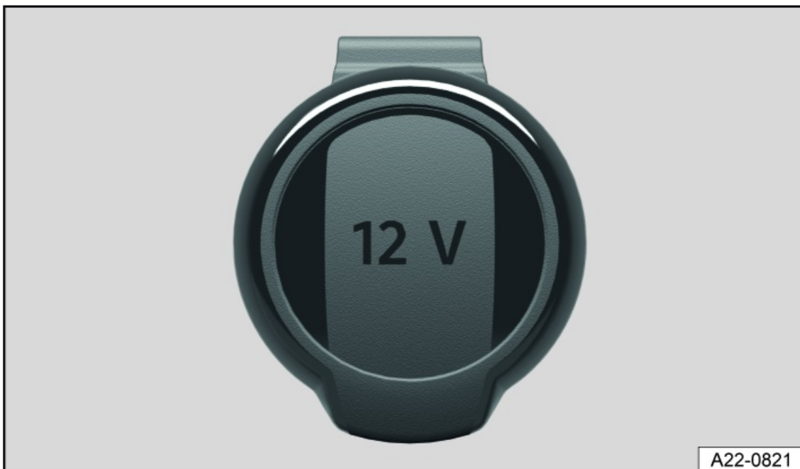
Fig. 125 In the lower part of the center console, at the rear of the center console or on the left-hand side of the luggage compartment: Hinged 12-volt socket (general example).
