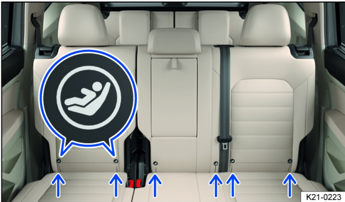
Fig. 25 On the second-row rear seats: designation and symbol showing the ISOFIX/lower LATCH anchorage points for child restraints.
