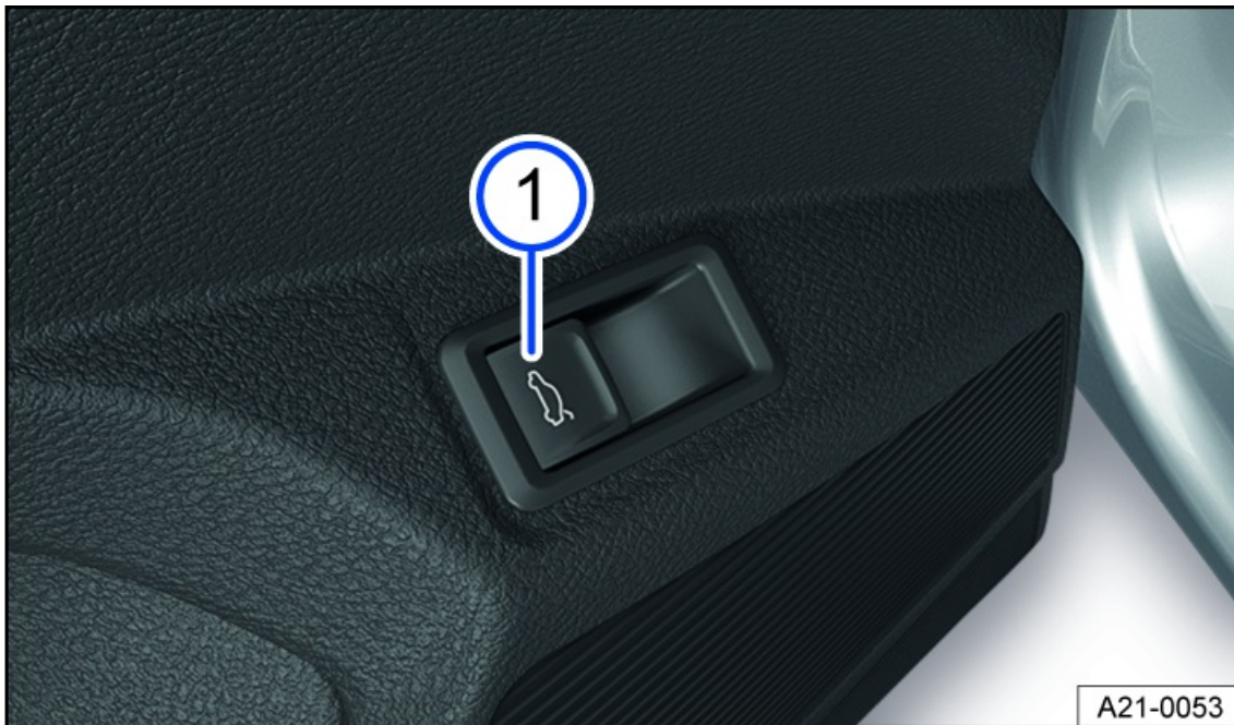
Fig. 45 In the driver's door: Button for powered opening of the trunk lid (general example).
