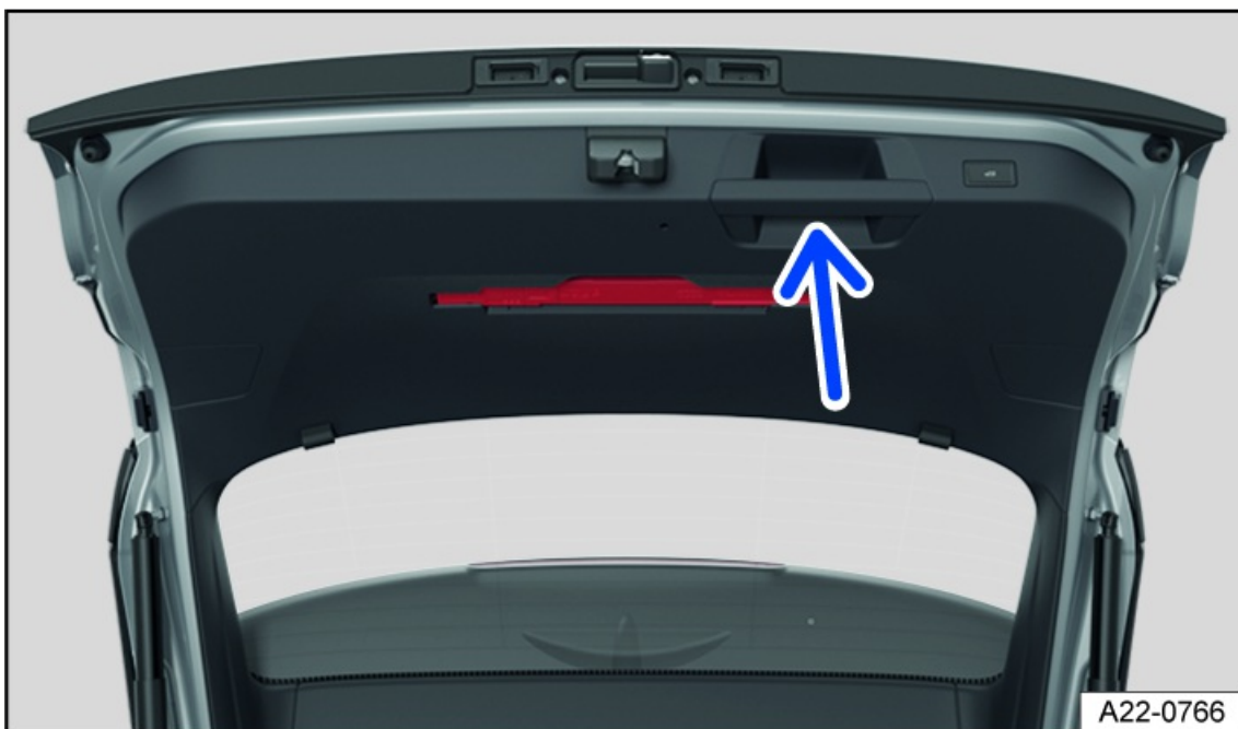
Fig. 50 In the open trunk lid: handle for closing the trunk lid (general example).
