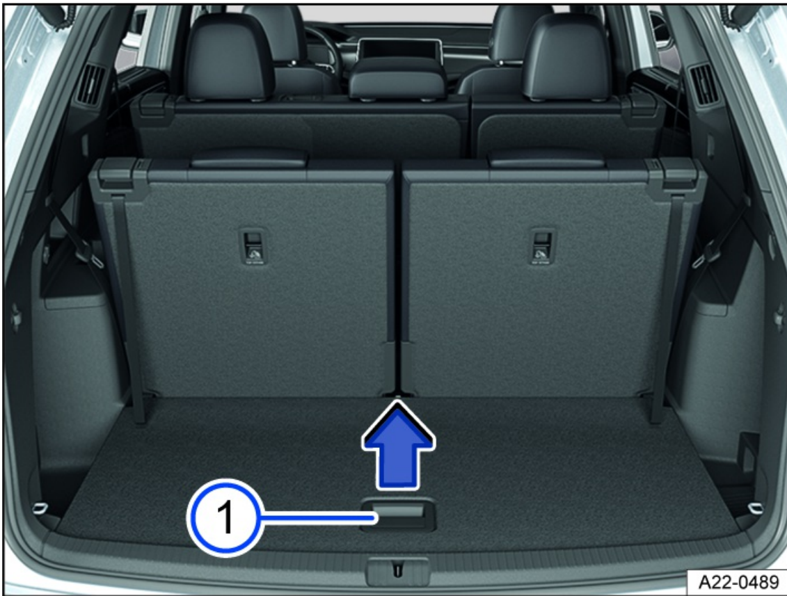
Fig. 132 In the luggage compartment: opening the luggage compartment floor.
