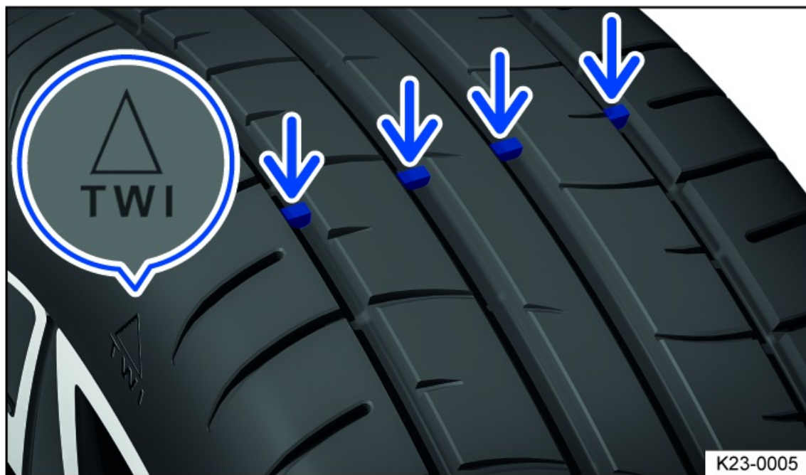
Fig. 181 In the tread grooves: wear indicator.
