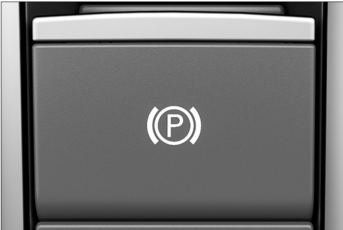
Fig. 111 In the center console: button for the electronic parking brake.
