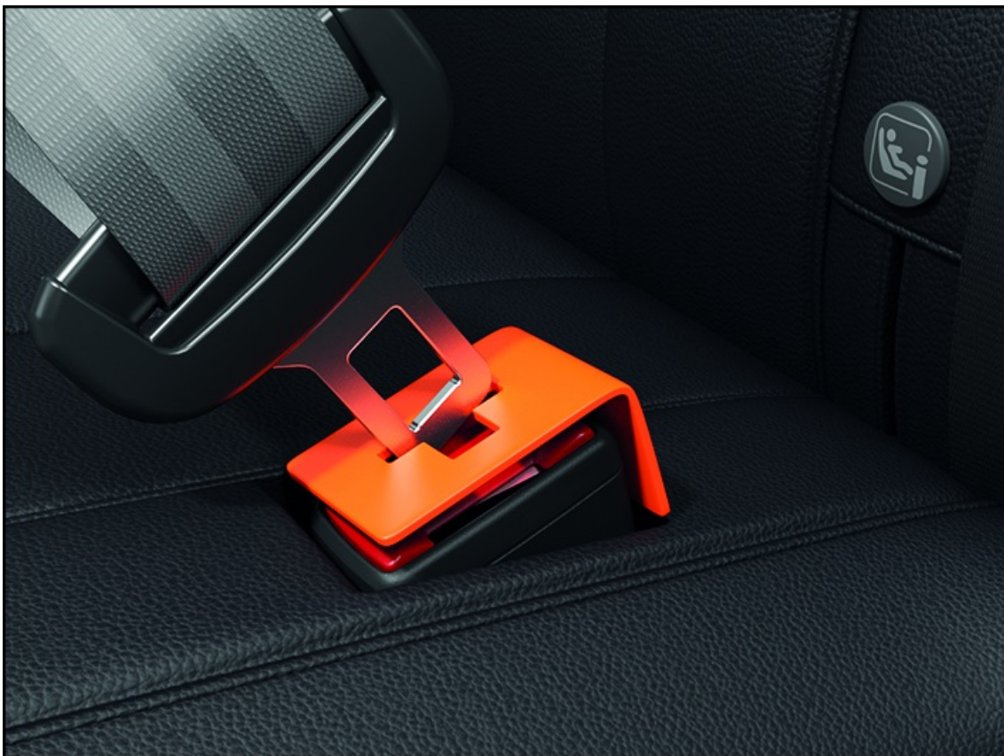
Fig. 32 In the second-row seats: removing the protective cap for belt buckles (general example).
