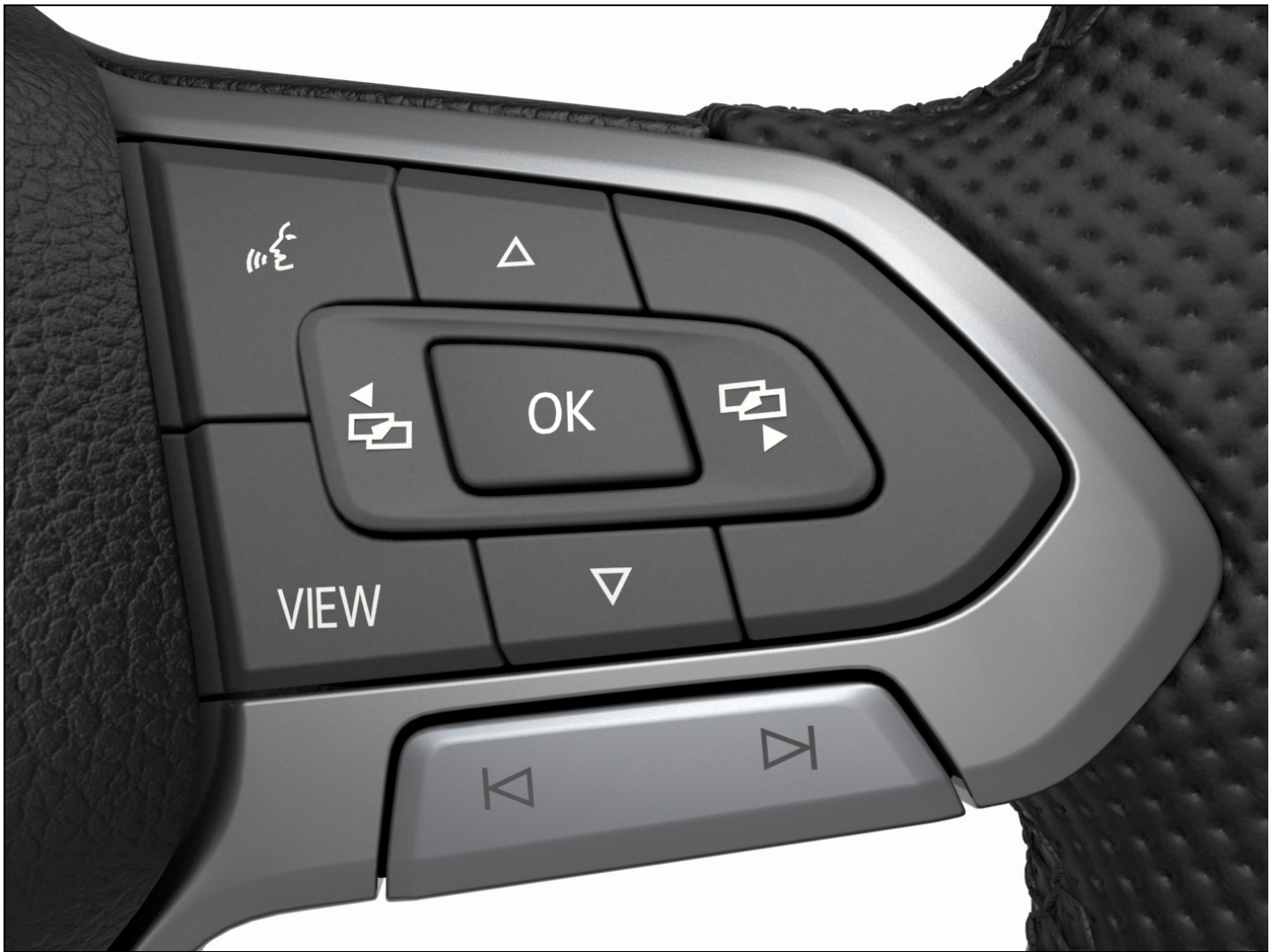
Fig. 10 Right side of the multi-function steering wheel: Operating the Volkswagen Digital Cockpit (variant 1).
