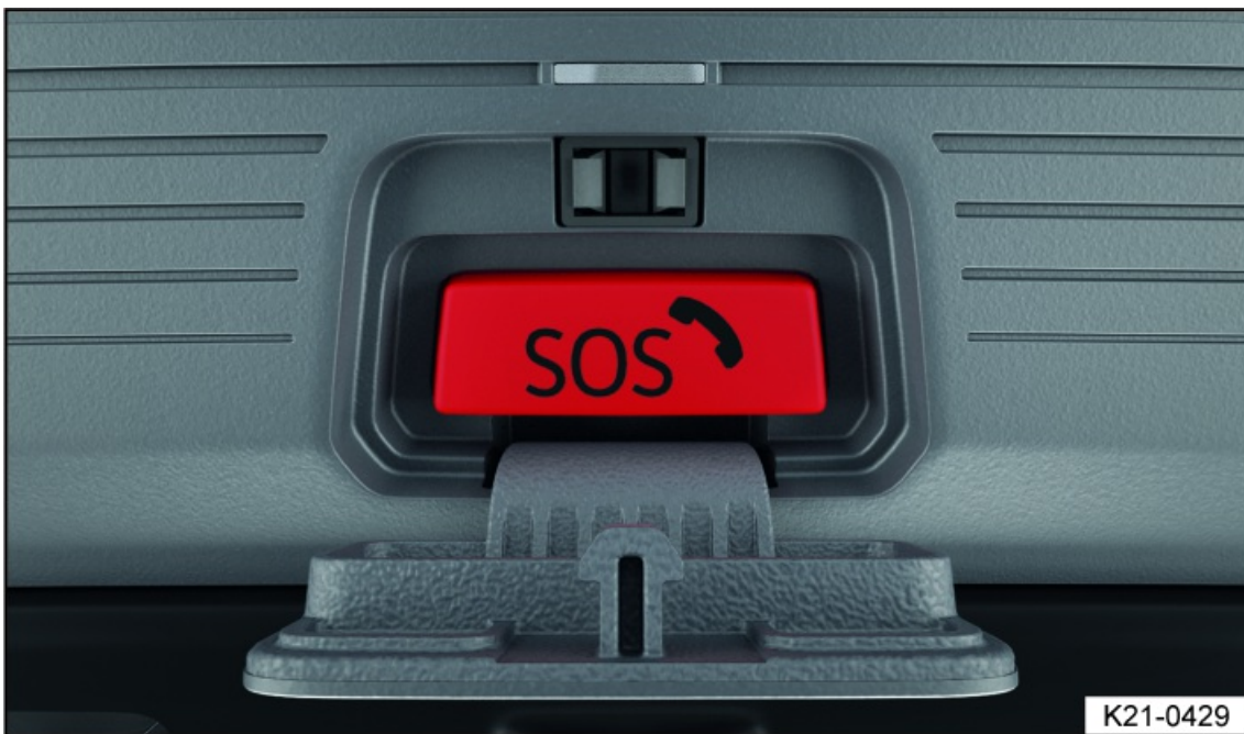
Fig. 35 Located on the roof console: Emergency Call Service button.
