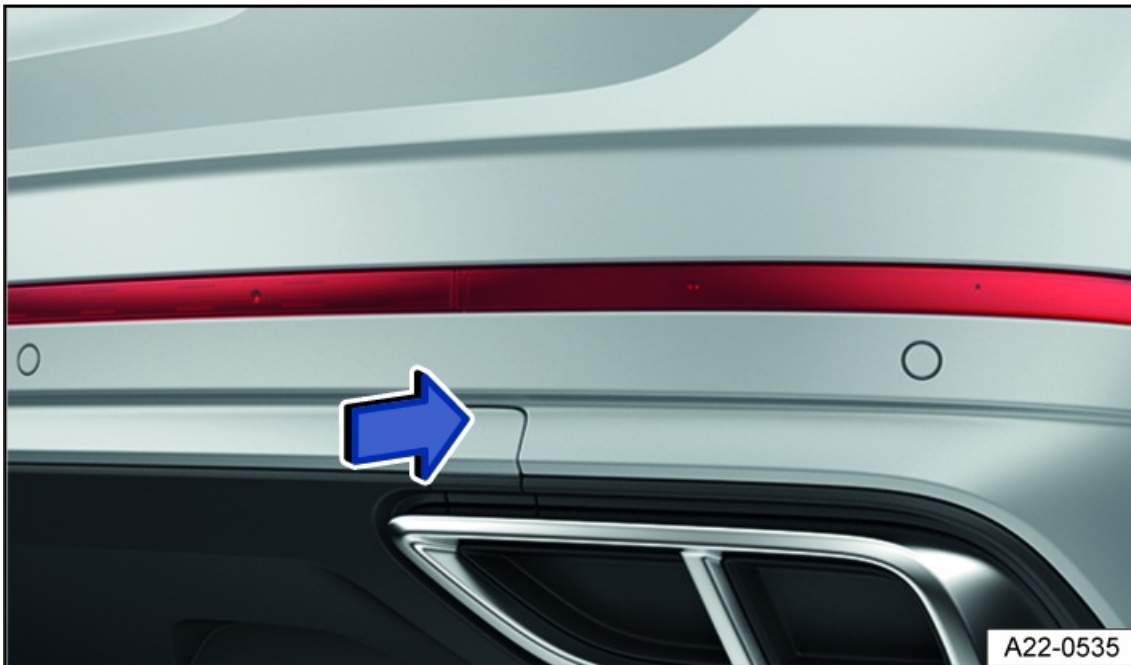
Fig. 163 In the right rear bumper: Remove the cover, variant 2.
