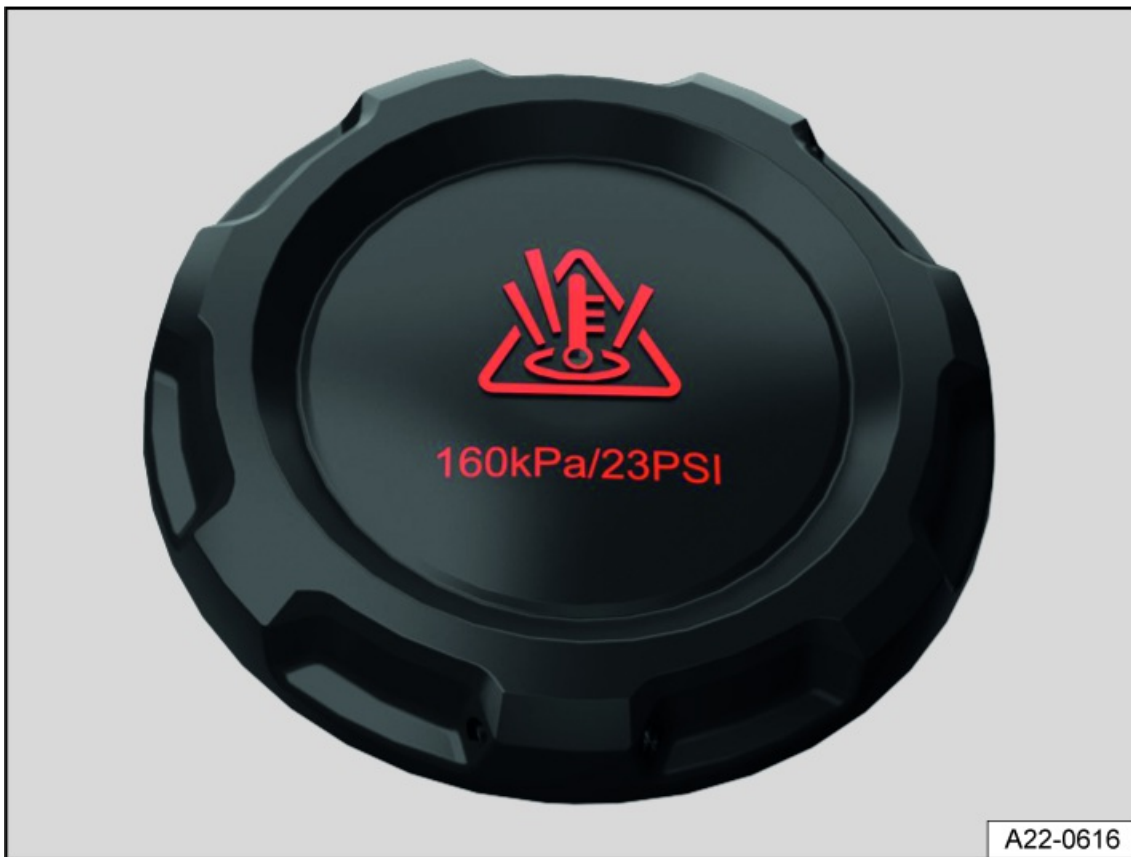
Fig. 175 In the hood space: cap of the coolant expansion tank (general example).
