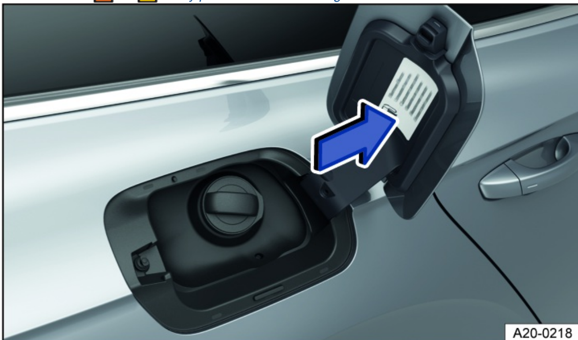
Fig. 145 On the inside of the fuel filler flap: fuel label (general example)
