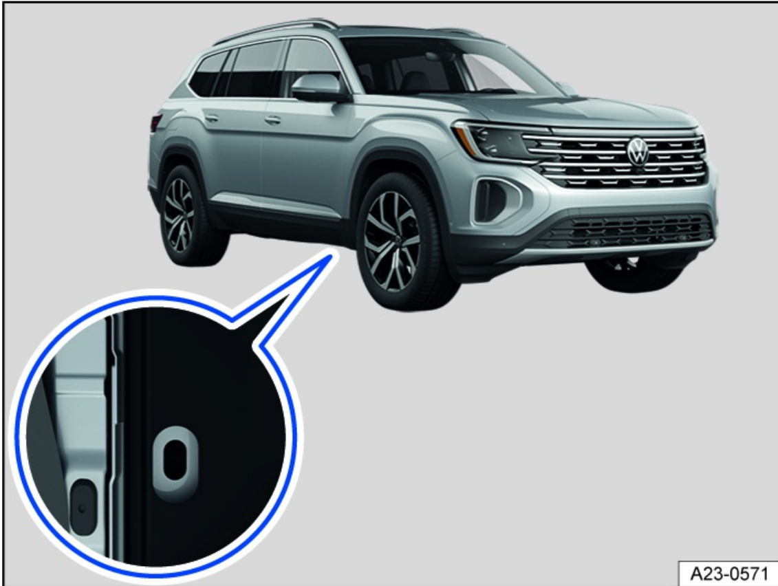
Fig. 161 Behind the front wheels on the left and right: attachment points for a tow truck under a cover.
