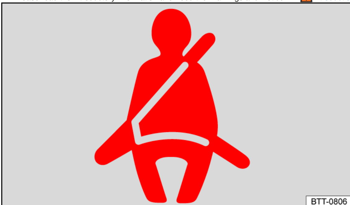
Fig. 15 In the instrument cluster display: warning light for the fasten seat belts reminder.
