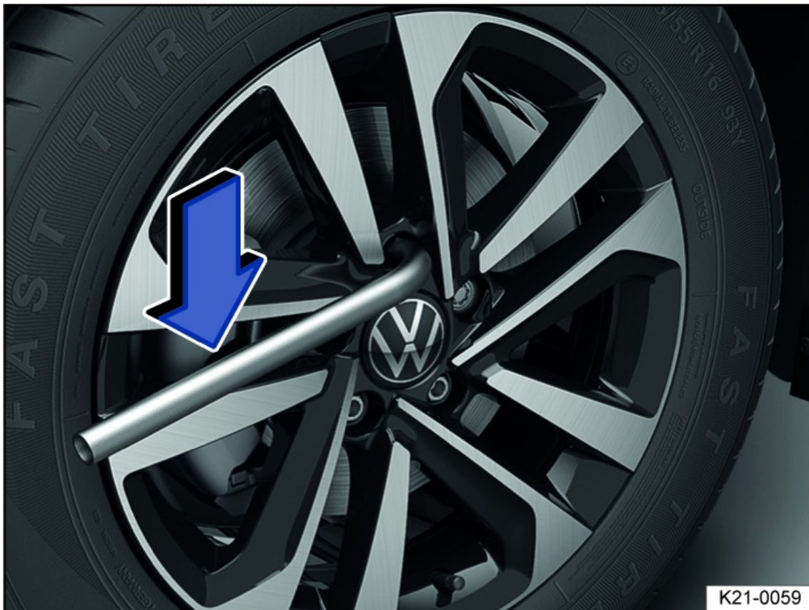
Fig. 191 Removing wheel bolts with the lug wrench.
