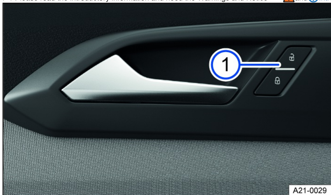
Fig. 44 In the driver's door: Central locking button (general example).
