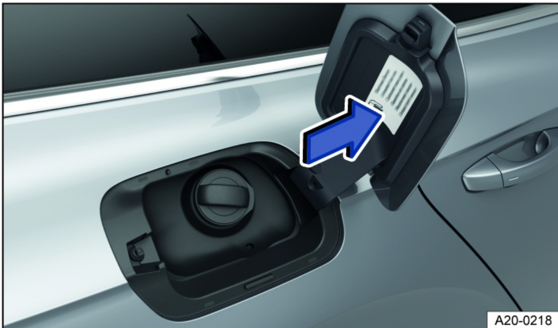
Fig. 141 On the inside of the fuel filler flap: fuel label (general example)
