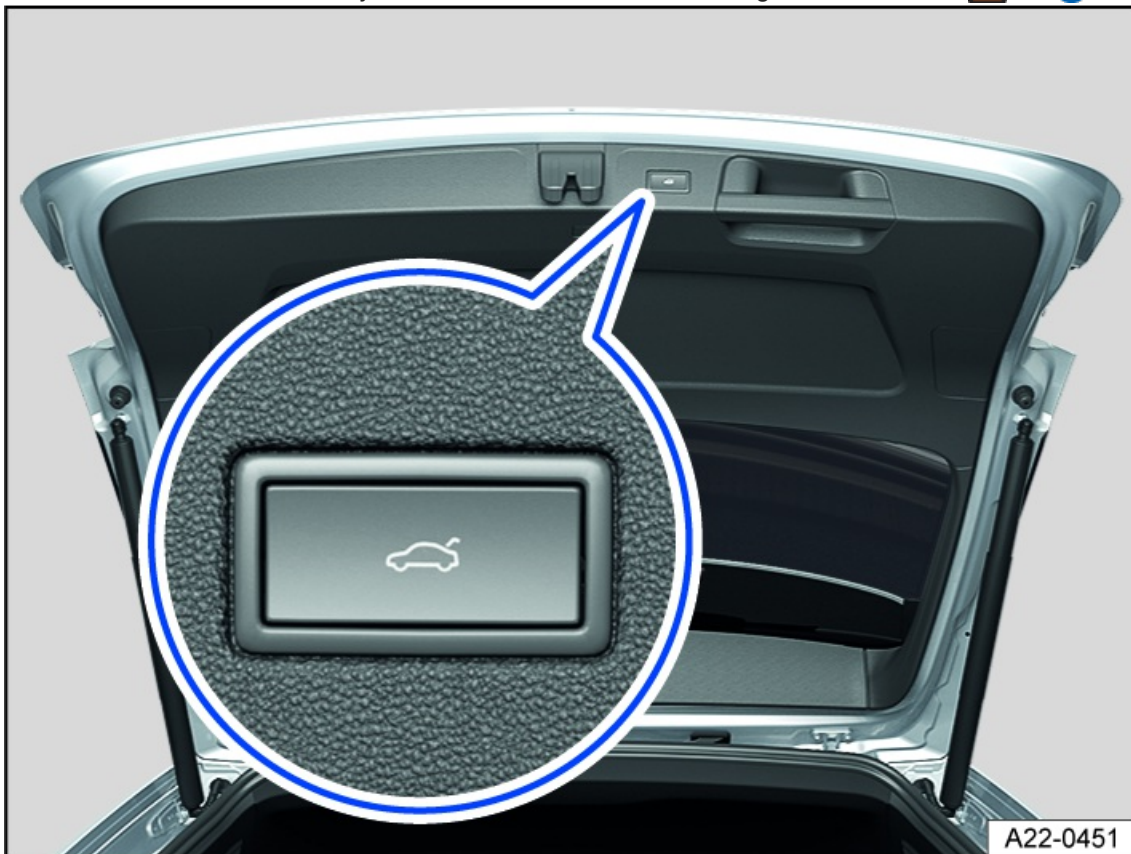
Fig. 51 In the open trunk lid: Button for power closing the trunk lid.
