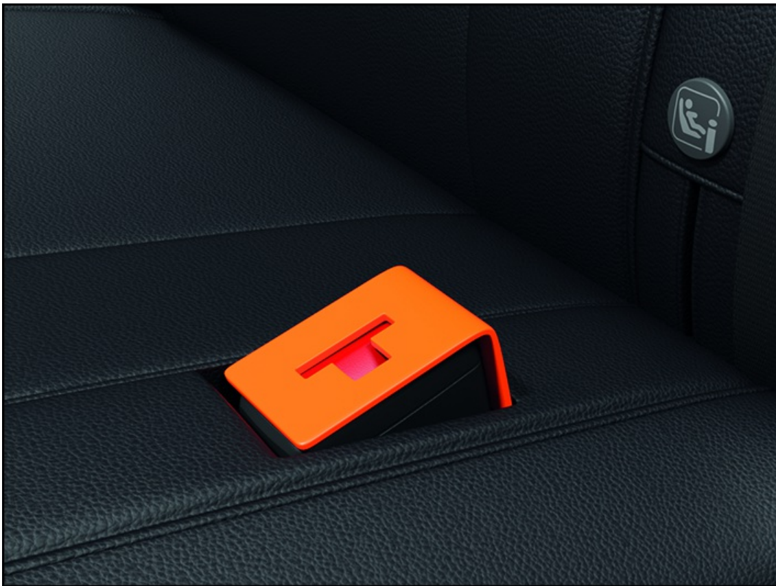
Fig. 31 In the second-row seats: fitted protective cap for belt buckles (general example).
