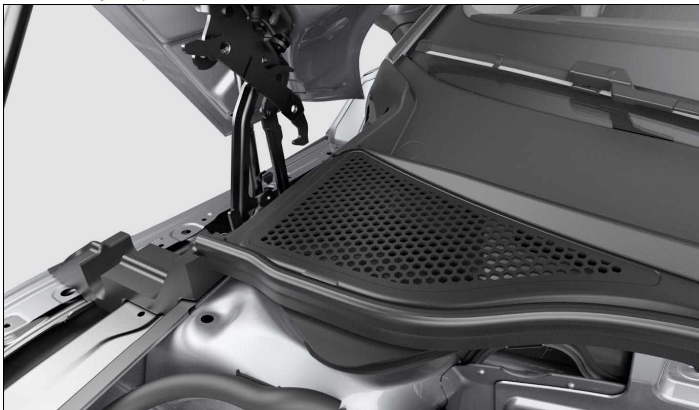
Fig. 212 Between the engine compartment and windshield: plenum chamber (general example).
