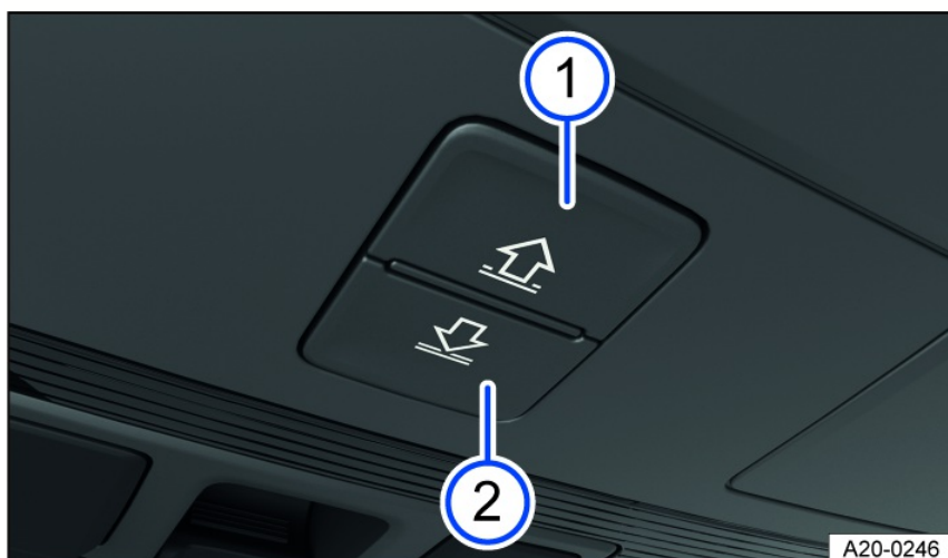
Fig. 103 In the headliner: buttons for controlling the sunshade.
