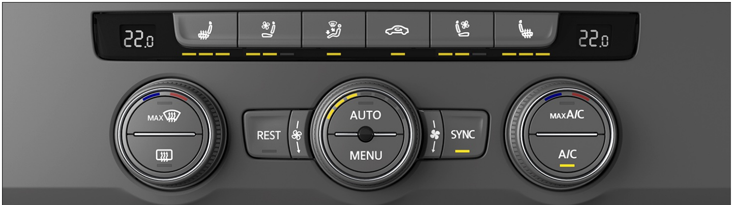
Fig. 105 In the upper section of the center console: Climate control bar for the Climatronic system.
