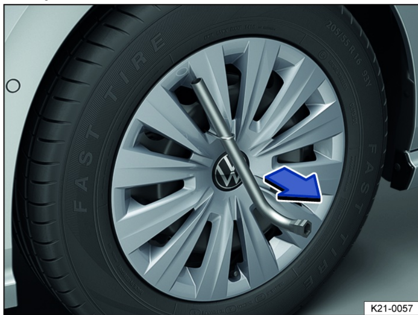
Fig. 200 Remove the wheel hub cover.
