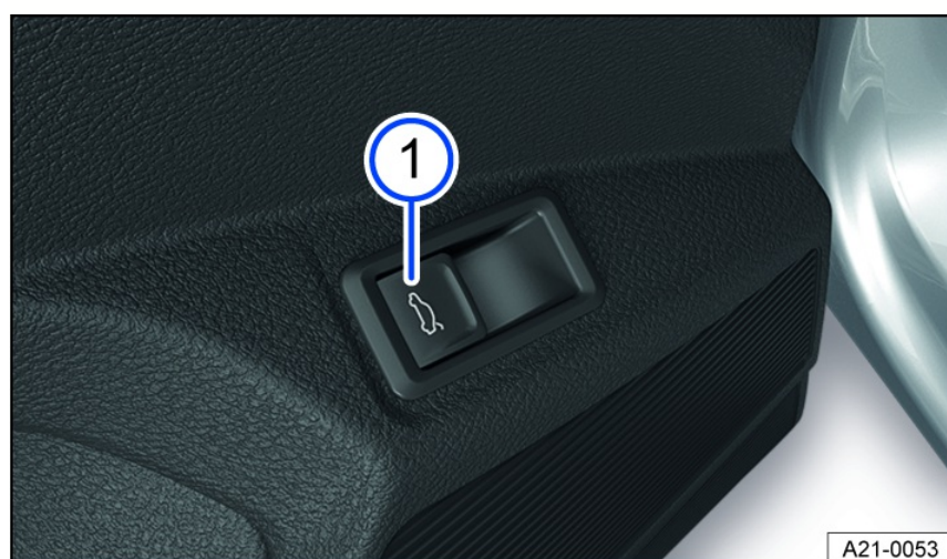
Fig. 59 In the driver's door: Button for powered opening of the trunk lid (general example).
