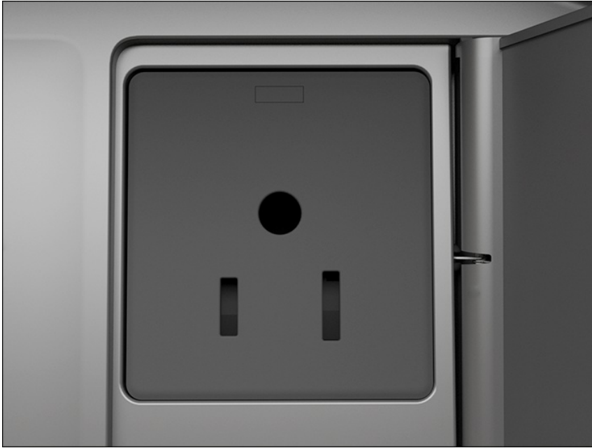
Fig. 154 In the center console at the rear: 115 V socket (depending on the vehicle equipment).
