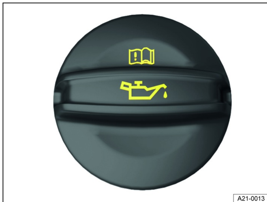
Fig. 190 In the engine compartment: engine oil filler cap (general example).
