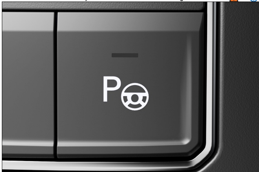
Fig. 147 In the center console: Park Assist button.
