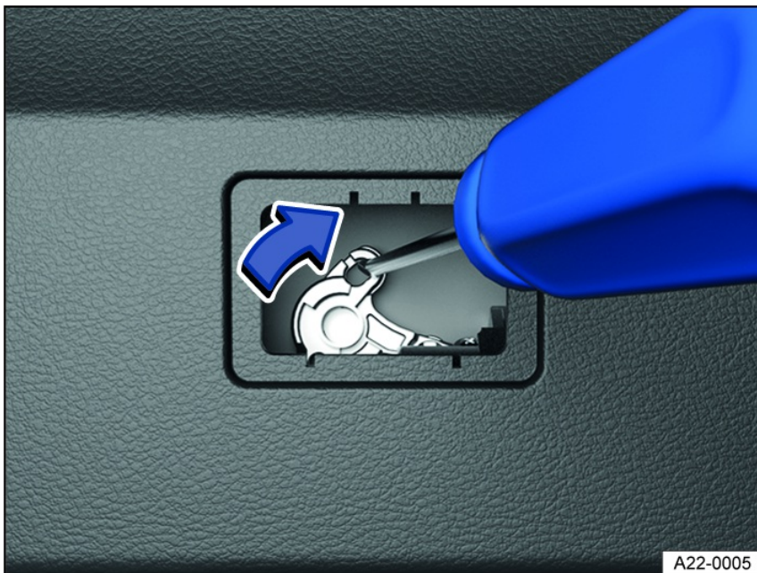
Fig. 69 In the luggage compartment: trunk lid emergency release.
