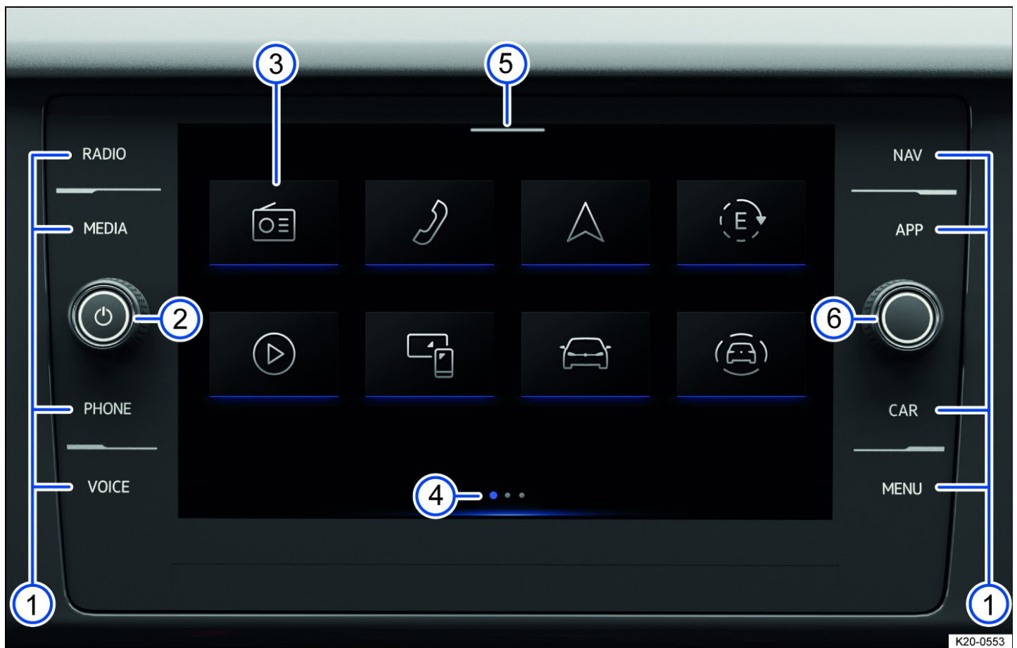
Fig. 156 Overview: display and control unit, 8" version.
