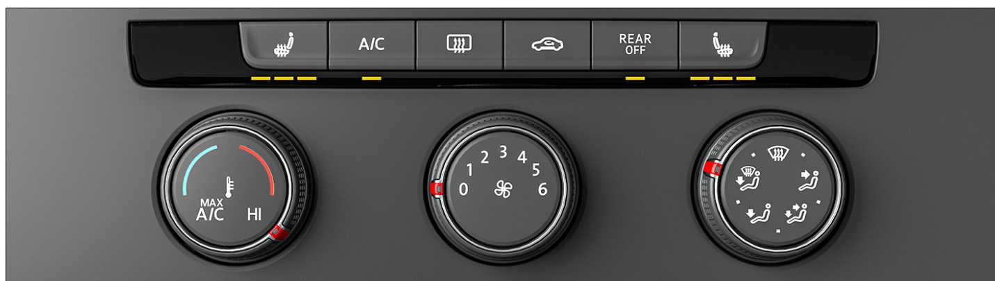
Fig. 106 In the upper section of the center console: Climate control bar for the manual climate control system.
