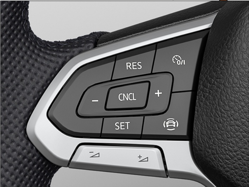
Fig. 125 Left side of the multi-function steering wheel (variant 1).
