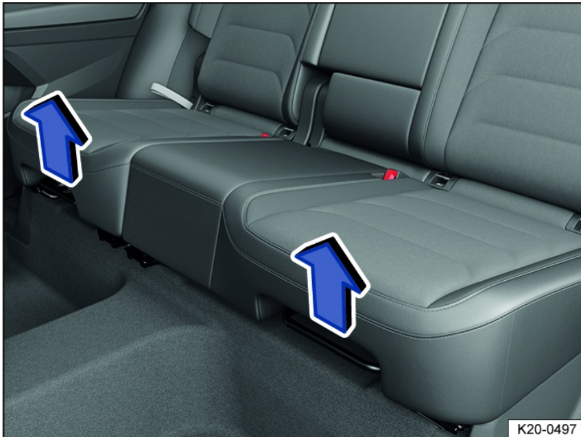
Fig. 77 Under the seat cushion in the rear bench seat: Adjusting lever.
