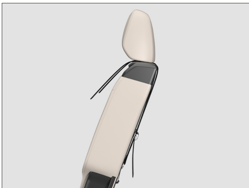
Fig. 43 On the back of the second or third row of seats: attached top tether safety belt.
