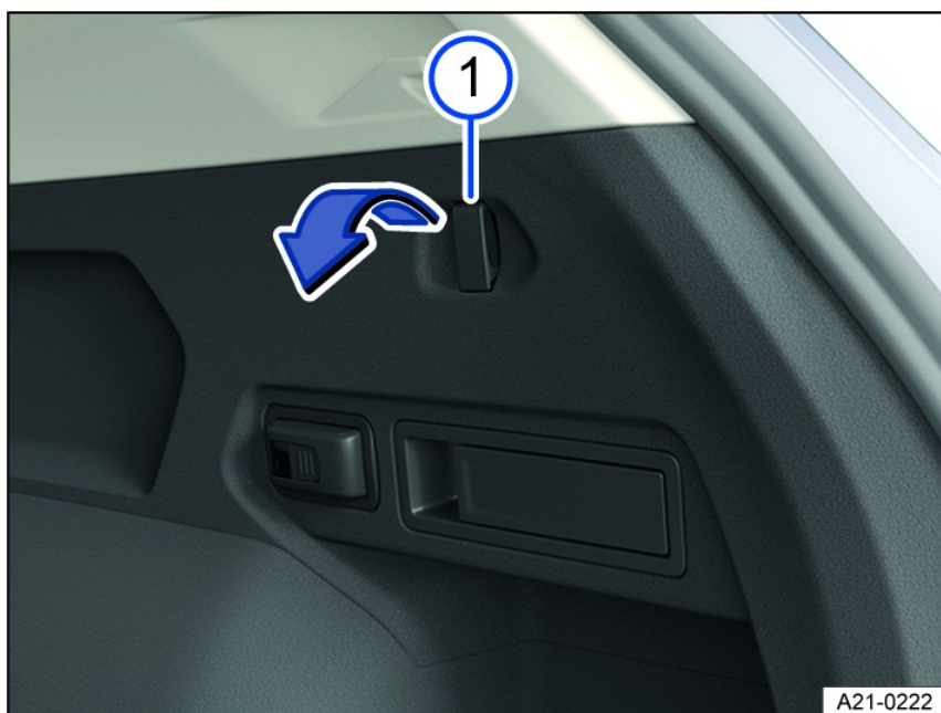
Fig. 166 In the luggage compartment: fold-out shopping bag hooks.
