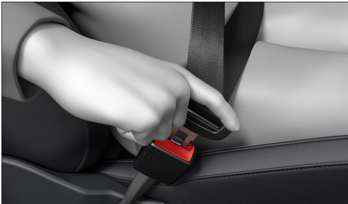
Fig. 27 Inserting the buckle tongue into the safety belt buckle.
