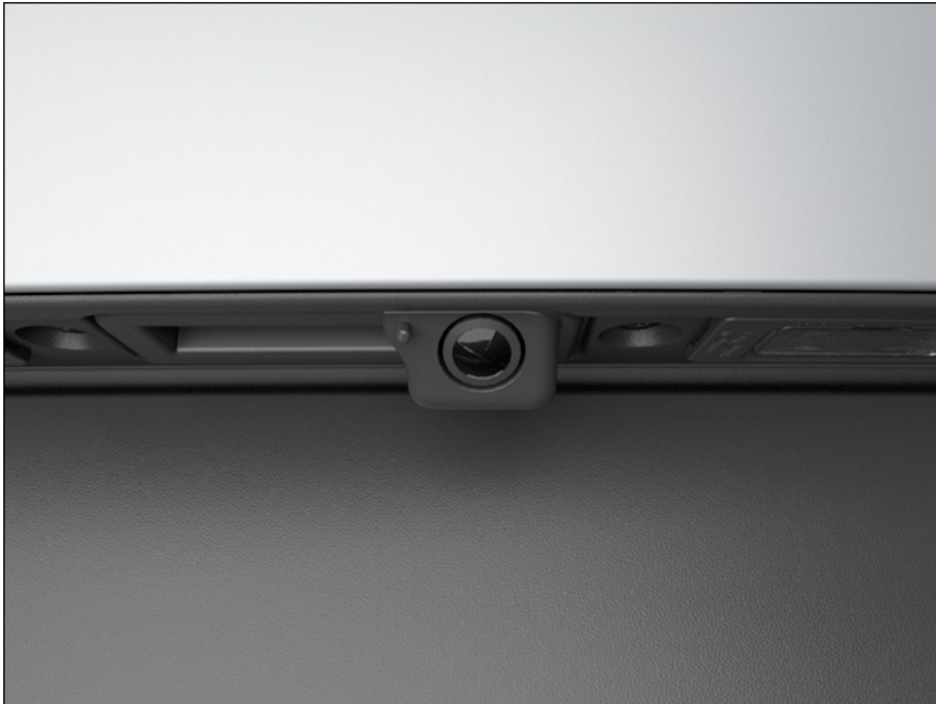
Fig. 213 In the rear of the vehicle: Rear View Camera system on the handle (general example).
