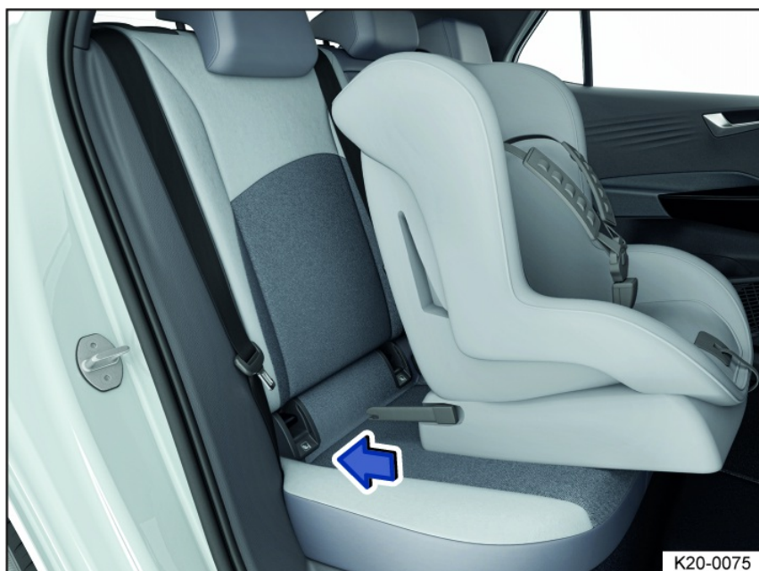
Fig. 40 General example: fitting a child restraint with attachment arms.
