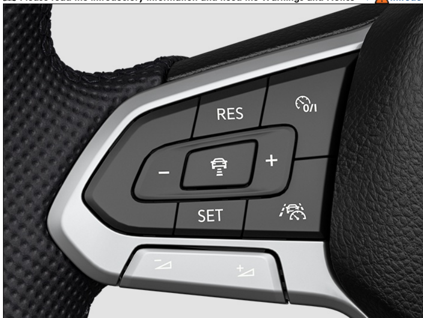
Fig. 131 Left side of the multi-function steering wheel (variant 1).
