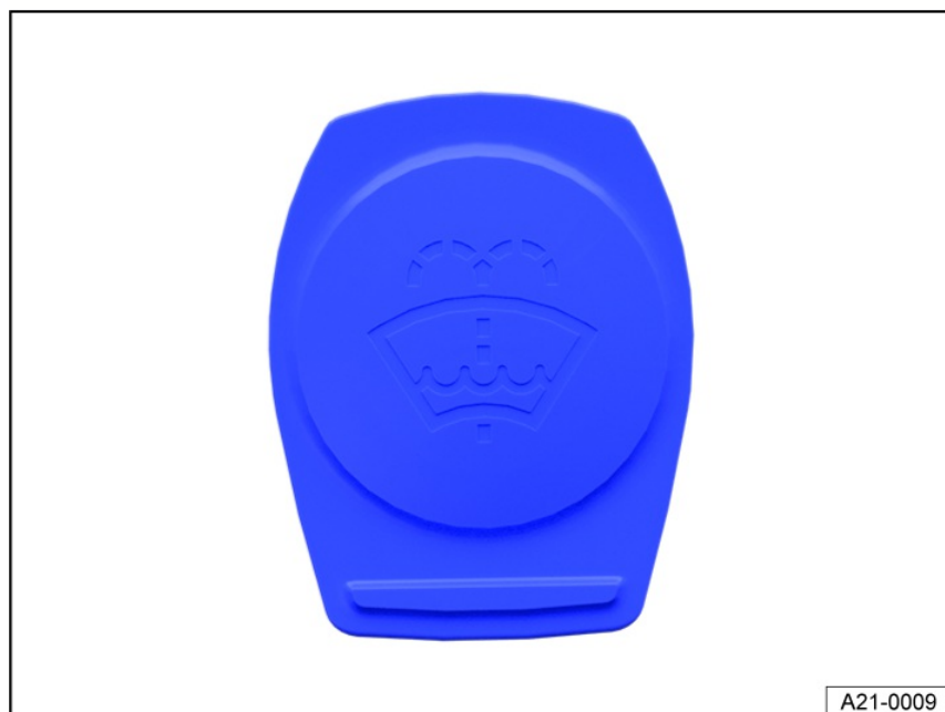
Fig. 189 In the engine compartment: Cap on the washer fluid reservoir (general example).
