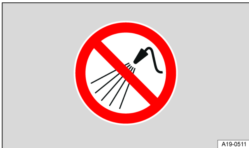
Fig. 211 Warning sign: Do not use pressure washers in the marked area.
