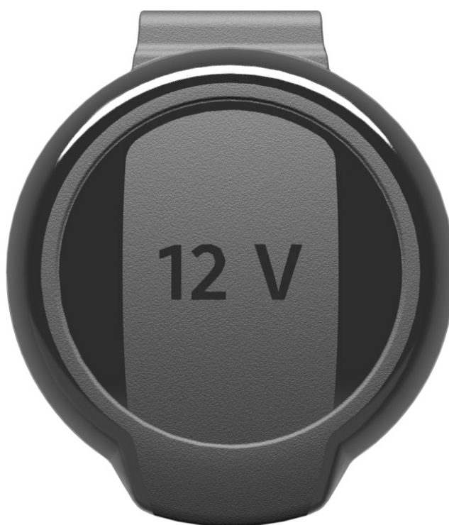
Fig. 153 In the lower part of the center console, at the rear of the center console or on the left-hand side of the luggage compartment: Hinged 12-volt socket (general example).
