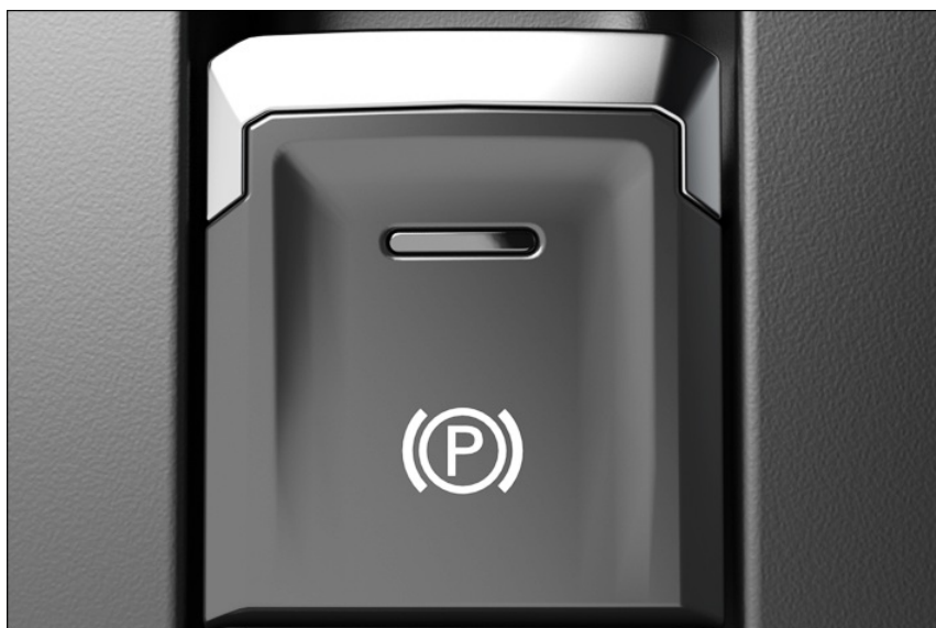
Fig. 139 In the center console: button for the electronic parking brake.
