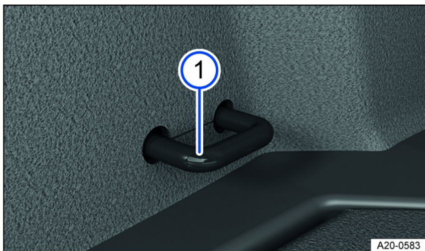
Fig. 163 In the luggage compartment: Tie-down (general example).
