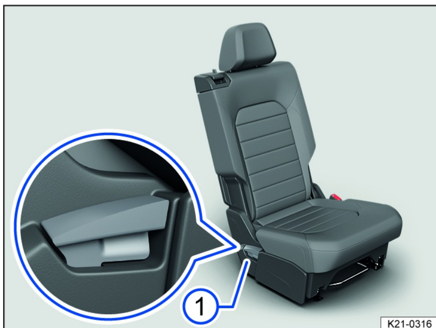
Fig. 78 Left side area in the rear bench seat: adjusting lever.
