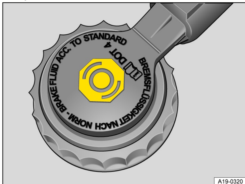
Fig. 194 In the engine compartment: cap on the brake fluid reservoir (version 1).
