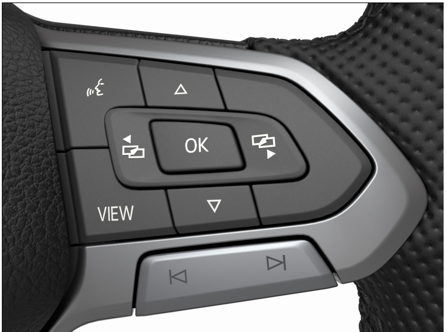
Fig. 16 Right side of the multi-function steering wheel: Operating the analog instrument cluster (variant 1).
