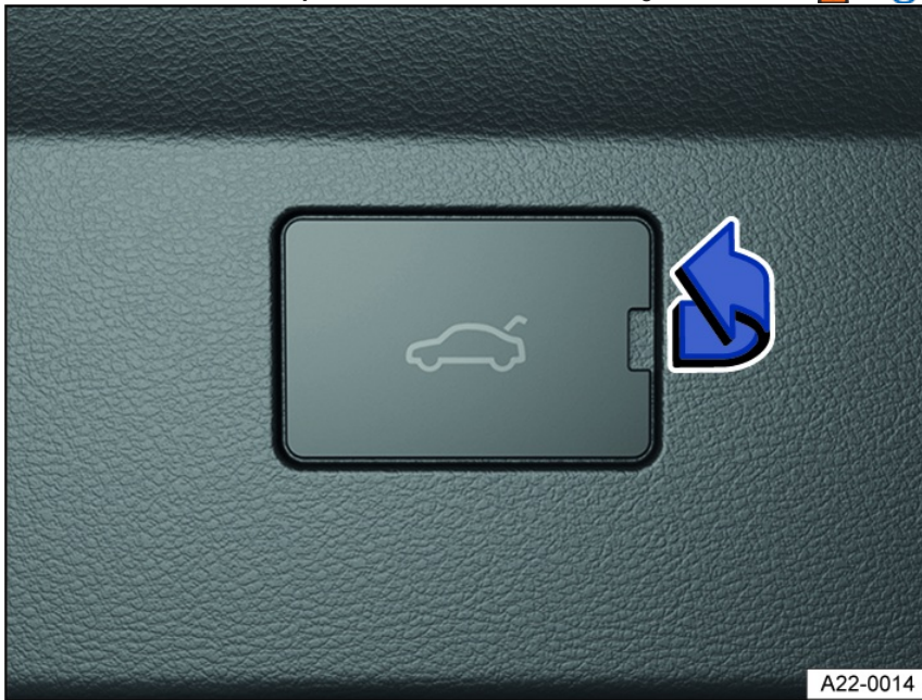
Fig. 68 In the trunk lid: cover for the trunk lid emergency release.
