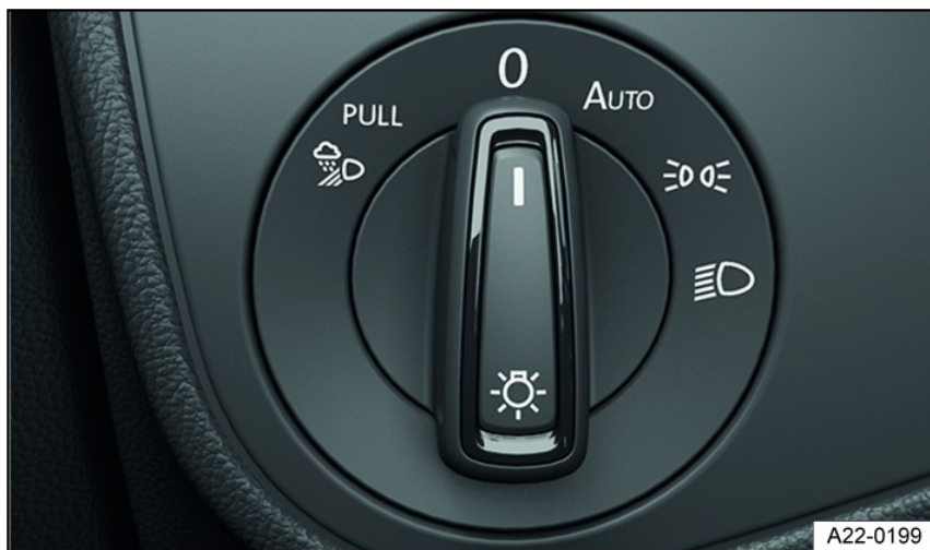
Fig. 94 Next to the steering wheel: light switch (one version).
