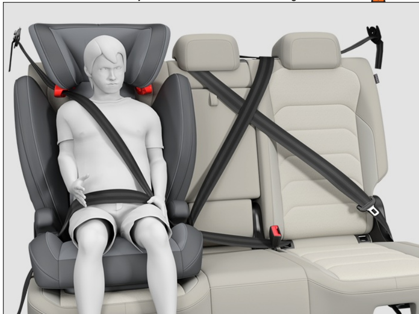
Fig. 47 Correctly fastened child on a booster seat.
