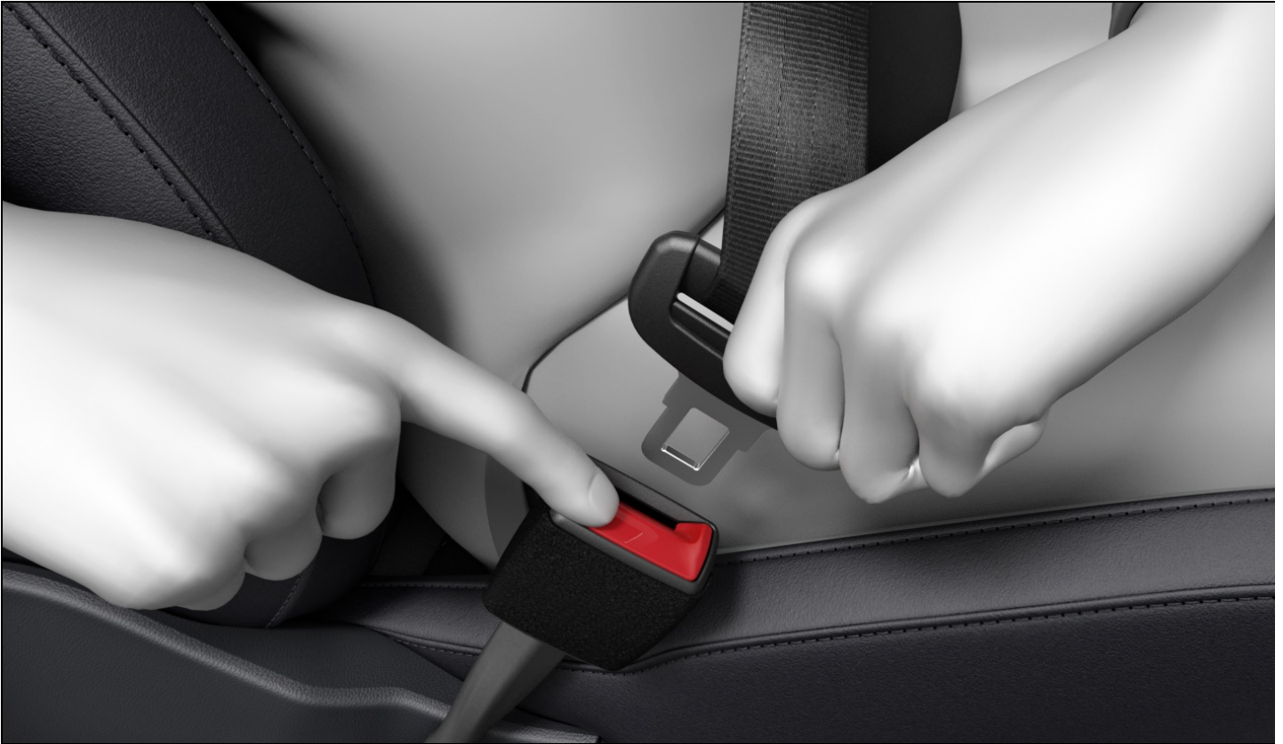
Fig. 28 Releasing the buckle tongue from the safety belt buckle.
