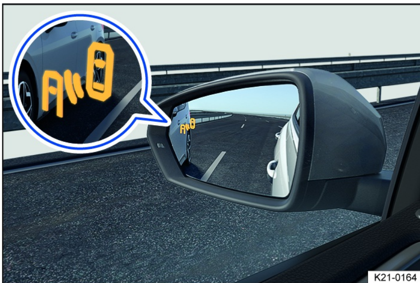
Fig. 138 In the outside mirror: Visual indicators for Side Assist.
