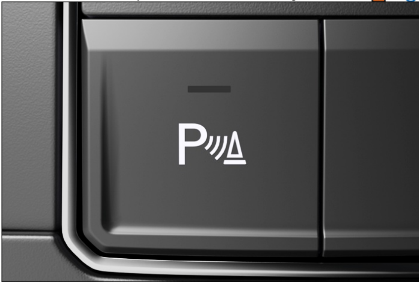
Fig. 141 In the center console: Park Distance Control button.
