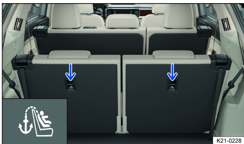
Fig. 42 On the back of the third-row seats: Top tether anchorages for the top tether safety belt.
