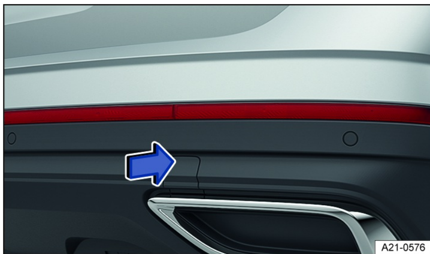
Fig. 184 In the right rear bumper: Remove cover.
