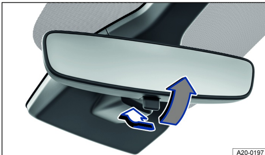
Fig. 100 On the windshield: manual dimming interior rearview mirror.
