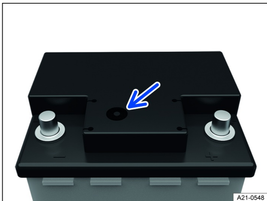
Fig. 196 On the top of the 12 V vehicle battery: Window (general example).
