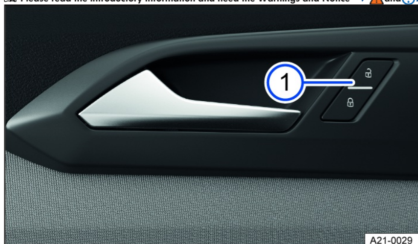
Fig. 58 In the driver's door: Central locking button (general example).
