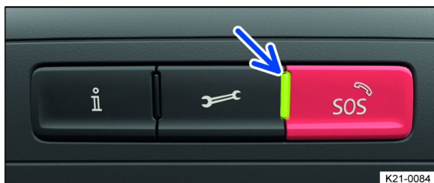
Fig. 48 In the roof console: Controls for call services and indicator light.
