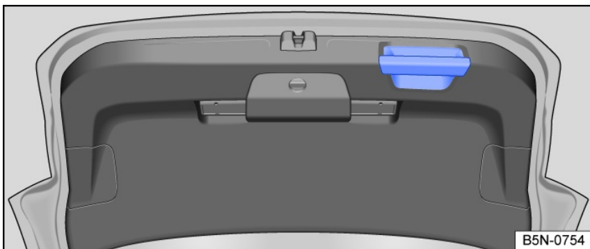
Fig. 64 In the open trunk lid: handle for closing the trunk lid.
