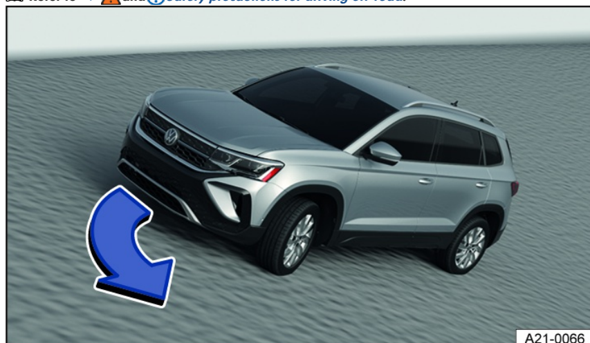
Fig. 123 General example: steering downhill along the fall line.
