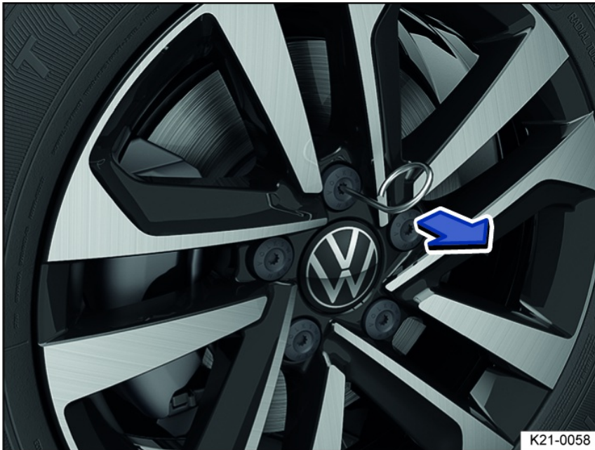
Fig. 201 Remove the caps from the wheel bolts.
