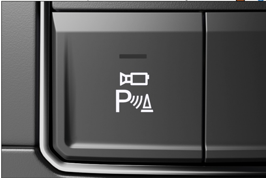
Fig. 145 In the center console: Button for switching the Area View on and off.
