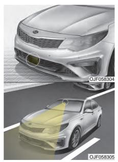
In order for the FCA system to operate properly, always make sure the sensor or sensor cover is clean and free of dirt, snow, and debris. Dirt, snow, or foreign substances on the sensor or its external parts may adversely affect the sensing performance of the sensor.
