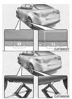
7. Place the jack at the front (1) or rear (2) jacking position closest to the tire you are changing. Place the jack at the designated locations under the frame. The jacking positions are plates welded to the frame with two tabs and a raised dot to line up with the jack.
