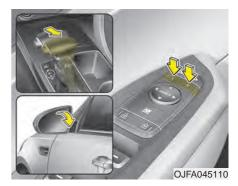
While the vehicle is moving in reverse, the outside rearview mirror(s) will move downward to aid reverse parking. According to the position of the outside rearview mirror switch (1), the outside rearview mirror(s) will operate as follows:
