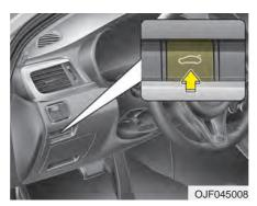
To open the trunk from inside the vehicle, push the trunk lid release button.
