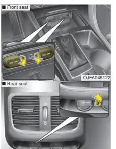
The power outlet is designed to provide power for mobile telephones or other devices designed to operate with vehicle electrical systems. The devices should draw less than 10 amps with the engine running.
