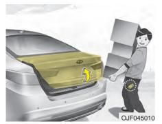
On a vehicle equipped with a smart key, the trunk lock is released with no-touch activation using the Smart Trunk system.
