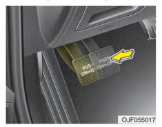
Check whether the stroke is within specification when the parking brake pedal is pressed with 66 lb, 294 N (30 kg) of force. Also, the parking brake alone should securely hold the vehicle on a fairly steep grade. If the stroke is more or less than specified, have the parking brake adjusted by an authorized Kia dealer.
