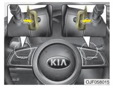
The paddle shifter is available when the shift lever is in the D position or the manual mode.
