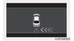
If the vehicle detected by the sensors approaches your vehicle, the warning chime will sound, the warning light on the outside rearview mirror will blink and a message will appear on the LCD display.
