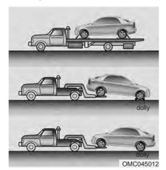
If emergency towing is necessary, we recommend having it done by an authorized Kia dealer or a commercial tow-truck service. Proper lifting and towing procedures are necessary to prevent damage to the vehicle. The use of wheel dollies or flatbed is recommended.
