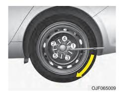
Position the wrench as shown in the drawing and tighten the wheel nuts. Be sure the socket is seated completely over the nut. Do not stand on the wrench handle or use an extension pipe over the wrench handle. Go around the wheel, tightening every nut following the numerical sequence shown in the image until they are all tight. Double-check each nut for tightness. After changing wheels, have an authorized Kia dealer tighten the wheel nuts to their proper torque as soon as possible.
