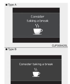
The "Consider taking a break" message appears on the LCD display and a warning sounds in order to suggest the driver to take a break, when the driver's attention level is below 1.
