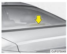
If the high mounted stop lamp (LED) does not operate, have the vehicle checked by an authorized Kia dealer.
