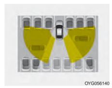
The Rear Cross-Traffic Collision Warning function monitors approaching cross traffic from the left and right side of the vehicle when your vehicle is in reverse.
