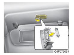
WARNING - Interior lamps Prior to working on the Interior lamps, ensure that the "OFF" button is pressed to avoid burning your fingers or receiving an electric shock.
