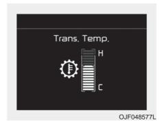
This mode displays the temperature of the dual clutch transmission.
