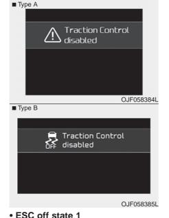
It means the traction control function does not operate. Brake control function only operates.
