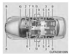
The SRS consists of the following components:
