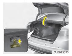
If the fuel filler lid does not open using the fuel filler lid opener button, you can open it manually. Remove the panel in the cargo area. Pull the handle out slightly.
