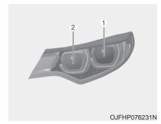
If the low beam (1) and high beam (2) do not operate, have the vehicle checked by an authorized Kia dealer.
