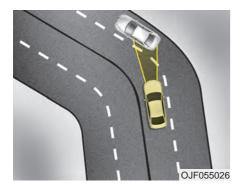
While driving on a curve, the FCA may recognize the vehicle in front in the next lane. Pay great caution, and, if necessary, depress the brake pedal.
