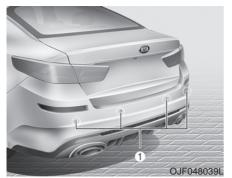
The parking distance warning-reverse assists the driver during backward movement of the vehicle by chiming if any object is sensed within a distance of 47 in. (120 cm) behind the vehicle.
