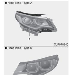
If the position lamp + DRL (LED) (1) does not operate, have the vehicle checked by an authorized Kia dealer.
