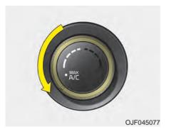
The MAX A/C mode is used to cool the inside of the vehicle faster.
