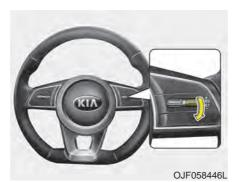
Move the lever down (to SET-), and release it at the desired speed. The SET indicator light in the instrument cluster will illuminate. Release the accelerator at the same time. The desired speed
