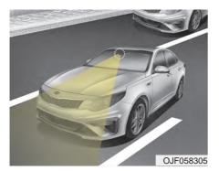
In order for the FCA system to operate properly, always make sure the sensor is clean and free of dirt, snow, and debris
