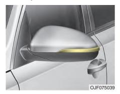
If the side repeater lamp (LED) does not operate, have the vehicle checked by an authorized Kia dealer. The LED lamp cannot be replaced as a single component because it is an integrated unit. The LED lamp has to be replaced with the unit.
