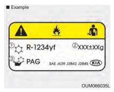
\* The actual Air Conditioning refrigerant label in the vehicle may differ from the illustration. Each symbol and specification on the air conditioning refrigerant label is represented below:
