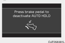
If you do not apply the brake pedal when you release the Auto Hold by pressing the [AUTO HOLD] switch, a warning will sound and a message will appear.
