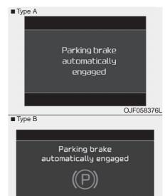
If the EPB is applied while Auto Hold is activated because of an ESC (Electronic Stability Control) signal, a warning will sound and a message will appear.
