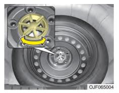
Turn the tire hold-down wing bolt counterclockwise.
