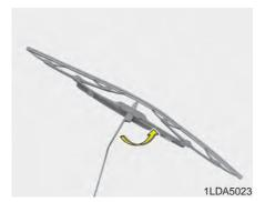
Type B1. Raise the wiper arm and turn the wiper blade assembly to expose the plastic locking clip.
