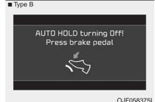
When the conversion from Auto Hold to EPB is not working properly a warning will sound and a message will appear.
