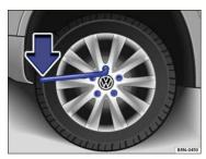
Fig. 195 Changing a wheel: Loosening the wheel bolts.
