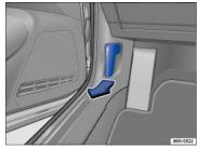
Fig. 176 In the footwell on the driver side: Inside engine hood release lever.
