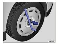
Fig. 193 Pulling the wheel cover off.
