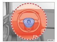
Fig. 32 Location and deployment zone of the driver front airbag.
