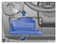
Fig. 169 On the driver side in the instrument panel: Removing the storage compartment to access the fuses.
