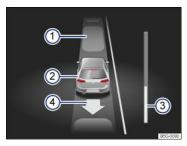
Fig. 140 In the instrument cluster display: Driving out of a parallel parking space.
