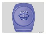
Fig. 179 In the engine compartment: Cap of the windshield washer fluid reservoir
