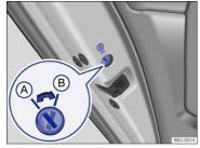
Fig. 62 In the rear driver side door: Child safety lock (A) deactivated, (B) activated.
