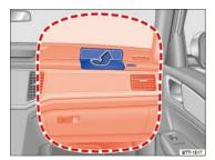
Fig. 33 Location and deployment zone of the front passenger front airbag.
