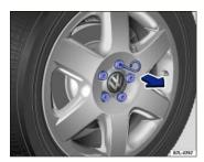
Fig. 194 Pulling cover caps off wheel bolts.
