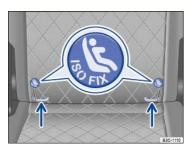
Fig. 43 On the second row seat backrests: Markings indicating the location of the LATCH/UAS lower universal anchorages.
