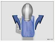
Fig. 115 Removing the selector gate cover.
