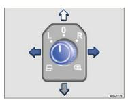
Fig. 98 In the driver door: Adjusting knob for the outside mirrors.
