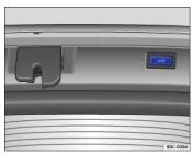
Fig. 66 Button in the open trunk lid.
