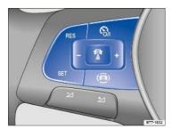
Fig. 126 Left-hand side of the multi-function steering wheel: Buttons for operating the Adaptive Cruise Control (ACC).
