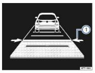
Fig. 127 In the instrument cluster display: distance interval is being set (displayed in color on an instrument cluster with color display).
