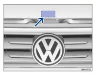
Fig. 177 Above the radiator grille: Outside engine hood release.
