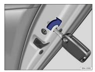
Fig. 61 On the front side of the rear passenger side door: Locking the vehicle with the key bit in the vehicle key.
