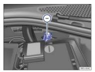
Fig. 173 In the engine compartment: Negative jump-start terminal  $\bigcirc$ .
