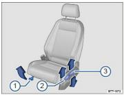
Fig. 73 Driver seat: Manual seat adjustment controls.
