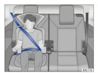
Fig. 42 Child properly restrained in a booster seat in the third row.
