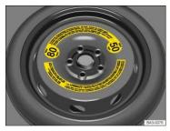
Fig. 190 In the luggage compartment: Compact spare wheel.
