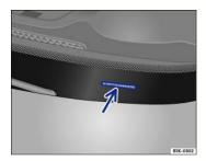
Fig. 202 Vehicle identification number (VIN).
