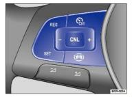
Fig. 123 Left-hand side of the multi-function steering wheel: Buttons for operating the cruise control.
