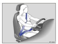
Fig. 29 Proper safety belt positioning for expectant mothers.
