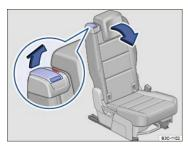
Fig. 87 In the second row: The entry assistance lever.
