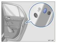
Fig. 60 on the rear passenger door: Manual lock, covered by a rubber seal.
