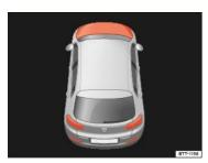
Fig. 178 In the instrument cluster display: Engine hood open or not properly closed.
