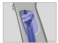
Fig. 30 Next to the front seats: Safety belt height adjuster.
