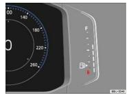
Fig. 12 Volkswagen Digital Cockpit: Fuel gauge
