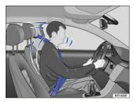
Fig. 25 Belted driver secured by the correctly worn safety belt in the event of a sudden braking maneuver.
