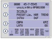
Fig. 201 Vehicle identification label: Shown in the example with engine identification code CBFA  $\ 3$ .
