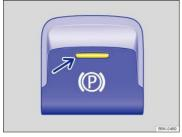
Fig. 131 In the lower center console: Electronic parking brake switch.
