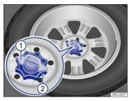
Fig. 189 In the luggage compartment: Handwheel holding the compact spare wheel in place.
