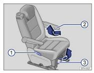
Fig. 76 In the second row: Adjusting the seats.
