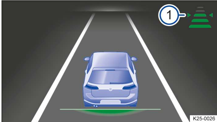
Fig. 1 On the instrument cluster display: set distance for control (illustration).
