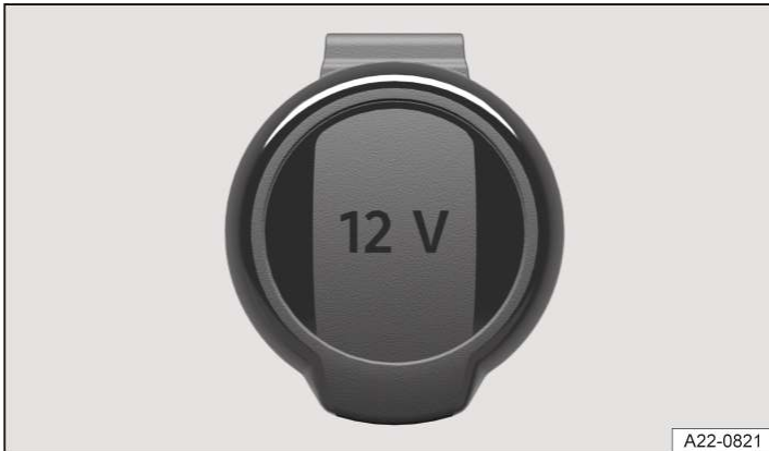
Fig. 1 In the storage compartment in the front centre console and on the right-hand side of the luggage compartment: fold-open 12-volt socket (illustration).
