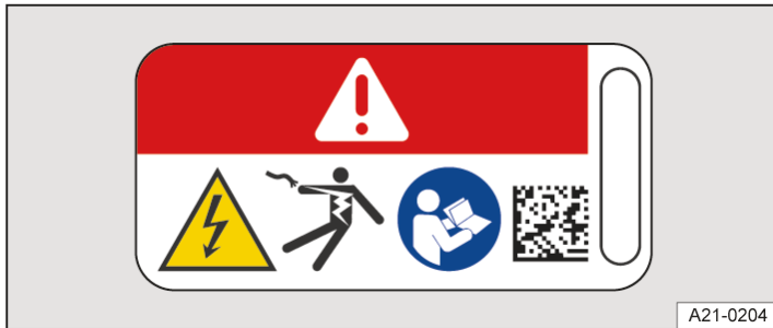
Fig. 1 Warning sign on high-voltage components.
