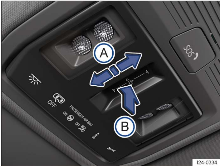
Fig. 1 In the roof: touch control for the glass roof.
