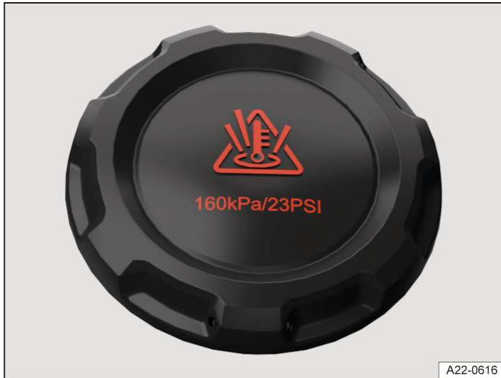
Fig. 2 In the bonnet space: coolant expansion tank cap (illustration).
