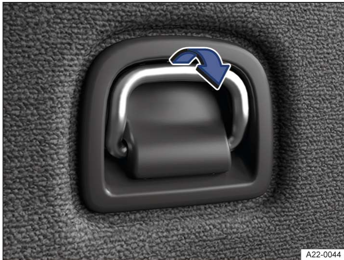
Fig. 1 In the luggage compartment: folding fastening ring (illustration).
