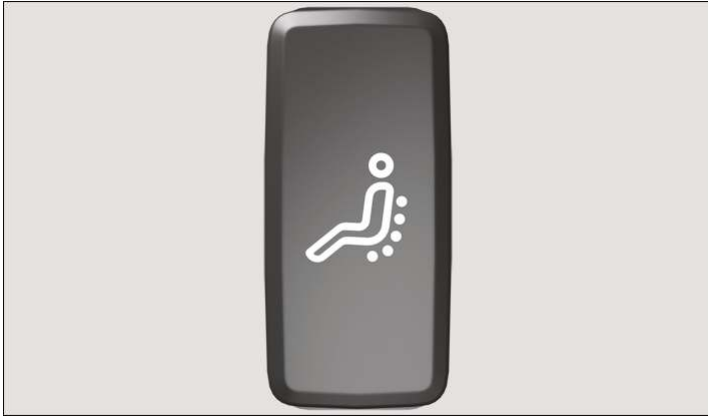
Fig. 1 On the outside of the driver seat: button for the massage function.
