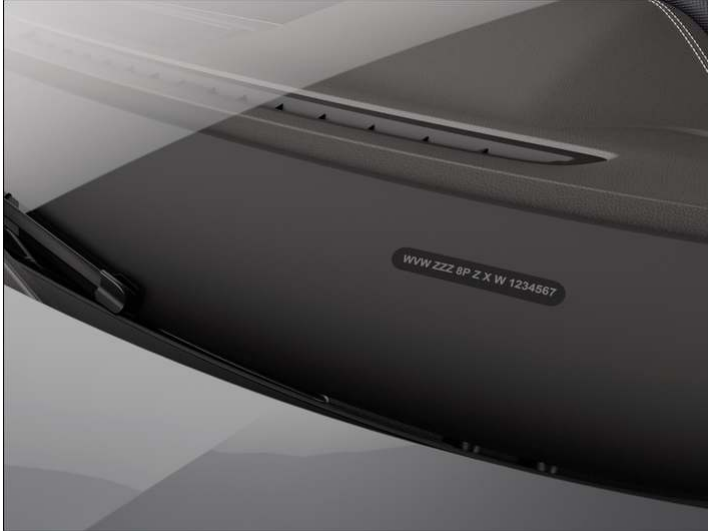
Fig. 1 In the windscreen: vehicle identification number.
