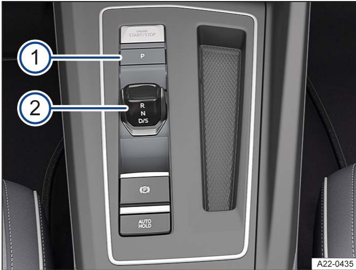
Fig. 1 In centre console: selector lever of the automatic gearbox.
