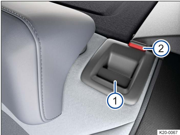
Fig. 1 In the rear seat backrest: release button.
