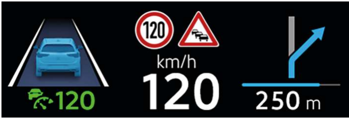
Fig. 1 In the driver's field of vision: displays in the head-up display (illustration).
