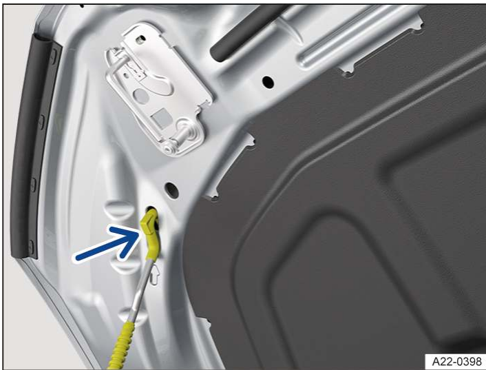
Fig. 4 On the bonnet: holder for bonnet stay (illustration).
