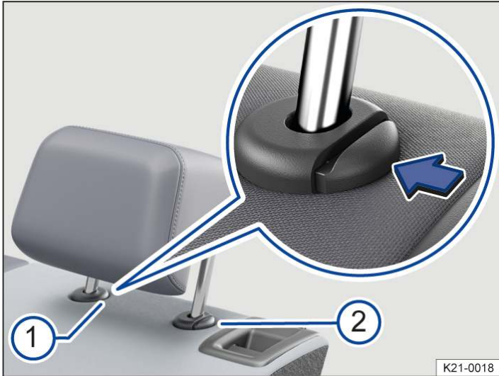
Fig. 1 Removing a rear head restraint (illustration).
