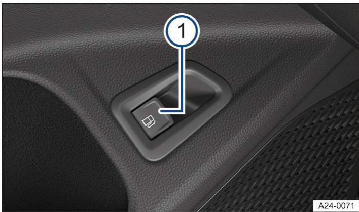
Fig. 2 In the driver door: button for tank flap release (illustration).
