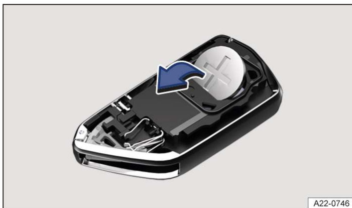
Fig. 2 Vehicle key: replacing the button cell.
