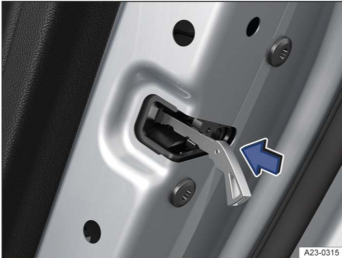
Fig. 1 In the front edge of a door: locking the vehicle manually with the manual key (illustration).
