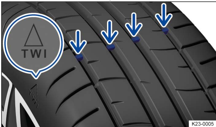
Fig. 1 In the tread grooves: tread wear indicator.
