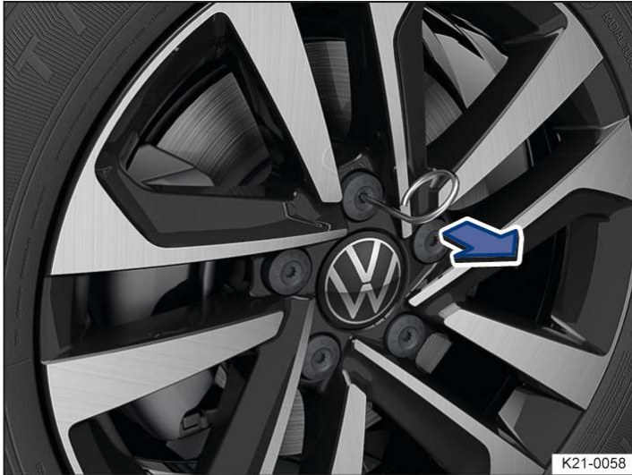
Fig. 1 Removing the wheel bolt caps.
