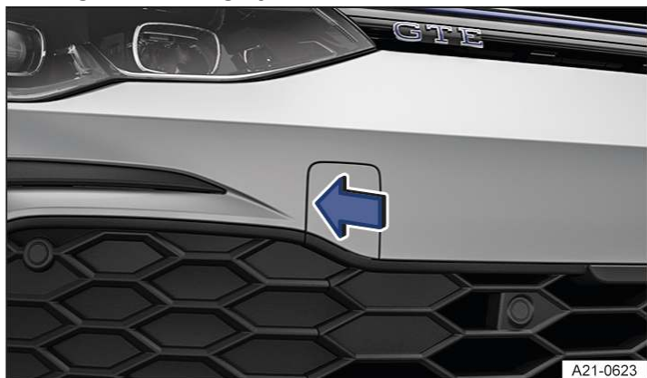
Fig. 1 In the front bumper on the right: removing the cover, variant 1.
