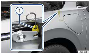
Fig. 1 Between the left wing and the bonnet space: manual release of the charging connector.
