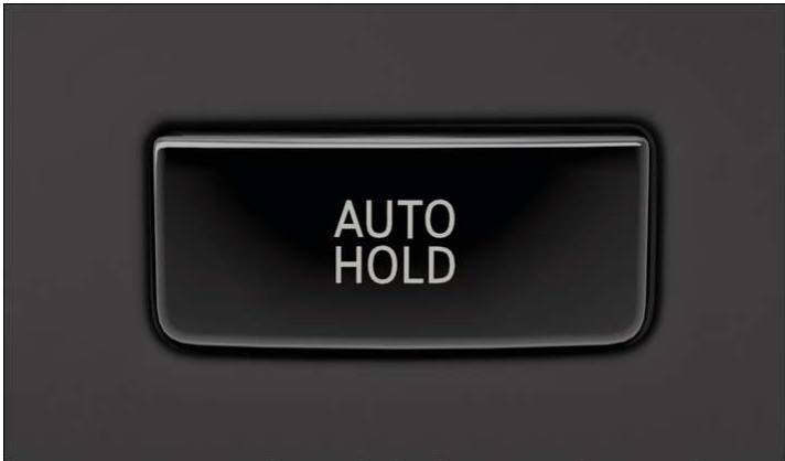
Fig. 1 In the centre console: button for the Auto Hold function.
