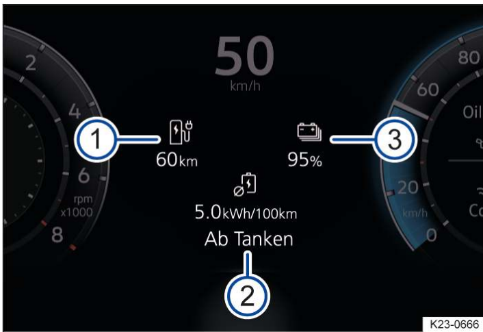
Fig. 1 In the main display area of the digital instrument cluster: charge level and range (illustration).
