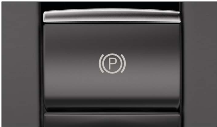
Fig. 1 In the centre console: button for the electronic parking brake (automatic gearbox).
