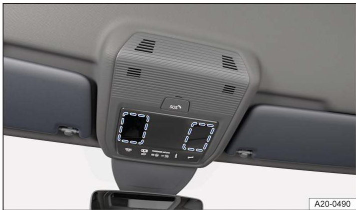
Fig. 1 In the roof console: touch-sensitive reading lights.
