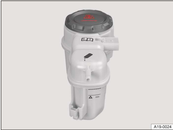
Fig. 4 In the bonnet space: markings on the coolant expansion tank (illustration).
