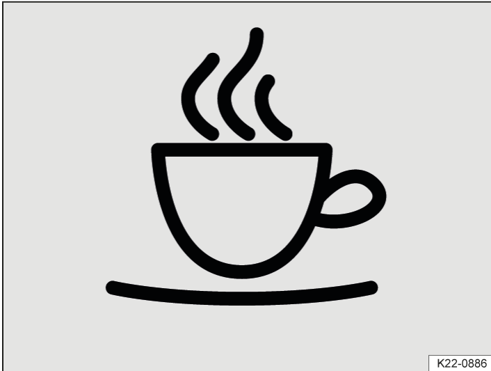
Fig. 1 On the display of the digital instrument cluster: Drowsiness Monitor symbol.
