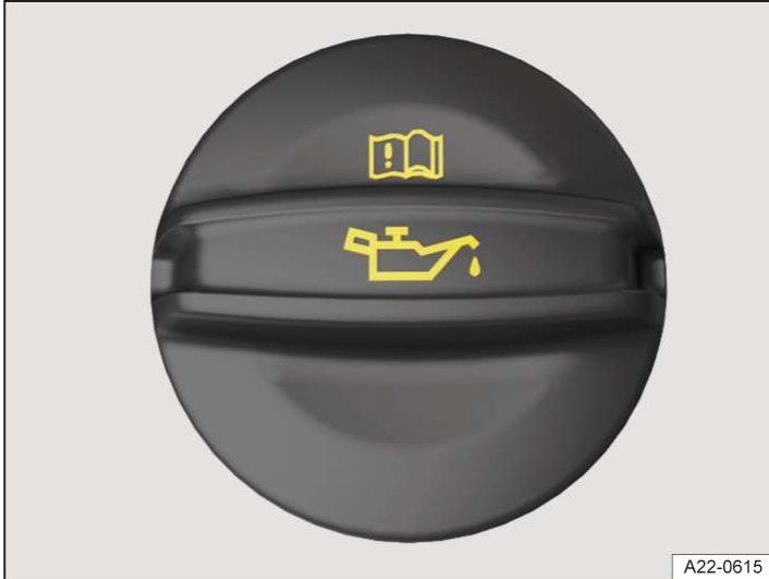
Fig. 1 In the bonnet space: cap of engine oil filler opening (illustration).
