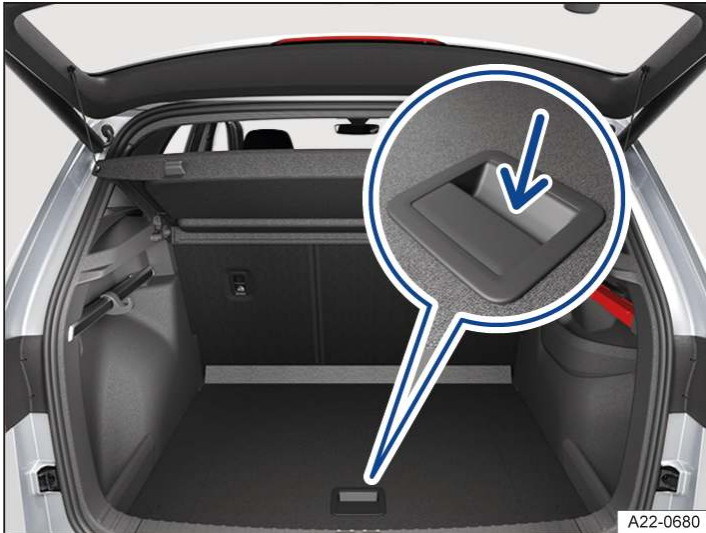
Fig. 1 In the luggage compartment: opening the luggage compartment cover (illustration).
