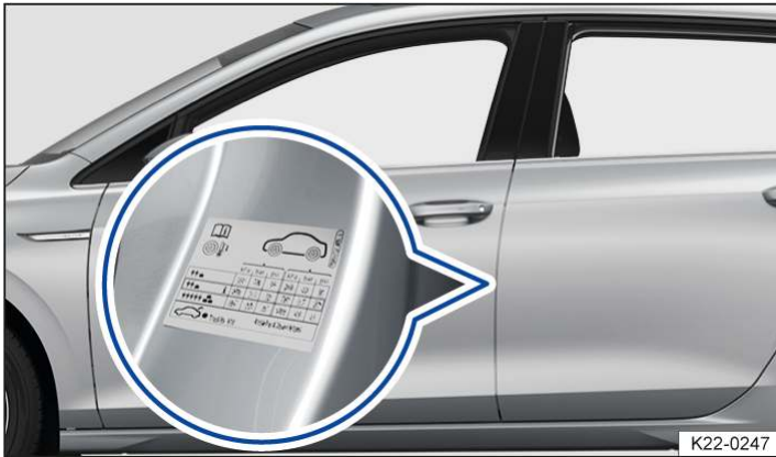
Fig. 1 On the driver door pillar: tyre pressure sticker (alternatively on the inside of the tank flap).
