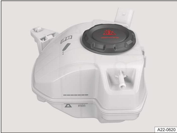
Fig. 3 In the bonnet space: markings on the coolant expansion tank (illustration).
