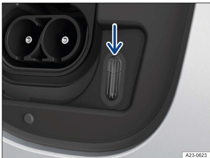
Fig. 1 Behind the charging socket flap: charging process display.
