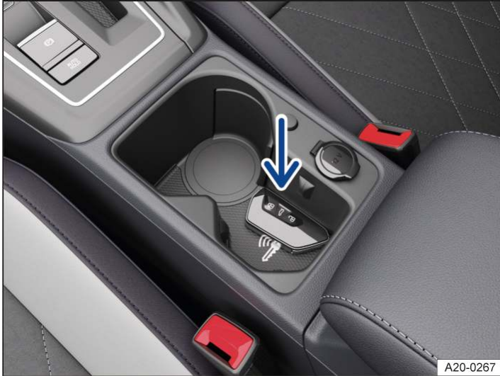
Fig. 1 In the centre console: emergency start function.
