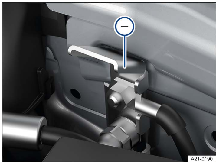
Fig. 2 In the bonnet space: jump-start connection point (earth).
