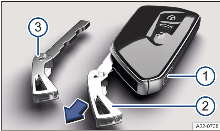
Fig. 1 Vehicle key: releasing the manual key (illustration).
