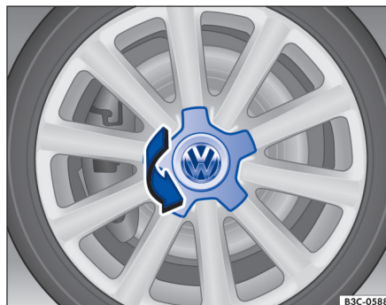
Fig. 182 Twisting the hubcap off.
