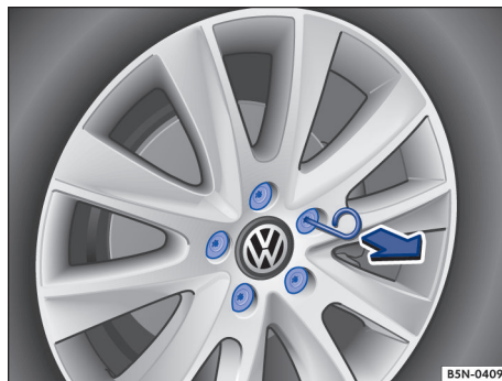
Fig. 184 Pulling cover caps off wheel bolts.
