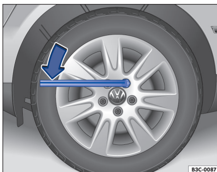
Fig. 185 Changing a wheel: Loosening the wheel bolts.
