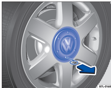
Fig. 181 Pulling the hubcap off.
