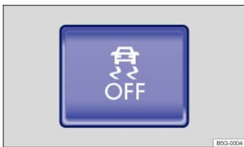
Fig. 158 In the center console: Button for switching ASR or ESC Sport mode on and off manually (if equipped).
