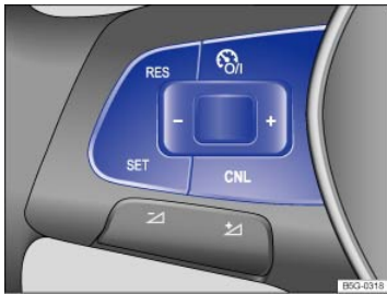
Fig. 124 Left-hand side of the multi-function steering wheel: Buttons for operating the cruise control.
