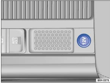
Fig. 173 In the lower center console: 12 Volt socket (vehicles with electronic parking brake).
