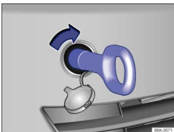
Fig. 204 In the right front bumper: Installing the towing eye.
