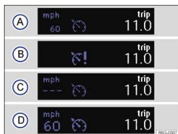
Fig. 123 In the instrument cluster display: Cruise control status indications.
