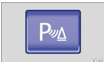
Fig. 144 In the lower center console: Button to switch the Park Distance Control system on or off.
