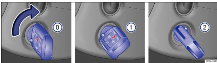
Fig. 110 In the ignition switch: Vehicle key positions for vehicles without Keyless Access.
