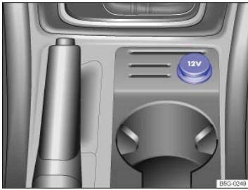
Fig. 172 In the lower center console: 12 Volt socket (vehicles with parking brake lever).
