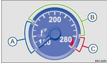
Fig. 16 Engine coolant temperature gauge in the instrument cluster: (A) Engine cold; (B) Normal temperature range; (C) Warning zone.
