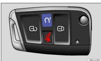
Fig. 69 On the remote control vehicle key: Button to unlock the trunk lid.
