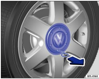
Fig. 223 Pulling the hubcap off.
