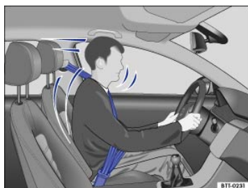
Fig. 31 Belted driver secured by the correctly worn safety belt in the event of a sudden braking maneuver.
