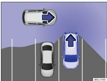
Fig. 138 Rear Traffic Alert: Monitored area around the vehicle that is backing out of a parking space.
