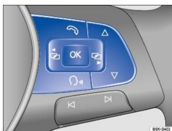
Fig. 20 Right side of the multi-function steering wheel: Controls for the menus and information in the instrument cluster display.
