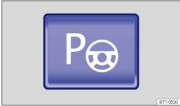
Fig. 152 In the lower center console: Button for switching on the Park Assist system.
