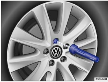
Fig. 233 Changing a wheel: Remove previously loosened wheel bolts using the screwdriver handle.
