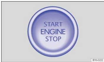
Fig. 111 In the lower center console: Starter button for the Keyless Access system.
