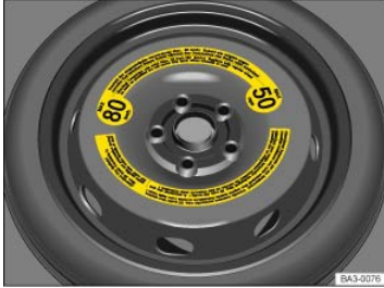
Fig. 221 In the luggage compartment: Compact spare wheel (if equipped, label design may vary).
