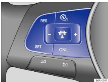
Fig. 128 Left-hand side of the multi-function steering wheel: Buttons for operating the Adaptive Cruise Control (ACC).
