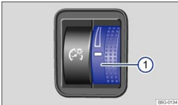
Fig. 92 To the left of the steering wheel: Thumbwheel to adjust instrument panel lighting ①.
