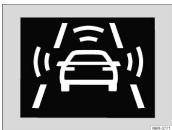
Fig. 131 In the instrument cluster display: Advance warning (symbol displayed in color on an instrument cluster with color display).
