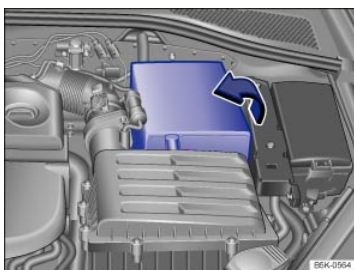
Fig. 216 In the engine compartment: Open the sleeve covering of the vehicle battery.
