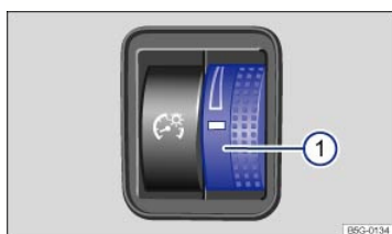
Fig. 87 To the left of the steering wheel: Thumbwheel to adjust instrument panel lighting ①.
