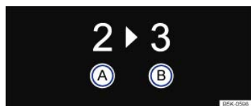
Fig. 144 In the instrument cluster display: Gear recommendation.
