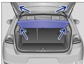
Fig. 100 In the luggage compartment: Installing and removing the luggage compartment cover.
