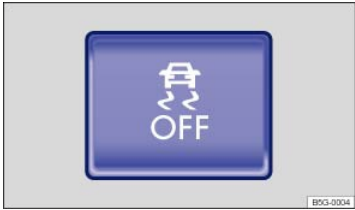
Fig. 147 In the center console: Button for switching ASR or ESC Sport mode on and off manually (if equipped).
