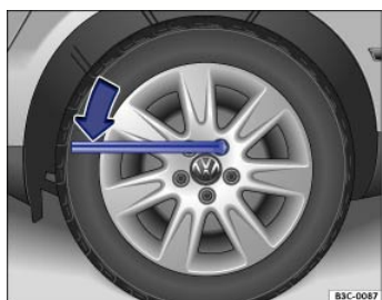
Fig. 222 Changing a wheel: Loosening the wheel bolts.
