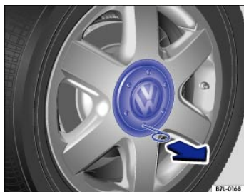
Fig. 218 Pulling the hubcap off.
