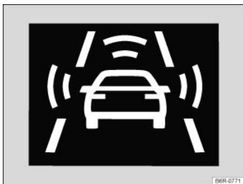
Fig. 164 In the instrument cluster display: Advance warning (symbol displayed in color on an instrument cluster with color display).
