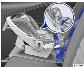
Fig. 77 Rearward-facing infant seat properly installed on the rear seat.
