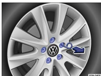
Fig. 220 Pulling cover caps off wheel bolts.
