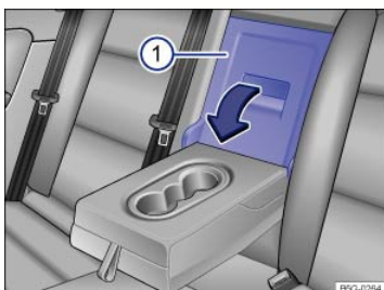
Fig. 101 In the rear seat backrest: Opening the luggage compartment pass-through.
