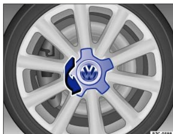
Fig. 219 Twisting the hubcap off.
