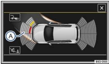
Fig. 177 PDC display (depending on vehicle equipment): Vehicle path display with steering input.
