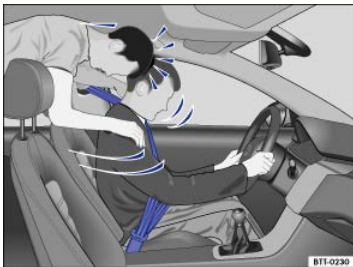
Fig. 60 Unbelted passengers in the rear seats are thrown forward on top of the belted driver.
