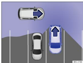
Fig. 185 Rear Traffic Alert: Monitored area around the vehicle that is backing out of a parking space.
