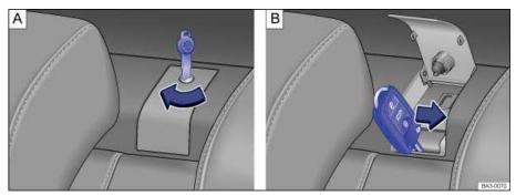
Fig. 198 Behind the rear seat backrest on the driver side: releasing the rear seat backrest.
