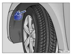
Fig. 218 In the wheel housing: Removing cover.
