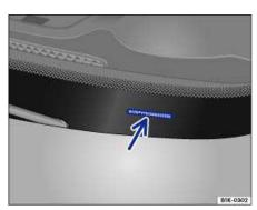
Fig. 19 Vehicle identification number (VIN).
