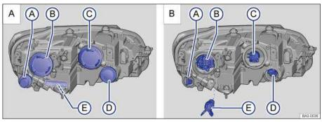
**Fig. 217** In the engine compartment: Covers in the left headlight assembly: A Side marker light, B Low beam headlight, C High beam headlight, D Turn signal and parking light, E Daytime running light.
