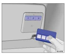
Fig. 52 In the driver side sun visor: The remote control and buttons for the HomeLink Universal Transmitter.
