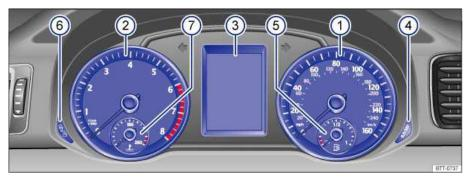
Fig. 10 Instrument cluster in the instrument panel.
