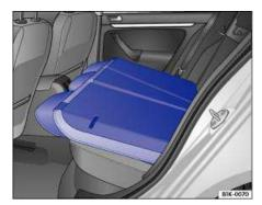
Fig. 113 Rear seat bench: Seat backrest folded down.
