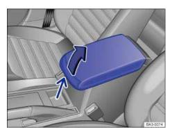
Fig. 135 In the front center armrest: Storage compartment.
