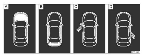
Fig. 12 In the instrument cluster display: A: Open engine hood, B: Open luggage compartment lid, C: Open front driver side door, D: Open rear passenger side door.
