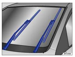
Fig. 104 Windshield wiper in service position.
