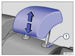
Fig. 61 Adjusting the rear head restraints.
