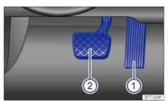
Fig. 153 Pedals in vehicles with automatic transmission: 1 Accelerator pedal, 2 Brake pedal.
