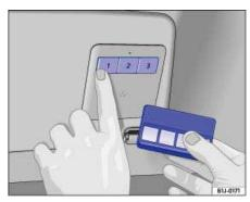
Fig. 53 To program: Simultaneously press the buttons for the HomeLink Universal Transmitter and the remote
