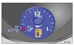
Fig. 172 In the instrument cluster: Fuel gauge.
