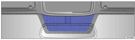
Fig. 102 Heat-reflective windshield with communications window (blue shaded area).
