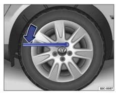
Fig. 208 Changing a wheel: Loosening wheel bolts.
