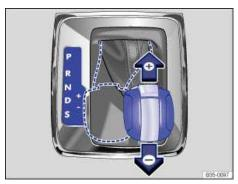
Fig. 157 Selector lever in Tiptronic position.
