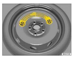
Fig. 125 In the luggage compartment: Compact spare wheel.
