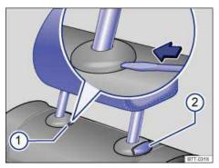
Fig. 63 Removing the rear head restraints.
