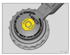
Fig. 160 In engine compartment: Brake fluid reservoir cap.
