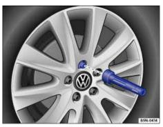
Fig. 212 Changing a wheel: remove previously loosened wheel bolts using the screwdriver handle.
