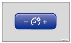
Fig. 100 To the left of the steering wheel: Control for instrument panel lighting.
