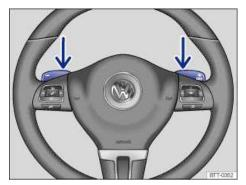
Fig. 158 Steering wheel with optional Tiptronic shift paddles.
