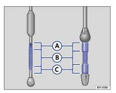
Fig. 179 Oil dipstick with engine oil level marks.
