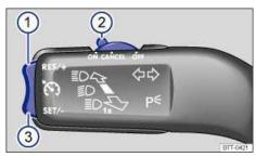
Fig. 165 On the left side of the steering column: Cruise control buttons and switches.
