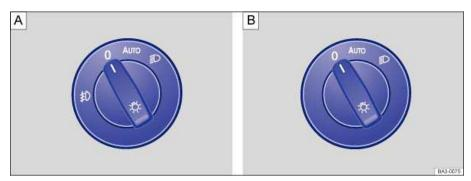
Fig. 98 Headlight switch next to the steering wheel: A vehicles with front fog lights. B vehicles without front fog lights.
