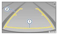
Fig. 168 On the screen: Static orientation lines for the parking space behind the vehicle.
