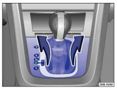
Fig. 202 Removing the selector gate cover.
