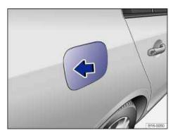
Fig. 173 Right rear side of vehicle: Opening the fuel filler flap.
