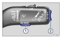
Fig. 15 Basic version (vehicles without menu control multi-function steering wheel): Control buttons 1 and 2 on the windshield wiper lever.
