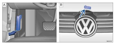
Fig. 178 A: In the footwell on the driver side: Inside engine hood release lever. B: Above the radiator grille: Outside engine hood release (under the hood).
