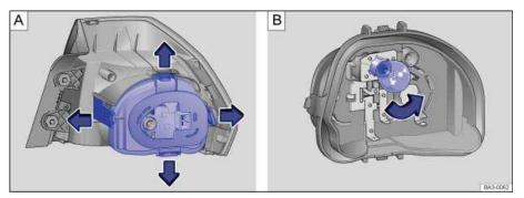
Fig. 224 A: Removing bulb socket assembly. B: Removing the light bulbs.
