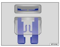
Fig. 215 Illustration of a blown fuse.
