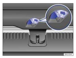
Fig. 199 Inside the luggage compartment: Unlocking the luggage compartment lid.
