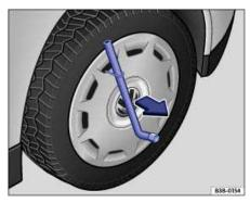
Fig. 207 Pulling the wheel cover off.
