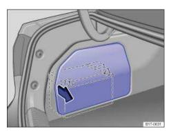
Fig. 186 In the side of the luggage compartment: On vehicles with 3.6 liter engines, the vehicle battery is on the left side of the luggage compartment.
