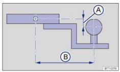
Fig. 117 Dimensions of the ball mount support.
