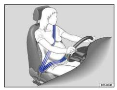
Fig. 78 Proper safety belt positioning for expectant mothers.
