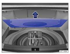
Fig. 204 In the luggage compartment under the floor panel: Compact spare wheel and vehicle tool kit.
