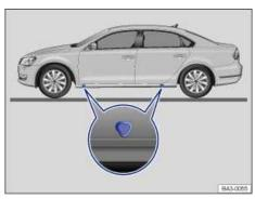
Fig. 210 Lift points for the jack.
