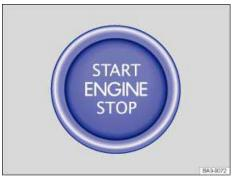
Fig. 148 In the center console: Starter button of the Keyless Access locking and starting system.
