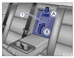
Fig. 114 In the rear seat backrest: Opening luggage compartment pass-through without lock.
