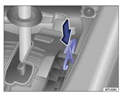
Fig. 203 Releasing the selector lever lock.
