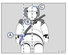
Fig. 83 Positioning of the safety belt extender.
