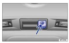
Fig. 166 In the luggage compartment lid: Location of the Rear Assist camera.
