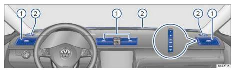
Fig. 171 In the instrument panel: Air vents.
