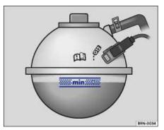
Fig. 183 Coolant expansion tank in the engine compartment.
