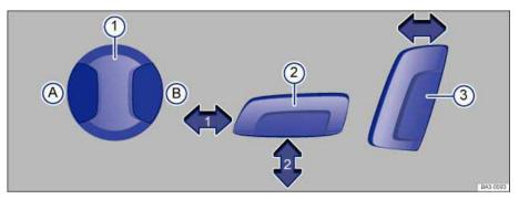
Fig. 59 Driver seat: controls to adjust lumbar support 1, seat cushion 2, and seat backrest angle 3.
