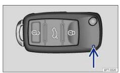
Fig. 27 Indicator light in the remote control vehicle key (version 1).
