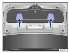
Fig. 46 Opened luggage compartment lid: Recessed grips for closing.
