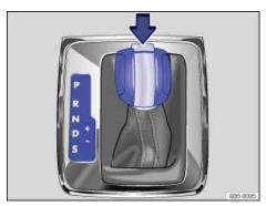
Fig. 156 Automatic transmission selector lever with shift lever release button (arrow).
