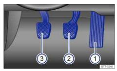
Fig. 152 Pedals in vehicles with manual transmission: 1 Accelerator pedal, 2 Brake pedal, 3 Clutch pedal.
