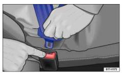
Fig. 76 Releasing the buckle tongue from the belt buckle.
