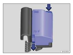
Fig. 214 In the engine compartment: Fuse box cover.
