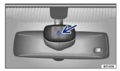
Fig. 106 Inside the front windshield above the inside mirror: Sensitive rain sensor surface.
