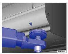
Fig. 188 Front lift point for workshop hoist or floor jack.
