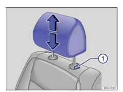
Fig. 60 Adjusting the front head restraints.
