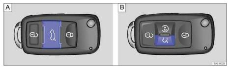
Fig. 42 In the remote control vehicle key (different versions): Button to unlock and open the luggage
