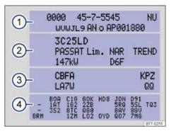
Fig. 18 Vehicle identification label: shown in the example with engine identification code CBFA 3.
