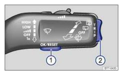
Fig. 17 Premium version (vehicles without menu control multi-function steering wheel): Control buttons 1 and 2 on the windshield wiper lever.
