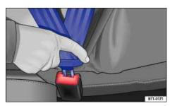
Fig. 75 Inserting the buckle tongue into the belt buckle.
