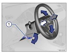
Fig. 64 Manual adjustment for the steering wheel position.
