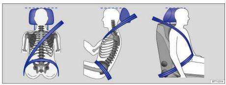
Fig. 77 Proper safety belt positioning and head restraint adjustment.
