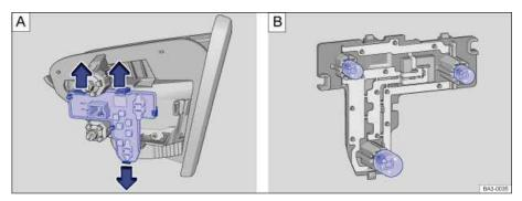
Fig. 222 A: Taillight assembly: removing the bulb socket assembly. B: Removing the light bulbs.
