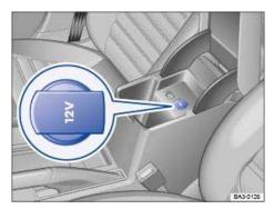
Fig. 146 12 Volt socket in the front center armrest.
