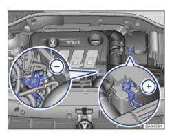
Fig. 228 In the engine compartment (2.0 liter TDI engine): Positive jump-start terminal + and negative jump-
