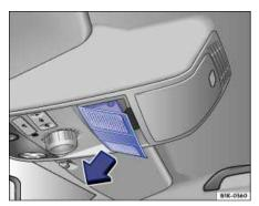
Fig. 200 In headliner: Removing cover.
