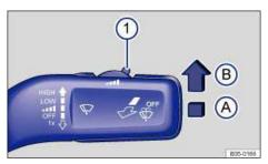
Fig. 105 Windshield wiper lever: Adjusting rain sensor 1.
