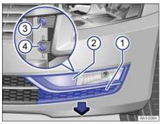
Fig. 219 In left front bumper: Removing light assembly.
