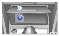
Fig. 145 12 Volt socket in the front center console.
