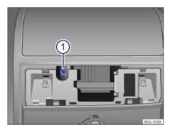
Fig. 201 Hexagonal head screw for closing the power sunroof.
