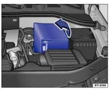
Fig. 185 In the engine compartment: Open the sleeve covering of the vehicle battery.
