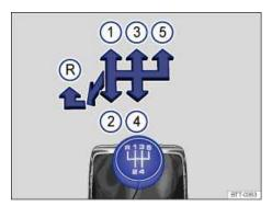
Fig. 154 Gearshift pattern of a 5-speed manual transmission.
