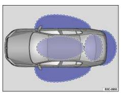
Fig. 38 Ranges of the Keyless Access locking and starting system. Outside the vehicle: Unlocking range. Inside the vehicle: Starting range.
