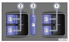
Fig. 47 In the driver door: Switches for front and rear power windows.
