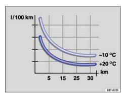
Fig. 162 Fuel consumption in I/100 km at 2 different outside air temperatures.
