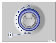
Fig. 49 In the headliner: Sunroof rotary switch.
