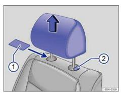
Fig. 62 Removing the front head restraints.
