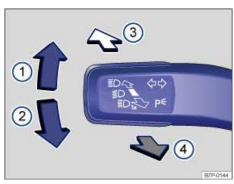
Fig. 97 Turn signal lever and high beam switch.
