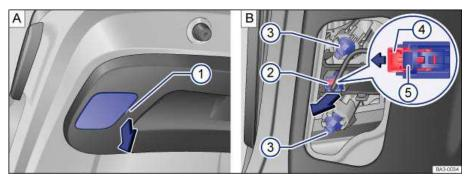
Fig. 221 A: In the luggage compartment lid: Removing the taillight cover. B: Removing the taillight assembly.
