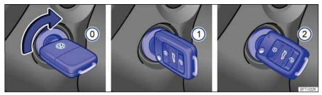
Fig. 147 In the ignition switch: Vehicle key positions.
