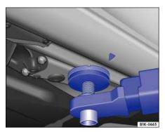
Fig. 189 Rear lift point for workshop hoist or floor jack.
