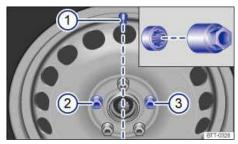
Fig. 209 Changing a wheel: tire valve 1 and installation points for the anti-theft wheel bolt 2 or 3 (where
