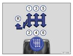
Fig. 155 Gearshift pattern of a 6-speed manual transmission.
