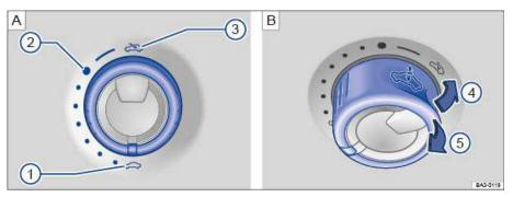
Fig. 48 In the headliner: Rotary switch for the power sunroof. (A) Turn the rotary switch to slide the sunroof open or closed. (B) Press or pull the switch to tilt open or to close.
