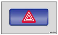
Fig. 190 In the center of the instrument panel: Switch for emergency flashers.
