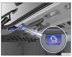
**Fig. 112** On the left side of the luggage compartment: Release lever for the left-side rear seat backrest. The release lever for the right-side rear seat backrest is on the right side of the luggage compartment.
