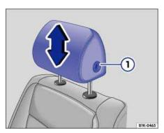
Fig. 46 Adjusting the front head restraints.
