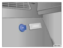
Fig. 132 In the luggage compartment: 12 Volt socket.
