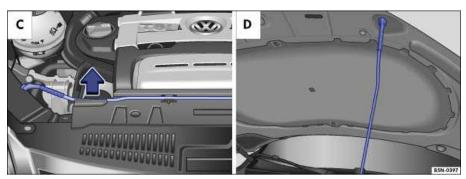
Fig. 163 A: Bracket for hood support in the engine compartment. B: Hood propped open.
