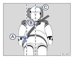
Fig. 69 Positioning of the safety belt extender.
