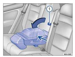
Fig. 52 Folded down rear center armrest with storage compartment (arrow).
