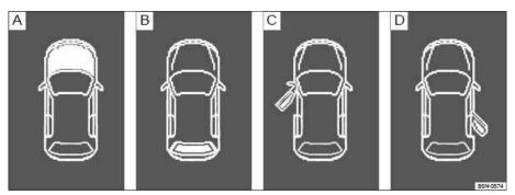
Fig. 13 In the instrument cluster display: A: Open engine hood, B: Open rear hatch, C: Open front driver side
