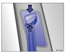
Fig. 67 Next to the front seats: Safety belt height adjuster.
