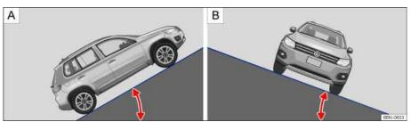
Fig. 159 Illustration of A: Ascent angle. B: Lateral gradient.
