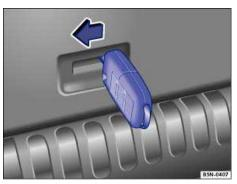
Fig. 181 View from luggage compartment: Emergency unlocking rear hatch with the remote control vehicle
