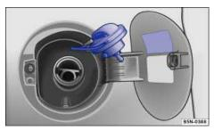
Fig. 158 Fuel cap placed on the open fuel filler flap.
