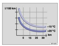
Fig. 146 Fuel consumption in I/100 km at 2 different outside air temperatures.
