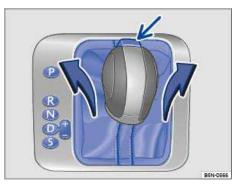
Fig. 182 Removing the selector gate cover.
