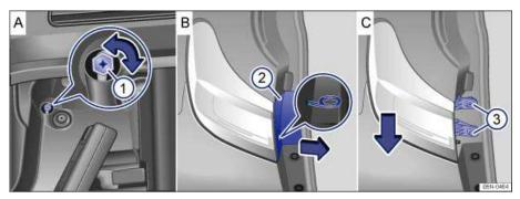
Fig. 206 In the side of the luggage compartment: Releasing the tail light, removing the trim panel and removing the screws.
