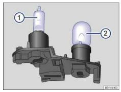
Fig. 205 Bulb holder with backup light bulb 2.
