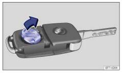
Fig. 24 Remote control vehicle key: Remove old battery.
