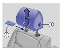
Fig. 48 Removing the front head restraints.
