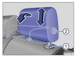
Fig. 47 Adjusting or folding the rear head restraints.
