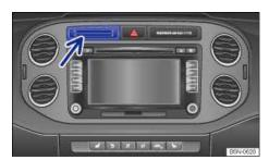
Fig. 124 In the upper part of the center console: Card holder.
