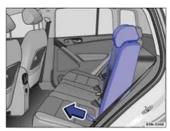
Fig. 45 Adjusting the rear backrest.
