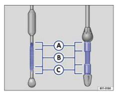
Fig. 164 Oil dipstick with engine oil level marks.
