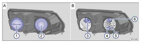
Fig. 200 In the engine compartment: Cover 1 on the left headlight for the low beam bulb holder 3 and cover 2 for the parking light bulb holder 4, turn signal bulb holder 5 and high beam or daytime running light bulb 6.
