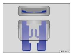
Fig. 198 Illustration of a blown fuse.
