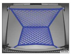
Fig. 104 In the luggage compartment: Luggage net hooked in place.
