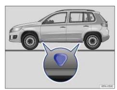
Fig. 192 Lift points for the jack.
