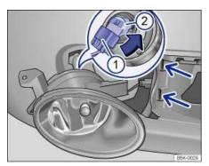
Fig. 203 Replacing light bulb in headlight.
