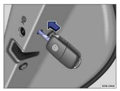
Fig. 180 On the front side of the right rear door: Manual vehicle locking with the key bit in the vehicle key.
