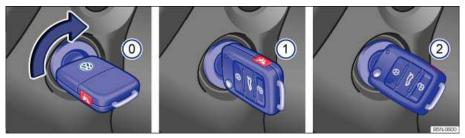
Fig. 134 In the ignition switch: Vehicle key positions.
