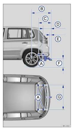
Fig. 110 Dimensions and attachment points for retrofitting a trailer hitch.
