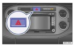
Fig. 177 In the center of the instrument panel: Switch for emergency flashers.
