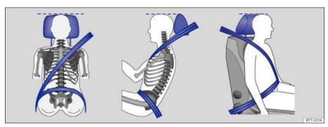
Fig. 65 Proper safety belt positioning and head restraint adjustment.
