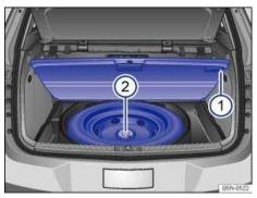
Fig. 114 In the luggage compartment: Compact spare wheel.
