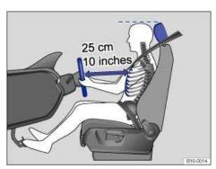
Fig. 39 The driver should never sit closer than 10 inches (25 cm) of the steering wheel.
