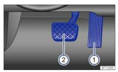
Fig. 138 Pedals in vehicles with automatic transmission: 1 Accelerator pedal, 2 Brake pedal.
