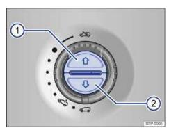
Fig. 174 In the headliner: Buttons for sunshade.
