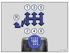
Fig. 139 Gearshift pattern of a 6-speed manual transmission.
