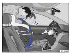
Fig. 61 Unbelted passengers in the rear seats are thrown forward on top of the belted driver.
