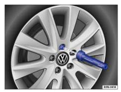
Fig. 194 Changing a wheel: Remove previously loosened wheel bolts using the screwdriver handle.
