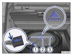
Fig. 195 Under the luggage compartment floor: Fender Premium Audio subwoofer.
