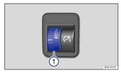
Fig. 85 Next to the headlight switch: Control for instrument cluster lighting.
