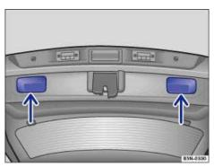
Fig. 33 Opened rear hatch: Recessed grips for closing
