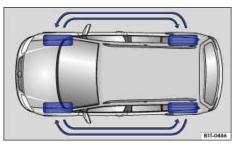
Fig. 111 Tire rotation diagram.
