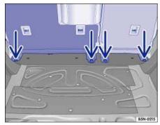
Fig. 99 Rear attachment of the rear seat.
