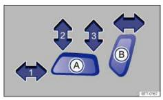
Fig. 42 Driver seat controls to adjust the seat backward and forward, change seat cushion height and angle, and adjust backrest angle.
