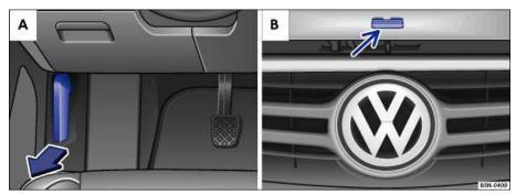
Fig. 162 A: Inside engine hood release in the footwell on the driver side. B: Outside engine hood release in
