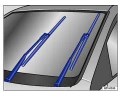
Fig. 90 Windshield wiper in service position.
