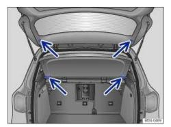
Fig. 100 Installing and removing the luggage compartment cover.
