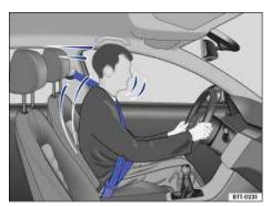
Fig. 62 Belted driver secured by the correctly worn safety belt in the event of a sudden braking maneuver.
