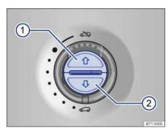
Fig. 173 In the headliner: Buttons for sunshade.
