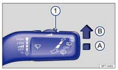
Fig. 91 Windshield wiper lever: Adjusting rain sensor 1.
