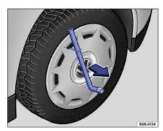
Fig. 190 Pulling the wheel cover off.
