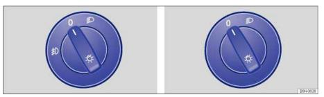
Fig. 84 Headlight switch next to the steering wheel: A: Vehicles with front fog lights. B: Vehicles without front
