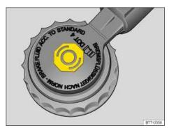
Fig. 144 In engine compartment: Brake fluid reservoir cap
