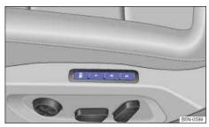
Fig. 54 Memory buttons on the outer side of the driver seat.
