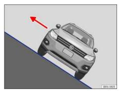
Fig. 161 On a slope, always exit on the uphill side of the vehicle.
