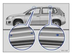
Fig. 107 Vehicles without roof railing: Attachment points for the base carrier and roof rack.
