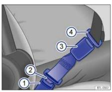
Fig. 68 A safety belt extender properly attached to the factory-installed safety belt.
