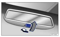
Fig. 94 Manually adjustable inside mirror.
