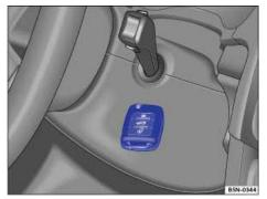
Fig. 136 Emergency starting feature on vehicles with Keyless Access.
