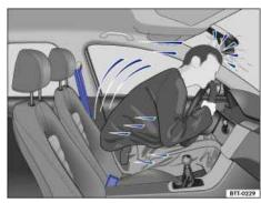
Fig. 60 The unbelted driver is thrown forward.
