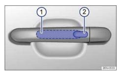
**Fig. 28** Keyless Access locking and starting system: Sensor 1 for unlocking on the inside of the front door handles. Sensor for locking 2 on the outside of the door handles.
