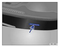
Fig. 19 Vehicle identification number (VIN).
