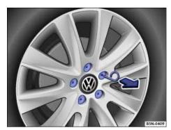
Fig. 189 Pulling cover caps off wheel bolts.
