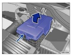
Fig. 169 In the engine compartment: Remove the cover from the vehicle battery.
