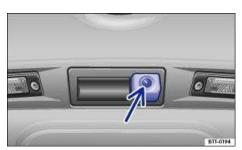
Fig. 150 In the luggage compartment lid: Location of the Rear Assist camera.
