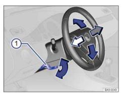
Fig. 50 Manual adjustment for steering wheel position.
