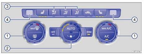
Fig. 154 In the center console: Climatronic controls.
