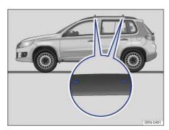
Fig. 108 Vehicles with roof railing: Attachment points for the base carrier and roof rack.
