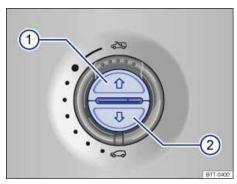
Fig. 37 In the headliner: Buttons for sunshade.
