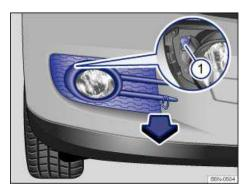
Fig. 202 In right front bumper: Removing light assembly.
