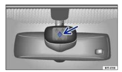
Fig. 92 Sensitive rain sensor surface.
