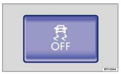
Fig. 143 In the center console: Button to manually switch ASR on and off.
