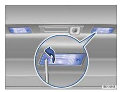
Fig. 209 In the rear hatch: Screwed license plate lamp.
