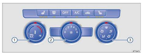
Fig. 153 In the center console: Manual AC controls.
