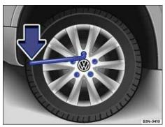
Fig. 191 Changing a wheel: Loosening wheel bolts.
