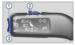
Fig. 149 On the left side of the steering column: Cruise control buttons and switches.
