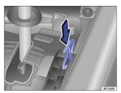
Fig. 183 Releasing the selector lever lock.
