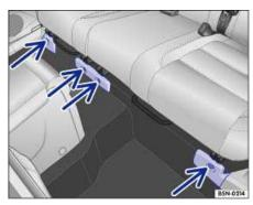
Fig. 98 Front attachment of the rear seat.
