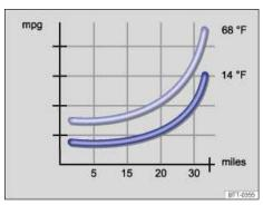
Fig. 145 Fuel consumption in mpg at 2 different outside air temperatures.
