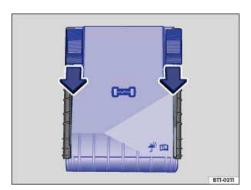
Fig. 197 In the engine compartment: Fuse box cover.
