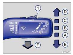
Fig. 88 Operating the front windshield wiper.
