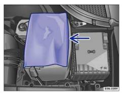
Fig. 170 In the engine compartment: Open the sleeve covering of the vehicle battery.
