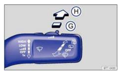
Fig. 89 Operating the rear wiper.
