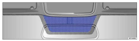
Fig. 87 Heat-reflective windshield with communications window (blue shaded area).
