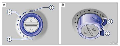
**Fig. 35** In the headliner: Rotary switch for the power sunroof. A: Turn the rotary switch to slide the sunroof open or closed. B: Press or pull the switch to tilt open or to close.
