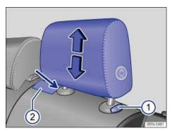
Fig. 49 Removing the rear head restraints.
