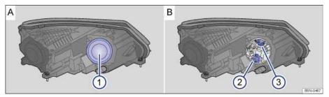
Fig. 201 In the engine compartment: cCover 1 on the left headlight for the turn signal bulb holder 2 and the cornering light bulb holder 3.
