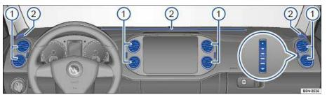
Fig. 155 In the instrument panel: Air vents.
