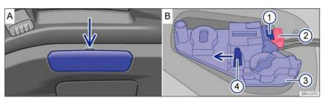
Fig. 204 In the rear hatch: Removing the cover and the bulb holder.
