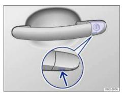
Fig. 178 Door handle on driver door: Concealed lock cylinder.
