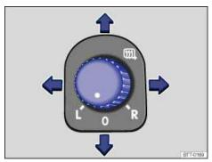
Fig. 96 In the driver door: Adjusting knob for outside mirrors.
