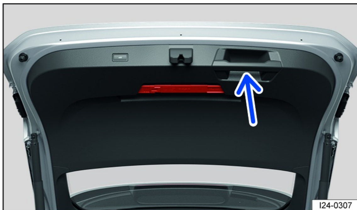
Fig. 48 In the open trunk lid: handle for closing the trunk lid (general example).
