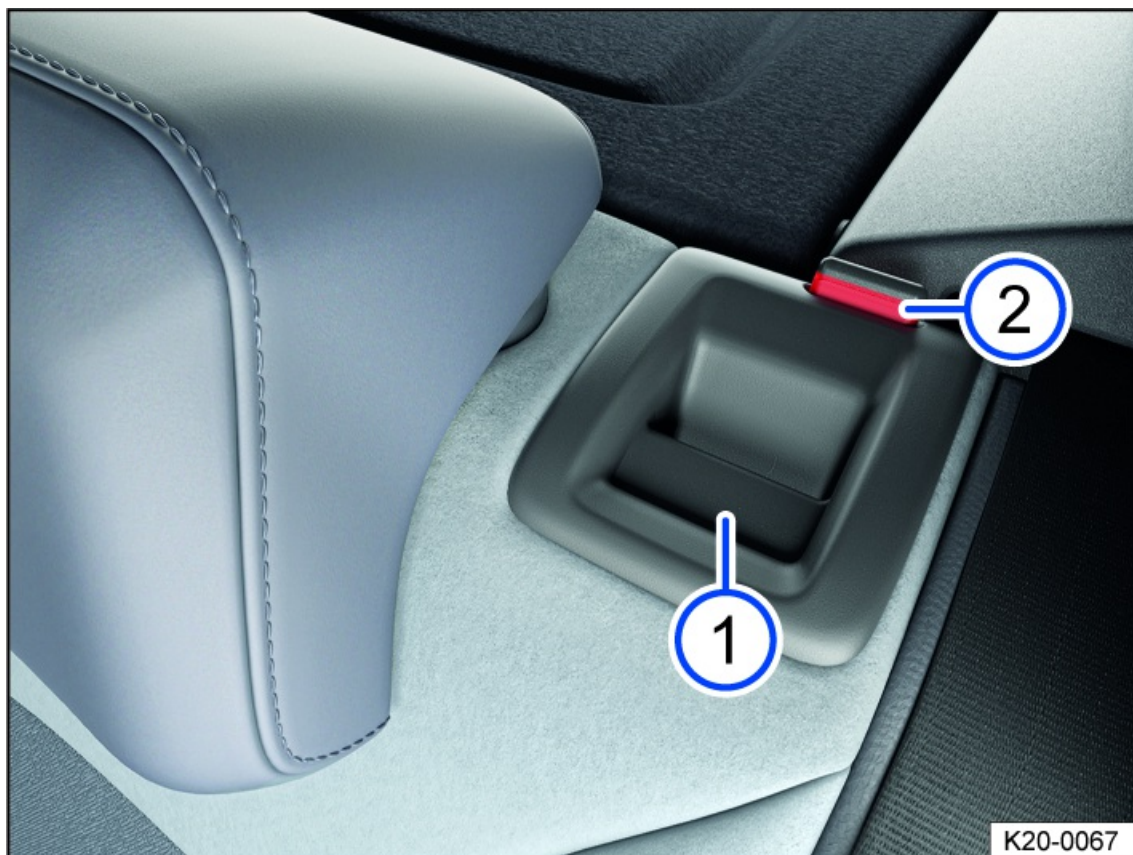
Fig. 59 In the rear seat backrest: release button.
