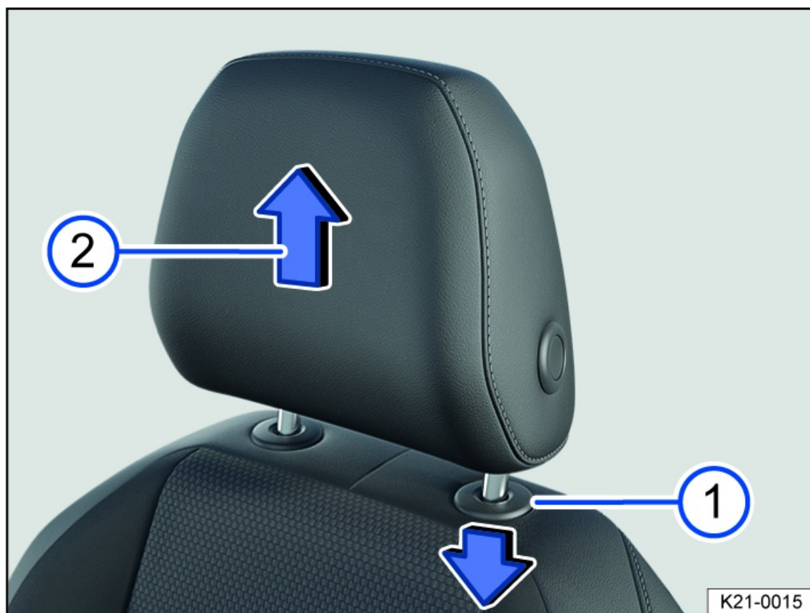
Fig. 63 Removing the front head restraint (general example).
