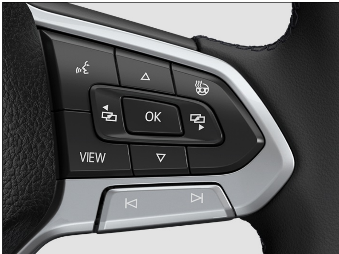
Fig. 9 Right-hand side of the multi-function steering wheel: operating the Pro digital instrument cluster (general example).
