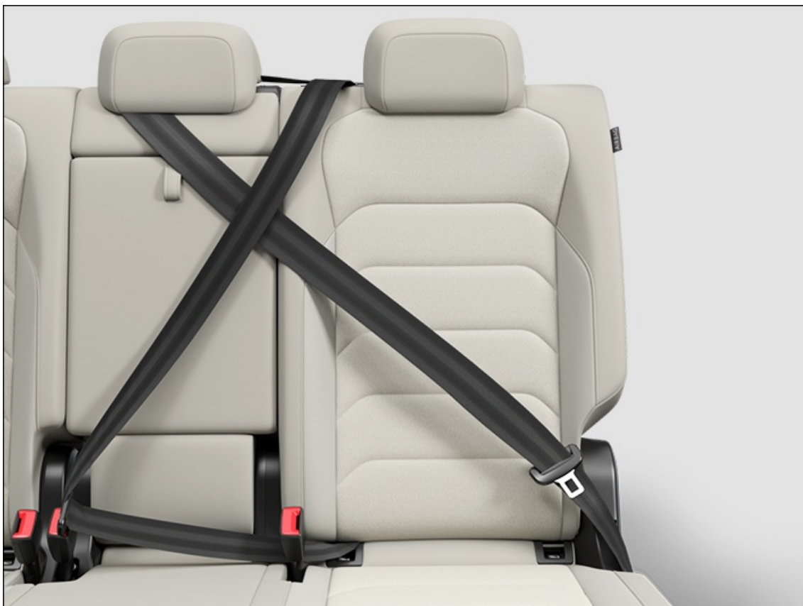
Fig. 31 Securing unused safety belts (general example).
