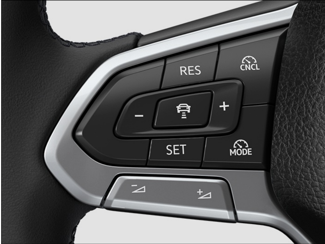
Fig. 100 Left side of the multi-function steering wheel.
