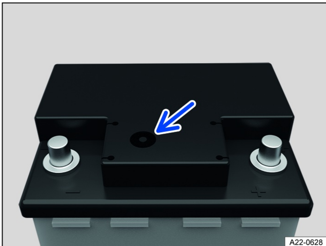
Fig. 164 On the top of the 12 V vehicle battery: Window (general example).
