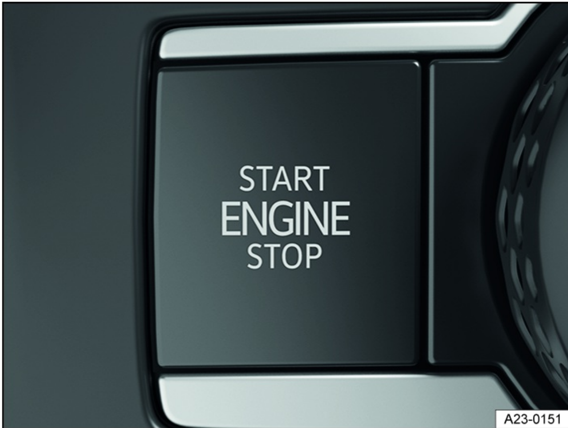
Fig. 84 In the lower section of the center console: starter button.
