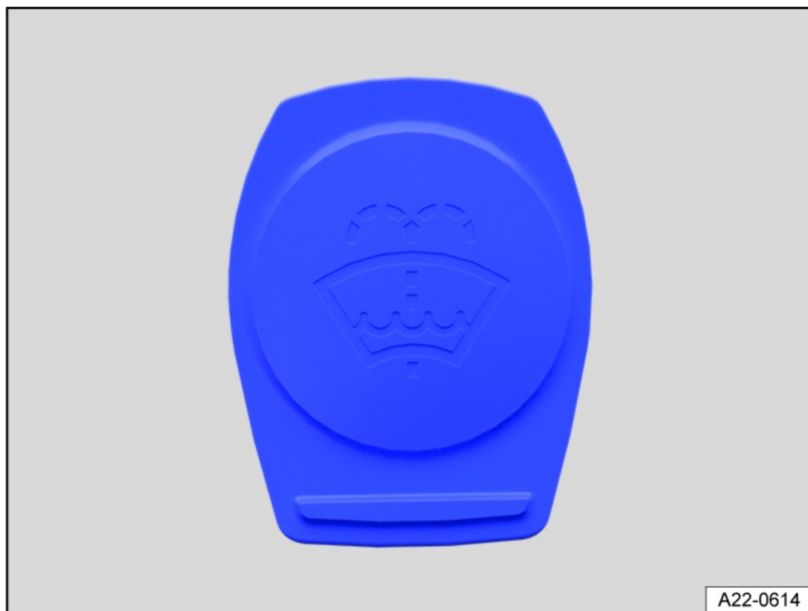
Fig. 156 In the hood space: Cap on the washer fluid reservoir (general example).
