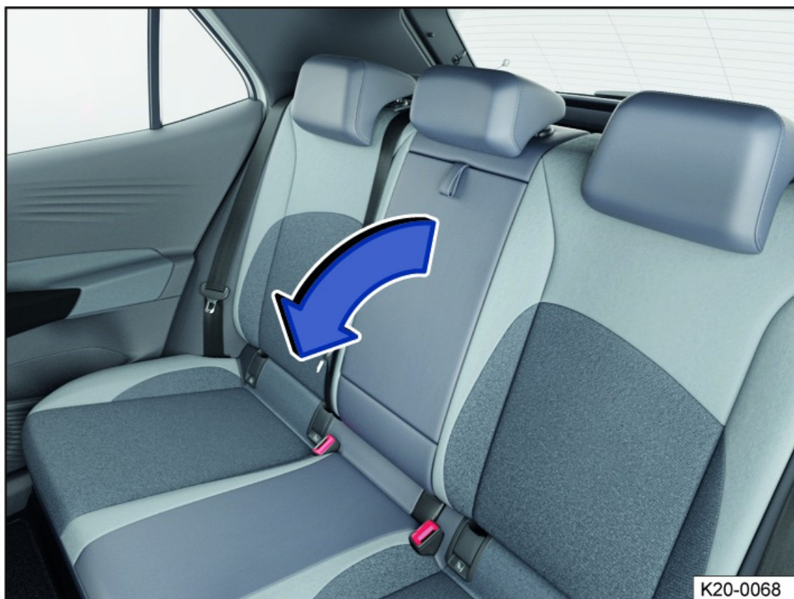
Fig. 66 In the backrest of the center seat: folding rear center armrest.
