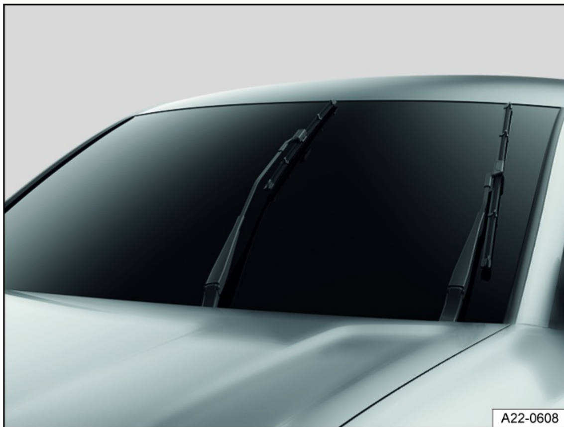
Fig. 140 Windshield wipers in service position (general example).
