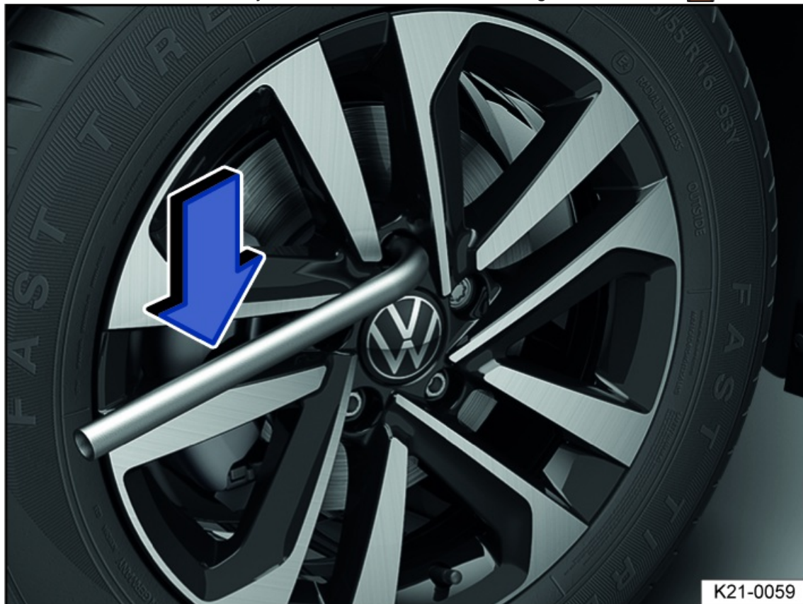
Fig. 174 Loosening wheel bolts.
