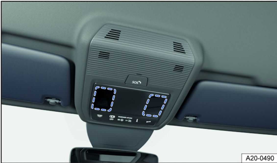
Fig. 73 On the overhead console: touch-sensitive reading lights.
