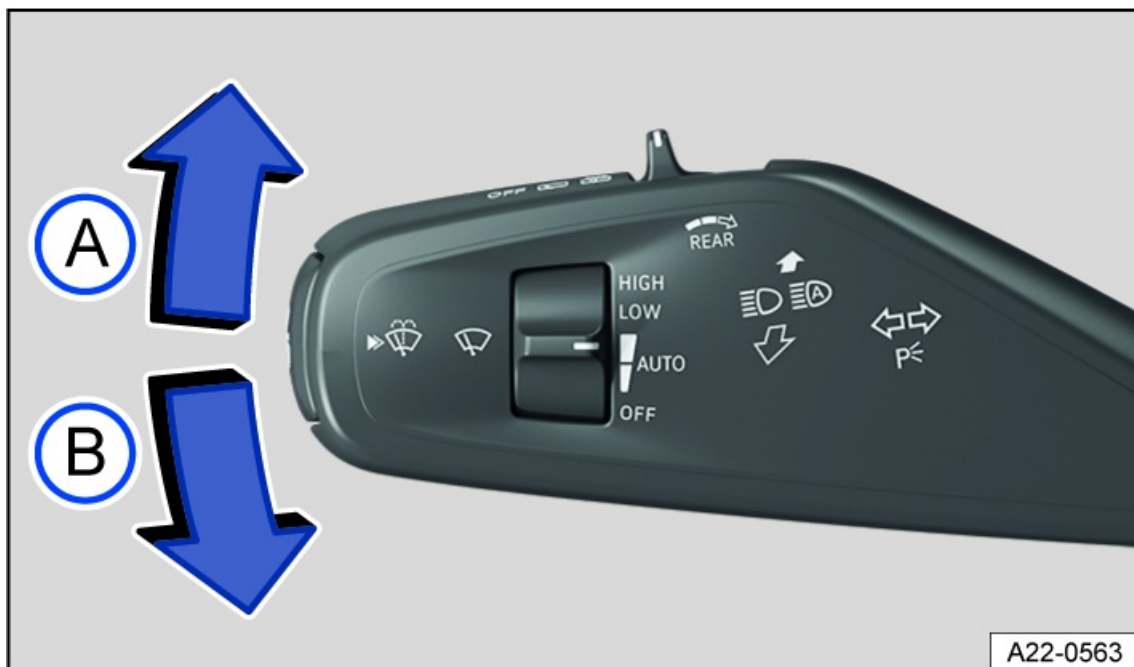
Fig. 69 On the left-hand side of the steering column: lever for turn signal, high beam and windshield wiper.
