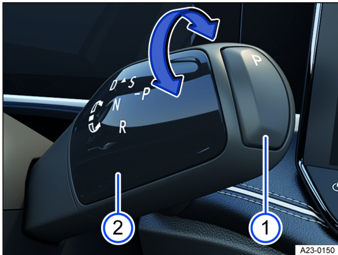
Fig. 86 On the right side of the steering column: driving mode selector for the automatic transmission.
