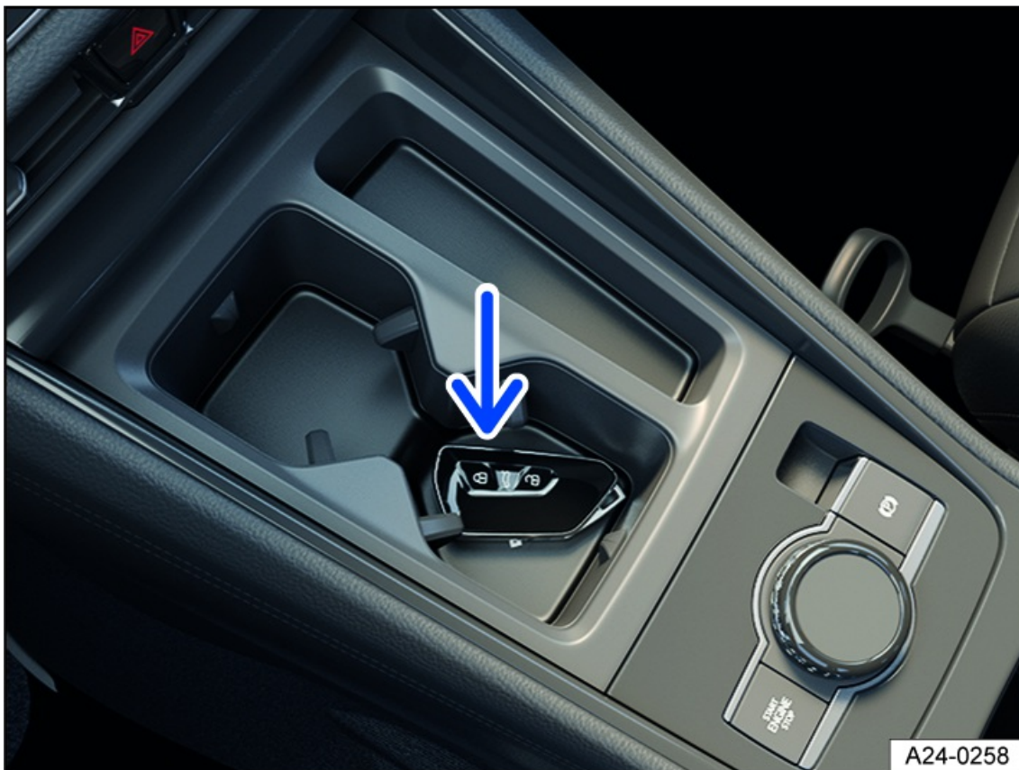
Fig. 85 In the center armrest: Emergency start function.
