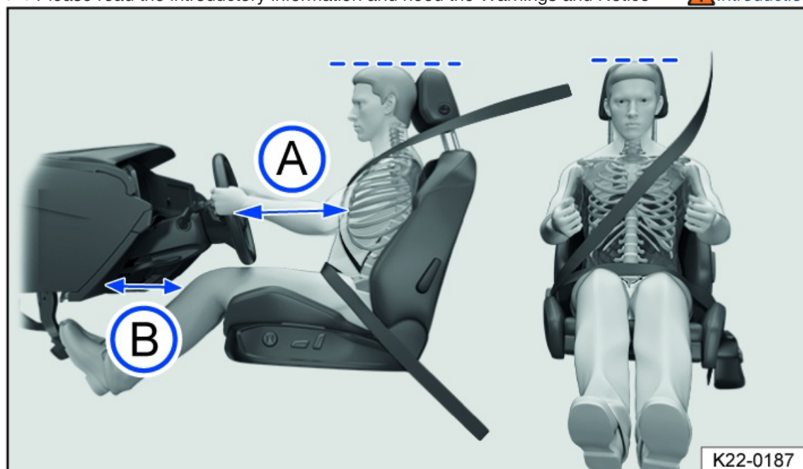
Fig. 16 Correct distance between the driver and the steering wheel, correct safety belt position and correct head restraint adjustment (general example).
