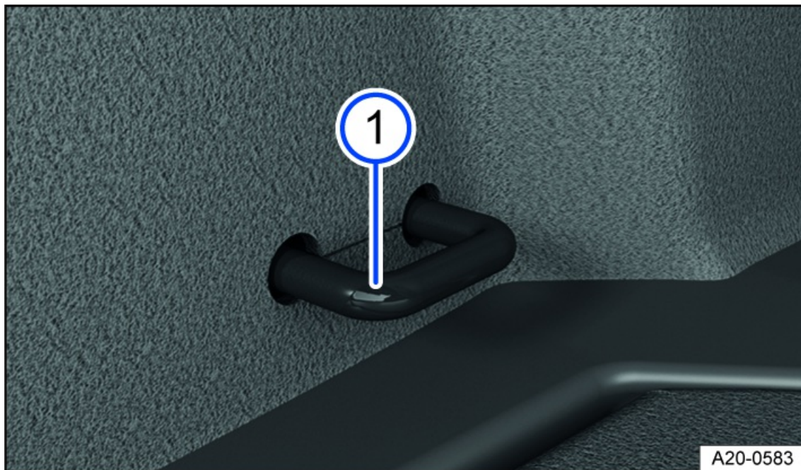
Fig. 131 In the luggage compartment: rigid tie-down (general example).
