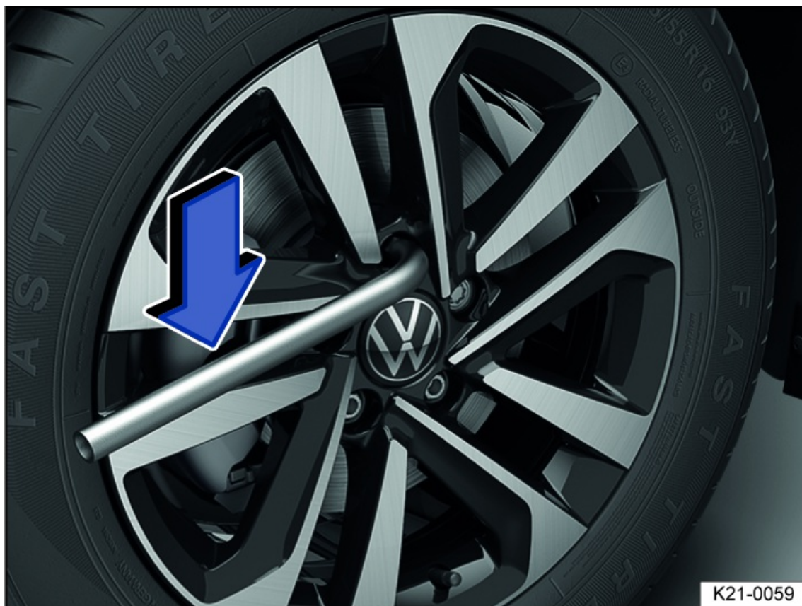
Fig. 178 Removing wheel bolts with the lug wrench.
