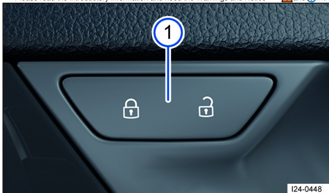
Fig. 43 In the driver's door: Central locking button (general example).
