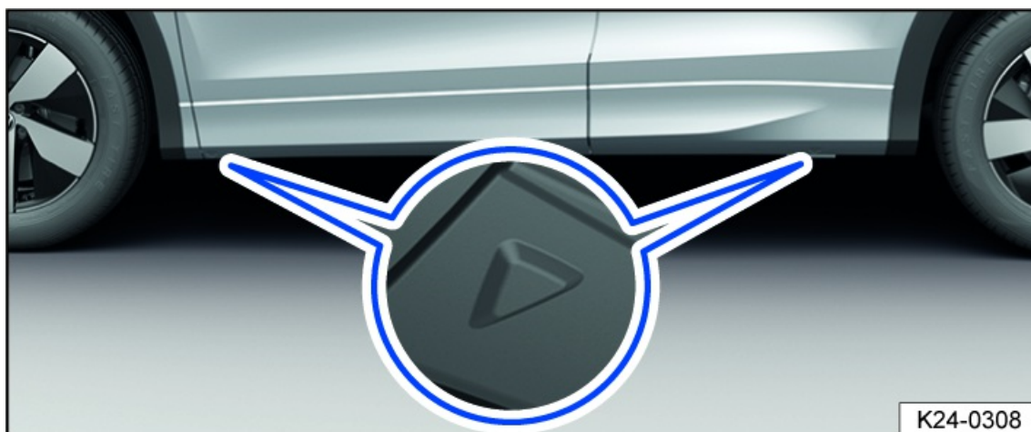
Fig. 175 On the side sill: markings for the jack lift points.
