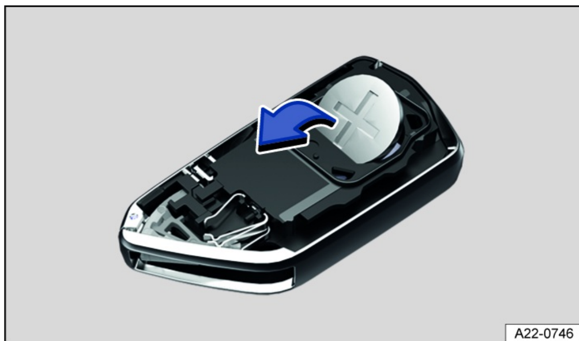
Fig. 40 Vehicle key: replacing the button cell battery
