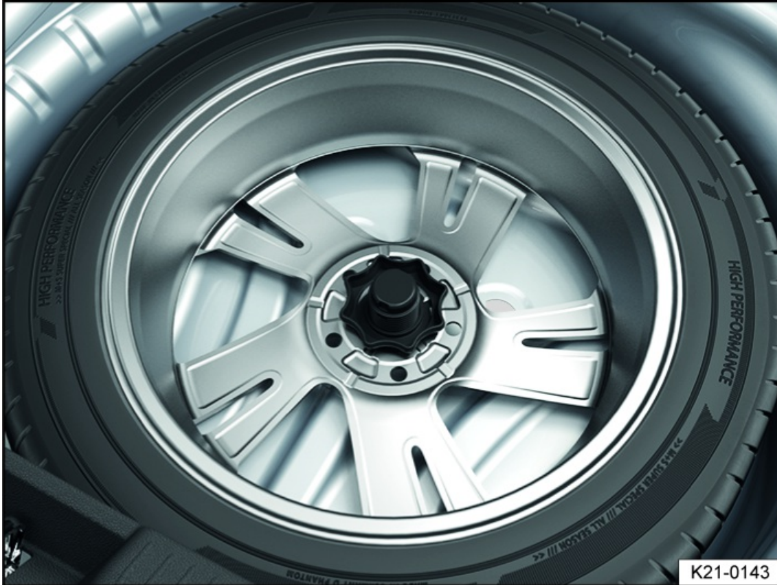
Fig. 172 Under the luggage compartment floor: handwheel to secure the spare wheel.
