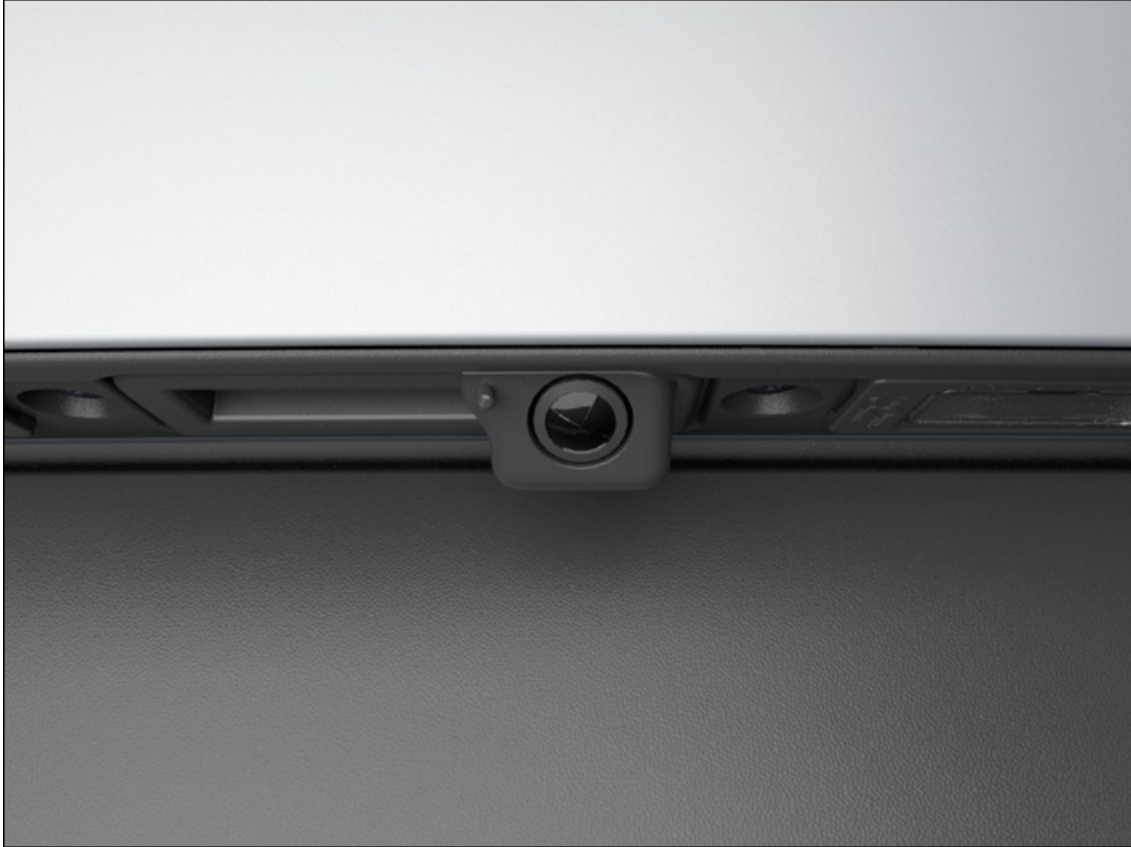
Fig. 183 In the rear of the vehicle: Rear View Camera system on the handle (general example).
