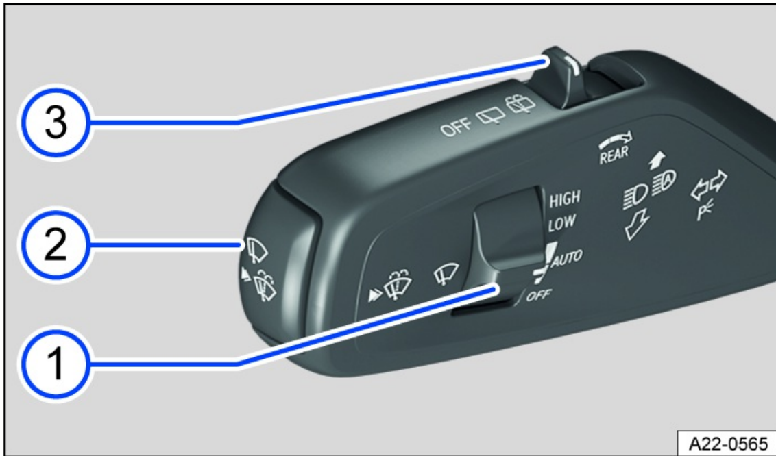
Fig. 74 On the left-hand side of the steering column: lever for turn signal, high beam and windshield wiper.
