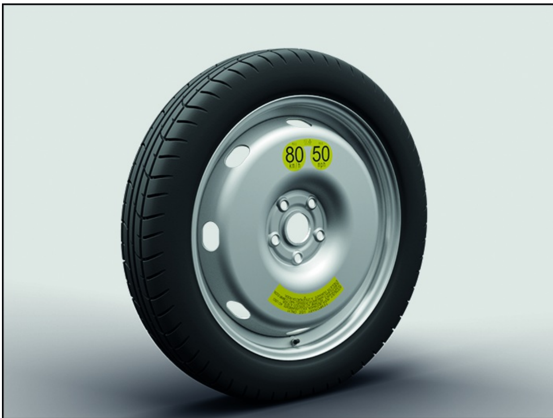
Fig. 166 Compact spare wheel.
