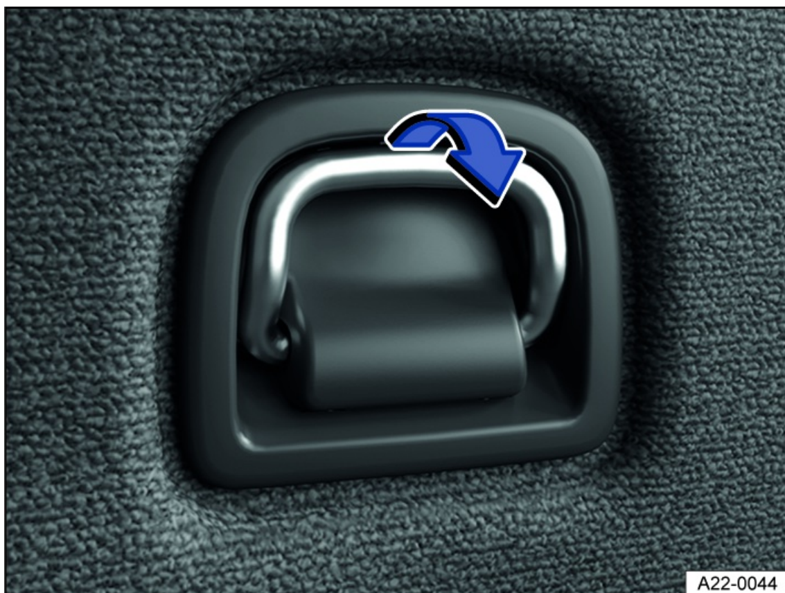
Fig. 132 In the luggage compartment: Foldable tie-down (general example).
