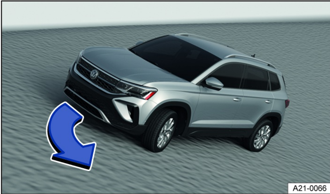
Fig. 92 General example: steering downhill along the fall line.
