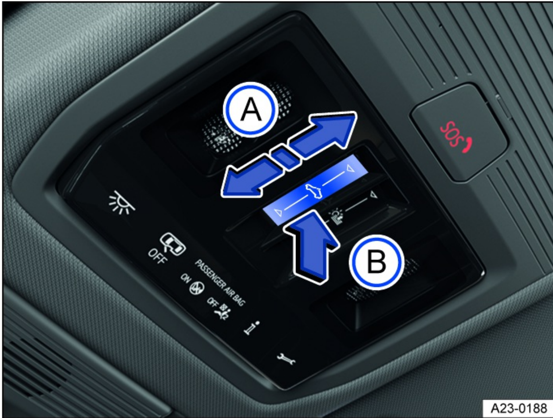
Fig. 53 In the headliner: Control for the tilting and sliding panoramic sunroof.
