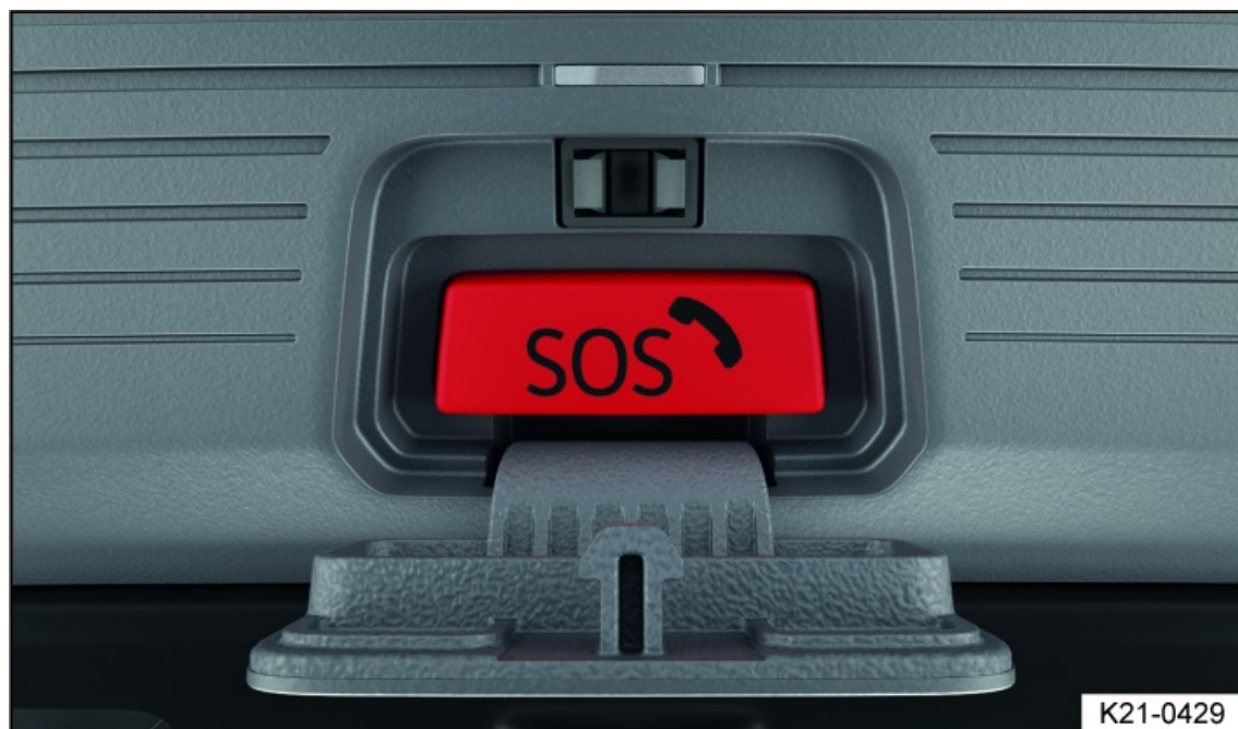
Fig. 34 Located on the roof console: Emergency Call Service button.
