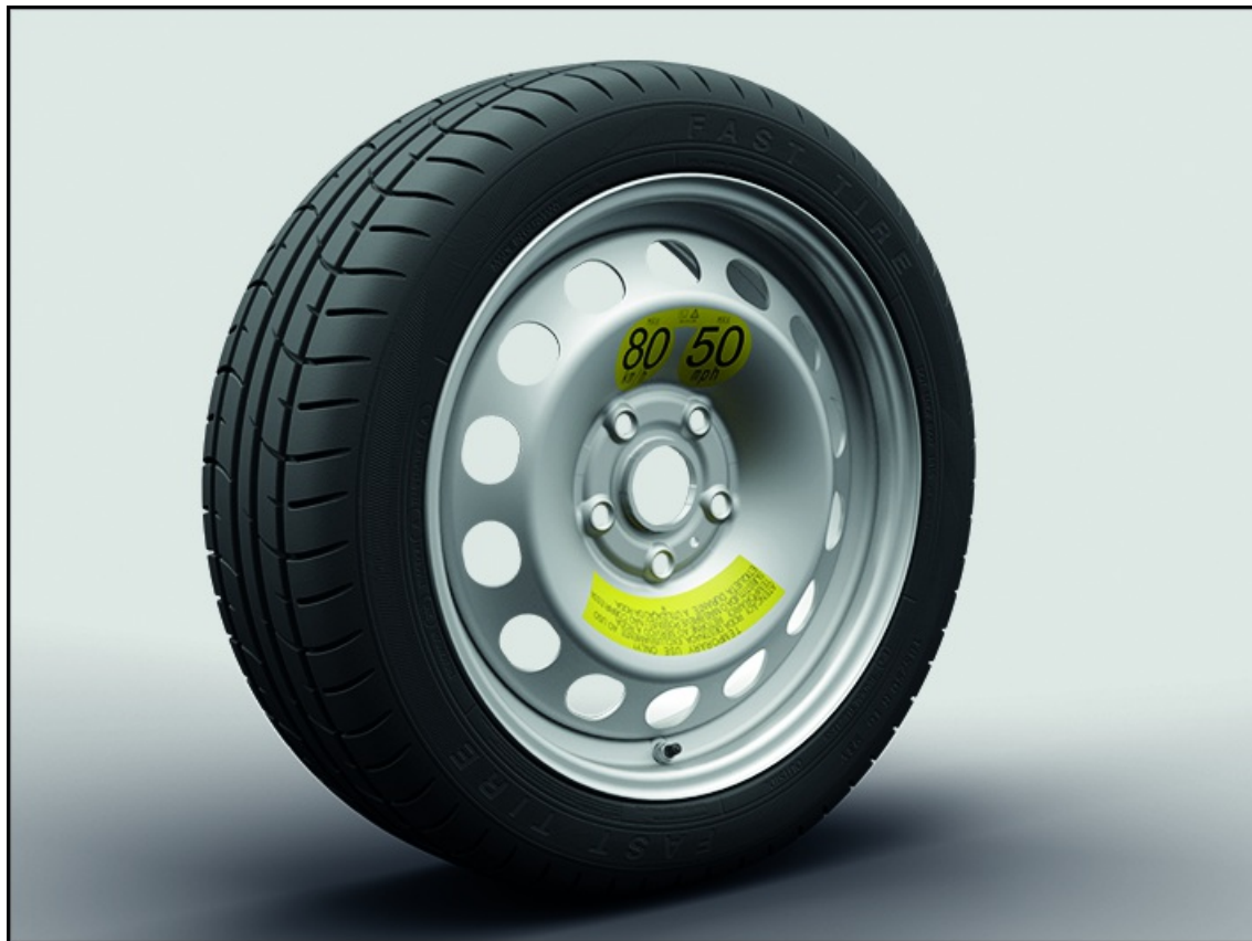
Fig. 165 Space-saving spare wheel.
