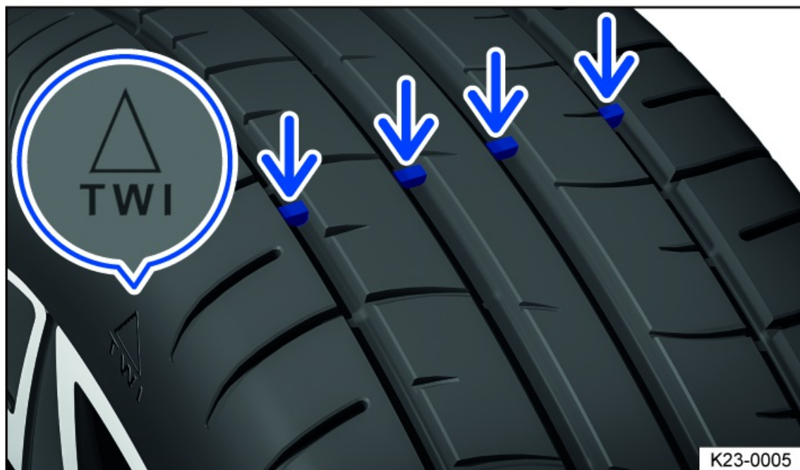
Fig. 169 In the tread grooves: wear indicator.
