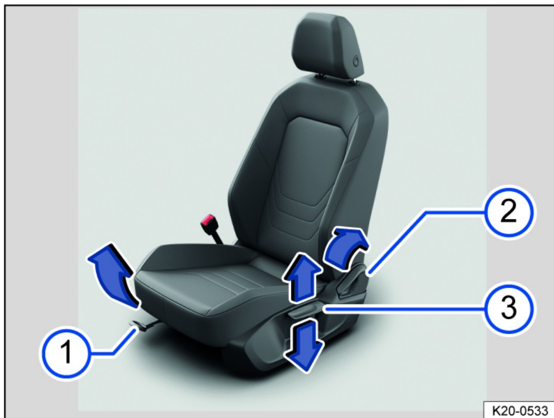
Fig. 56 On the driver seat: Controls.
