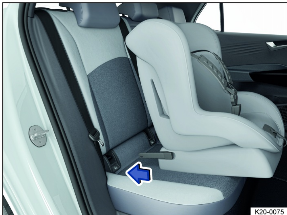
Fig. 28 Fitting a child restraint with arms (general example).
