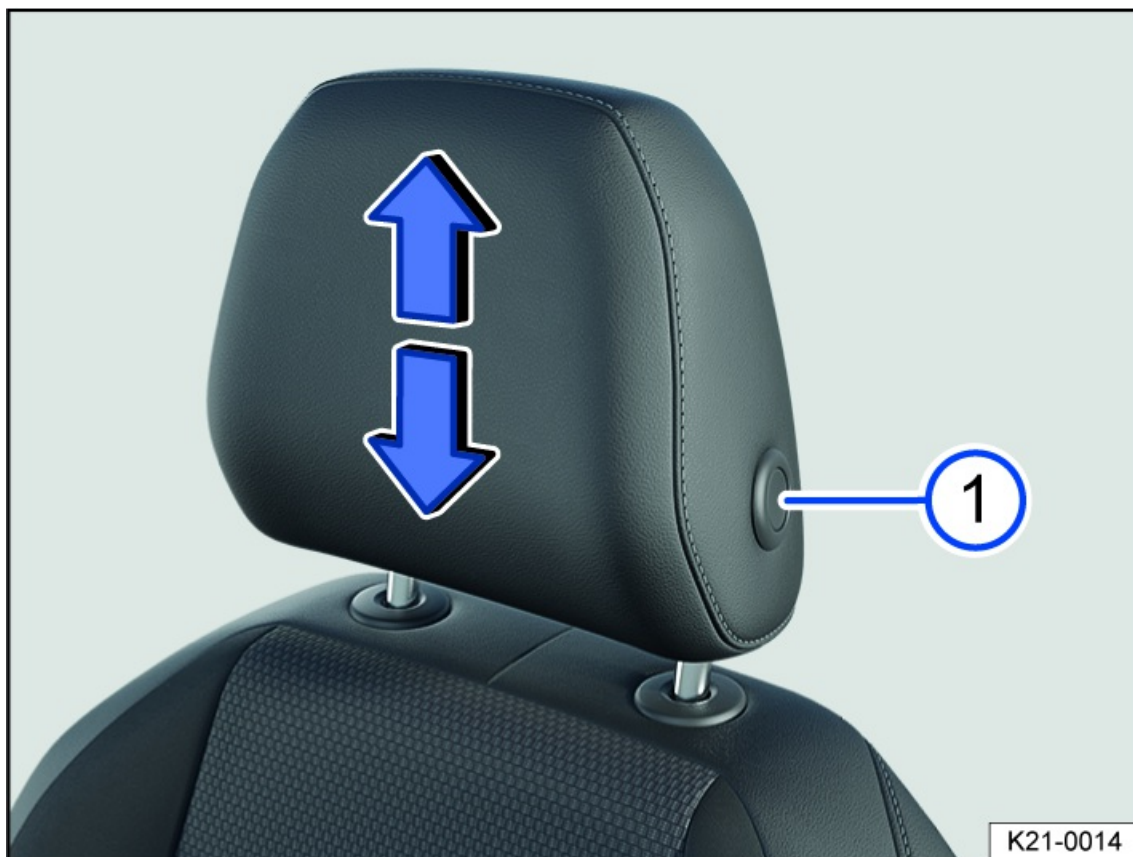
Fig. 61 Adjusting the front head restraint (general example).
