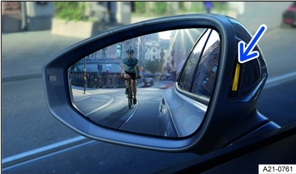
Fig. 110 In the outside mirror housing: display of the exit warning system (general example).
