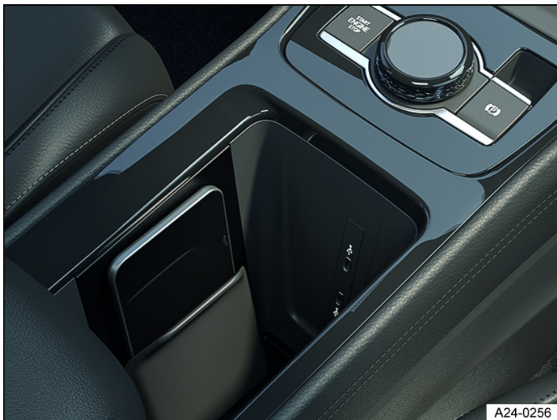
Fig. 125 In the center console: storage compartment with a holder for wireless charging (general example). The charging capacity is 15 W.
