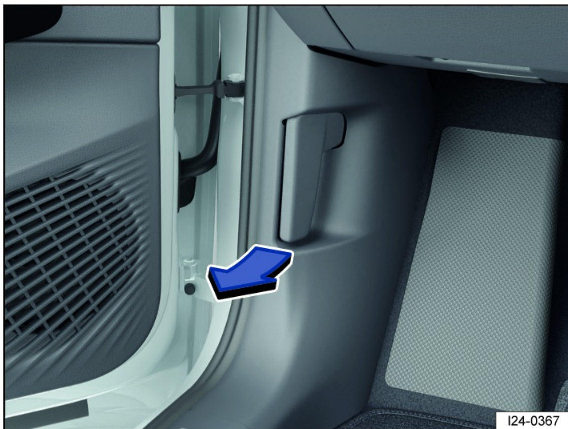
Fig. 153 In the driver's side footwell: Release lever for the hood (general example).
