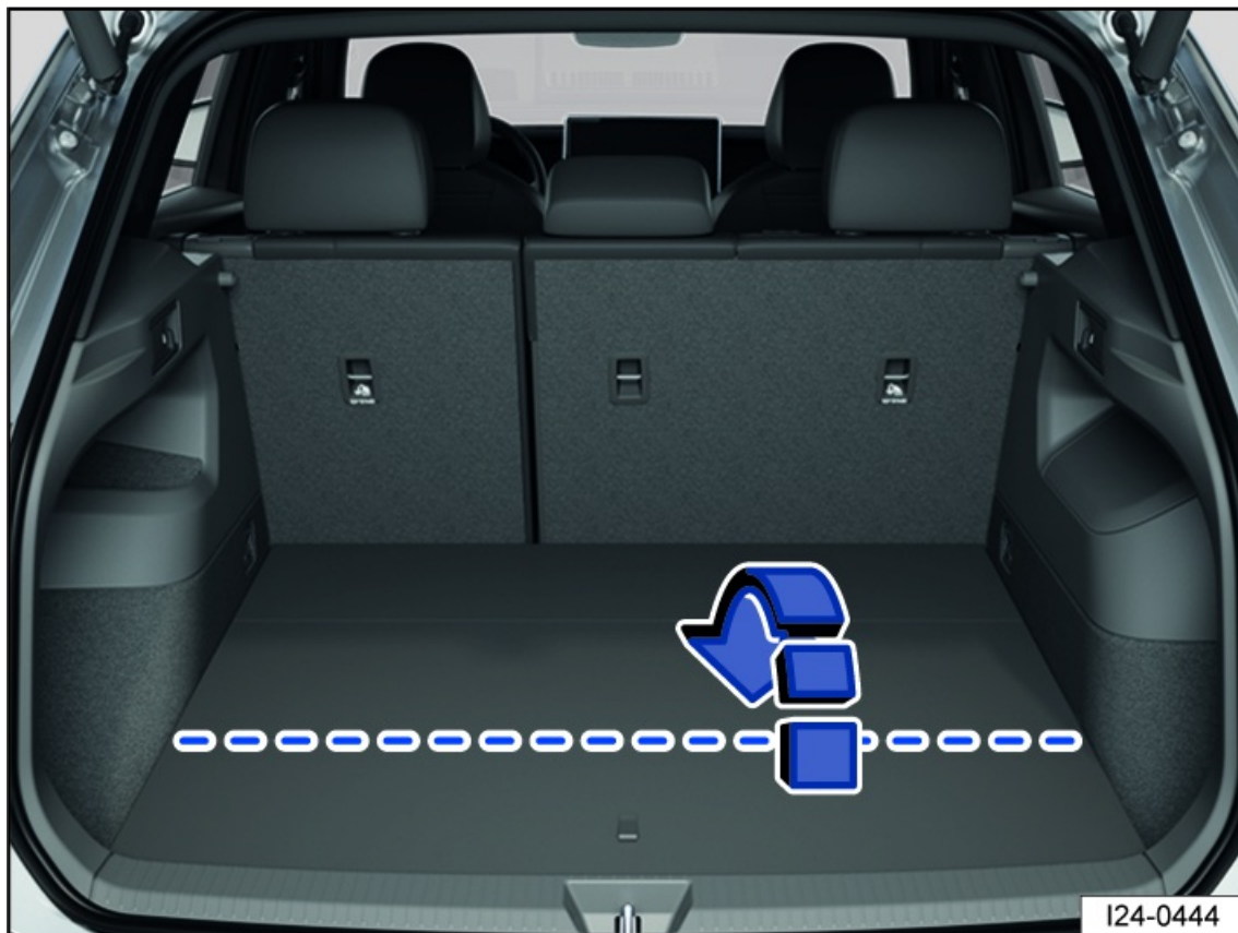
Fig. 129 In the luggage compartment: fold the rear section of the luggage compartment floor forward.
