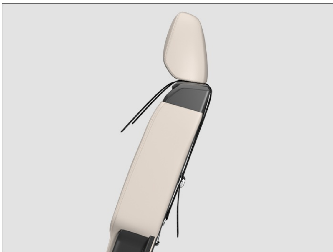
Fig. 30 On the back of the rear seats: attached top tether safety belt.
