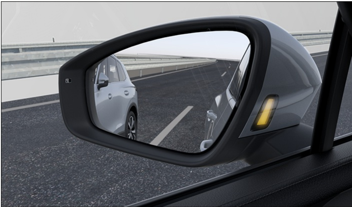
Fig. 108 In the outside mirror housing: displays of Side Assist.
