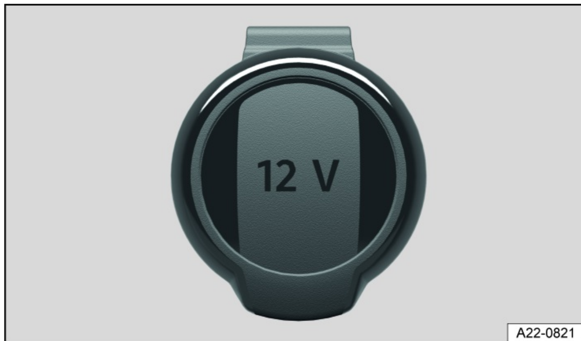
Fig. 124 In the storage compartment in the center console under the center armrest, in the luggage compartment on the right-hand side: folding 12 V socket (general example).
