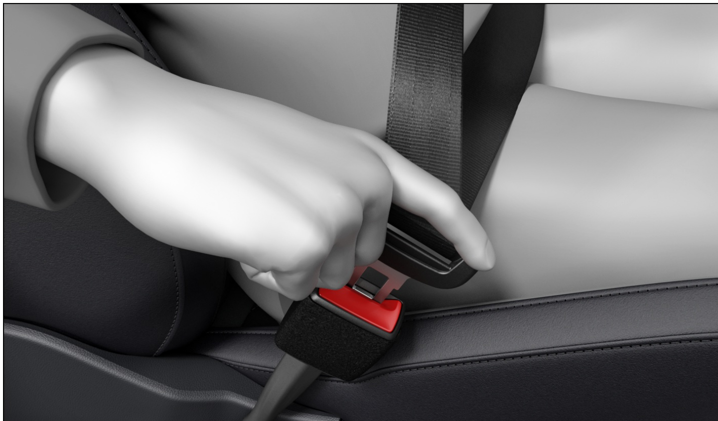
Fig. 18 Inserting the buckle tongue into the safety belt buckle (general example).
