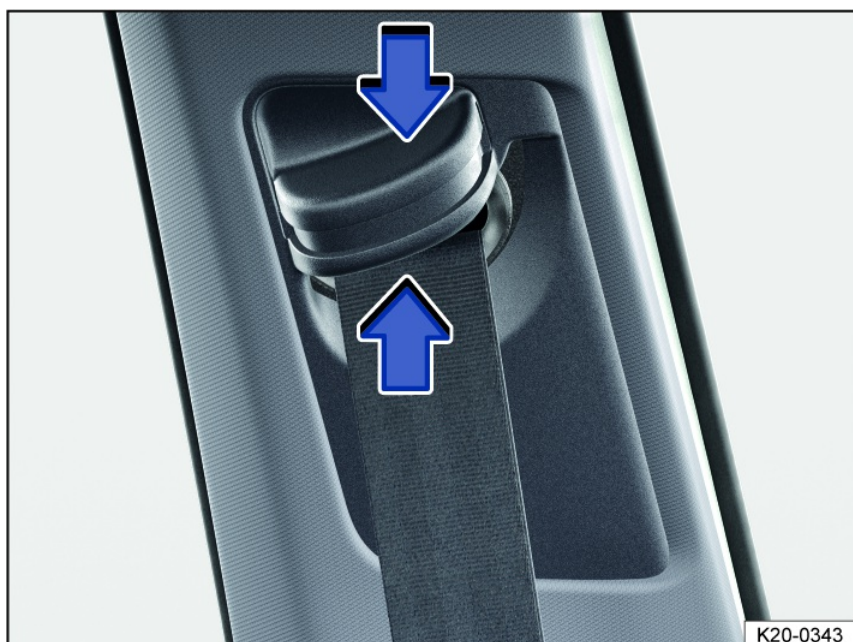
Fig. 34 Next to the front seats: safety belt height adjuster.
