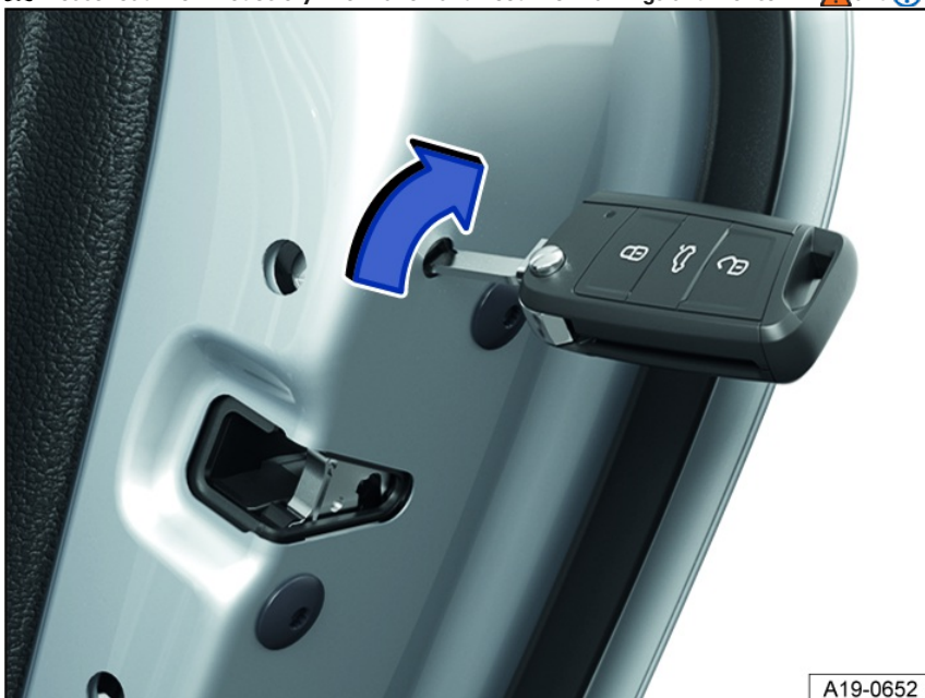
Fig. 62 On the front of the right rear door: emergency locking the vehicle with the vehicle key (general example).
