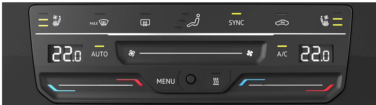
Fig. 112 In the upper section of the center console: air conditioning block for the Climatronic system (version 1).
