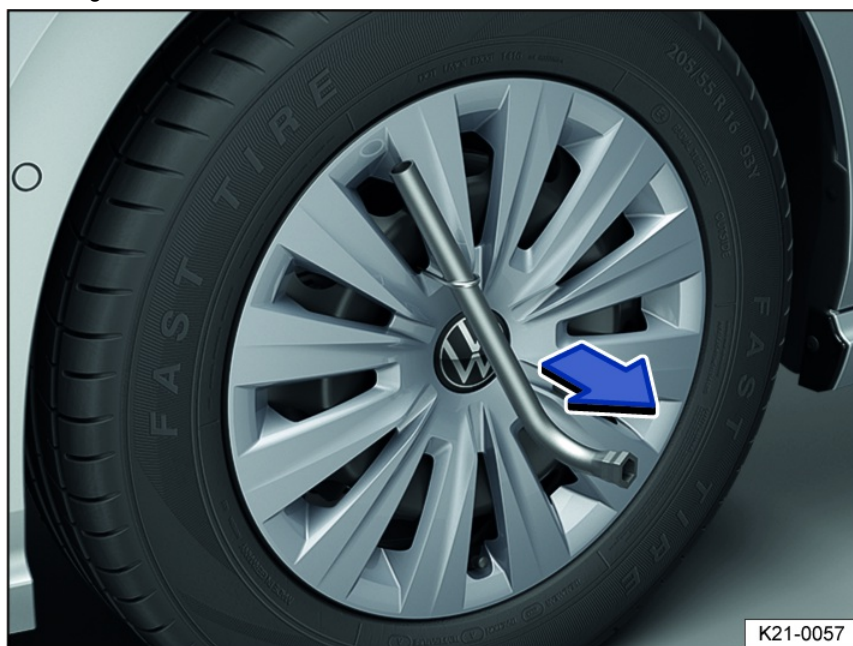
Fig. 216 Remove the wheel hub cover.
