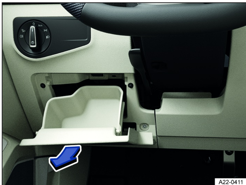
Fig. 188 To the left of the steering wheel: Fuse box cover in the instrument panel (left-hand drive vehicles).
