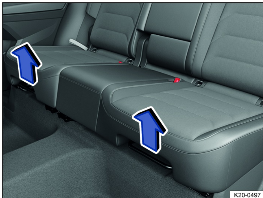
Fig. 82 Under the seat cushion in the rear bench seat: Adjusting lever.
