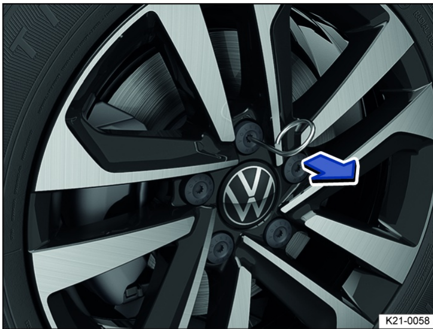
Fig. 217 Remove the caps from the wheel bolts.
