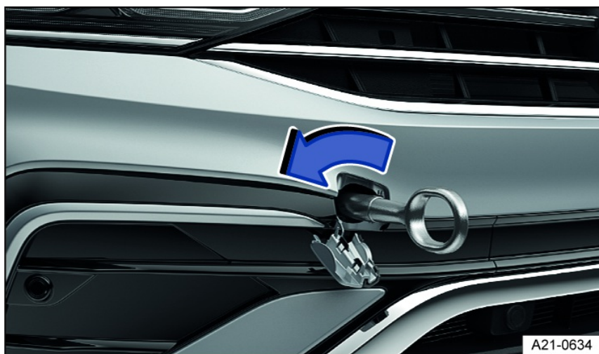
Fig. 196 In the right front bumper: Screw in towing eye.
