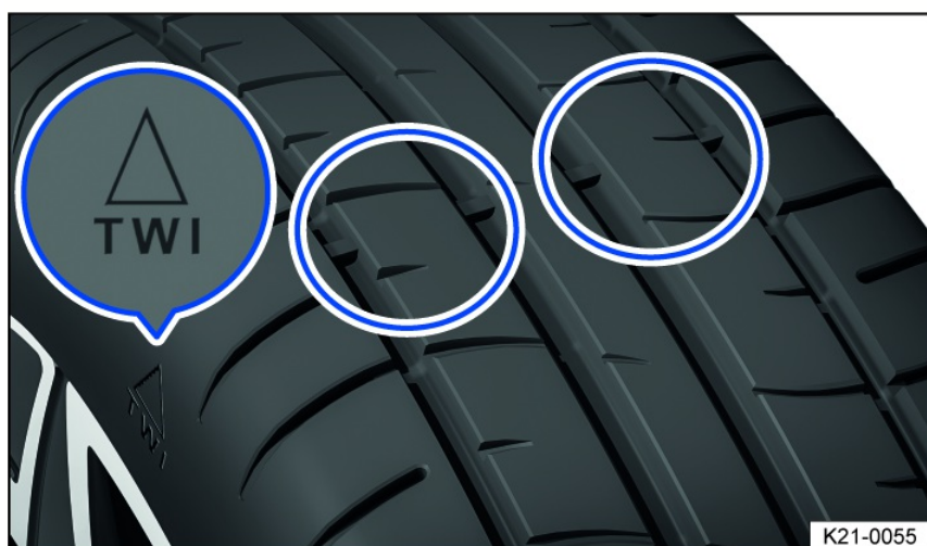
Fig. 212 Tire tread: tread wear indicator.
