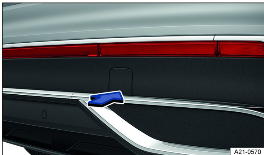
Fig. 197 In the right rear bumper: Remove the cover, variant 1.
