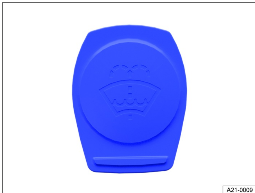
Fig. 203 In the engine compartment: Cap on the washer fluid reservoir (general example).
