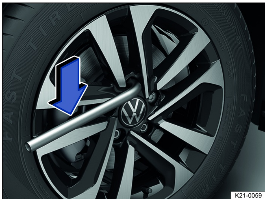
Fig. 218 Changing a tire: loosening the wheel bolts.
