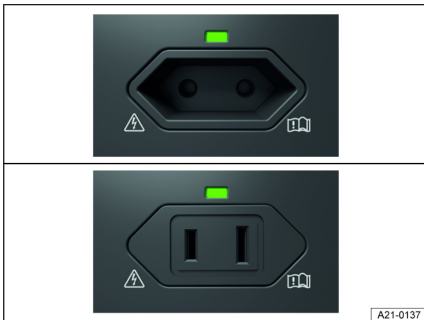
Fig. 163 In the luggage compartment on the left-hand side: 230-volt socket, 115-volt socket, or 100-volt socket.
