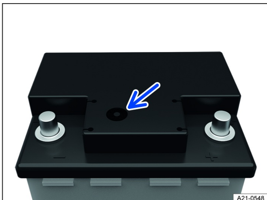
Fig. 209 On the top of the 12 V vehicle battery: Window (general example).
