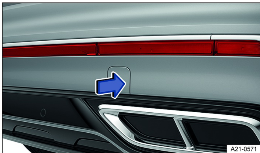
Fig. 198 In the right rear bumper: Remove the cover, variant 2.
