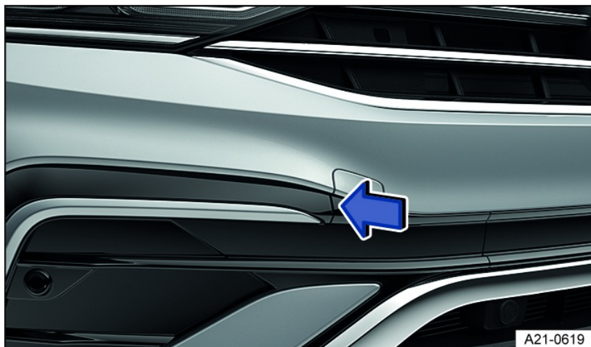
Fig. 195 In the right front bumper: Remove cover.
