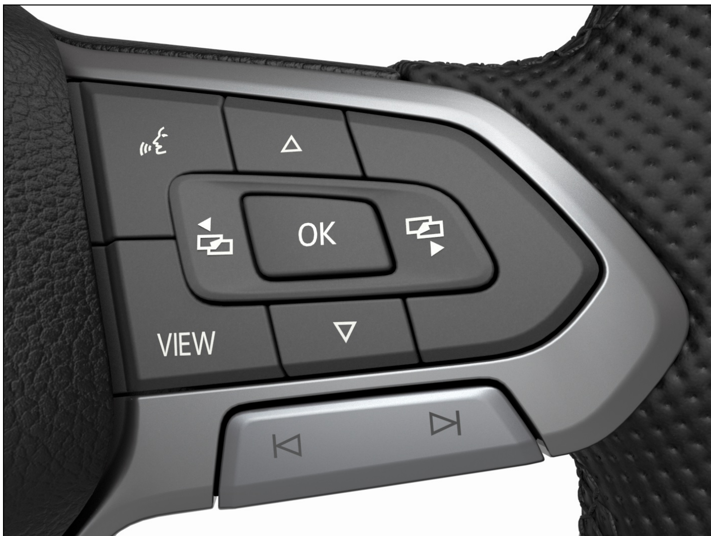
Fig. 18 Right side of the multi-function steering wheel: Operating the analog instrument cluster (variant 1).
