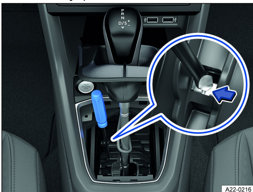
Fig. 123 In the center console: manually release the Automatic Shift Lock (ASL) (variant 1).
