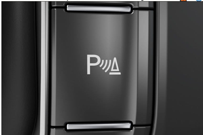
Fig. 149 In the center console: Park Distance Control button.
