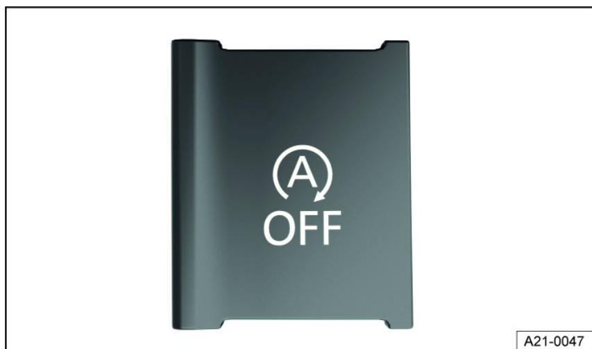
Fig. 120 In the lower section of the center console: Button for the start-stop system.
