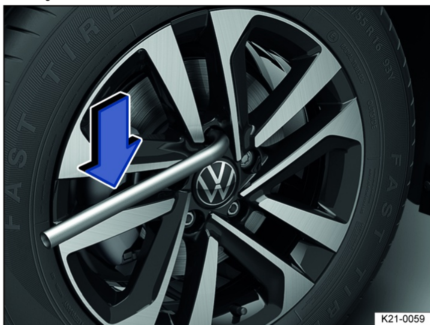
Fig. 222 Wheel change: removing wheel bolts with the lug wrench.
