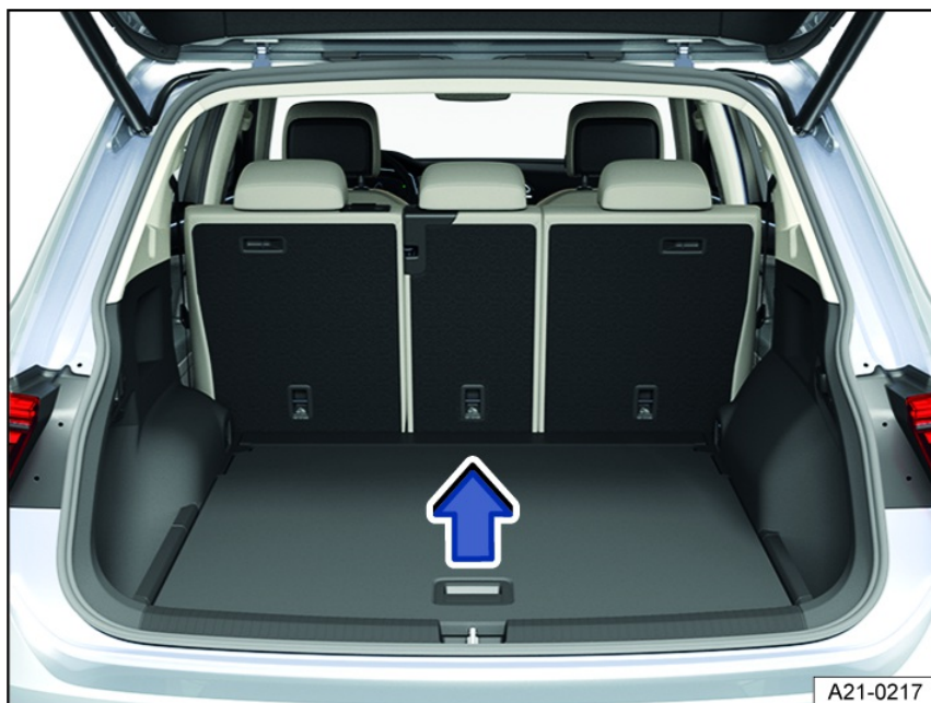
Fig. 170 In the luggage compartment: Lifting up the luggage compartment floor.
