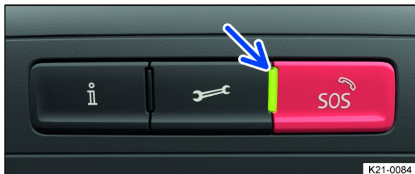
Fig. 50 In the roof console: Controls for call services and indicator light.
