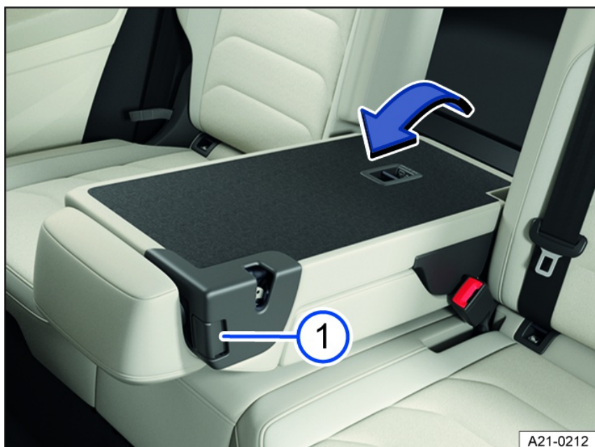
Fig. 175 In the rear seat backrest: Open load-through hatch.
