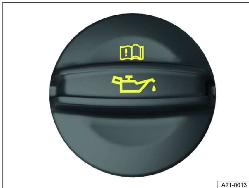
Fig. 204 In the engine compartment: engine oil filler cap (general example).
