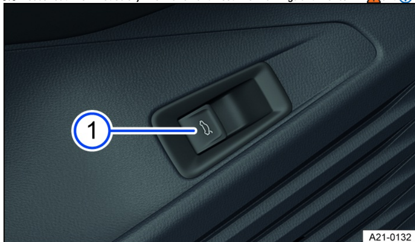
Fig. 66 In the driver's door: unlock button for the trunk lid.
