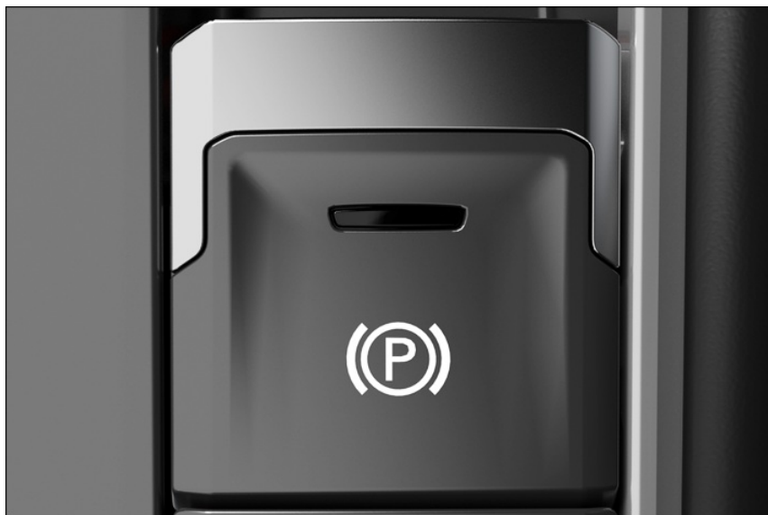
Fig. 147 In the center console: button for the electronic parking brake.
