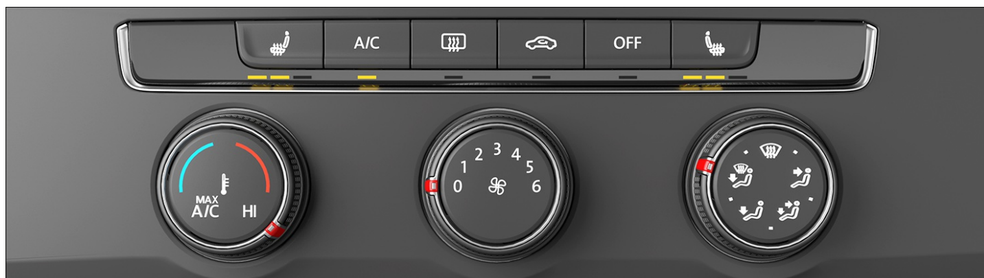
Fig. 114 In the upper section of the center console: Climate control bar for the manual climate control system.
