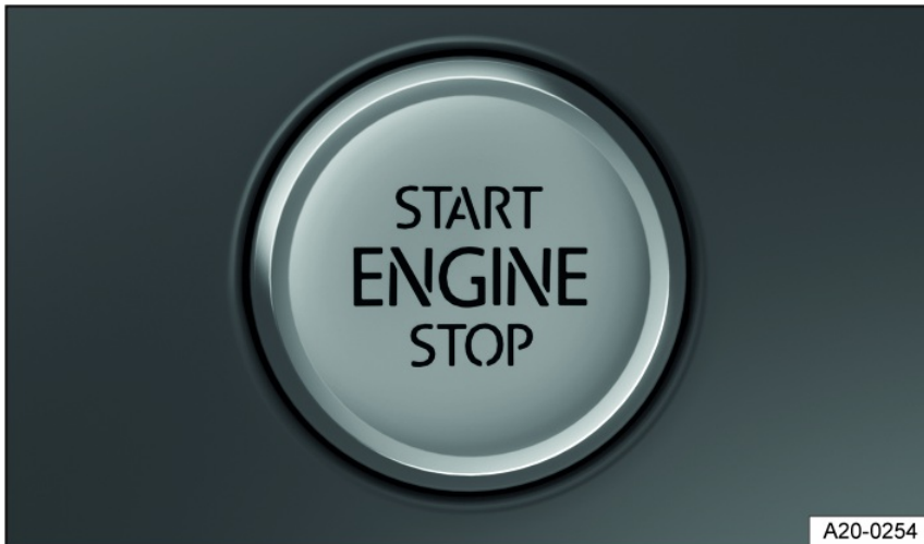
Fig. 118 In the lower area of the center console: starter button for starting the engine.
