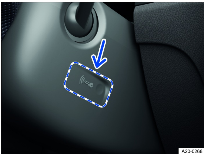
Fig. 119 On the right side of the steering column: emergency start function on vehicles with Keyless Access with push-button start.
