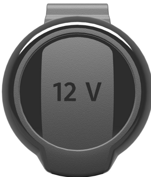
Fig. 162 In the front storage compartment, in the rear center console, or in the luggage compartment on the left side: folding 12-volt socket (general example).
