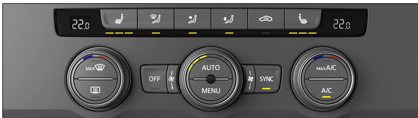
Fig. 113 In the upper section of the center console: air conditioning block for the Climatronic system (version 2).
