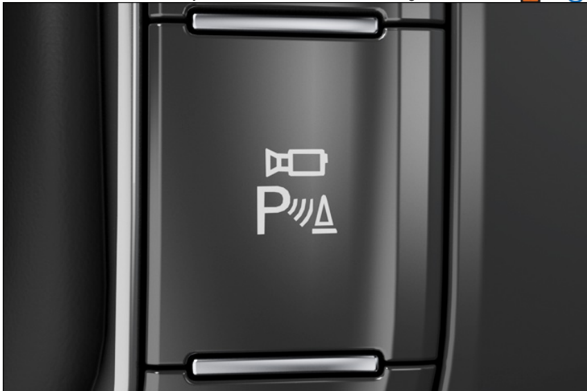
Fig. 153 In the center console: Button for switching the Area View on and off.
