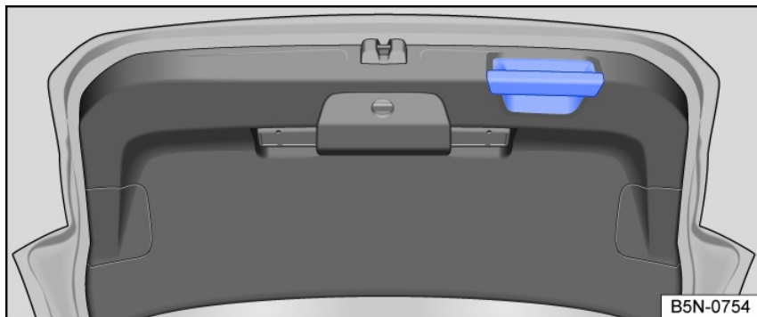
Fig. 62 In the open trunk lid: handle for closing the trunk lid.
