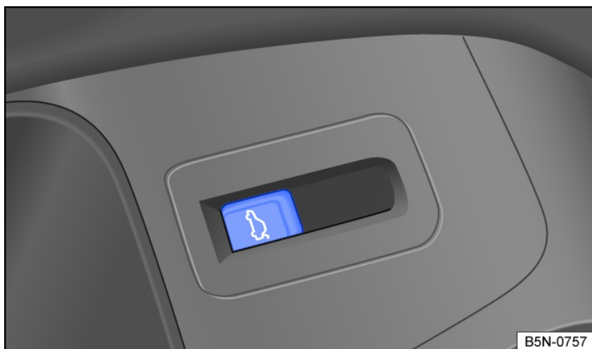
Fig. 57 In the driver door: Button for power opening the trunk lid.
