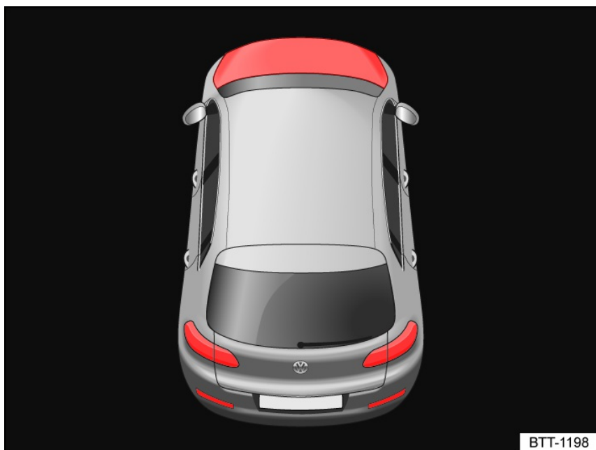
Fig. 195 In the instrument cluster display: the hood is open or not closed correctly (general example).
