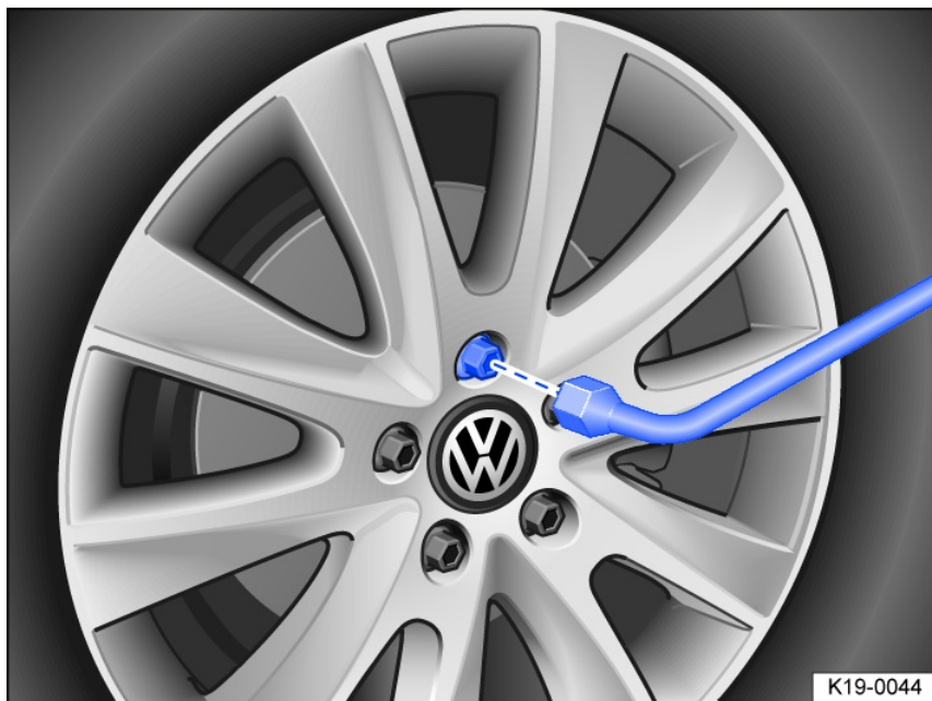
Fig. 218 Wheel change: removing wheel bolts with the lug wrench.
