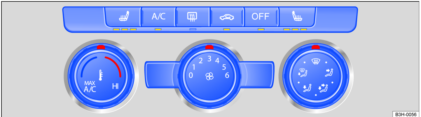
Fig. 104 In the upper section of the center console: Climate control bar for the manual climate control system.
