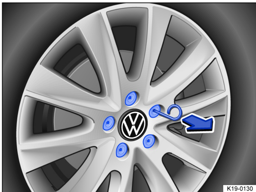
Fig. 210 Remove the caps from the wheel bolts.
