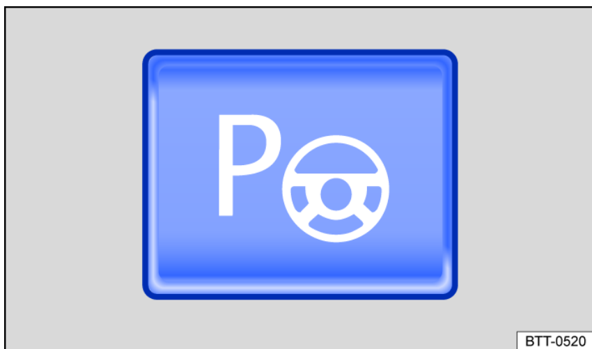
Fig. 141 In the center console: Button to manually switch on Park Assist (general example).
