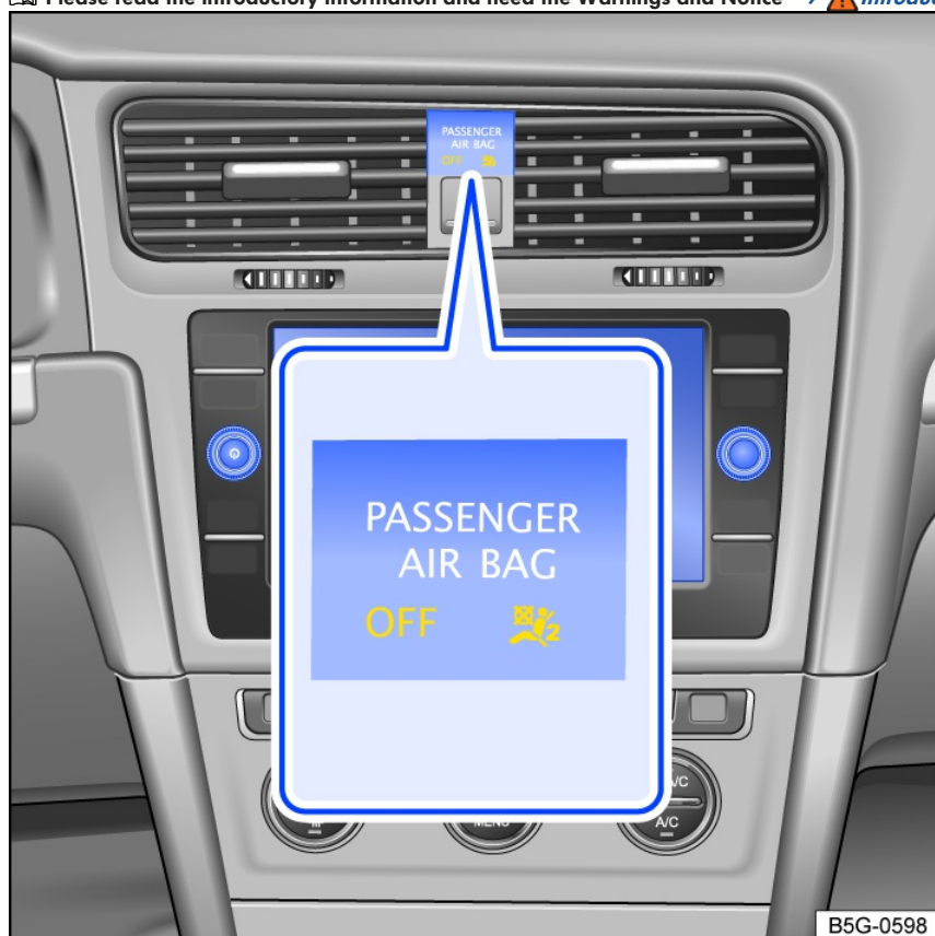
Fig. 33 In the instrument panel: Indicator light for the deactivated front passenger's front airbag.
