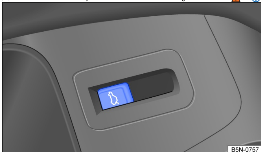
Fig. 63 In the driver's door: unlock button for the trunk lid.
