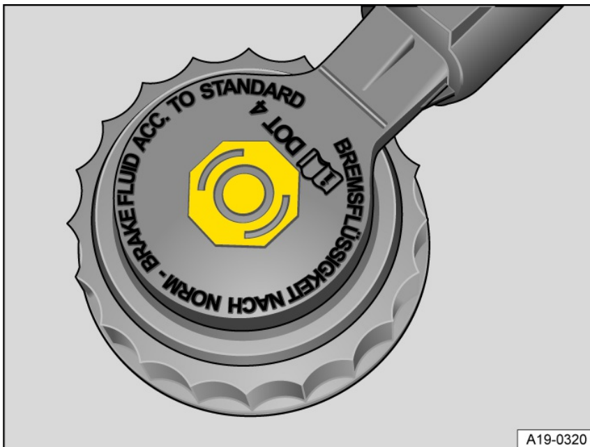
Fig. 201 In the engine compartment: cap on the brake fluid reservoir (version 1).
