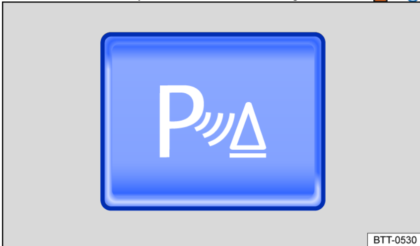
Fig. 136 In the center console: button for switching the PDC on or off (general example).
