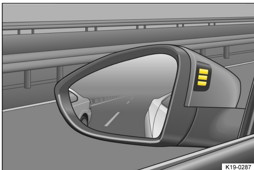
Fig. 133 In the exterior mirror housings: visual lane change system displays.
