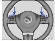
Fig. 141 Steering wheel with Tiptronic shift paddles (if equipped).
