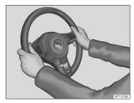
Fig. 50 Steering wheel: 9 o'clock and 3 o'clock positions.
