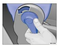
Fig. 56 Unlocking the foldable front passenger backrest.
