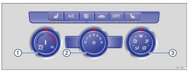
Fig. 157 In the center console: Manual air conditioning controls.
