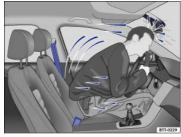
Fig. 60 The unbelted driver is thrown forward.
