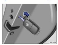
Fig. 183 On the front side of the right rear door: Locking the vehicle with the key bit in the vehicle key.
