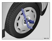
Fig. 193 Pulling the wheel cover off.
