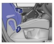
Fig. 55 Folding the front passenger backrest forward.
