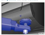
Fig. 178 Front lift point for workshop hoist or floor jack.
