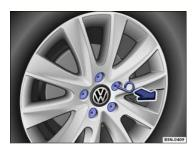
Fig. 192 Pulling cover caps off wheel bolts.
