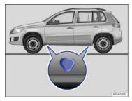
Fig. 195 Lift points for the jack.
