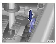
Fig. 186 Releasing the selector lever lock.
