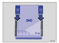
Fig. 200 In the engine compartment: Fuse box cover.
