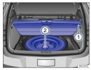
Fig. 114 In the luggage compartment: Handwheel holding the compact spare wheel in place.
