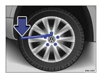
Fig. 194 Changing a wheel: Loosening the wheel bolts.
