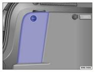
Fig. 127 On the left in the luggage compartment: Side storage compartment.
