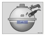
Fig. 171 Coolant expansion tank in the engine compartment.
