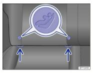
Fig. 80 Markings for the LATCH/UCRA lower universal anchorages on the seat.
