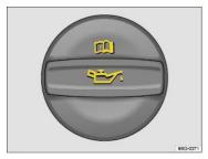
Fig. 169 In the engine compartment: Engine oil filler cap (cap design may vary depending on vehicle equipment).
