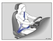
Fig. 66 Proper safety belt positioning for expectant mothers.
