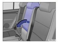
Fig. 102 In the rear seat backrest: Opening the luggage compartment pass-through.
