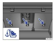
Fig. 82 Anchorages for the top tether strap on the back of the rear seat.
