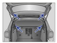
Fig. 101 Installing and removing the luggage compartment cover.
