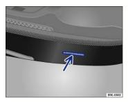
Fig. 20 Vehicle identification number (VIN).
