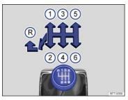
Fig. 138 Gearshift pattern of a 6-speed manual transmission.
