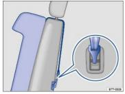
Fig. 81 Example of a mounted upper tether strap: The top tether strap reduces the forward movement of the child restraint in a crash, to help reduce the risk of head injury if the child hits the vehicle interior.
