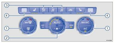
Fig. 158 In the center console: Climatronic controls.
