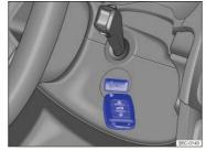
Fig. 135 Hold the remote control vehicle key to the right of the steering column: Emergency starting feature.
