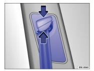
Fig. 67 Next to the front seats: Safety belt height adjuster.
