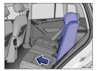
Fig. 98 Folding the backrest forward and back.
