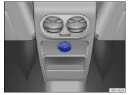
Fig. 132 In the rear center console: 12 Volt socket.
