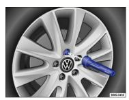
Fig. 197 Changing a wheel: Remove previously loosened wheel bolts using the screwdriver handle.
