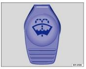
Fig. 94 In the engine compartment: Cap of the windshield washer fluid reservoir.
