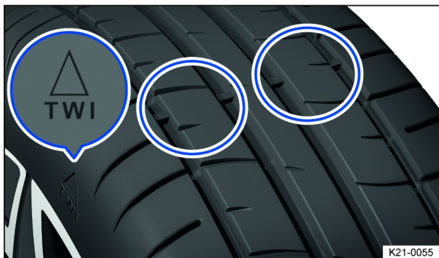
Fig. 150 Tire tread: tread wear indicator.
