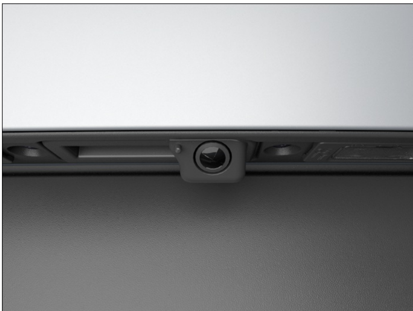
Fig. 163 In the rear of the vehicle: Rear View Camera system on the handle (general example).
