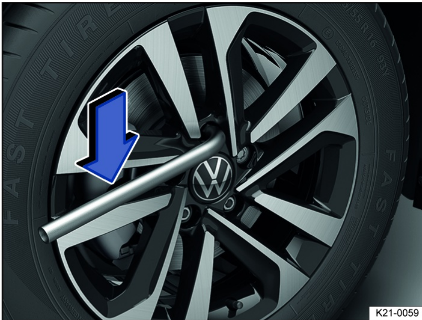
Fig. 155 Changing a tire: loosening the wheel bolts.
