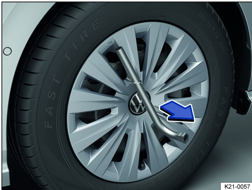
Fig. 153 Remove the wheel hub cover.
