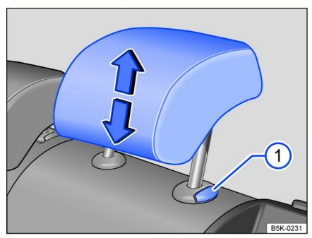
Fig. 68 Rear head restraint: adjusting.
