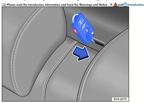
Fig. 53 Behind the rear seat backrest: mechanically unlocking the rear seat backrest using the emergency release.
