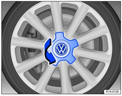
Fig. 170 Twist off the hubcap.
