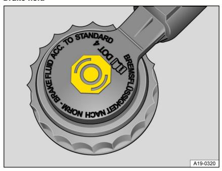
Fig. 160 In the engine compartment: cap on the brake fluid reservoir (version 1).
