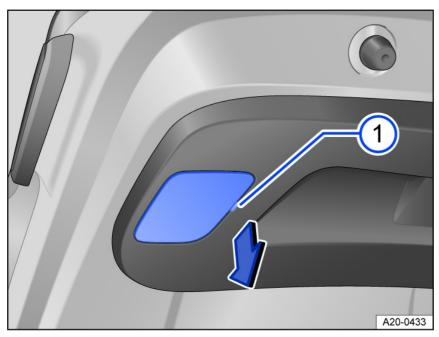
Fig. 133 In the trunk lid: Remove the cover on the taillight.
