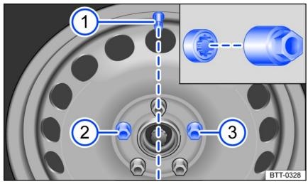
Fig. 174 Changing a tire: tire valve (1) and locations of the anti-theft wheel bolt (2) or (3).
