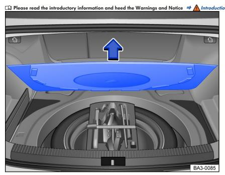
Fig. 127 In the luggage compartment under the luggage compartment floor: tool box.
