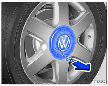
Fig. 169 Remove the wheel center trim.
