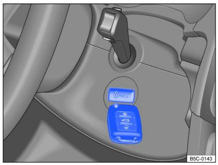
Fig. 91 On the right side of the steering column: emergency start function on vehicles with Keyless Access with push-button start.
