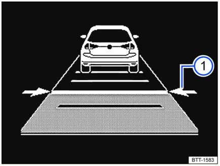
Fig. 103 In the instrument cluster display: set distance (1) (schematic diagram, ACC is regulating).
