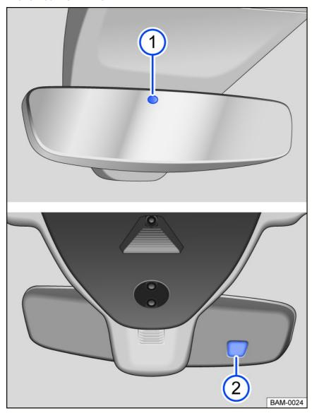
Fig. 80 On the windshield: automatic dimming interior rearview mirror.
