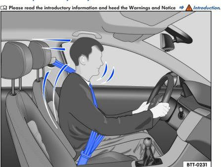
Fig. 21 Driver that is restrained during a braking maneuver by a safety belt that is fastened correctly.
