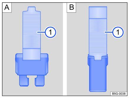
Fig. 146 Remove or install a fuse with the plastic pliers (general example).
