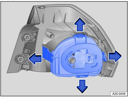
Fig. 141 Taillight: removing the bulb holder.
