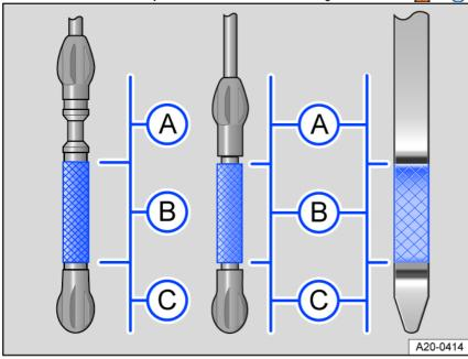
Fig. 156 Engine oil level markings on the oil dipstick (versions).
