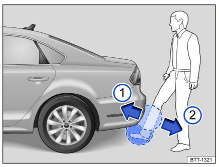
Fig. 52 Trunk lid with sensor-controlled opening (Easy Open).
