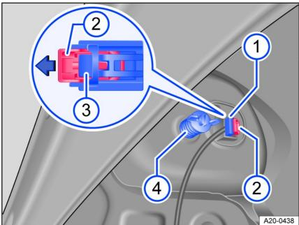
Fig. 140 Side of the luggage compartment: removing the taillight.
