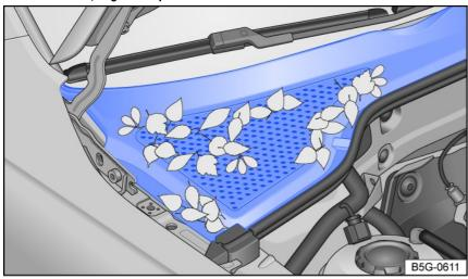
Fig. 180 Between the engine compartment and windshield: plenum chamber (general example).
