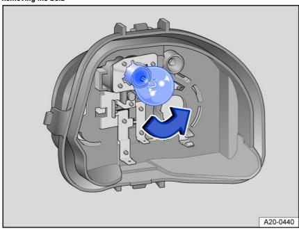
Fig. 142 Taillight: Removing the bulbs.
