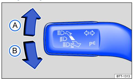
Fig. 74 On the left side of the steering column: turn signal and high beam lever.
