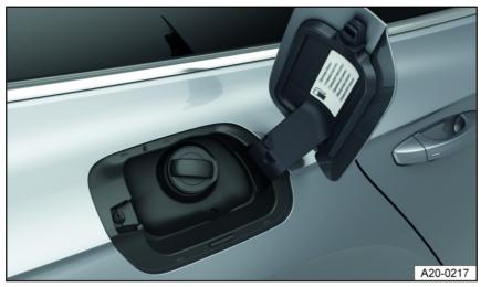
Fig. 126 Behind the fuel filler flap: fuel tank cap (general example)
