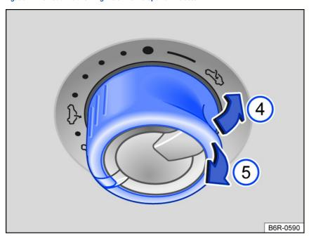
Fig. 56 In the headliner: pushing the switch to raise and pulling the switch to close.
