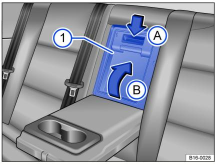
Fig. 124 In the rear seat backrest: Open load-through hatch.
