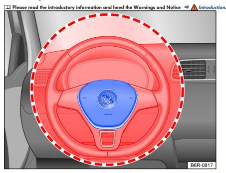
Fig. 28 Installation location and deployment zone of the driver's front airbag.
