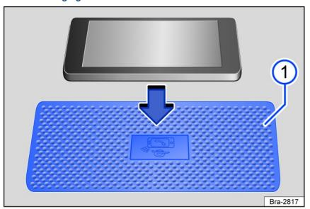
Fig. 121 Diagram: storage compartment with a liner pad for wireless charging. The symbol on the liner mat may look different in some vehicles.
