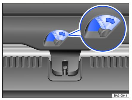
Fig. 54 In the luggage compartment: unlocking the trunk lid.
