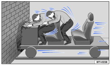
Fig. 18 A vehicle with occupants who are not wearing safety belts collides with a wall.
