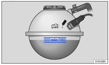
Fig. 159 In the engine compartment: markings on the engine coolant expansion tank.
