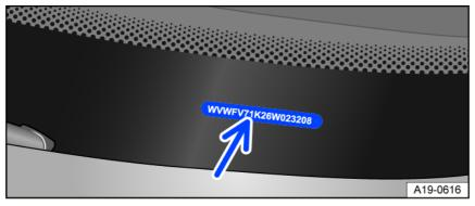
Fig. 182 In the windshield: vehicle identification number (VIN)
