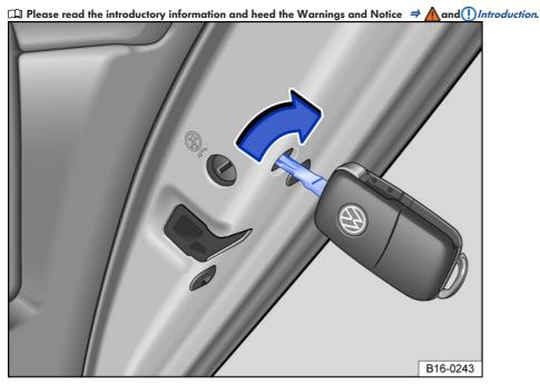
Fig. 48 On the front of the right rear door: manually locking the vehicle with the vehicle key.
