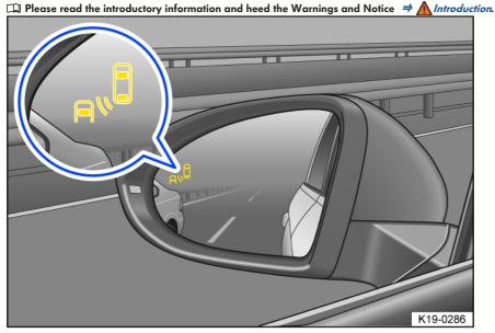
Fig. 106 In the outside mirrors: Blind Spot Monitor indicator.
