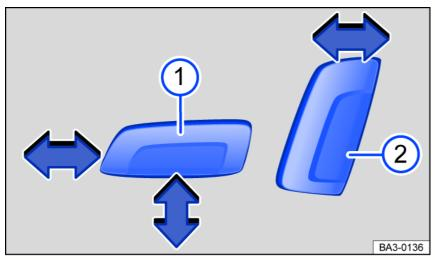
Fig. 64 Switch on the left front seat: adjusting the front seat forward/back, the height and angle of the seat surface, and the front seat backrest.
