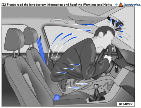
Fig. 19 A driver not wearing a safety belt is propelled forward.
