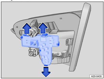
Fig. 135 Taillight: removing the bulb holder.
