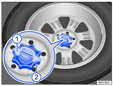
Fig. 175 In the luggage compartment: handle to secure the compact spare wheel.
