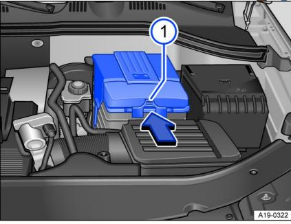
Fig. 162 In the engine compartment: Remove the plastic cover for the 12 V vehicle battery.
