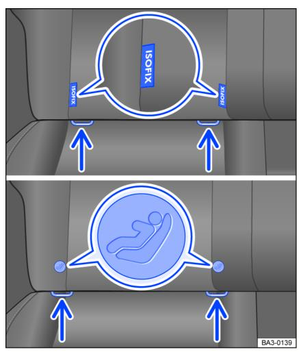
Fig. 34 On the vehicle seat: label for child restraint LATCH/UAS anchor points.
