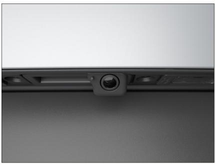
Fig. 181 In the rear of the vehicle: Rear View Camera system on the handle (general example).
