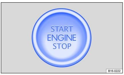
Fig. 89 In the lower area of the center console: starter button for starting the engine.
