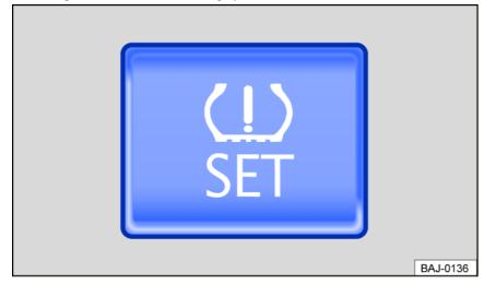
Fig. 164 In the glove box on the front passenger side: button for Tire Pressure Monitoring System.
