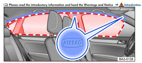
Fig. 32 On the left side of the vehicle: installation location and deployment zone of the Side Curtain Protection®.
