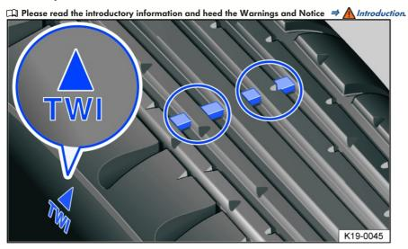
Fig. 167 Tire tread: tread wear indicator.
