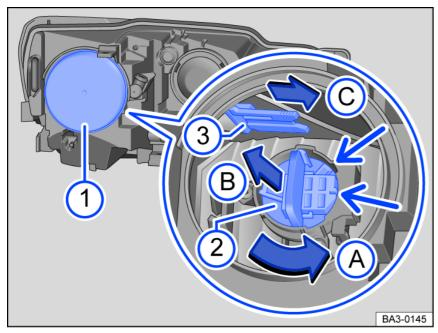
Fig. 137 In the engine compartment: Rear view of the left-side headlight.
