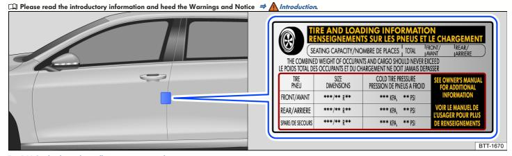
Fig. 166 On the driver door pillar: tire pressure sticker
