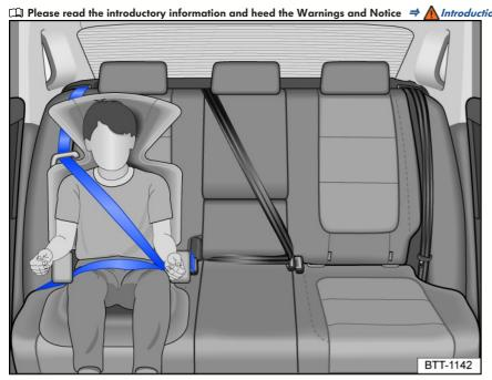
Fig. 38 Correctly secured child on a booster seat.
