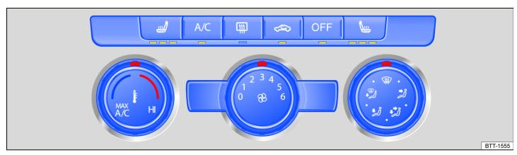
Fig. 84 In the upper section of the center console: Climate control bar for the manual climate control system.
