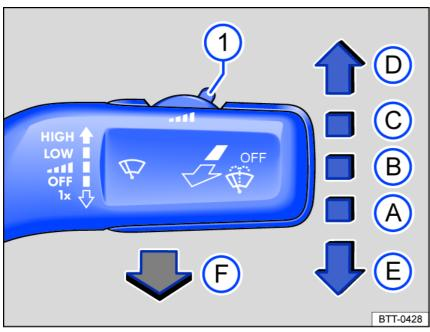
Fig. 78 On the right side of the steering column: operating the windshield wipers.
