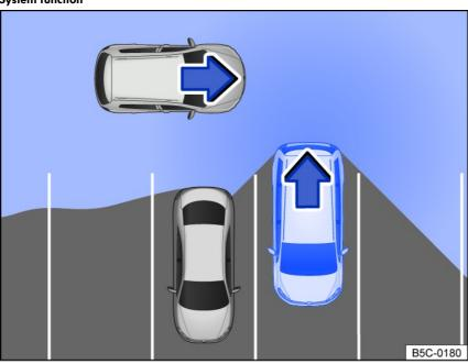
Fig. 114 Rear Traffic Alert, general example: monitored area around the vehicle that is exiting a parking space.
