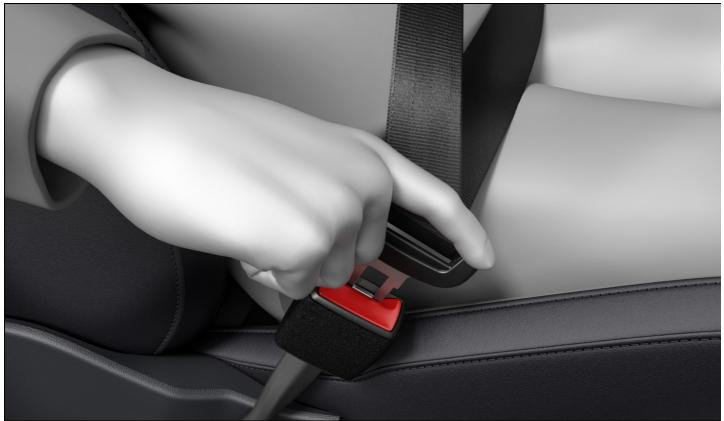
Fig. 22 Inserting the buckle tongue into the safety belt buckle.
