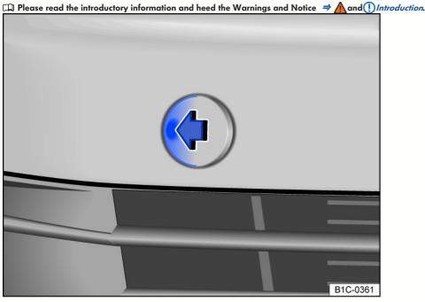
Fig. 148 In the right front bumper: Remove cover.
