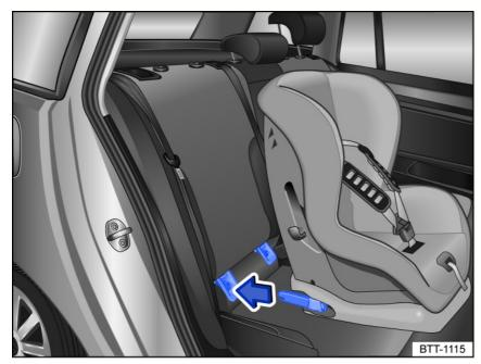
Fig. 35 General example: fitting a child restraint with attachment arms.
