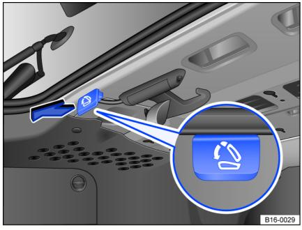
Fig. 66 In the luggage compartment: Remote release lever.
