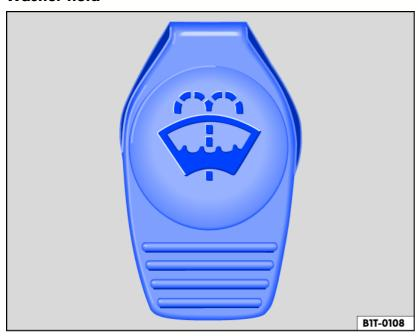
Fig. 155 In the engine compartment: cap on the washer fluid reservoir.
