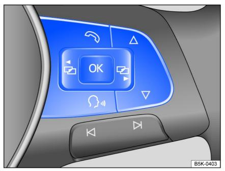
Fig. 14 Right side of the multi-function steering wheel: buttons for operating the menus and information displays in the instrument cluster
