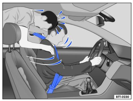
Fig. 20 A passenger in the rear seat who is not wearing a safety belt will be propelled forward toward the driver who has their own safety belt fastened.
