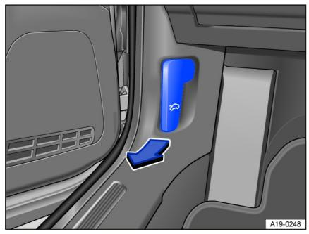
Fig. 150 In the driver's side footwell: Release lever for the hood (general example).
