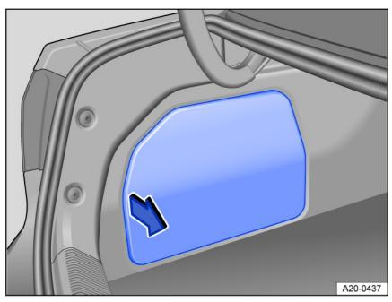
Fig. 139 In the side of the luggage compartment: Opening the cover of the rear side trim panel.
