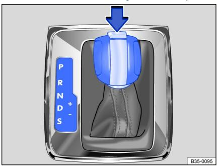
Fig. 92 Left-hand drive: selector lever with lock button (arrow) on an automatic transmission.
