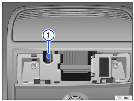
Fig. 59 Hexagon socket head bolt for closing the power sunroof.
