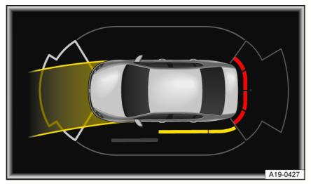
Fig. 108 Infotainment system: Park Distance Control with obstacle detection and steering lock (general example).
