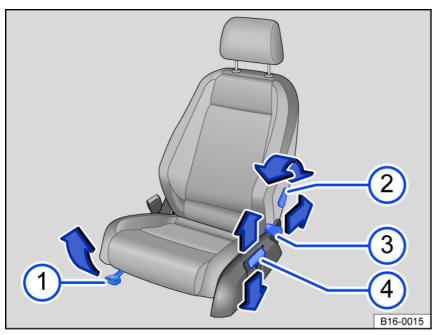
Fig. 62 On the left front seat: Controls (Version 1).
