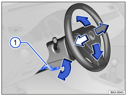
Fig. 60 Under the steering wheel in the steering column trim panel: lever to adjust the steering wheel position manually.
