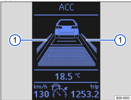
Fig. 104 In the instrument cluster display: Lane Assist indicators.
