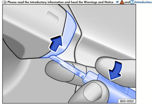
Fig. 47 Driver's door handle: prying off the cap.
