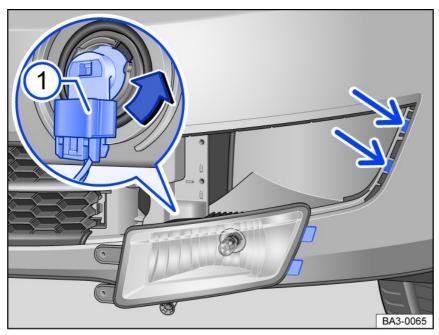
Fig. 132 Replacing the bulb in the headlight.
