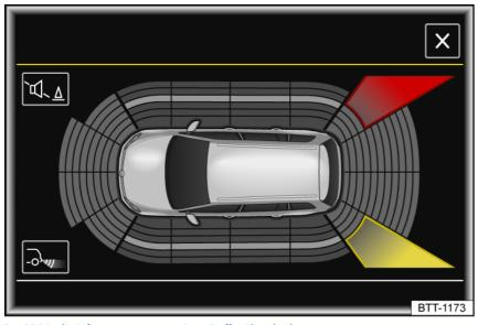
Fig. 115 In the Infotainment system: Rear Traffic Alert display.
