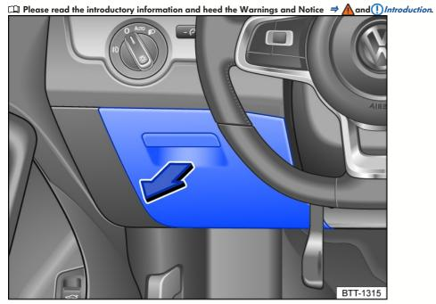
Fig. 144 On the driver side in the instrument panel: fuse box cover.
