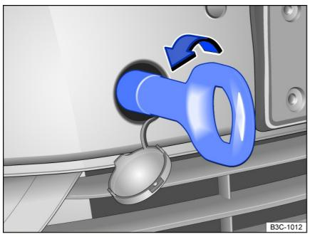
Fig. 149 In the right front bumper: Screw in towing eye.
