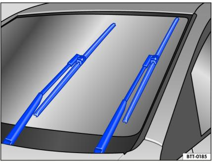
Fig. 129 Wipers in service position.
