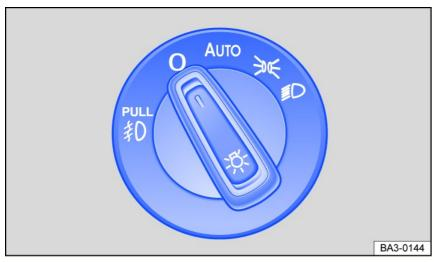
Fig. 75 Next to the steering wheel: light switch (one version).
