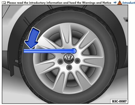
Fig. 173 Changing a tire: loosening the wheel bolts.
