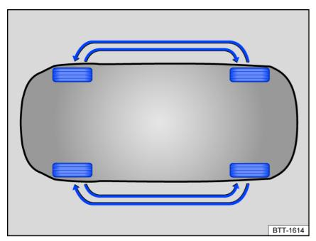
Fig. 165 General example: Diagram for rotating the wheels.
