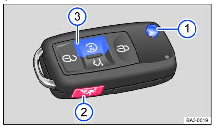
Fig. 41 Vehicle key with remote start relay function.
