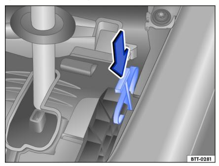
Fig. 96 Manually release the selector lever lock.
