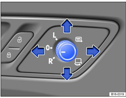
Fig. 82 In the driver door: knob for the outside mirrors.
