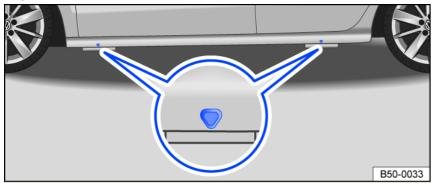
Fig. 176 Mounting points for the vehicle jack.
