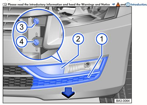
Fig. 131 In the front bumper on the left: replacing the headlight.
