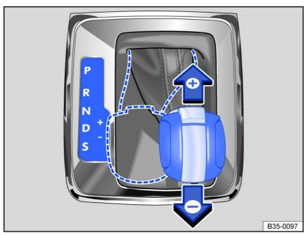
Fig. 93 Selector lever in Tiptronic position.
