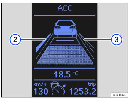
Fig. 105 In the instrument cluster display: Lane Assist indicators.
