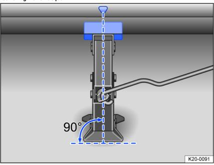
Fig. 177 Correct jack setup.
