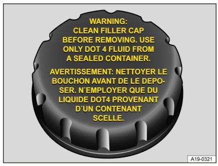
Fig. 161 In the engine compartment: cap on the brake fluid reservoir (version 2).
