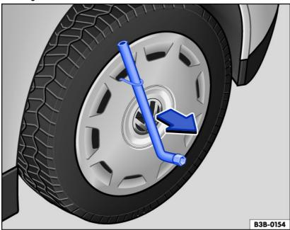
Fig. 171 Remove the full wheel cover.
