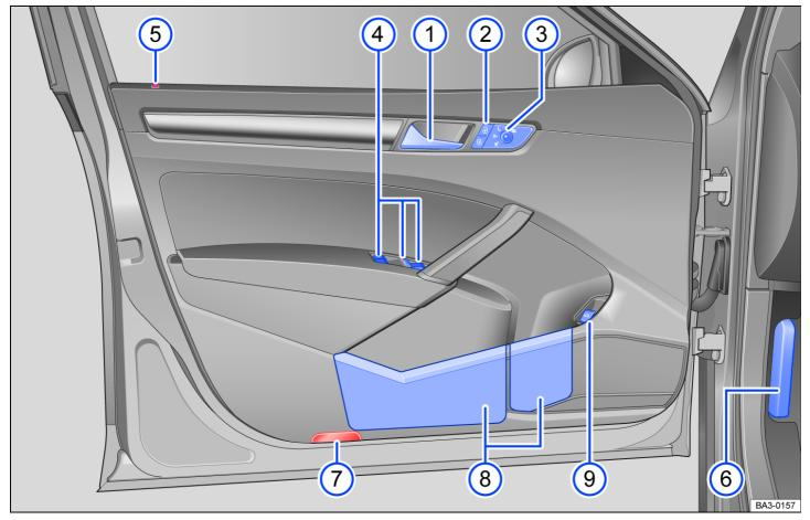
Fig. 6 Driver door (left-hand drive vehicle): controls (right-hand drive vehicles are a mirror image).
