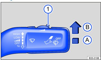
Fig. 79 On the right side of the steering column: windshield wiper lever.
