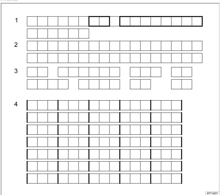
Fig. 1 Vehicle data label. 1: VIN; 2: Vehicle model, engine output, transmission; 3: Engine code, transmission code, paint number, interior equipment; 4: Optional equipment, PR numbers.
