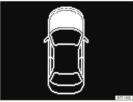
Fig. 154 In the instrument cluster display: the hood is open or not closed correctly (general example).
