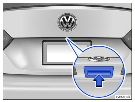
Fig. 51 In the trunk lid: button to open the trunk lid.
