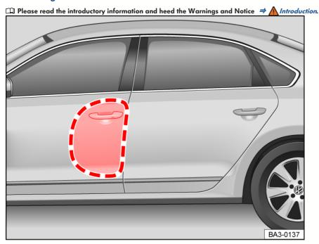
Fig. 30 In the vehicle interior on the left-hand side: Side airbag deployment zone.
