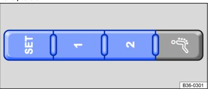
Fig. 73 On the outer side of the driver's seat: memory buttons.
