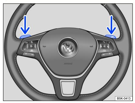
Fig. 94 Steering wheel with shift paddles for Tiptronic.
