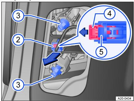
Fig. 134 In the trunk lid: Remove the taillight.
