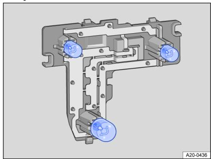
Fig. 136 Taillight: Removing the bulbs.
