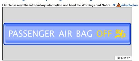
Fig. 27 In the instrument panel: Indicator light for the deactivated front passenger's front airbag.
