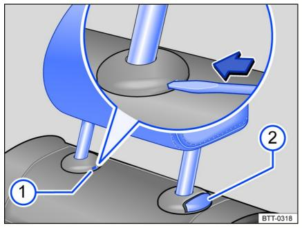
Fig. 70 Rear head restraint: removing.
