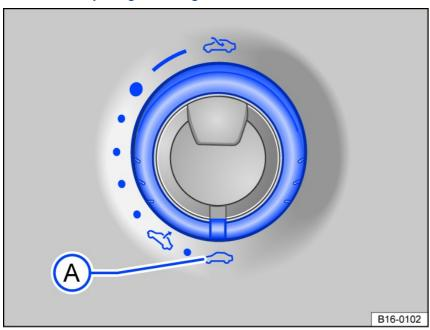
Fig. 57 In the headliner: switch for the power sunroof.
