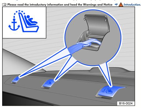
Fig. 36 In the storage compartment behind the rear bench seat: Anchorages for the upper strap.
