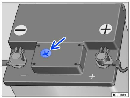
Fig. 163 Window on the top of the 12 V vehicle battery (general example).
