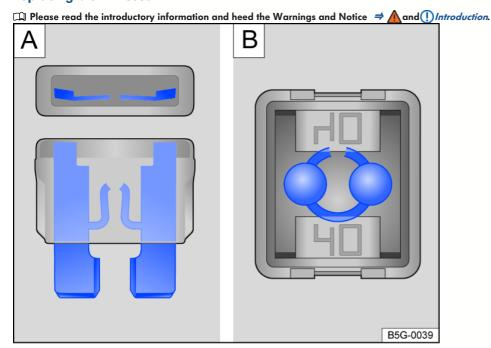
Fig. 145 Blown fuse (general example).
