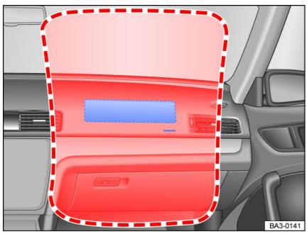
Fig. 29 Installation location and deployment zone of the front passenger's front airbag.
