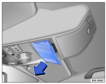
Fig. 58 In the headliner: remove the cover.
