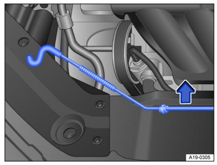
Fig. 152 In the engine compartment: Hood support bracket.
