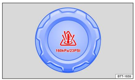
Fig. 158 In the engine compartment: cap on the engine coolant expansion tank.
