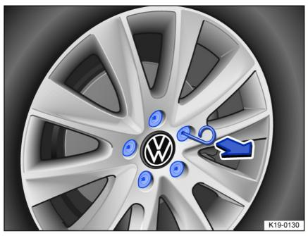
Fig. 172 Remove the caps from the wheel bolts.
