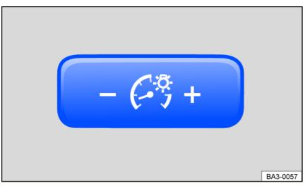
Fig. 77 Next to the steering wheel: control for instrument and switch lighting.
