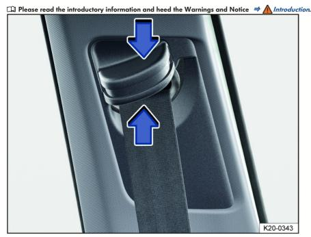
Fig. 26 Next to the front seats: safety belt height adjuster.
