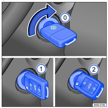
Fig. 88 Positioning the vehicle key in the ignition switch.
