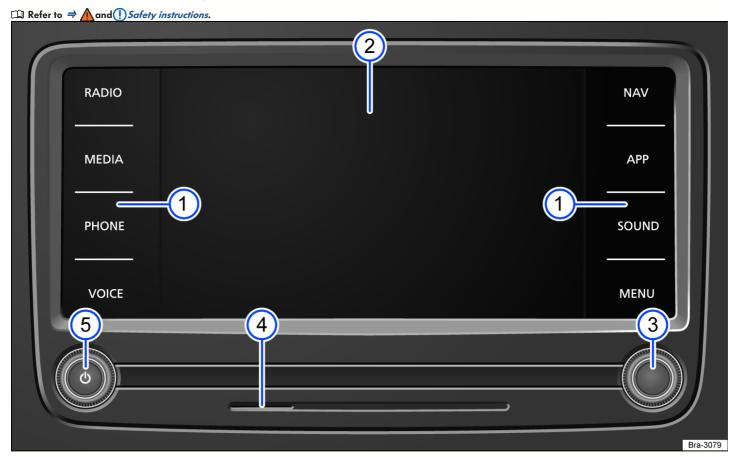
Fig. 118 Overview of the controls (6.33 inches).
