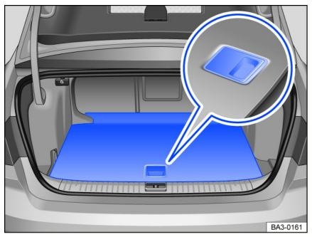
Fig. 122 In the luggage compartment: opening the luggage compartment floor.
