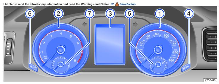
Fig. 11 General example: Analog instrument cluster in the instrument panel.
