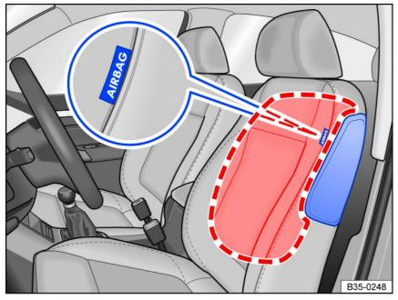
Fig. 31 In the side of the front seat: Side airbag installation location and deployment zone.
