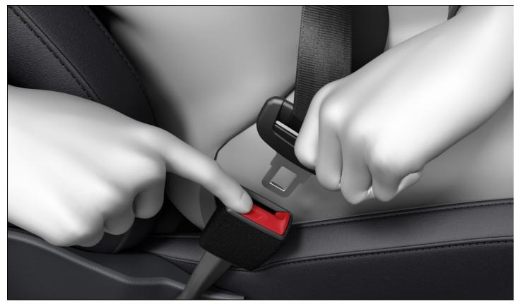
Fig. 23 Releasing the buckle tongue from the safety belt buckle.
