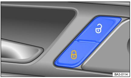
Fig. 46 In the driver's door: central locking button.
