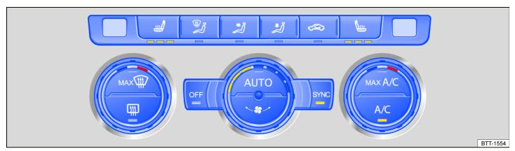
Fig. 85 In the upper section of the center console: Climate control bar for the Climatronic system.
