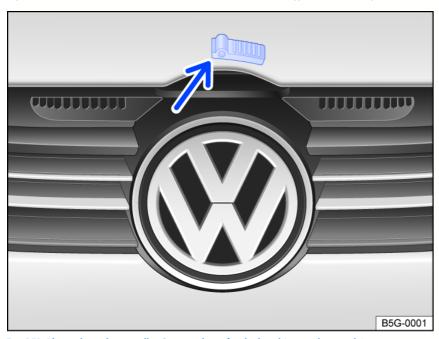
Fig. 151 Above the radiator grille: Opening lever for the hood (general example).
