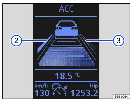
Fig. 106 On the instrument cluster display: Lane Assist display (example two).
