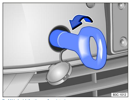
Fig. 146 In the right front bumper: Screw in towing eye.
