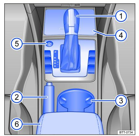
Fig. 9 Overview of the lower section of the center console.
