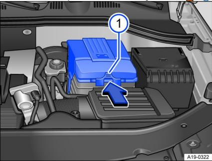
Fig. 159 In the engine compartment: Remove the plastic cover for the  $12\ V$  vehicle battery.
