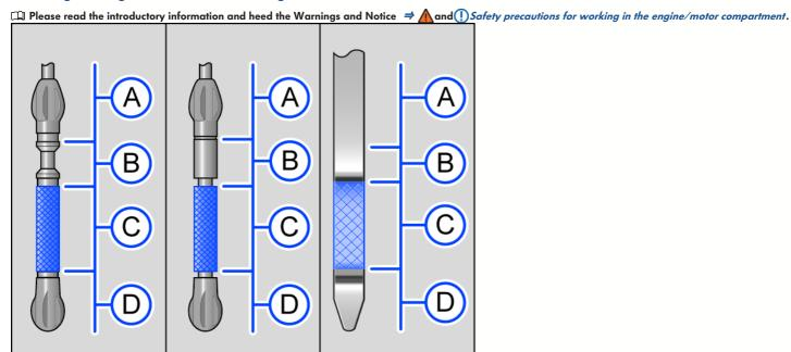
Fig. 153 Engine oil level markings on the oil dipstick (versions).
