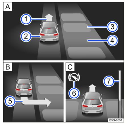
Fig. 112 In the instrument cluster display: parking perpendicular to the road.
