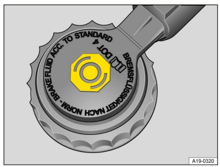
Fig. 157 In the engine compartment: cap on the brake fluid reservoir variant A.
