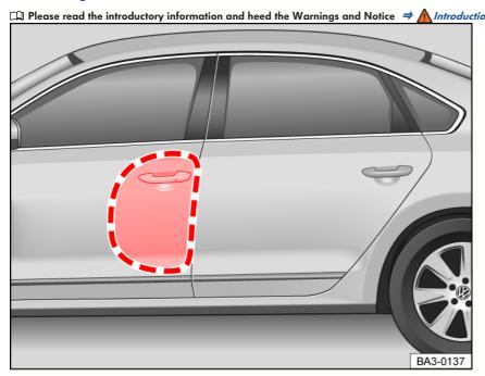
Fig. 32 On the left side of the vehicle: Side airbag deployment zones.
