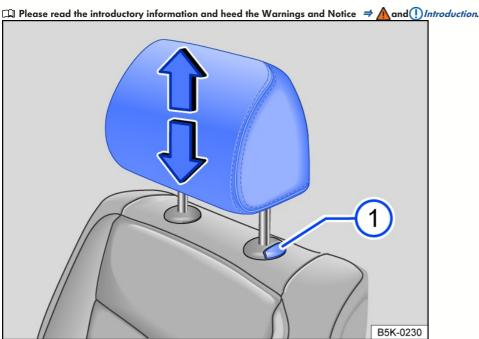
Fig. 70 Front head restraint: adjusting.
