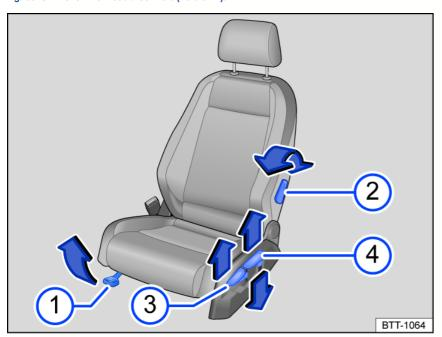
Fig. 66 On the left front seat: Controls (version 2).
