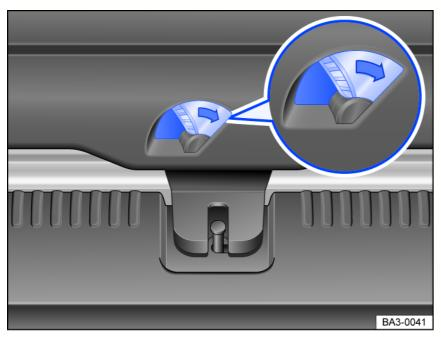
Fig. 57 In the luggage compartment: unlocking the trunk lid.
