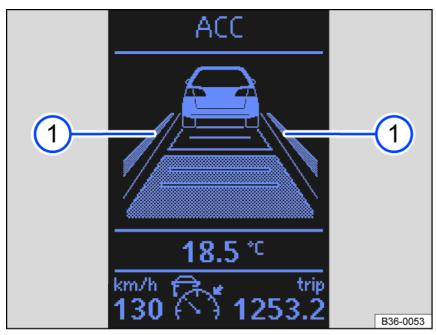
Fig. 105 On the instrument cluster display: Lane Assist display (example one).
