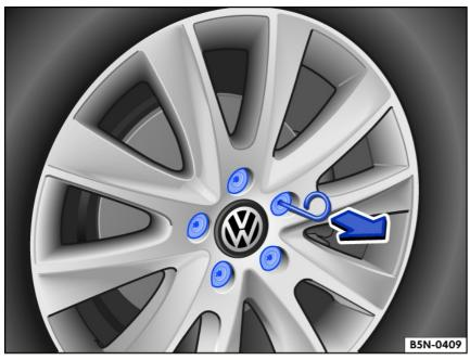
Fig. 170 Remove the caps from the wheel bolts.
