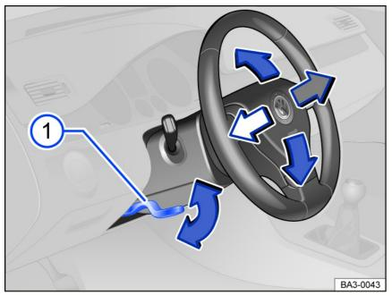
Fig. 63 Under the steering wheel in the steering column trim panel: lever to adjust the steering wheel position manually.
