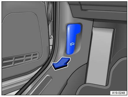
Fig. 147 In the driver's side footwell: Release lever for the hood (general example).
