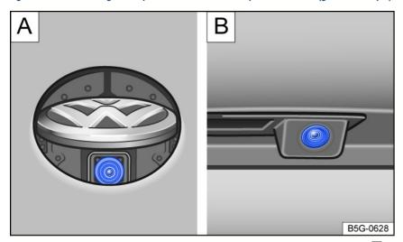
Fig. 178 In the rear of the vehicle: Rear View Camera system in the Volkswagen emblem 🛕 or on the handle 🖪 (schematic diagram).
