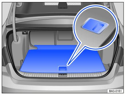
Fig. 123 In the trunk: opening the trunk floor panel.
