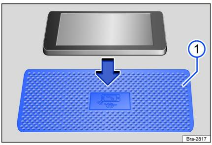
Fig. 122 Diagram: storage compartment with a liner pad for wireless charging.
