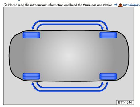
Fig. 163 General example: diagram for rotating tires
