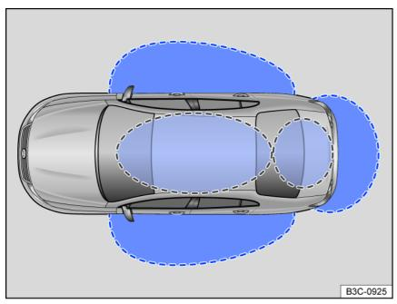
Fig. 46 Keyless Access: sensor range.
