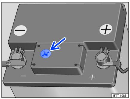
Fig. 161 Window on the top of the 12 V vehicle battery (general example).
