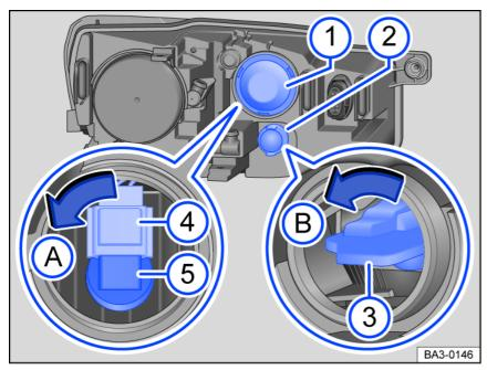
Fig. 133 In the engine compartment: Rear view of the left headlight.
