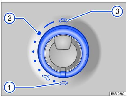
Fig. 58 In the headliner: turning the switch to open and close.
