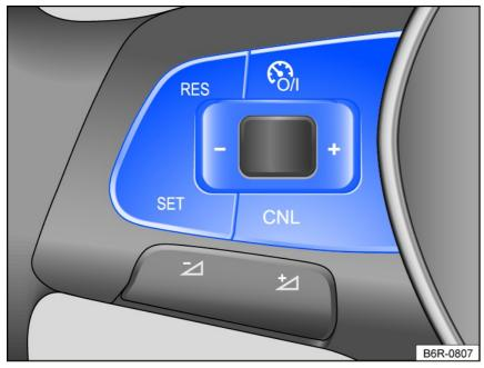
Fig. 100 Left side of the multifunction steering wheel: buttons for cruise control system operation.
