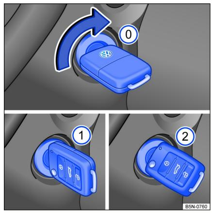
Fig. 91 Positioning the vehicle key in the ignition switch.
