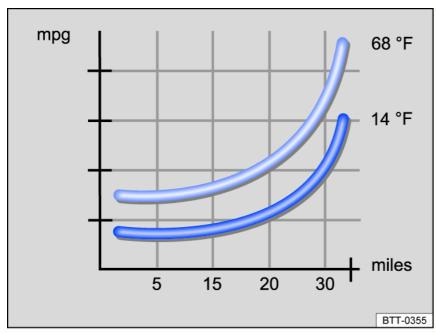
Fig. 90 Fuel consumption in mpg at two different ambient temperatures.
