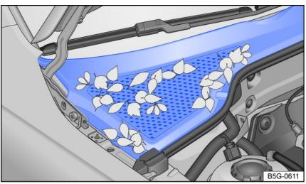
Fig. 177 Between the engine compartment and windshield: plenum chamber (general example).
