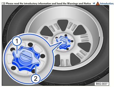
Fig. 173 In the luggage compartment: handle to secure the compact spare wheel.
