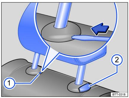
Fig. 73 Rear head restraint: removing.
