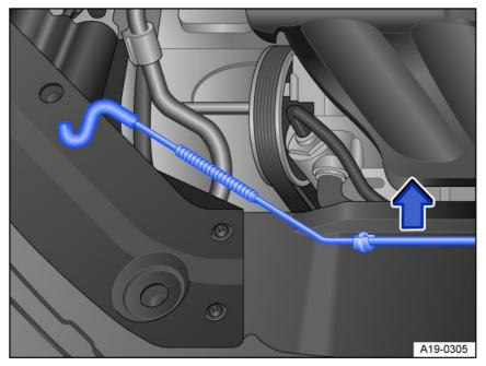
Fig. 149 In the engine compartment: Hood support bracket.
