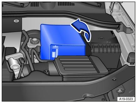
Fig. 160 In the engine compartment: Open the sleeve on the 12 V vehicle battery.
