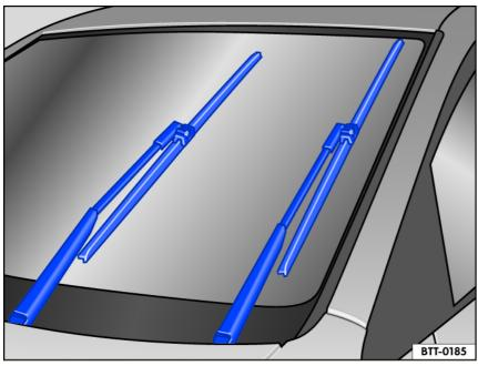
Fig. 130 Wipers in service position.
