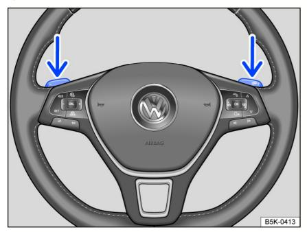
Fig. 97 Steering wheel with shift paddle for tiptronic.
