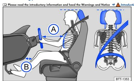
Fig. 17 General example: correct distance between the driver and steering wheel, correct safety belt routing, and correct head restraint adjustment.
