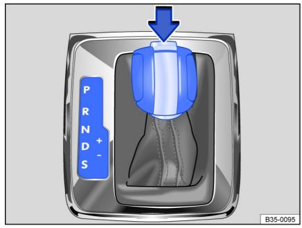
Fig. 95 Left-hand drive: selector lever with lock button (arrow) on an automatic transmission.
