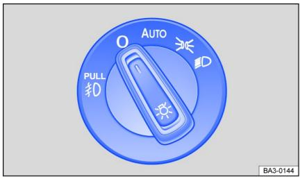
Fig. 78 Next to the steering wheel: light switch (one version).
