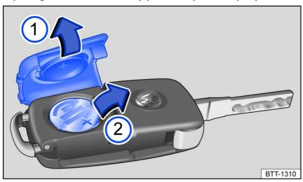
Fig. 45 Vehicle key: replacing the button cell battery
