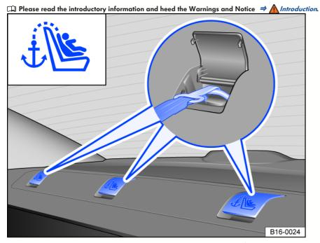
Fig. 38 In the storage compartment behind the rear bench seat: Anchorages for the upper strap.
