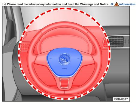
Fig. 30 Location and deployment zone of the driver's front airbag.
