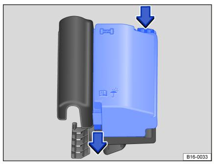
Fig. 141 In the engine compartment: cover of the fuse box.
