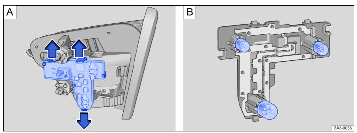
Fig. 139 Taillight: A: removing the bulb holder, B: removing the bulbs.
