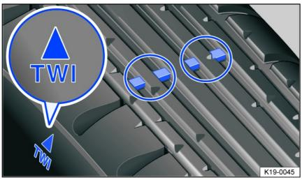
Fig. 165 Tire tread: tread wear indicator.
