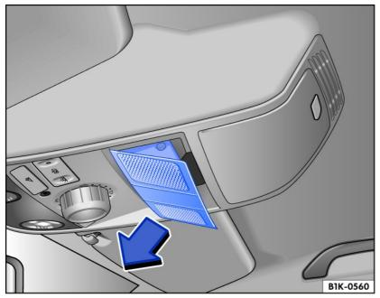
Fig. 61 In the headliner: remove the cover.
