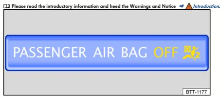
Fig. 29 In the instrument panel: Indicator light for the deactivated front passenger's front airbag.
