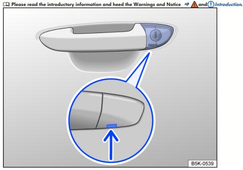
Fig. 49 Driver's door handle: covered lock cylinder.
