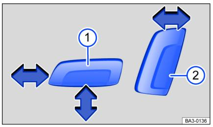
Fig. 67 Switch on the left front seat: adjusting the front seat forward/back, the height and angle of the seat surface, and the front seat backrest.
