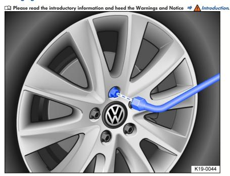
Fig. 176 Wheel change: removing wheel bolts with the lug wrench.
