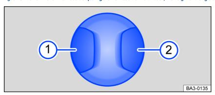
Fig. 68 Switch on the left front seat: adjusting the lumbar support.
