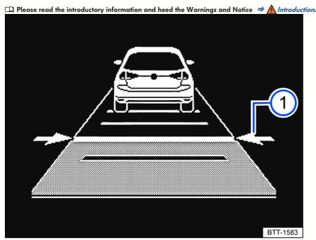
Fig. 104 In the instrument cluster display: set distance (1) (schematic diagram, ACC is regulating).
