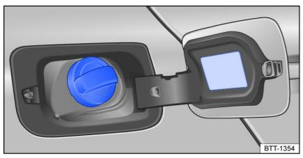
Fig. 127 Behind the fuel filler flap: fuel tank cap (general example)
