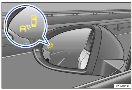
Fig. 107 In the exterior mirrors: Blind Spot Monitor indicator.
