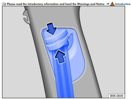
Fig. 28 Next to the front seats: safety belt height adjuster.
