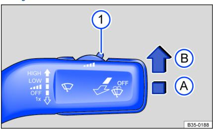
Fig. 82 On the right side of the steering column: windshield wiper lever.
