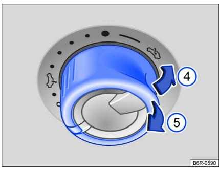
Fig. 59 In the headliner: pushing the switch to raise and pulling the switch to close.
