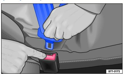
Fig. 25 Releasing the buckle tongue from the safety belt buckle.
