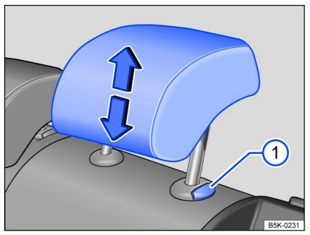
Fig. 71 Rear head restraint: adjusting.
