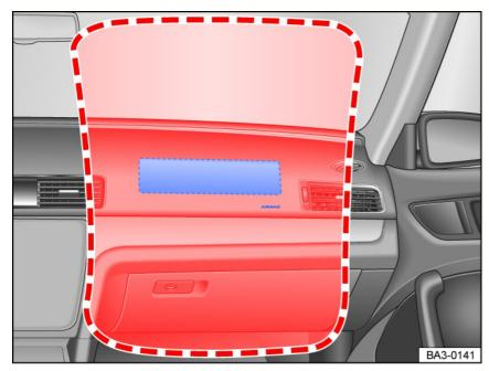
Fig. 31 Location and deployment zone of the front passenger's front airbag.
