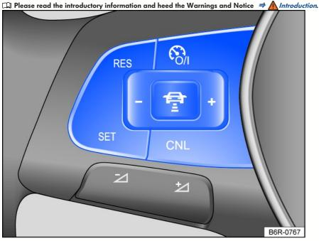
Fig. 103 Left side of the multi-function steering wheel: buttons for ACC operation.
