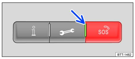
Fig. 41 In the roof console: controls for call services.
