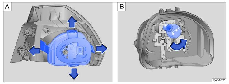
Fig. 137 A: Removing the bulb holder. B: Removing the bulbs.
