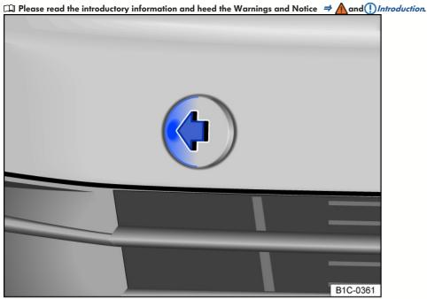
Fig. 145 In the right front bumper: Detach cover.
