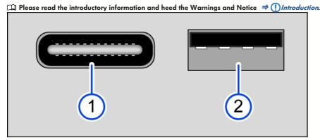
Fig. 118 Possible USB ports in the vehicle.
