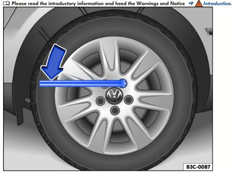
Fig. 171 Changing a tire: loosening the wheel bolts.
