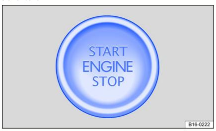
Fig. 92 In the lower area of the center console: starter button for starting the engine.
