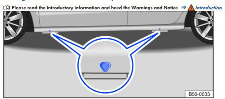
Fig. 174 Mounting points for the vehicle jack.
