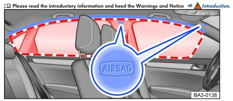
Fig. 34 On the left side of the vehicle: location and deployment zone of the Side Curtain Protection®.
