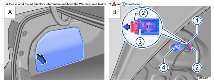
Fig. 136 In the side of the luggage compartment: A: opening the cover of the rear side trim panel. B: Removing the taillight.
