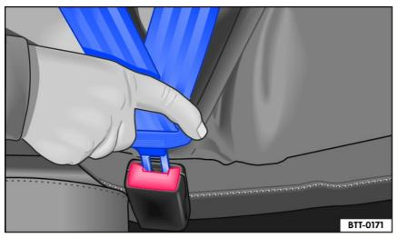
Fig. 24 Inserting the buckle tongue into the safety belt buckle.
