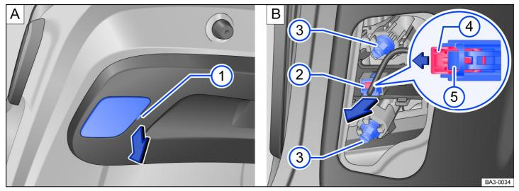
Fig. 138 In the trunk lid: A: removing the cover of the taillight, B: removing the taillight.
