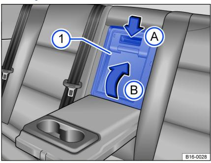
Fig. 125 In the rear seat backrest: Open load-through hatch.
