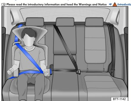
Fig. 40 Correctly secured child on a booster seat.
