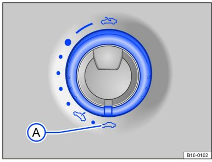
Fig. 60 In the headliner: switch for the power sunroof.
