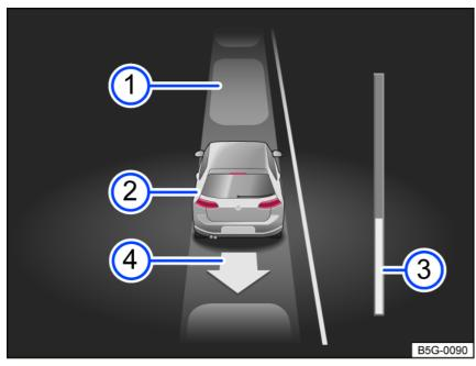
Fig. 113 In the instrument cluster display: reversing out of a parking space parallel to the road.
