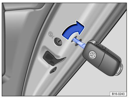
Fig. 51 On the front of the right rear door: manually locking the vehicle with the vehicle key.
