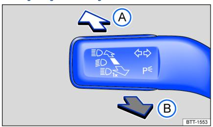
Fig. 79 On the left side of the steering column: turn signal and high beam lever.
