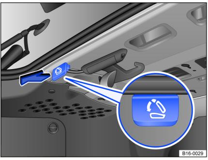
Fig. 69 In the luggage compartment: Remote release lever.
