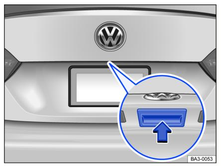
Fig. 54 In the trunk lid: button to open the trunk lid.
