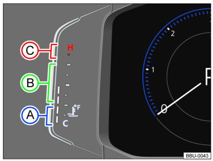
Fig. 14 Engine coolant temperature gauge in the digital instrument cluster.
