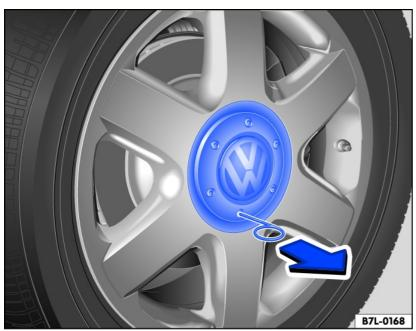
Fig. 167 Remove the hubcap.
