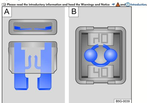
Fig. 142 Blown fuse: A flat connector fuse B block fuse.
