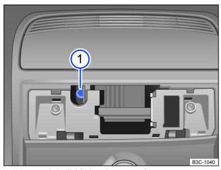
Fig. 62 Hexagon socket head bolt for closing the power sunroof.
