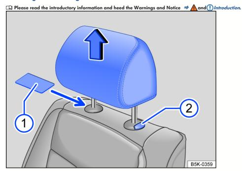
Fig. 72 Front head restraints: removing.
