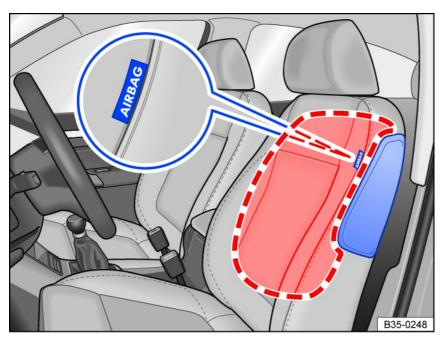
Fig. 33 In the side of the front seat: Side airbag installation location and deployment zone.
