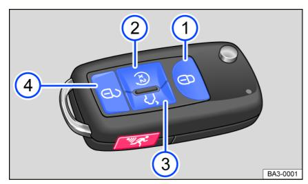
Fig. 93 Vehicle key with remote start relay function
