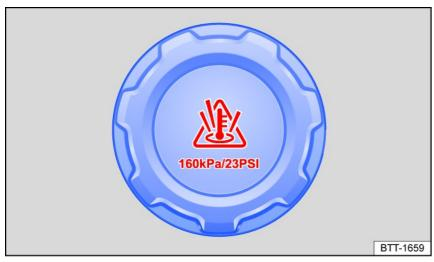
Fig. 156 In the engine compartment: cap on the engine coolant expansion tank.
