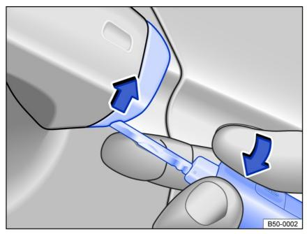
Fig. 50 Driver's door handle: prying off the cap.
