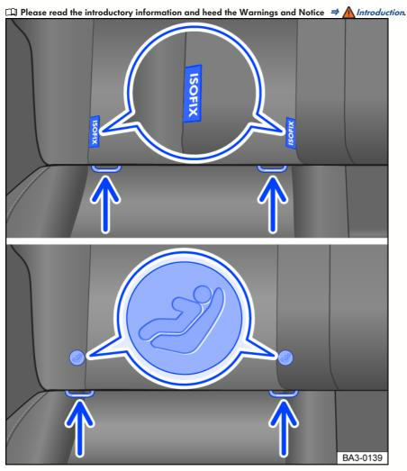
Fig. 36 On the vehicle seat: label for child restraint LATCH/UAS anchor points.
