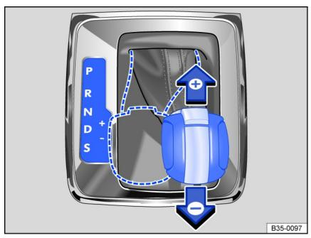
Fig. 96 Selector lever in tiptronic position.
