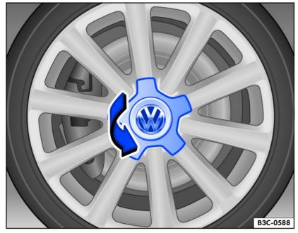
Fig. 168 Unscrew the hubcap.
