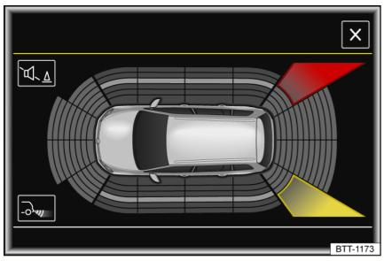
Fig. 115 On the Infotainment system screen: Rear Traffic Alert display.
