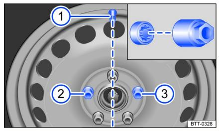
Fig. 172 Changing a tire: tire valve (1) and locations of the anti-theft wheel bolt (2) or (3).
