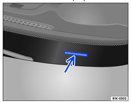
Fig. 179 In the windshield: vehicle identification number (VIN)
