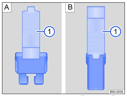
Fig. 143 Removing or installing a fuse with the plastic pliers: A: flat connector fuse, B: block fuse.
