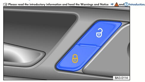
Fig. 48 In the driver's door: central locking button.
