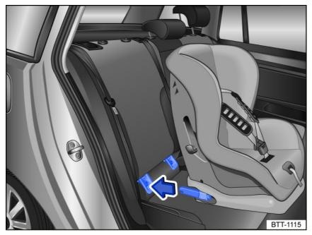
Fig. 37 General example: Installing a child restraint with attachment arms.
