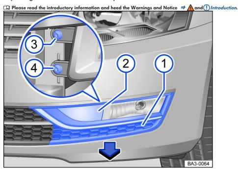
Fig. 134 In the front bumper on the left: replacing the headlight.
