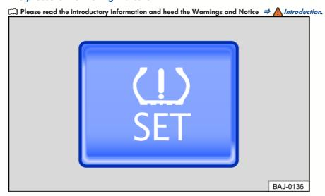
Fig. 162 In the glove box: Button for the Tire Pressure Loss Indicator.
