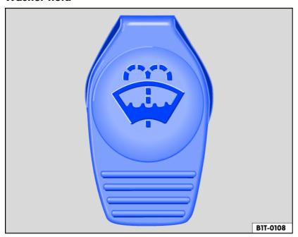
Fig. 152 In the engine compartment: cap on the washer fluid reservoir.
