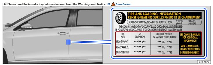
Fig. 164 On the driver door pillar: tire pressure sticker
