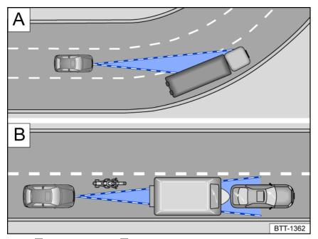
Fig. 101 A Driving around curves. B Vehicles outside of the radar sensor range.
