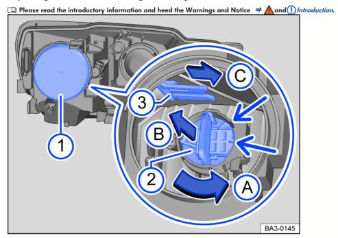
Fig. 132 In the engine compartment: Rear view of the left headlight.
