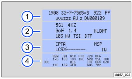
Fig. 181 General example: vehicle data label
