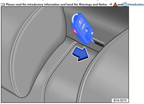
Fig. 56 Behind the rear seat backrest: mechanically unlocking the rear seat backrest using the emergency release.
