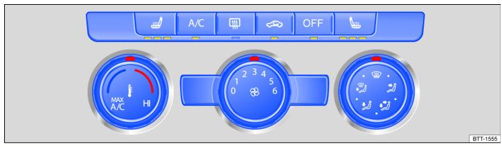
Fig. 87 In the upper section of the center console: climate control toolbar for the manual climate control system.
