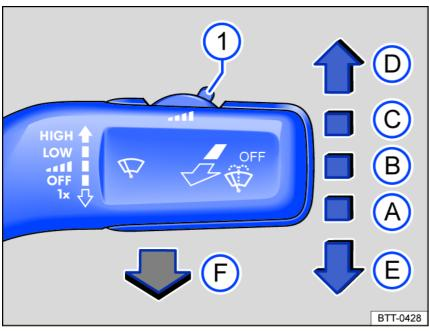
Fig. 81 On the right side of the steering column: operating the windshield wipers.
