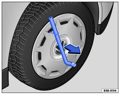
Fig. 169 Remove the full wheel cover.
