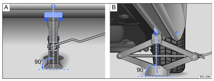
Fig. 175 Jack is positioned on the left side of the vehicle at the rear.
