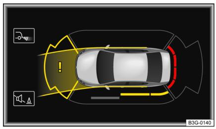
Fig. 109 On the Infotainment system screen: Park Distance Control display with steering wheel angle and obstacles.
