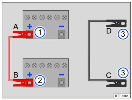
Fig. 144 Diagram for connecting the jump-start cables.
