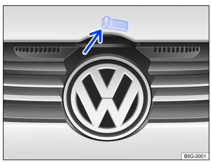
Fig. 148 Above the radiator grille: Opening lever for the hood.
