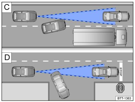
Fig. 102 C Changing lanes. D Turning and stationary vehicles.
