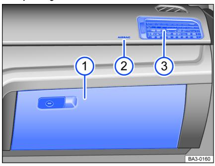
Fig. 10 Passenger's side: instrument panel overview.
