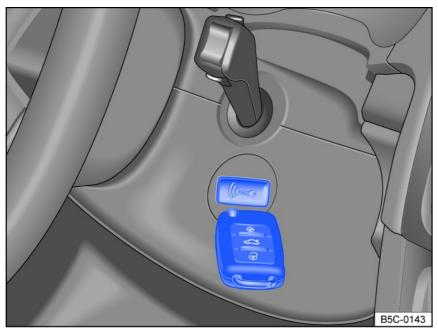
Fig. 94 On the right side of the steering column: emergency start function on vehicles with Keyless Access with push-button start.
