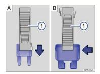
Fig. 193 Removing or inserting a fuse using the plastic tweezers.
