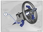
Fig. 44 Manual adjustment for the steering wheel position.
