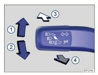
Fig. 76 Turn signal lever and high beam switch.
