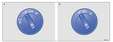
Fig. 77 Headlight switch next to the steering wheel: (A) vehicles with front fog lights. (B) vehicles without front fog lights.
