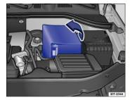
Fig. 169 In the engine compartment: Open the sleeve covering of the vehicle battery.
