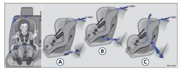
Fig. 72 Some child restraints are equipped with lower anchors and a top tether, illustration (A) and (B) show the correct installation of the attachments applicable to a LATCH/UCRA seat. Figure (C) shows the installation of the seat using the vehicle's safety belt system.
