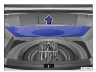
Fig. 172 In the luggage compartment under the floor panel: Compact spare wheel and vehicle tool kit.
