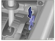
Fig. 182 Releasing the selector lever lock.
