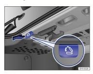
Fig. 89 On the left side of the luggage compartment: Release lever for the left-side rear seat backrest. The release lever for the right-side rear seat backrest is on the right side of the luggage compartment.
