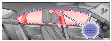
Fig. 68 On the left vehicle side: Installation location and deployment zone of the Side Curtain Protection® airbag.
