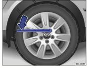
Fig. 185 Changing a wheel: Loosening wheel bolts.
