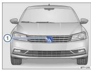
Fig. 132 Behind the Volkswagen emblem: Radar sensor.
