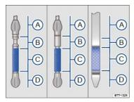
Fig. 164 Engine oil dipsticks with oil level marks.
