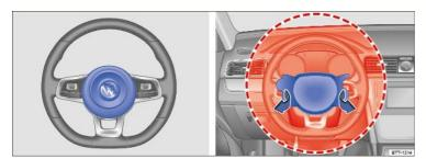
Fig. 65 Location and deployment zone of the driver front airbag.
