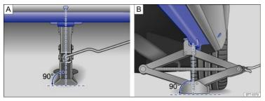
Fig. 188 Jack in position at the left rear lift point.
