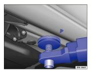
Fig. 175 Rear lift point for workshop hoist or floor jack.
