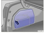
Fig. 170 In the side of the luggage compartment: On vehicles with 3.6 liter engines, the vehicle battery is on the left side of the luggage compartment.
