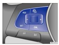
Fig. 129 Left-hand side of the multi-function steering wheel: Buttons for using the cruise control.
