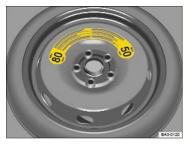
Fig. 100 In the luggage compartment: Compact spare wheel.
