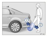
Fig. 30 Opening the sensor-controlled trunk lid (Easy Open).
