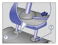
Fig. 43 Removing the rear head restraints.
