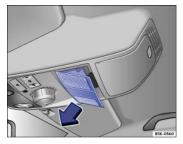
Fig. 179 In headliner: Removing cover.
