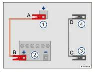
Fig. 197 Diagram for attaching the jumper cables with positive jump start terminals in the engine compartment: Positive jump start terminal ① and booster battery ②.
