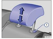
Fig. 41 Adjusting the rear head restraints.
