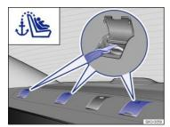
Fig. 75 Anchorages in the shelf behind the rear seat backrest.
