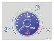
Fig. 166 Engine coolant temperature gauge in the instrument cluster: (A) Engine cold; (B) Normal temperature range; (C) Warning zone.
