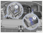
Fig. 194 In the engine compartment (2.0 liter engine): Positive jump-start terminal  $\oplus$  and negative jump-start terminal  $\ominus$ .
