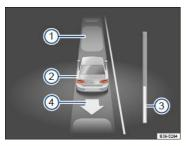
Fig. 152 In the instrument cluster display: Driving out of a parallel parking space.
