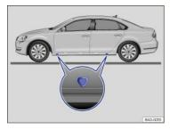
Fig. 187 Lift points for the jack.
