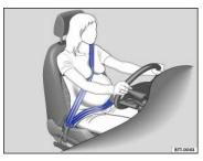
Fig. 60 Proper safety belt positioning for expectant mothers.
