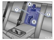
Fig. 92 In the rear seat backrest: Opening luggage compartment pass-through with lock.
