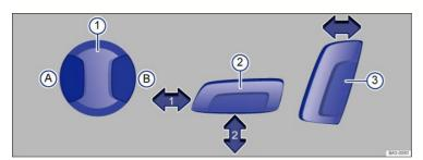
Fig. 39 Driver seat: controls to adjust lumbar support ①, seat cushion ②, and seat backrest angle ③.
