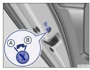
Fig. 25 In the rear driver side door: Child safety lock (A) switched off, (B) switched on.
