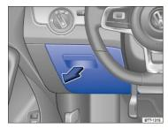
Fig. 190 On the driver side in the instrument panel: Fuse box behind the storage compartment.
