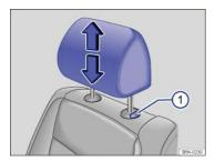
Fig. 40 Adjusting the front head restraints.
