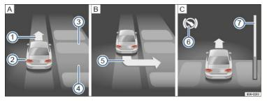
Fig. 151 In the instrument cluster display: Parking perpendicular to the road. Searching for a parking space, positioning the vehicle for parking, maneuvering.
