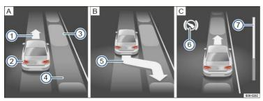
Fig. 150 In the instrument cluster display: Parallel parking. Searching for a parking space, positioning the vehicle for parking, maneuvering.
