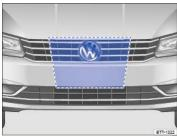
Fig. 133 Area around the radar sensor to be kept clean and free of obstructions.
