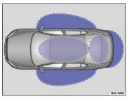
Fig. 23 Ranges of the Keyless Access with push button start. Outside the vehicle: Unlocking range. Inside the vehicle: Starting range.
