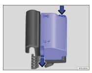
Fig. 191 In the engine compartment: Fuse box cover.
