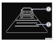
Fig. 130 In the instrument cluster display: ACC switched off temporarily; vehicle detected ahead, time interval set.
