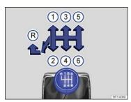
Fig. 120 Gearshift pattern of a 6-speed manual transmission.
