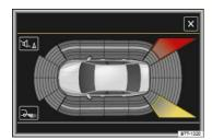
Fig. 157 Rear Traffic Alert display: Colored display shown (may vary depending on vehicle equipment).
