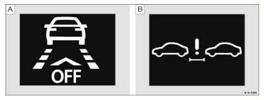
Fig. 137 Symbols in the instrument cluster display. : Distance warning. : System switched off (symbol displayed in color on an instrument cluster with color display).
