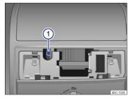
Fig. 180 Hexagonal head screw for closing the power sunroof.
