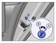
Fig. 26 In the rear passenger side door: Child safety lock A switched off, B switched on.
