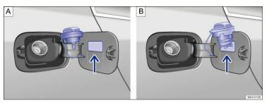
Fig. 162 Fuel cap placed on the open fuel filler flap.
