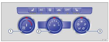
Fig. 158 In the center console: Manual air conditioning controls.
