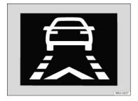
Fig. 138 In the instrument cluster display: Advance warning (symbol displayed in color on an instrument cluster with color display).
