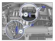
Fig. 195 In the engine compartment (3.6 liter engine): Positive jump-start terminal ⊕ and negative jump-start terminal ⊖.
