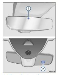
Fig. 87 Auto-dimming inside mirror.
