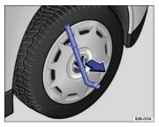
Fig. 184 Pulling the wheel cover off.
