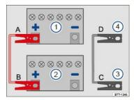
Fig. 196 Diagram for attaching the jumper cables: Dead battery ① and booster battery ②.
