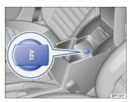
Fig. 112 12 Volt socket in the front center armrest.
