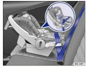
Fig. 71 Rearward-facing infant seat properly installed on the rear seat.
