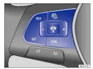
Fig. 134 Left-hand side of the multi-function steering wheel: Buttons for using ACC.
