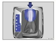
Fig. 121 Automatic transmission selector lever with shift lever release button (arrow).
