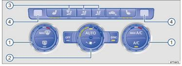
Fig. 159 In the center console: Climatronic controls.
