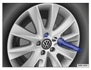
Fig. 189 Changing a wheel: remove previously loosened wheel bolts using the screwdriver handle.
