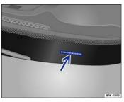
Fig. 199 Vehicle identification number (VIN).
