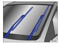
Fig. 82 Windshield wiper in service position.
