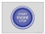
Fig. 114 In the center console: Starter button of the Keyless Access with push button start.
