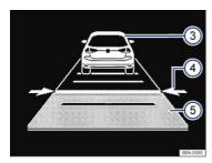
Fig. 131 In the instrument cluster display: ACC active, vehicle detected ahead, time interval is being set.
