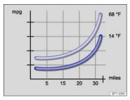
Fig. 126 Fuel consumption in mpg at 2 different outside air temperatures.
