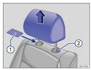
Fig. 42 Removing the front head restraints.
