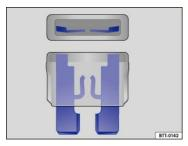
Fig. 192 Illustration of a blown fuse.
