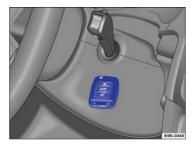
Fig. 115 Emergency starting feature on vehicles with Keyless Access.
