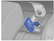
Fig. 31 Behind the rear seat backrest on the driver side: releasing the rear seat backrest.
