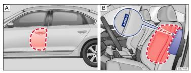
Fig. 67 On the driver side: Deployment zone of the side airbags (A). In the padding on the outboard side of the front seat backrests: Location and deployment zone of the side airbags (B).
