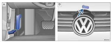
Fig. 163 A: In the footwell on the driver side: Inside engine hood release lever. B: Above the radiator grille: Outside engine hood release (under the hood).
