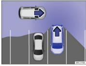
Fig. 156 Rear Traffic Alert: Monitored area around the vehicle that is backing out of a parking space.
