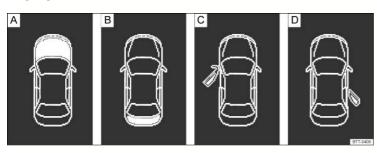
Fig. 10 In the instrument cluster display: A: Open engine hood, B: Open trunk lid, C: Open front driver side door, D: Open rear passenger side door.
