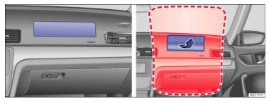
Fig. 66 Location and deployment zone of the front passenger front airbag.
