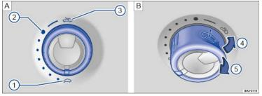
Fig. 34 In the headliner: Rotary switch for the power sunroof.
