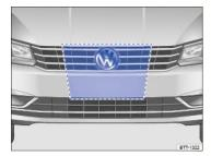
Fig. 140 Area around the radar sensor to be kept clean and free of obstructions.
