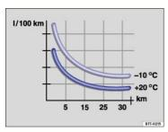
Fig. 127 Fuel consumption in I/100 km at 2 different outside air temperatures.
