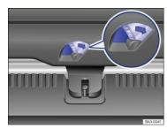
Fig. 32 Inside the luggage compartment: Unlocking the trunk lid.
