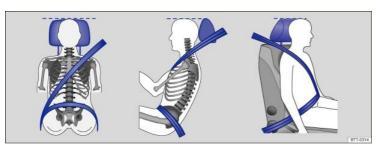
Fig. 59 Proper safety belt positioning and head restraint adjustment.
