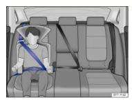
Fig. 73 Child properly restrained in a booster seat on the rear seat.
