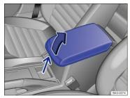
Fig. 106 In the front center armrest: Storage compartment.
