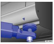
Fig. 174 Front lift point for workshop hoist or floor jack.
