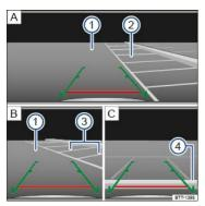
Fig. 146 On the screen: Orientation lines for the parking space behind the vehicle. : Searching for a parking space, : Backing into the parking space, :
