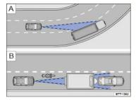
Fig. 135 Driving in a curve. Motorcycle traveling ahead outside of the sensor range.
