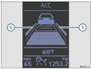
Fig. 141 In the instrument cluster display: Lane Assist display (example 1).
