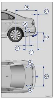
Fig. 95 Dimensions and attachment points for retrofitting a trailer hitch.
