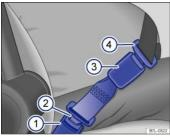
Fig. 62 A safety belt extender properly attached to the factory-installed safety belt.
