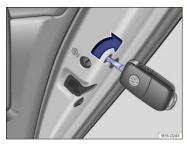
Fig. 178 On the front side of the right rear door: Manual vehicle locking with the key bit in the vehicle key.
