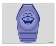
Fig. 85 In the engine compartment: Cap of the windshield washer fluid reservoir.
