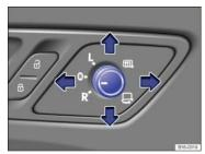
Fig. 88 In the driver door: Adjusting knob for outside mirrors.
