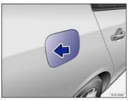
Fig. 161 Right rear side of vehicle: Opening the fuel filler flap.
