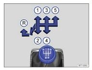
Fig. 119 Gearshift pattern of a 5-speed manual transmission.
