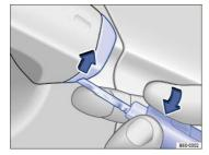
Fig. 177 Door handle on driver door: Concealed lock cylinder.
