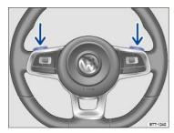
Fig. 123 Steering wheel with optional Tiptronic shift paddles.
