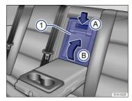
Fig. 91 In the rear seat backrest: Opening luggage compartment pass-through without lock.
