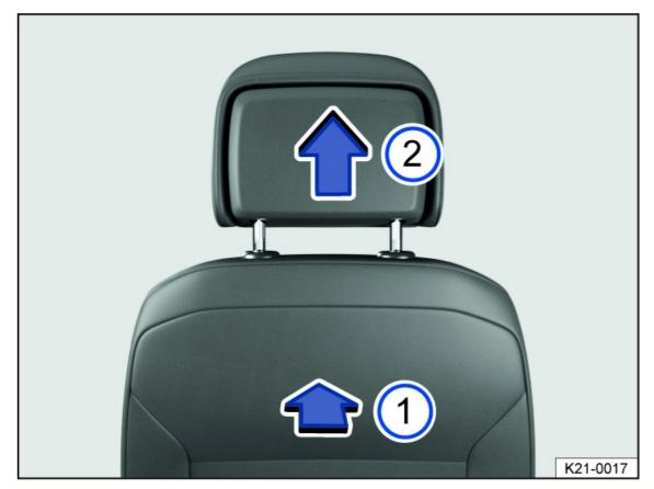
Fig. 70 Removing the front head restraint (general example).
