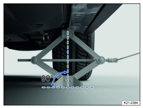
Fig. 188 On the left side of the vehicle at the rear: jack in position (variant 2).
