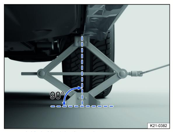
Fig. 186 On the left side of the vehicle at the rear: jack in position (variant 1).
