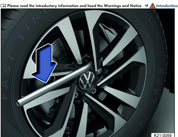
Fig. 182 Loosening wheel bolts.
