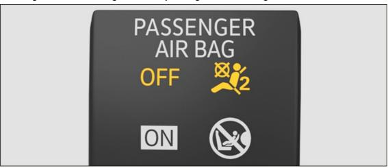
Fig. 29 In the center console: indicator light for the switched off front passenger's front airbag.
