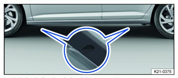
Fig. 184 On the side sill: markings for the jack lift points (variant 2).
