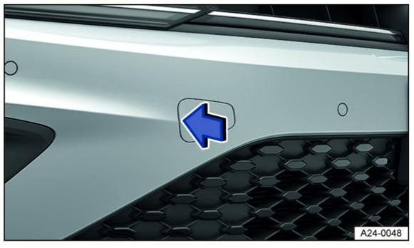
Fig. 152 In the right front bumper: Remove the cover, variant 1.
