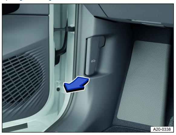
Fig. 160 In the driver's side footwell: Release lever for the hood (general example).
