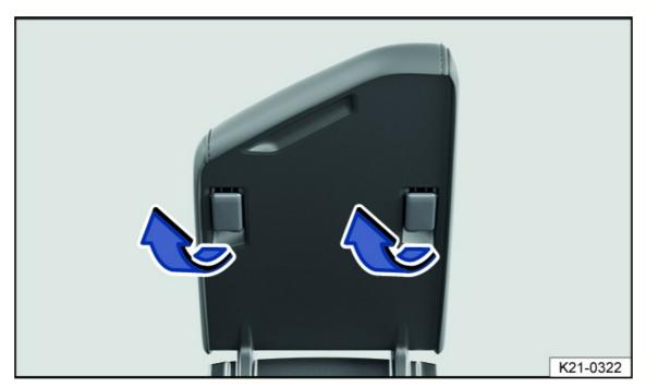
Fig. 73 Underside of the front center armrest: plastic supports of the center armrest.
