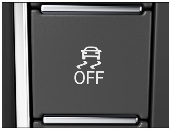
Fig. 103 Located on the center console: Button to manually switch ASR or ESC Sport on and off (depending on how your vehicle is equipped).
