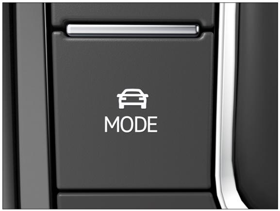
Fig. 104 In the center armrest: Diving Mode Selection MODE button.
