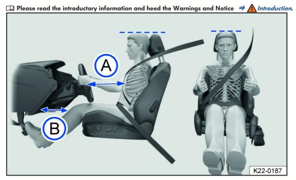
Fig. 22 Correct distance between the driver and the steering wheel, correct safety belt position and correct head restraint
