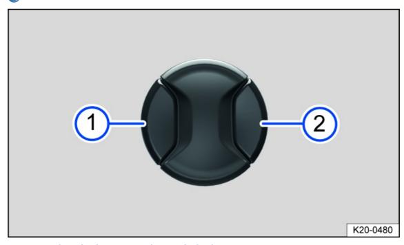
Fig. 65 Switch on the driver seat: Adjusting the lumbar support.
