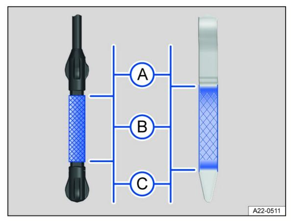
Fig. 168 Engine oil level markings on the oil dipstick (versions).
