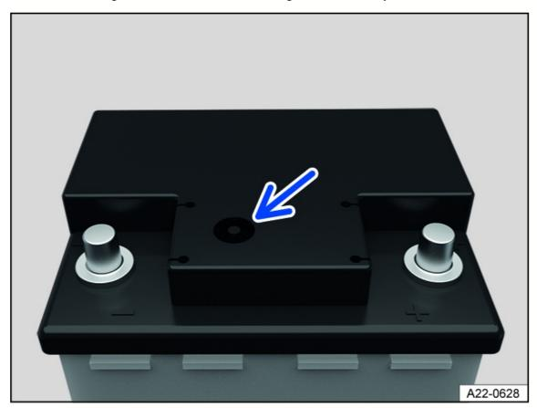
Fig. 172 On the top of the 12 V vehicle battery: Window (general example).
