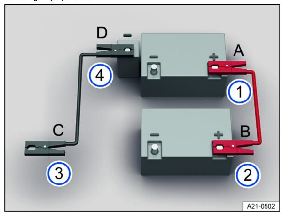
Fig. 150 Diagram for connecting the jumper cables.
