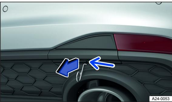
Fig. 158 In the right rear bumper: Remove cover.
