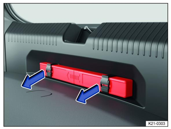
Fig. 40 Underneath the load sill: holder for the warning triangle.
