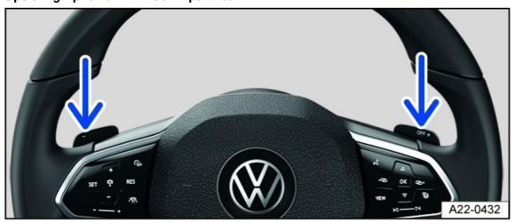
Fig. 100 Behind the steering wheel: shift paddles for the tiptronic.
