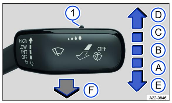
Fig. 81 On the right side of the steering column: operating the windshield wipers.
