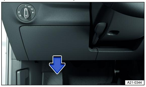
Fig. 145 Next to the steering wheel on the left: Cover for the fuse box in the dash panel.
