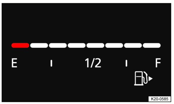
Fig. 16 In the Volkswagen Digital Cockpit Basic: fuel gauge (general example).
