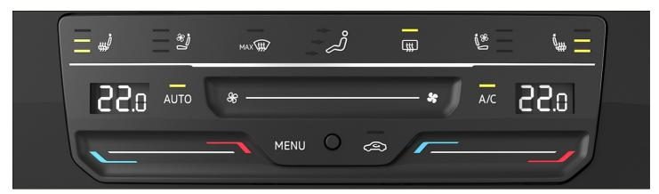
Fig. 87 In the upper section of the center console: air conditioning block for the Climatronic system (version 1).
