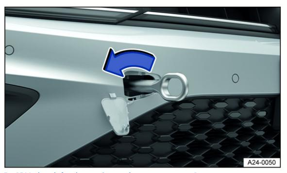
Fig. 154 In the right front bumper: Screw in the towing eye, variant 1.
