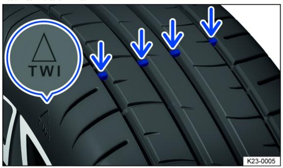
Fig. 177 In the tread grooves: wear indicator.
