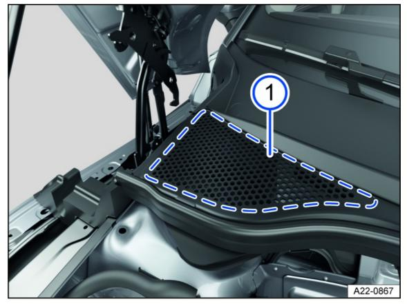
Fig. 195 Between the hood space and windshield: Plenum chamber (general example).
