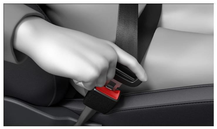
Fig. 24 Inserting the buckle tongue into the safety belt buckle (general example).
