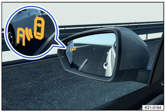
Fig. 121 In the mirror glass of the outside mirrors: Blind Spot Monitor indicator.
