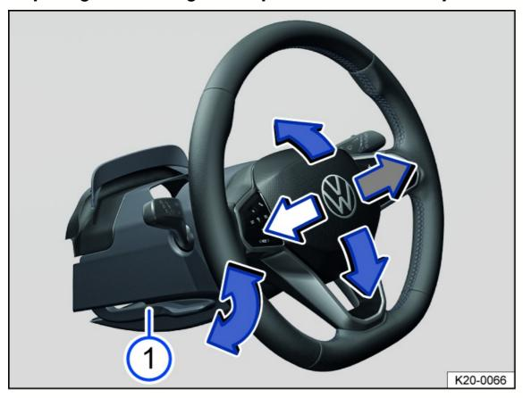
Fig. 61 Under the steering wheel in the steering column trim panel: lever to adjust the steering wheel position manually (general example).
