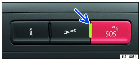
Fig. 41 In the roof console: buttons for call services and indicator light.
