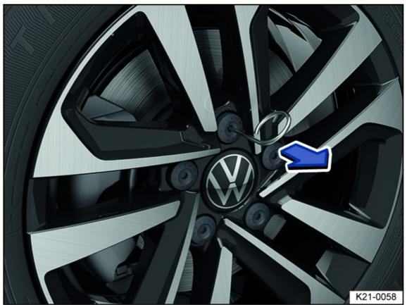
Fig. 181 Remove the caps from the wheel bolts.
