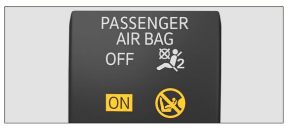
Fig. 30 In the center console: indicator light for the activated passenger's front airbag.
