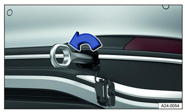
Fig. 157 In the right rear bumper: Screw in towing eye.
