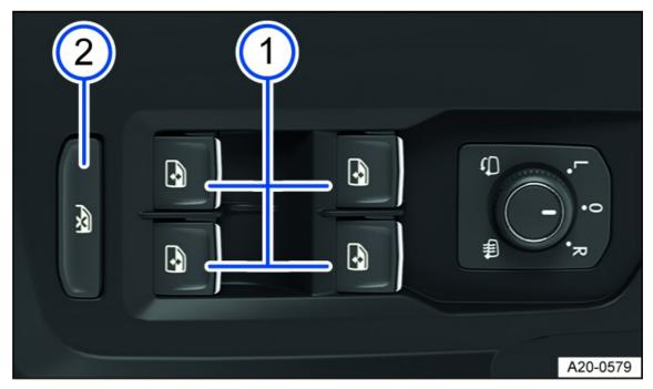
Fig. 59 In the driver door: Power window buttons.
