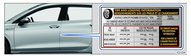
Fig. 173 On the driver door pillar: Tire inflation pressure label.
