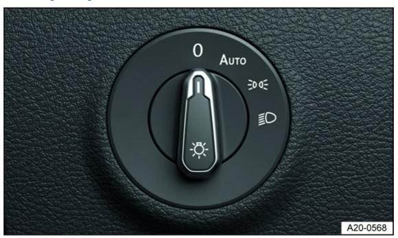
Fig. 77 Next to the steering wheel: light switch (one version).
