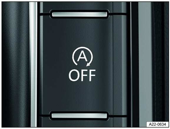
Fig. 96 In the lower section of the center console: Button for the start-stop system.
