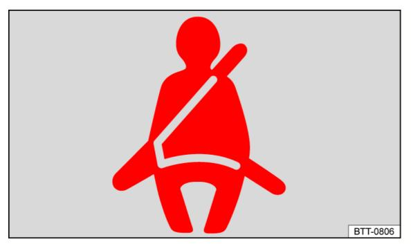
Fig. 23 In the instrument cluster display: warning light for the fasten seat belts reminder.
