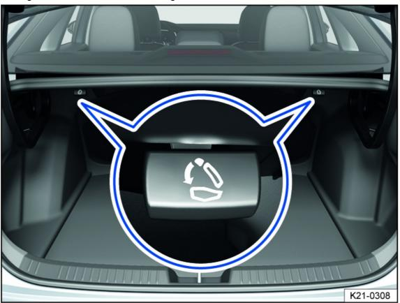
Fig. 66 In the luggage compartment: Remote release lever.
