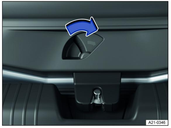
Fig. 58 In the luggage compartment: mechanically unlocking the trunk lid using the emergency release.
