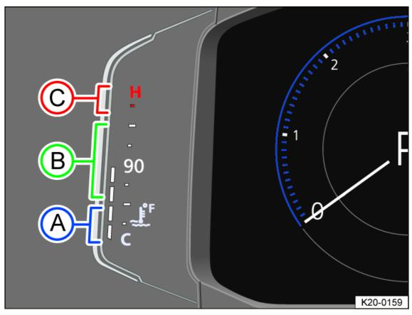
Fig. 17 In the Volkswagen Digital Cockpit Pro: coolant temperature gauge (general example).
