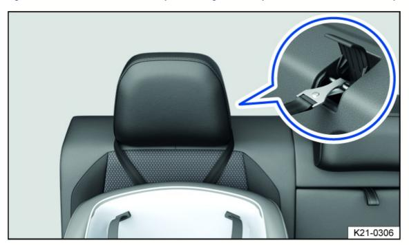
Fig. 37 On the rear seat backrest: Safety belt routing for non-adjustable head restraints with a V-shaped top tether safety
