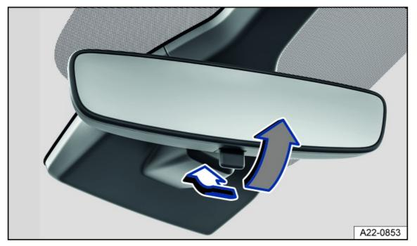
Fig. 84 On the windshield: manual dimming interior rearview mirror.
