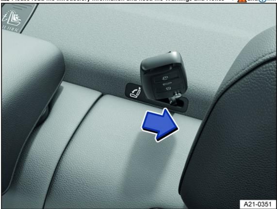
Fig. 57 Behind the rear seat backrest: mechanically unlocking the rear seat backrest using the emergency release.
