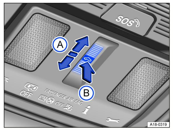
Fig. 60 In the headliner: Control for the tilting and sliding panoramic sunroof.
