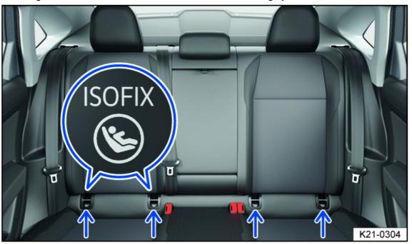
Fig. 33 On the outer rear seats: label for ISOFIX/lower LATCH anchorage points for child restraints.
