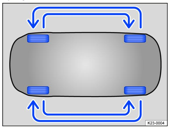
Fig. 176 Diagram for rotating the wheels (general example).
