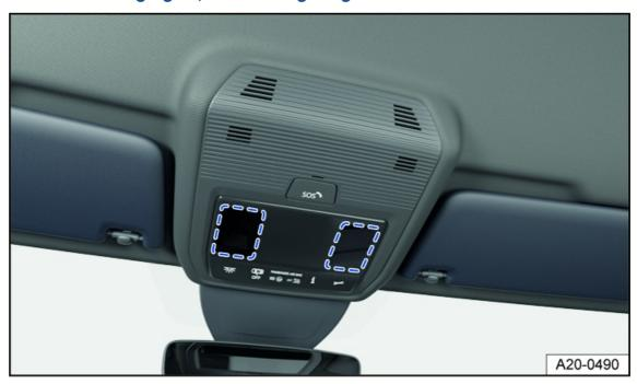
Fig. 80 On the overhead console: touch-sensitive reading lights.
