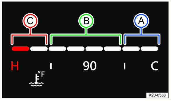
Fig. 18 In the Volkswagen Digital Cockpit Basic: coolant temperature gauge (general example).
