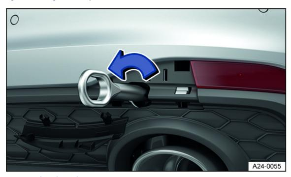
Fig. 159 In the right rear bumper: Screw in towing eye.
