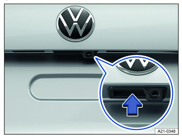
Fig. 56 In the trunk lid: button to open the trunk lid.
