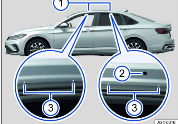
Fig. 134 Mounting points for base supports.
