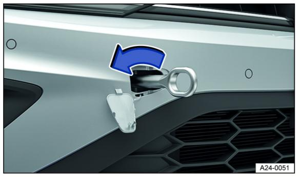
Fig. 155 In the right front bumper: Screw in the towing eye, variant 2.
