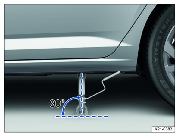
Fig. 185 Correct jack setup (variant 1).
