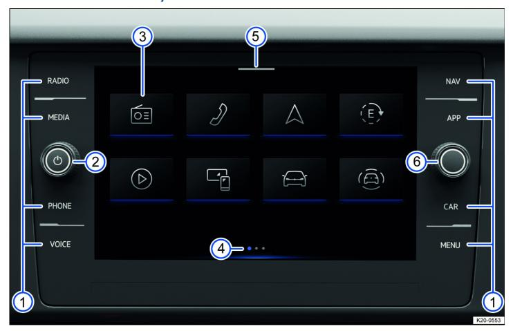
Fig. 131 Overview of the Infotainment system (general example).
