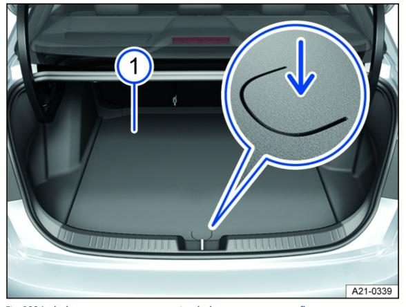
Fig. 133 In the luggage compartment: opening the luggage compartment floor.
