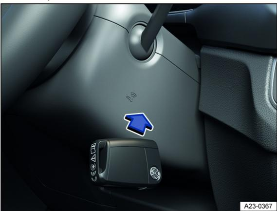
Fig. 95 On the right side of the steering column: emergency start function on vehicles with Keyless Access with push-button start.
