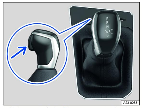
Fig. 98 In the center console: selector lever of the automatic transmission (general example).
