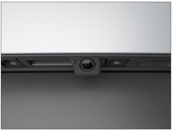
Fig. 196 In the rear of the vehicle: Rear View Camera system on the handle (general example).
