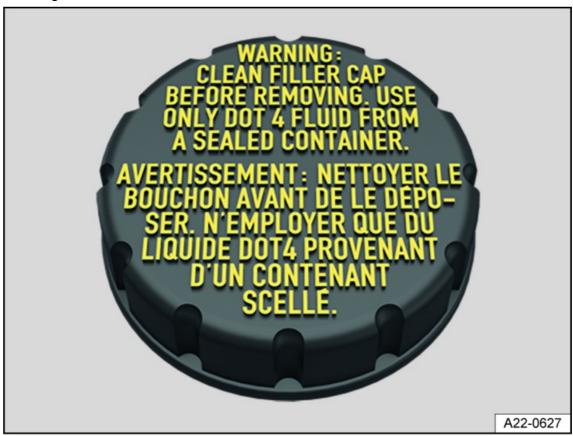
Fig. 171 In the hood space: Cap on the brake fluid reservoir.
