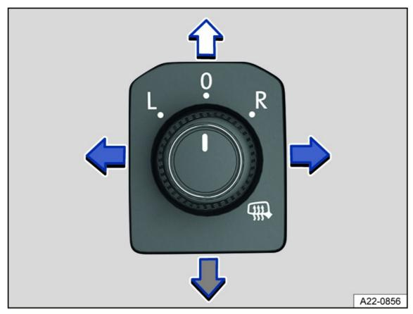
Fig. 85 In the driver door: knob for the outside mirrors.
