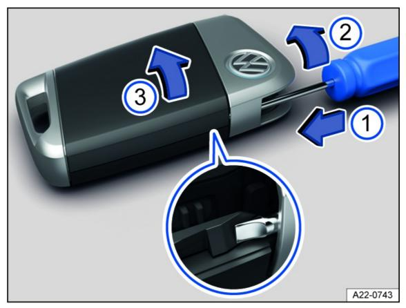
Fig. 47 Remote control vehicle key: opening the battery compartment cover.
