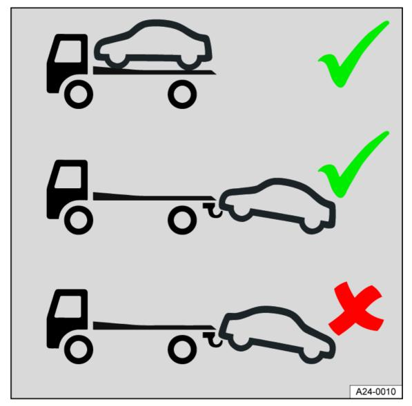
Fig. 151 Transporting the vehicle away with a tow truck.
