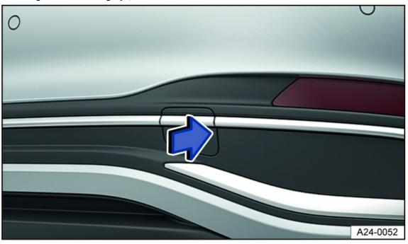
Fig. 156 In the right rear bumper: Remove cover.
