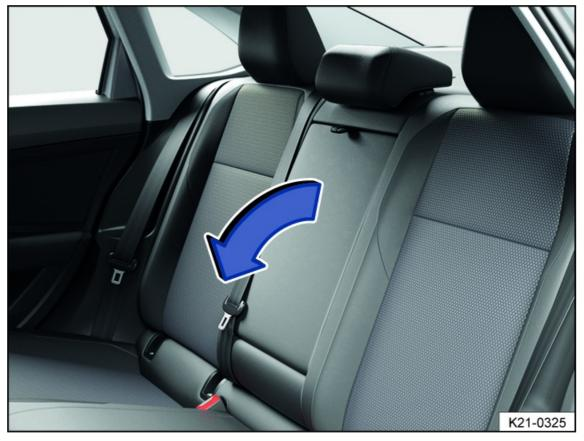
Fig. 74 In the backrest of the center seat: folding rear center armrest.
