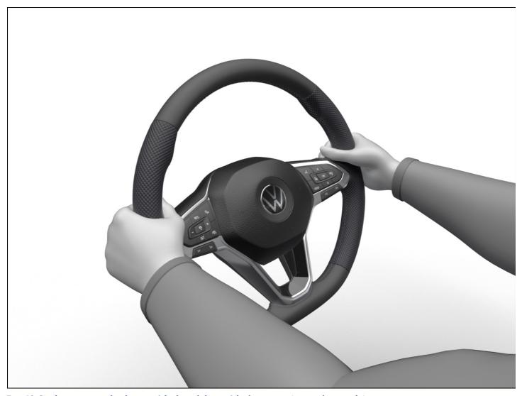
Fig. 62 On the steering wheel: nine o'clock and three o'clock position (general example).
