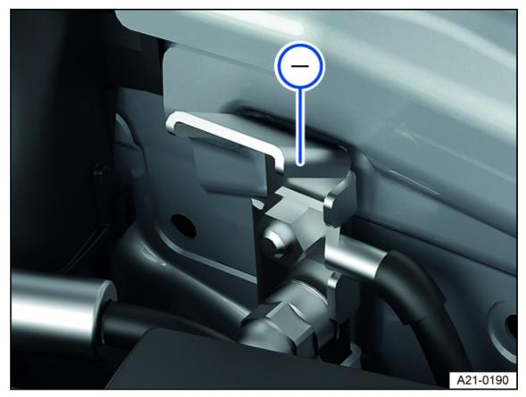
Fig. 149 In the hood space: Negative terminal jump-start point.
