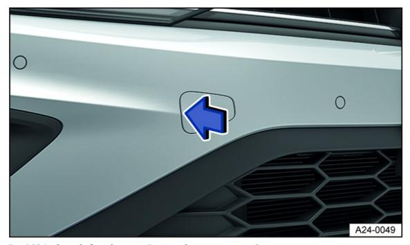
Fig. 153 In the right front bumper: Remove the cover, variant 2.
