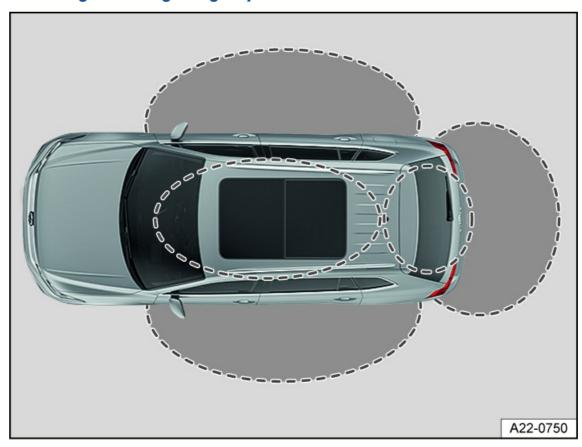
Fig. 49 Keyless Access: Sensor ranges (general example).
