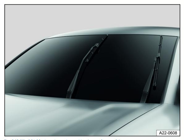
Fig. 140 Windshield wipers in service position (general example).
