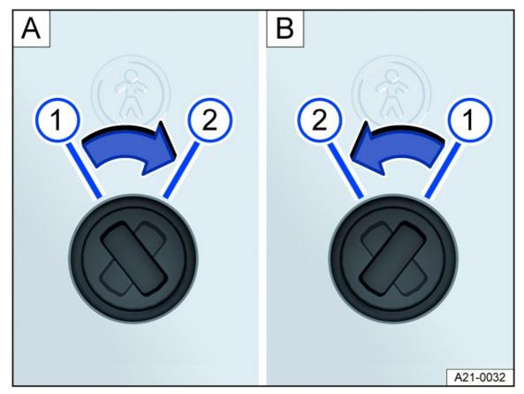
Fig. 54 Child safety lock: A left rear door, B right rear door.
