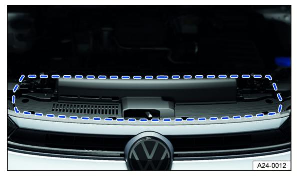
Fig. 165 Area for the engine oil label (general example).
