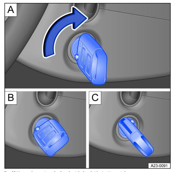
Fig. 93 Next to the steering wheel on the right-hand side: ignition switch.
