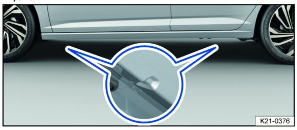
Fig. 183 On the side sill: markings for the jack lift points (variant 1).
