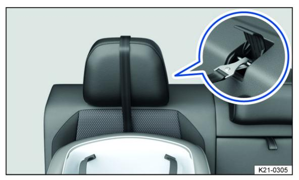
Fig. 36 On the rear seat backrest: Safety belt routing for non-adjustable head restraints with a top tether individual belt.
