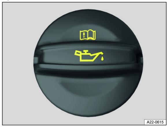
Fig. 167 In the hood space: engine oil filler cap (general example).
