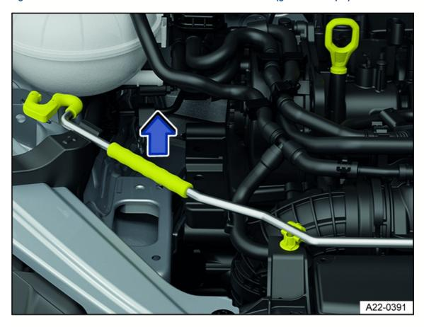
Fig. 161 In the hood space: Hood support in the bracket.
