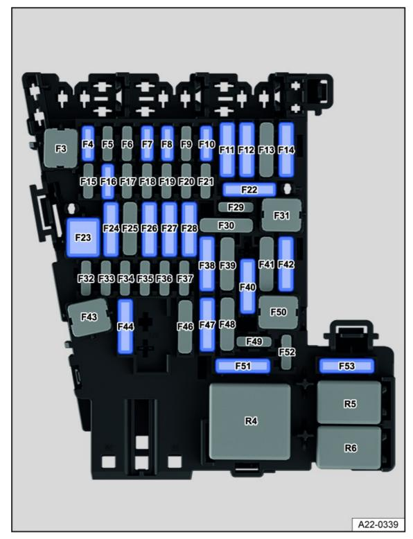
Fig. 146 Fuse assignment in the instrument panel.
