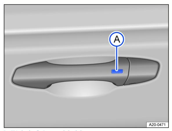
Fig. 50 In door handle: Button to unlock or lock.
