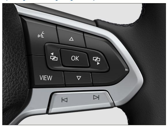
Fig. 13 Right side of the multi-function steering wheel: Operating the Volkswagen Digital Cockpit Basic (variant 1).
