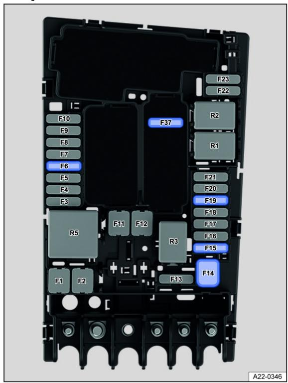
Fig. 144 In the hood space: Fuse locations.
