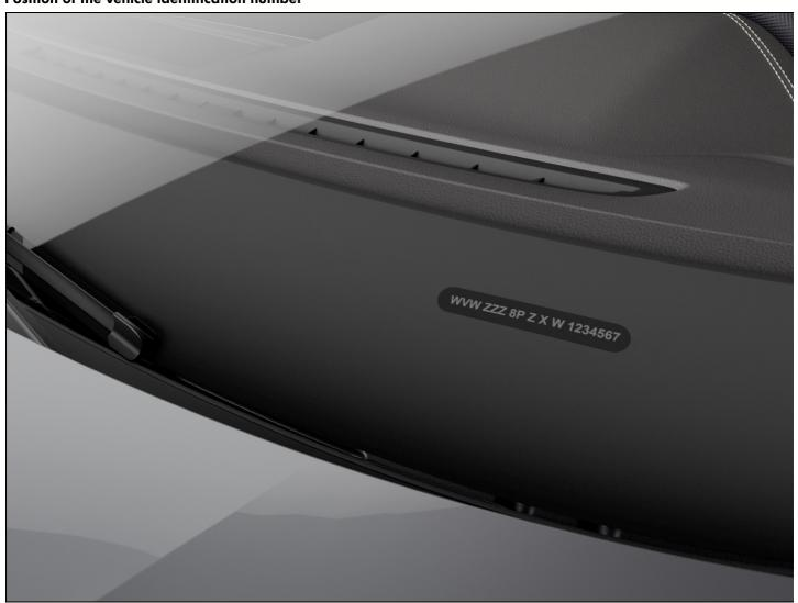
Fig. 197 In the windshield: vehicle identification number (VIN)
