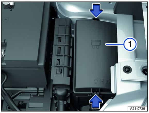
Fig. 143 In the hood space: fuse box.
