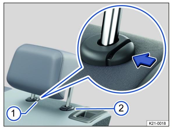
Fig. 71 Removing the middle rear head restraint (general example).
