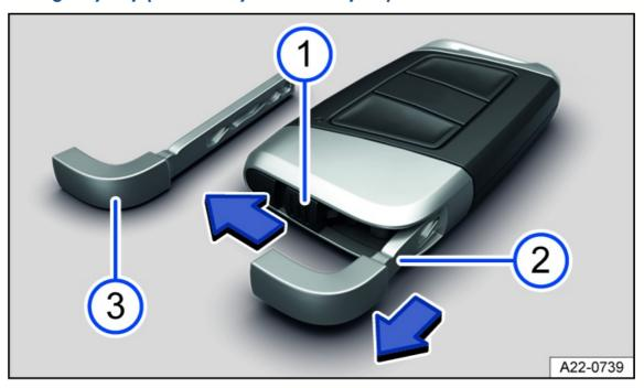
Fig. 45 Vehicle key: Unlocking the emergency key (general example).
