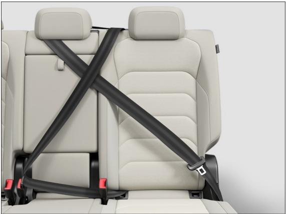
Fig. 38 Securing unused safety belts (general example).
