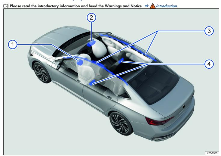
Fig. 31 Installation locations and deployment zones of the airbags.
