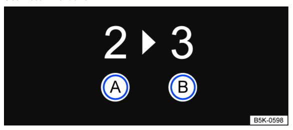
Fig. 106 Gear recommendation on the instrument cluster display.
