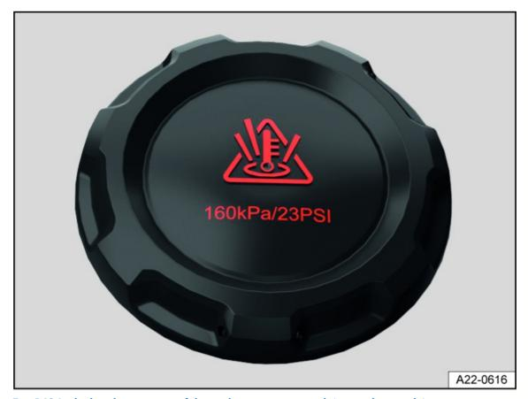
Fig. 169 In the hood space: cap of the coolant expansion tank (general example).
