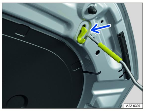
Fig. 162 On the engine hood: Hood support bracket.
