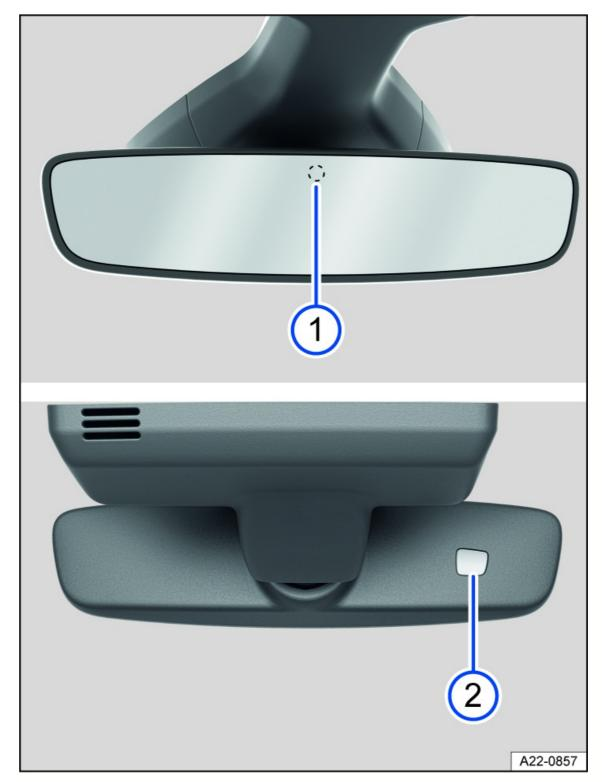
Fig. 83 On the windshield: automatic dimming interior rearview mirror.
