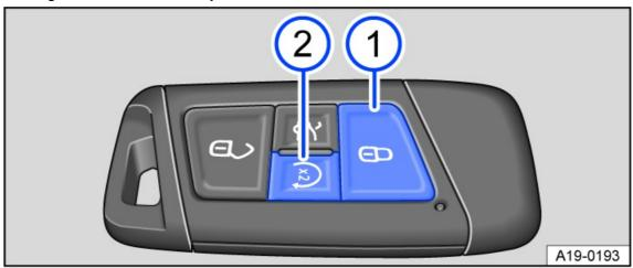
Fig. 92 On the remote control vehicle key: Button for remote start relay function.
