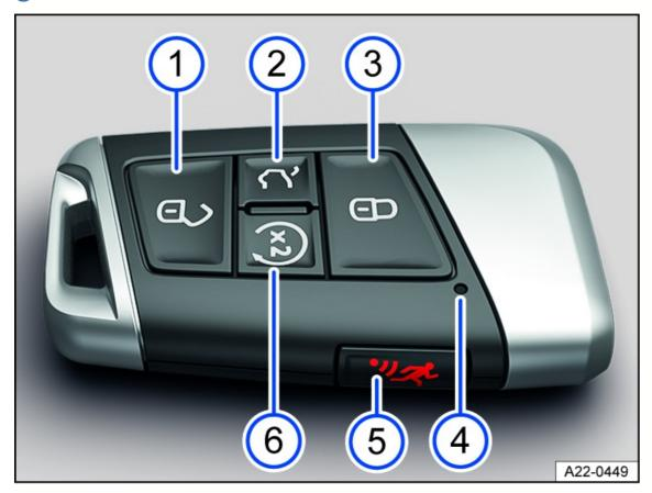
Fig. 44 Vehicle key with remote start relay function.
