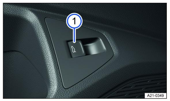
Fig. 55 In the driver's door: unlock button for the trunk lid.
