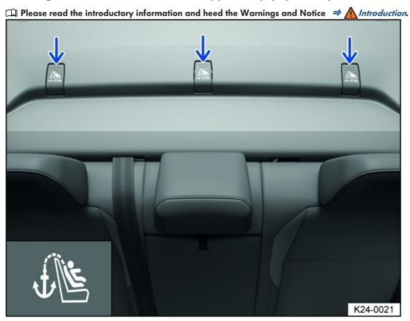
Fig. 35 In the storage compartment behind the rear seats: top tether anchorages for the top tether safety belt.
