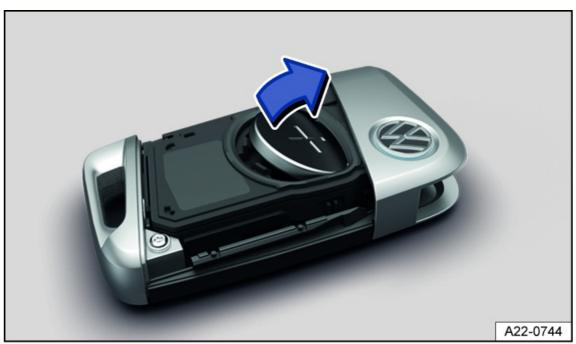
Fig. 48 Vehicle key: replacing the button cell battery
