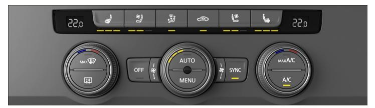
Fig. 88 In the upper section of the center console: air conditioning block for the Climatronic system (version 2).
