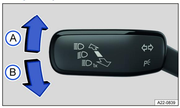
Fig. 76 On the left side of the steering column: turn signal and high beam lever.
