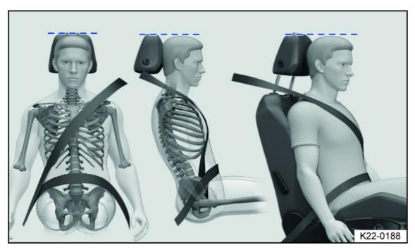
Fig. 26 Correct safety belt positioning and correct head restraint adjustment (general example).
