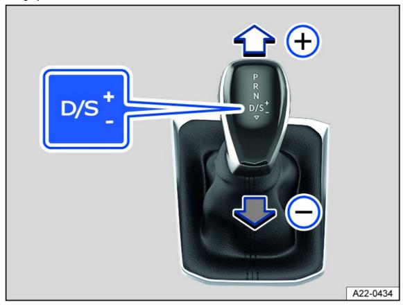
Fig. 99 In the center console: selector lever in the tiptronic position.
