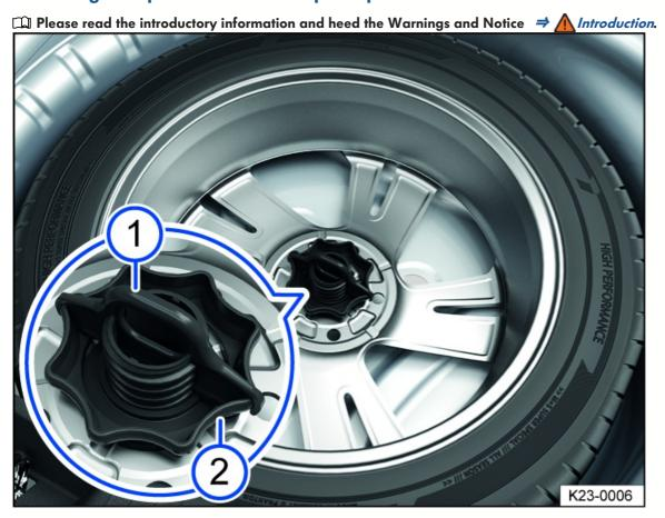
Fig. 179 Under the luggage compartment floor: handwheel to secure the spare wheel.
