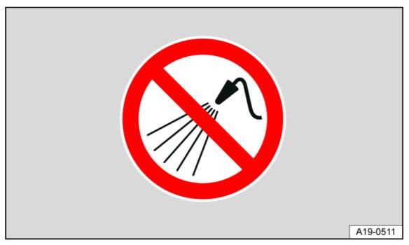
Fig. 194 In the hood space: do not use a pressure washer.
