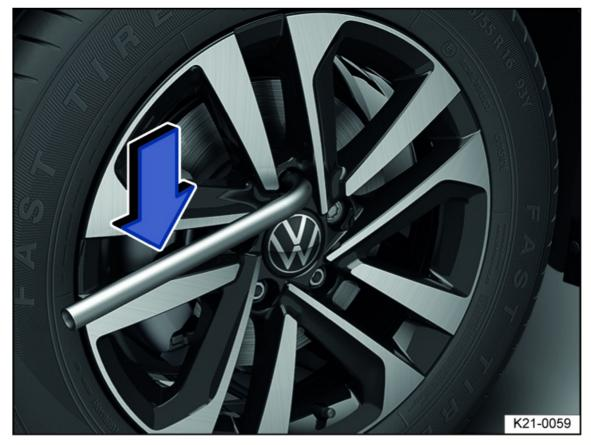
Fig. 189 Removing wheel bolts with the lug wrench.
