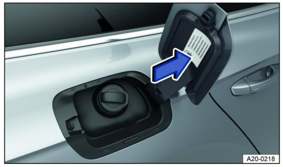
Fig. 135 On the inside of the fuel filler flap: fuel label (general example)
