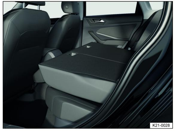
Fig. 67 Rear bench seat: Rear seat backrest folded forwards.
