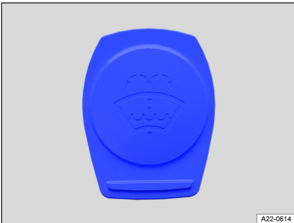
Fig. 163 In the engine compartment: Cap on the washer fluid reservoir (general example).
