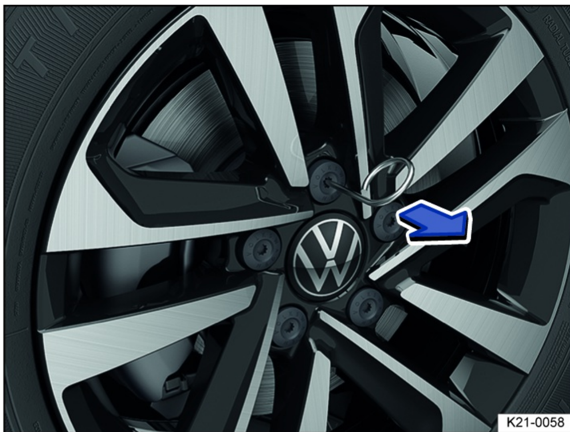
Fig. 179 Remove the caps from the wheel bolts.
