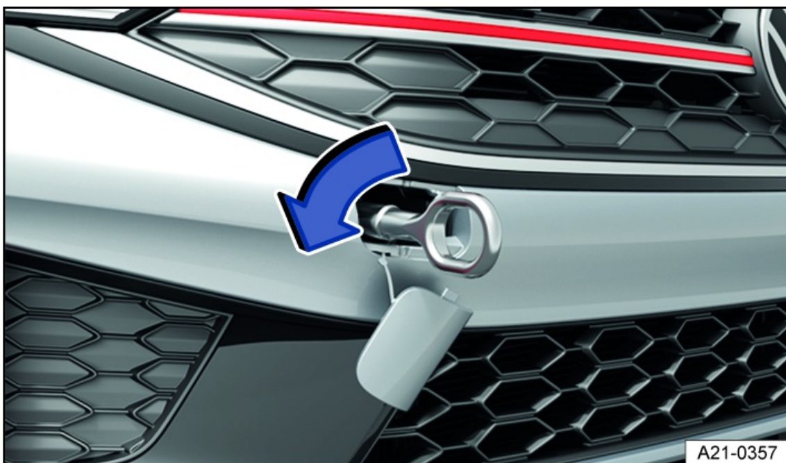
Fig. 154 In the right front bumper: Screw in the towing eye, variant 2.
