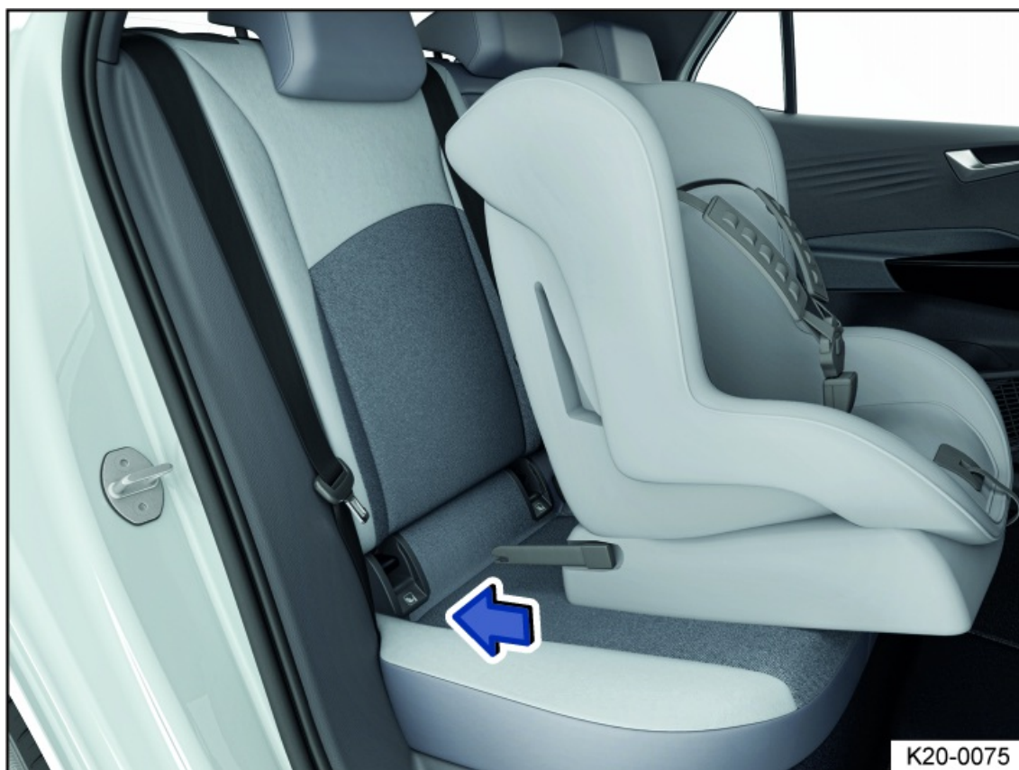
Fig. 37 Fitting a child restraint with arms (general example).
