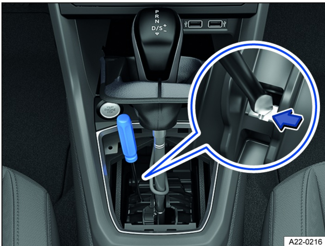
Fig. 102 In the center console: manually release the Automatic Shift Lock (ASL) (variant 1).
