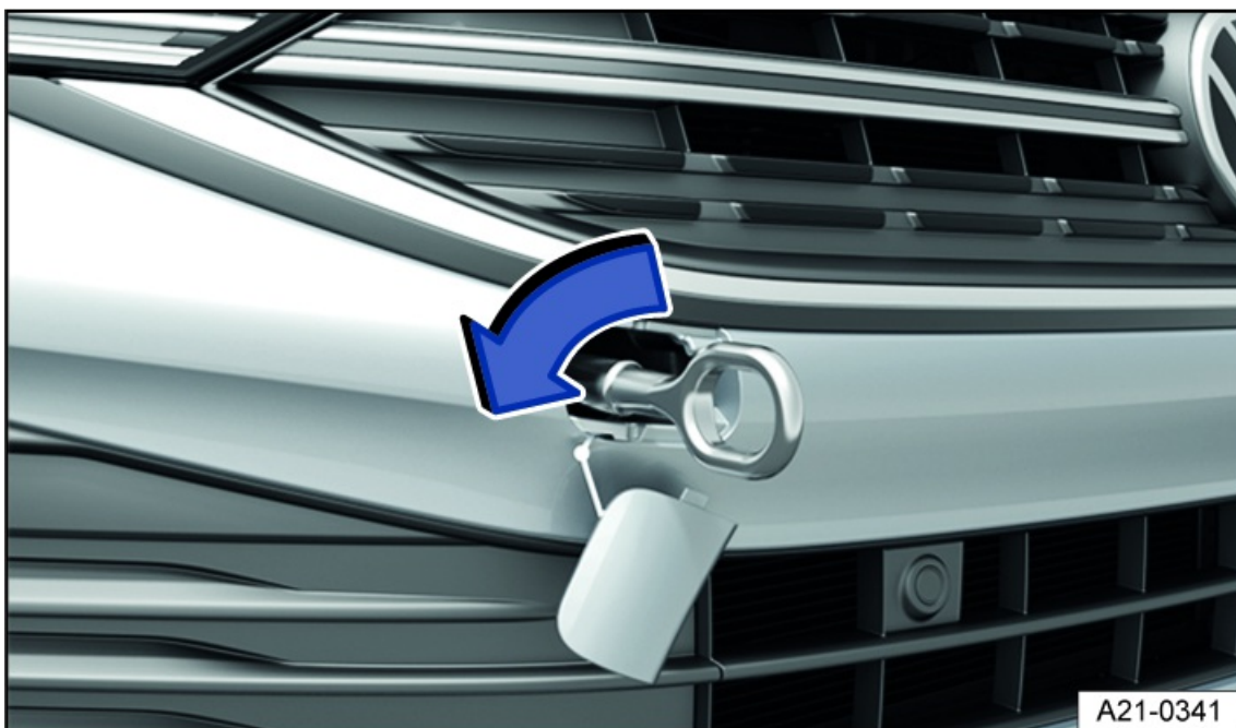
Fig. 153 In the right front bumper: Screw in the towing eye, variant 1.
