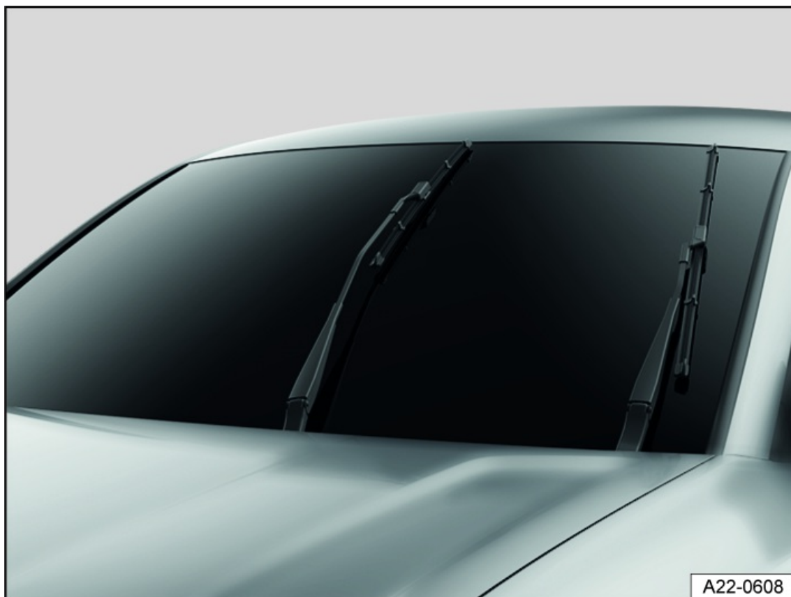
Fig. 140 Windshield wipers in service position (general example).
