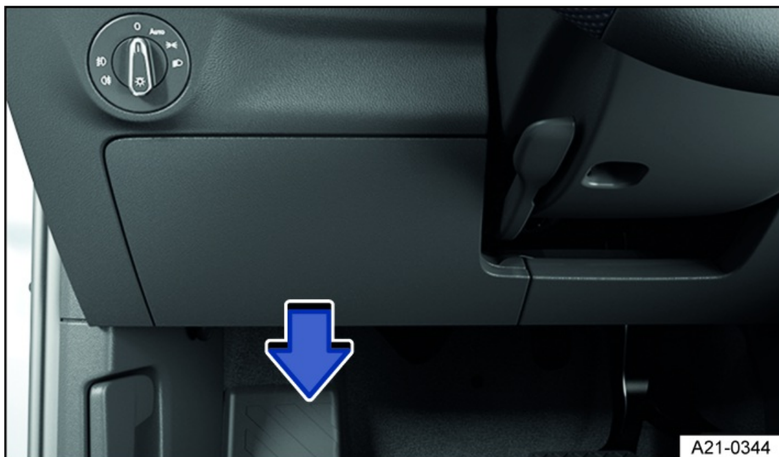
Fig. 145 Next to the steering wheel on the left: Cover for the fuse box in the dash panel.
