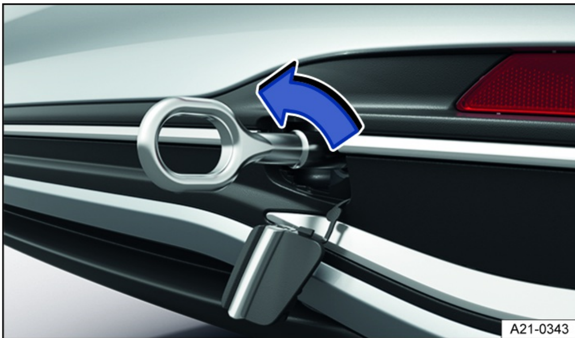
Fig. 156 In the right rear bumper: Screw in towing eye.
