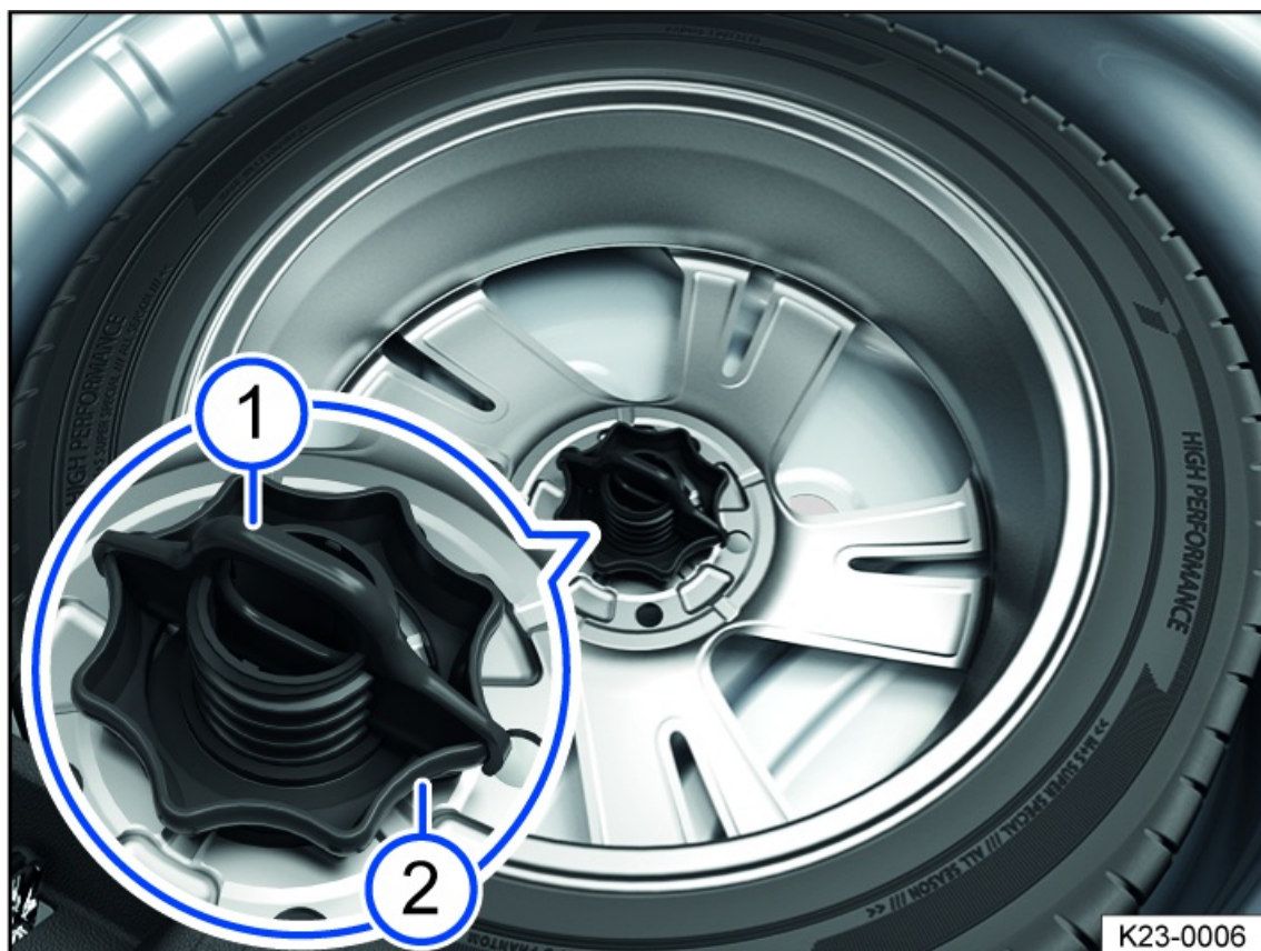
Fig. 176 Under the luggage compartment floor: handwheel to secure the spare wheel.
