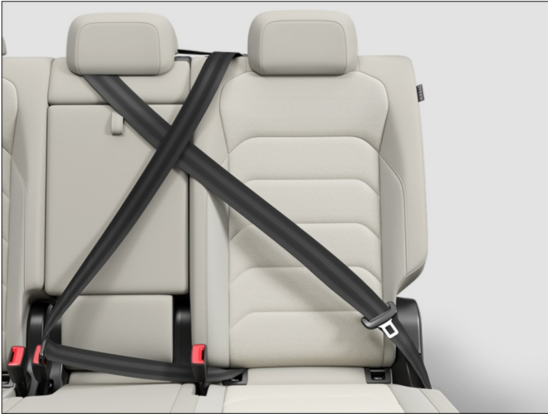
Fig. 41 Securing unused safety belts (general example).
