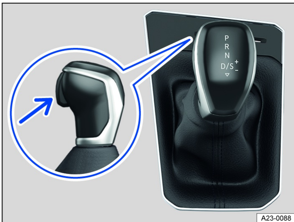
Fig. 99 In the center console: selector lever of the automatic transmission (general example).
