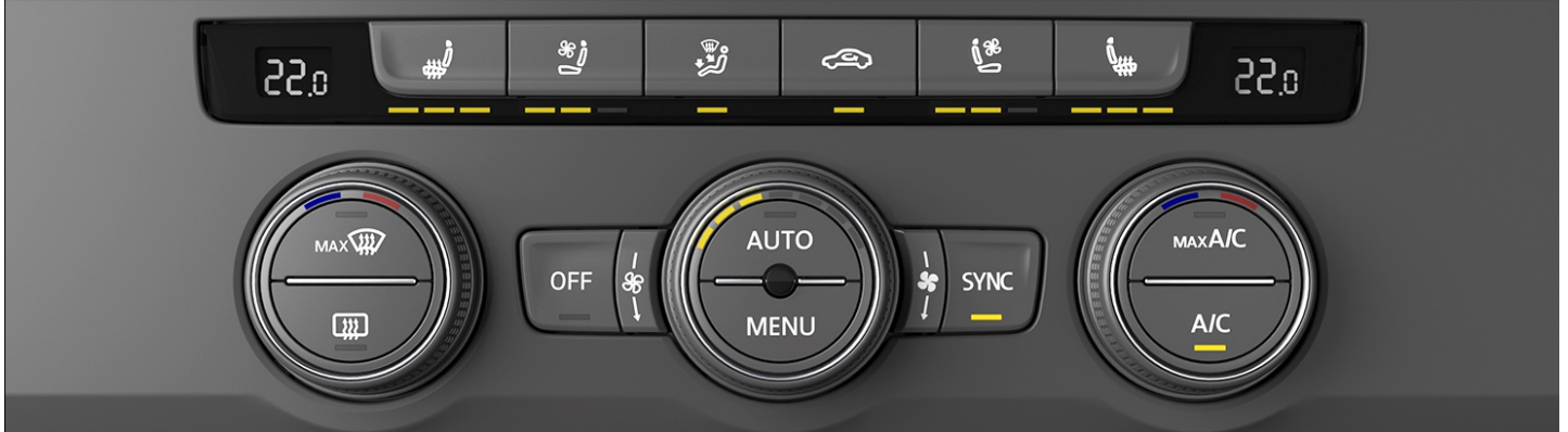
Fig. 89 In the upper section of the center console: Climate control bar for the Climatronic system.
