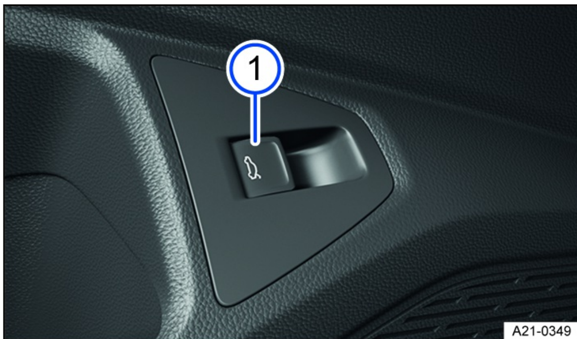
Fig. 58 In the driver's door: unlock button for the trunk lid.
