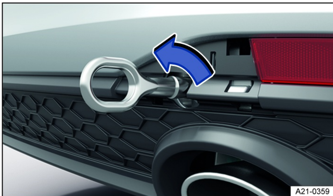
Fig. 158 In the right rear bumper: Screw in towing eye.
