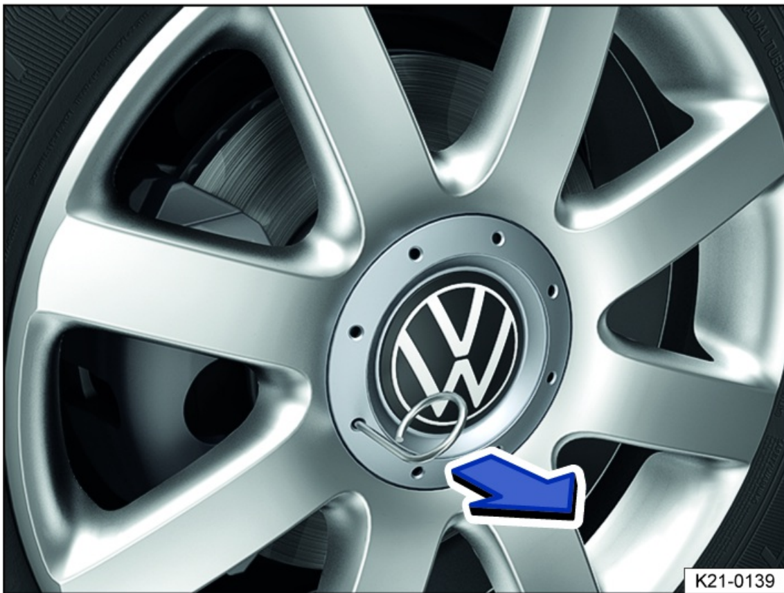
Fig. 177 Remove the hubcap.
