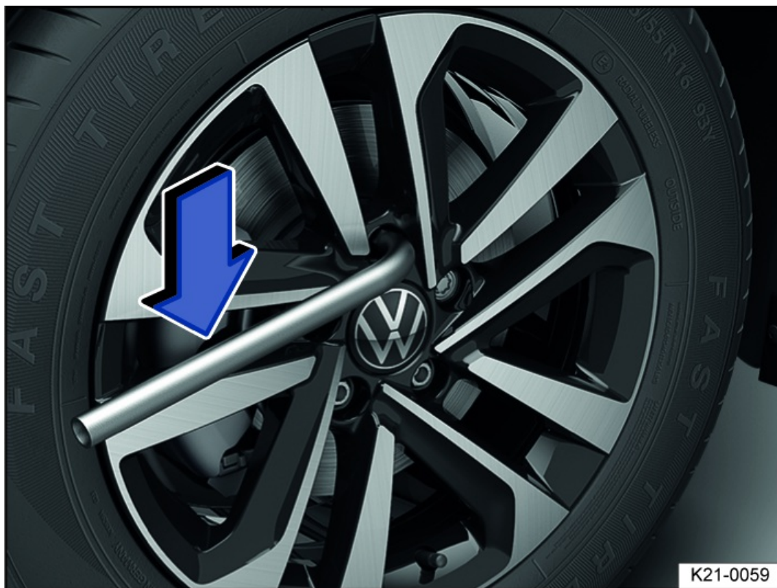
Fig. 187 Removing wheel bolts with the lug wrench.
