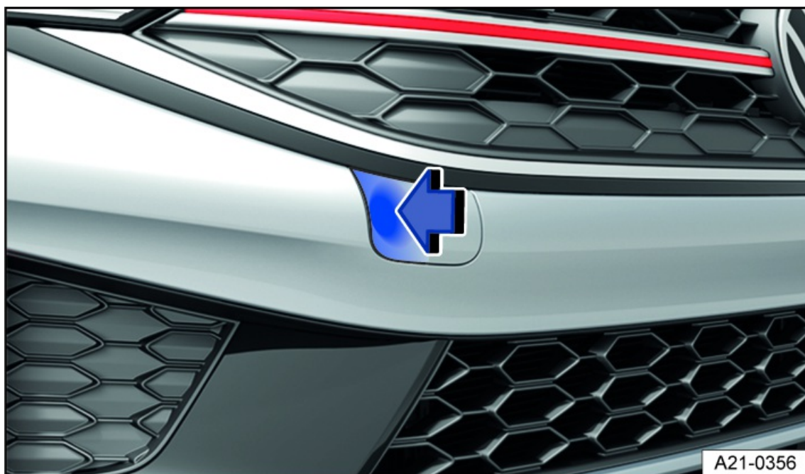
Fig. 152 In the right front bumper: Remove the cover, variant 2.
