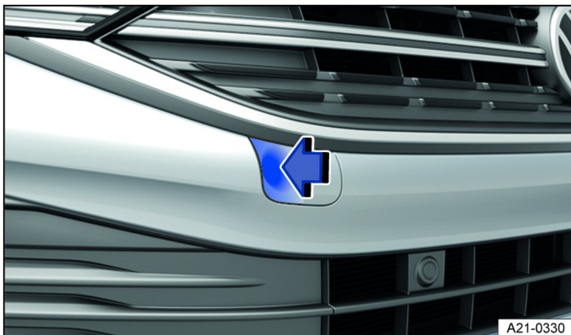
Fig. 151 In the right front bumper: Remove the cover, variant 1.
