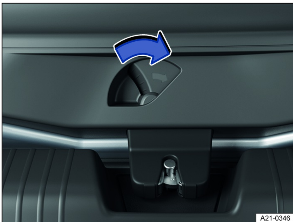
Fig. 61 In the luggage compartment: mechanically unlocking the trunk lid using the emergency release.
