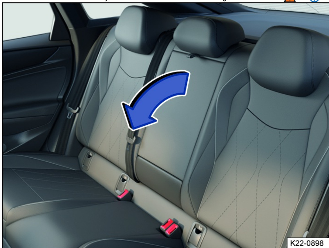
Fig. 127 In the backrest of the center seat: folding rear center armrest (general example).
