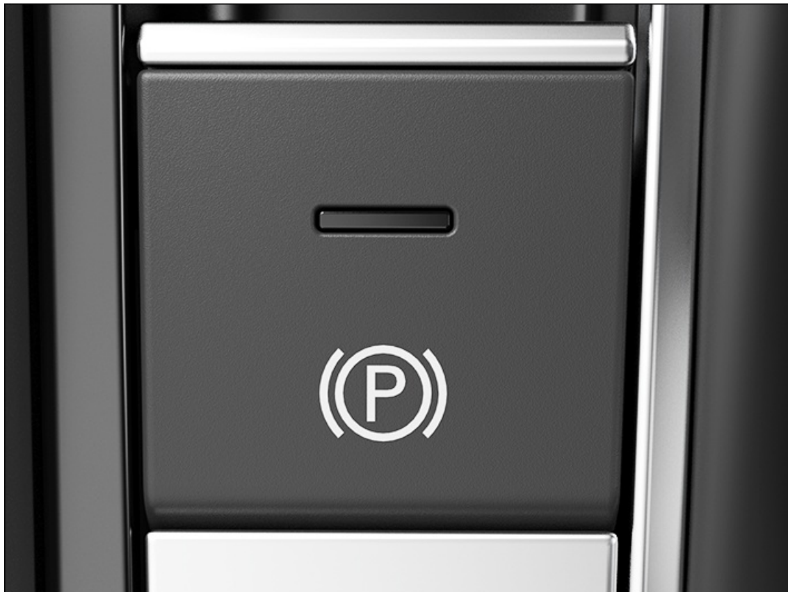
Fig. 122 In the center console: button for the electronic parking brake.
