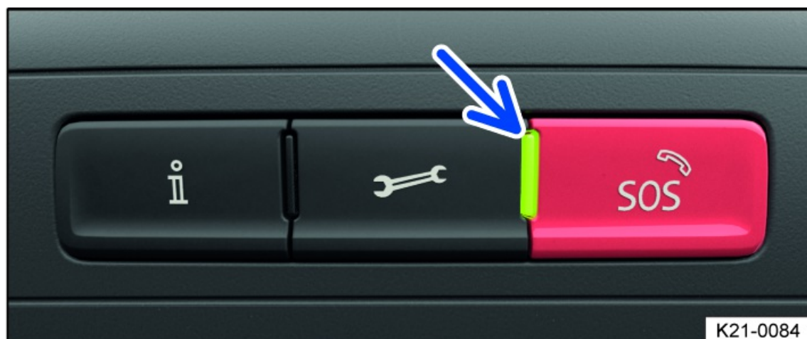
Fig. 44 In the roof console: Controls for call services and indicator light.
