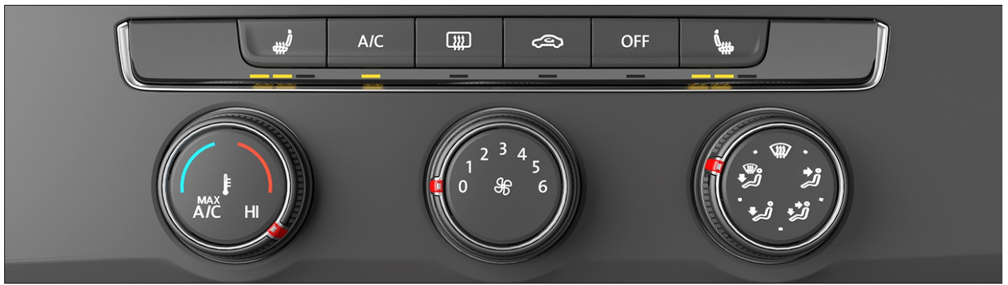
Fig. 90 In the upper section of the center console: Climate control bar for the manual climate control system.
