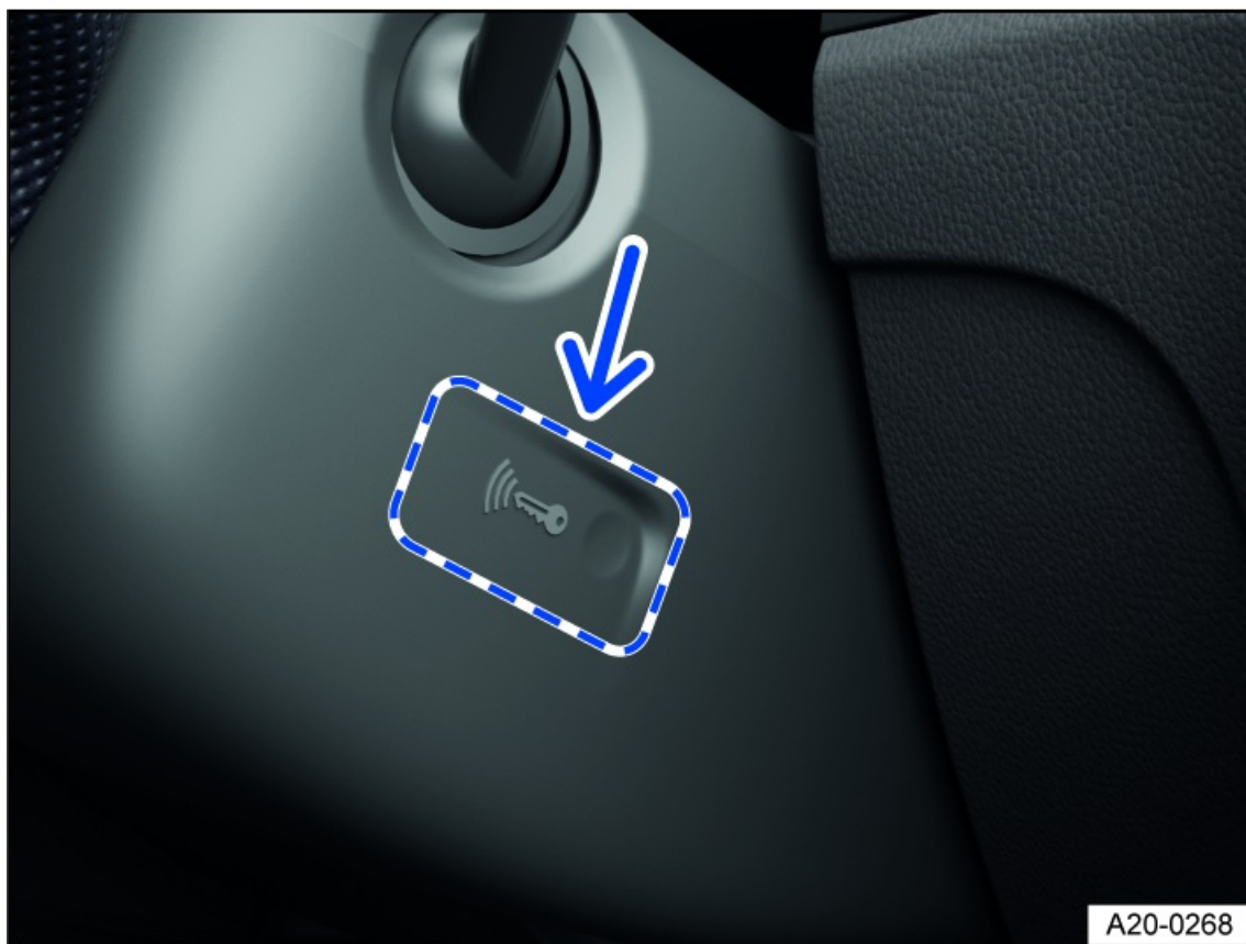
Fig. 96 On the right side of the steering column: emergency start function on vehicles with Keyless Access with push-button start.
