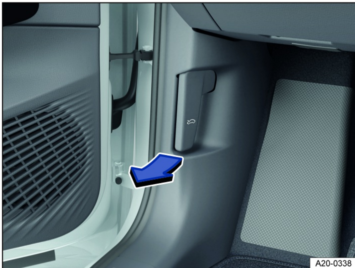
Fig. 159 In the driver's side footwell: Release lever for the hood (general example).
