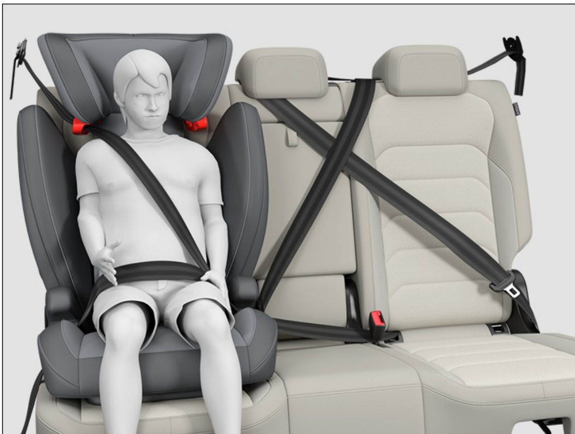
Fig. 42 Correctly fastened child on a booster seat (general example).
