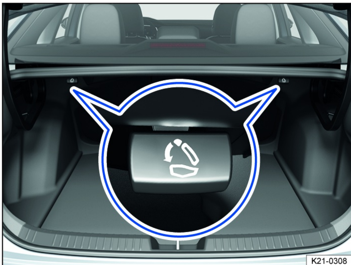
Fig. 69 In the luggage compartment: Remote release lever.
