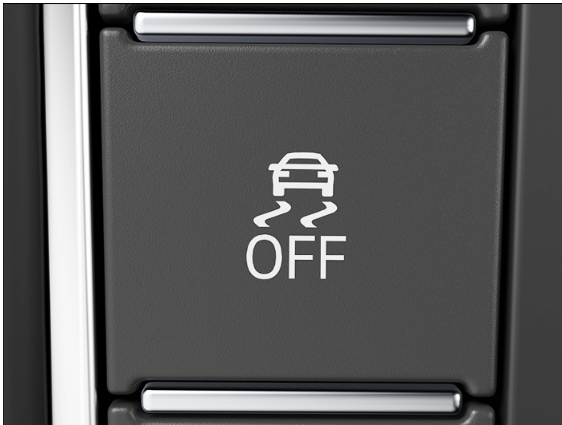
Fig. 126 Located on the center console: Button to manually switch ASR or ESC Sport on and off (depending on how your vehicle is equipped).
