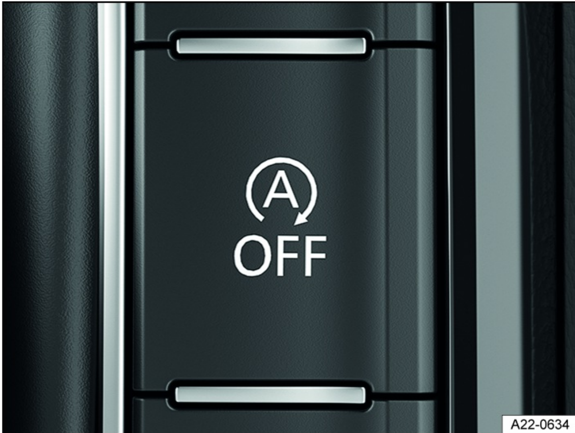
Fig. 97 In the lower section of the center console: Button for the start-stop system.
