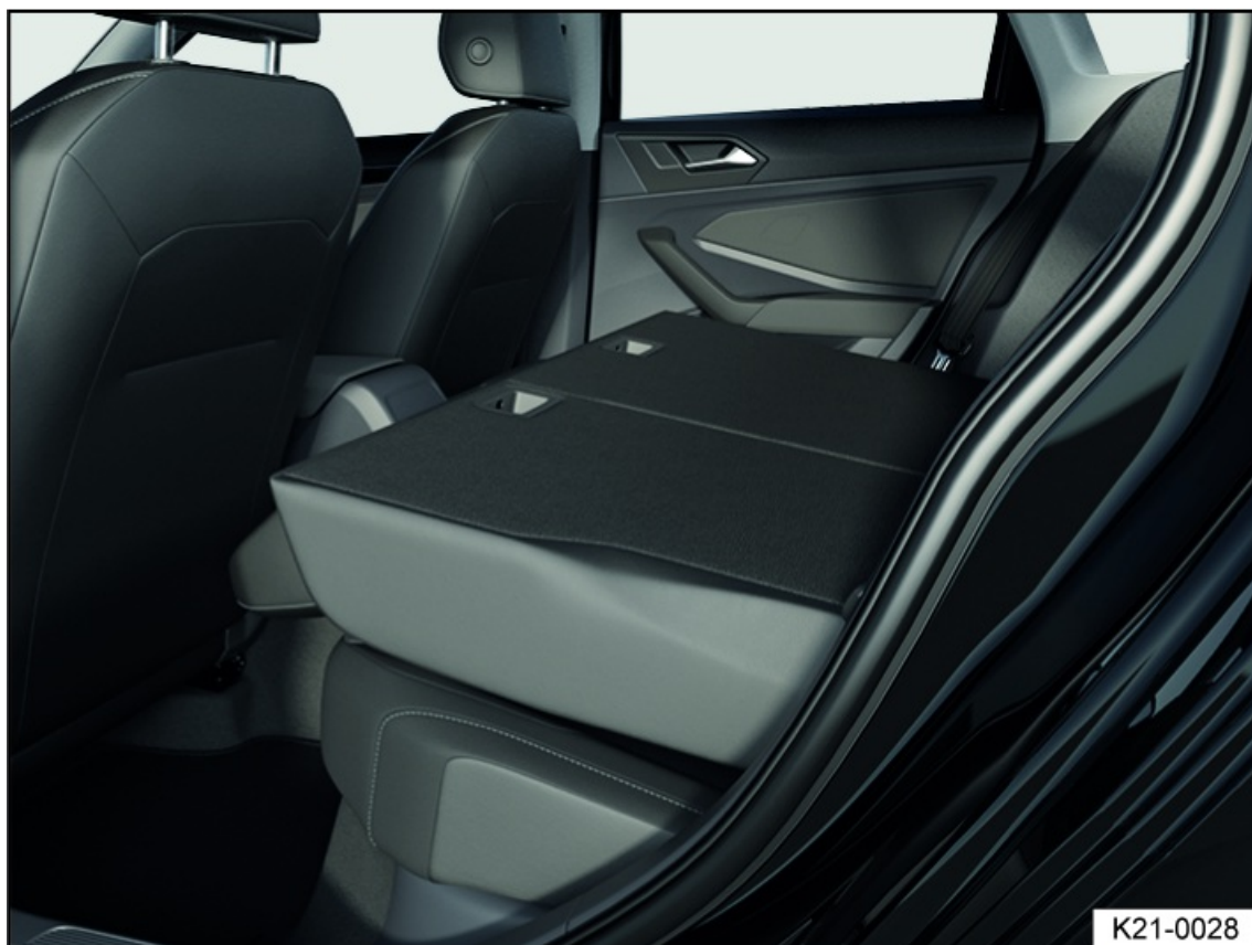
Fig. 70 Rear bench seat: Rear seat backrest folded forwards.
