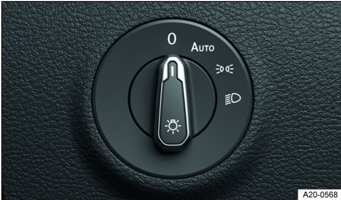
Fig. 80 Next to the steering wheel: light switch (one version).
