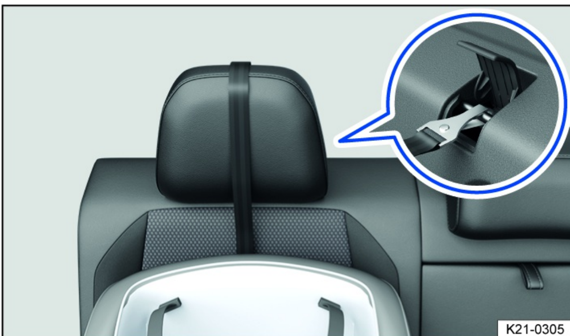
Fig. 39 On the rear seat backrest: Safety belt routing for non-adjustable head restraints with a top tether individual belt.
