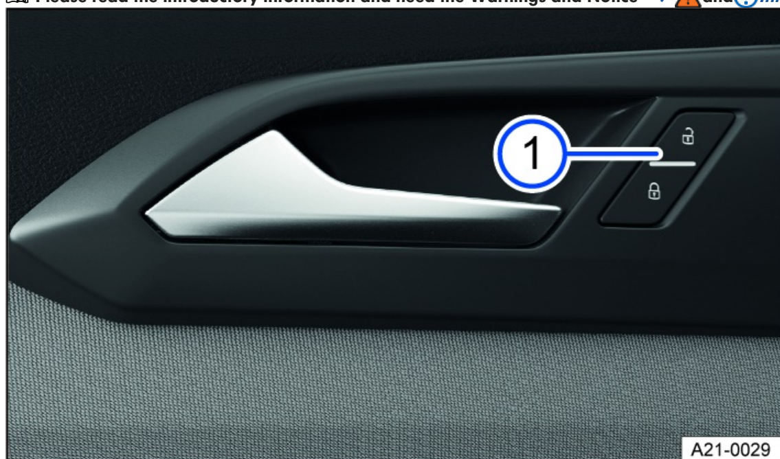
Fig. 54 In the driver's door: Central locking button (general example).
