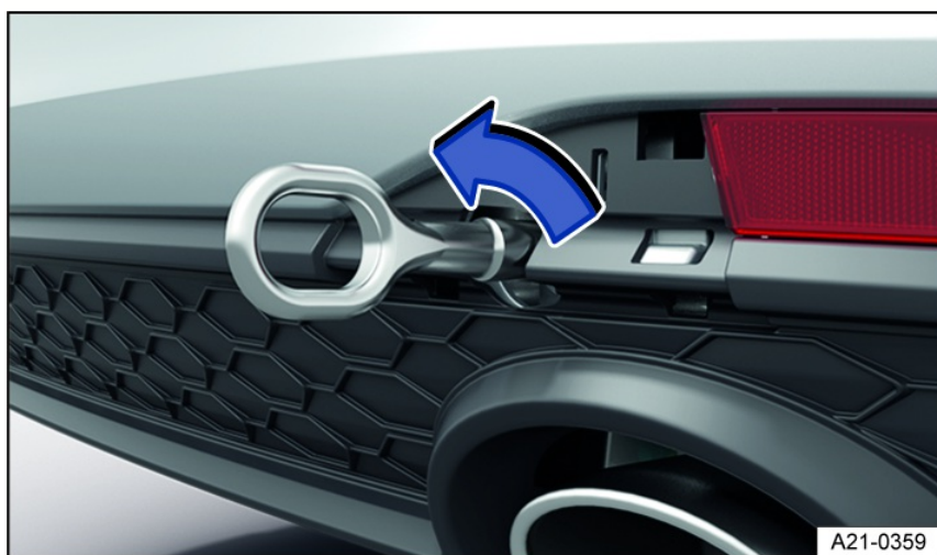
Fig. 155 In the right rear bumper: Screw in towing eye, variant 2.
