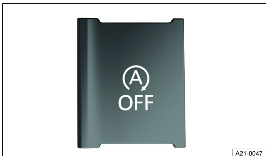
Fig. 96 In the lower section of the center console: Button for the start-stop system.
