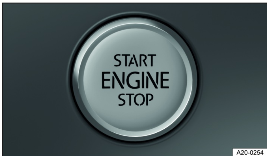
Fig. 94 In the lower area of the center console: starter button for starting the engine.
