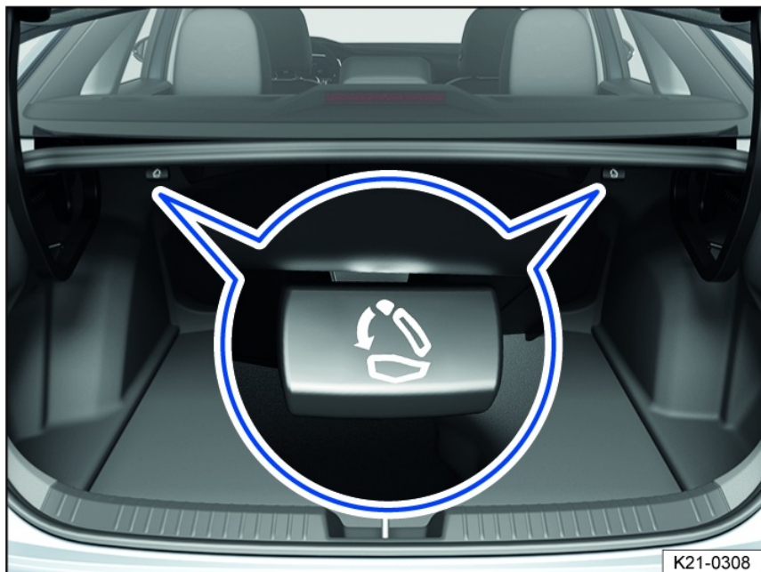
Fig. 69 In the luggage compartment: Remote release lever.
