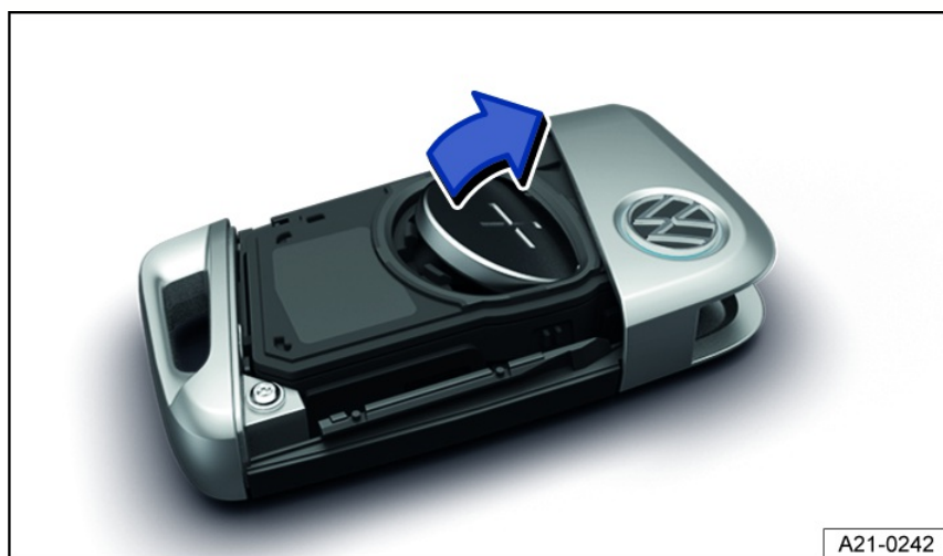
Fig. 51 Vehicle key: replacing the button cell battery
