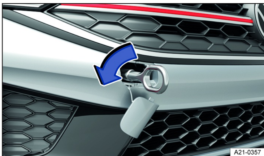
Fig. 151 In the right front bumper: Screw in the towing eye, variant 2.
