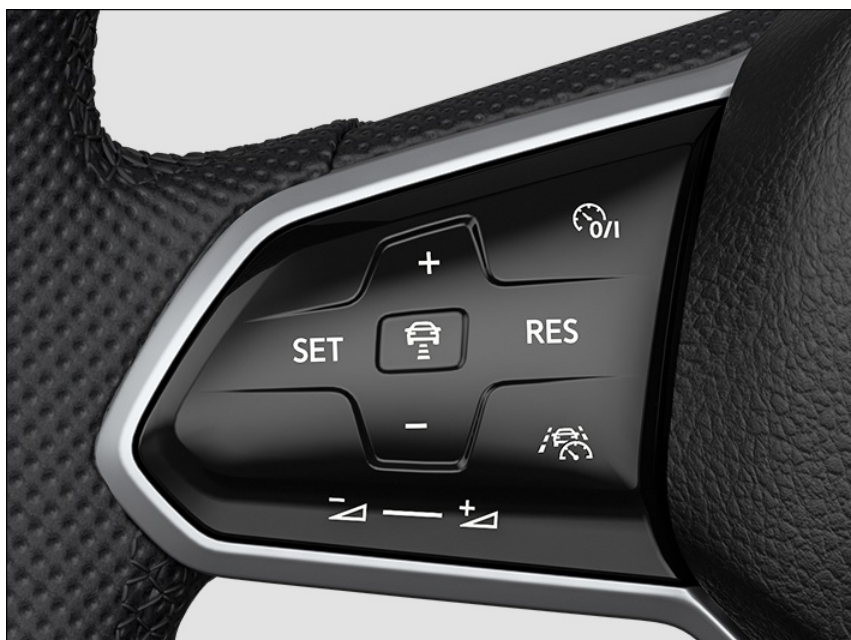
Fig. 119 Left side of the multi-function steering wheel (variant 2).
