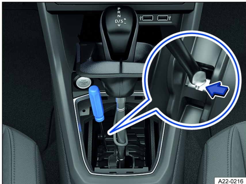
Fig. 101 In the center console: manually release the Automatic Shift Lock (ASL) (variant 1).
