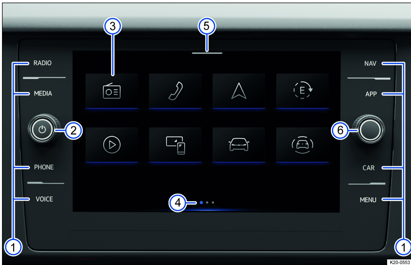
Fig. 129 Overview: display and control unit, 8" version.
