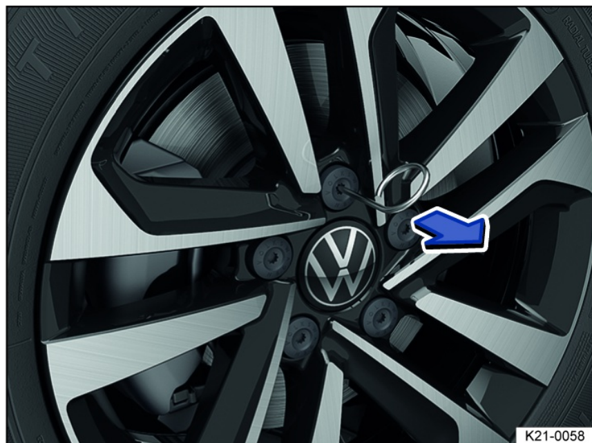
Fig. 174 Remove the caps from the wheel bolts.
