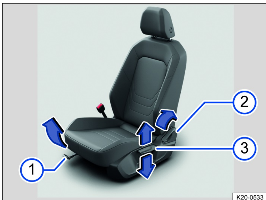
Fig. 66 On the driver seat: Controls.
