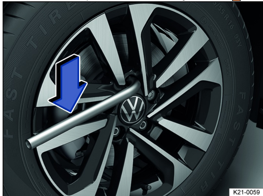
Fig. 175 Changing a tire: loosening the wheel bolts.
