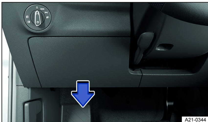
Fig. 142 Next to the steering wheel on the left: Cover for the fuse box in the dash panel.
