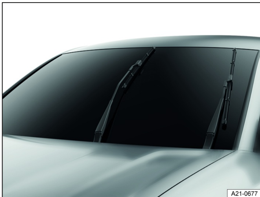
Fig. 137 Windshield wipers in service position (general example).
