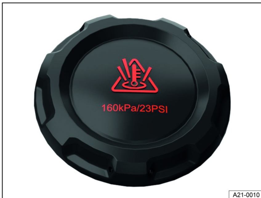
Fig. 163 In the engine compartment: cap on the engine coolant expansion tank.
