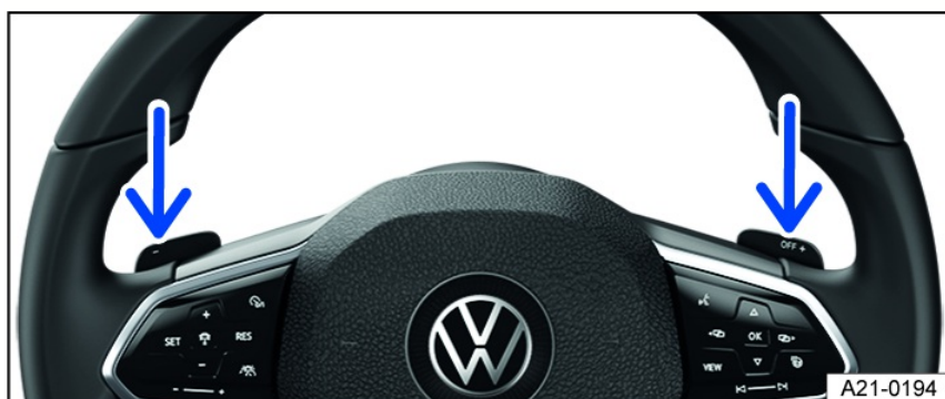
Fig. 100 Steering wheel with shift paddles for Tiptronic.
