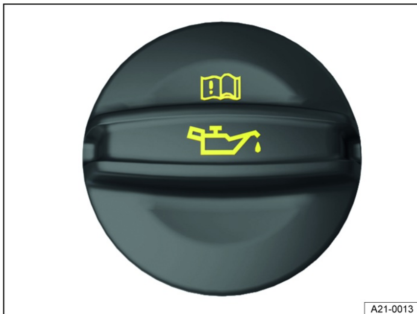
Fig. 161 In the engine compartment: engine oil filler cap (general example).
