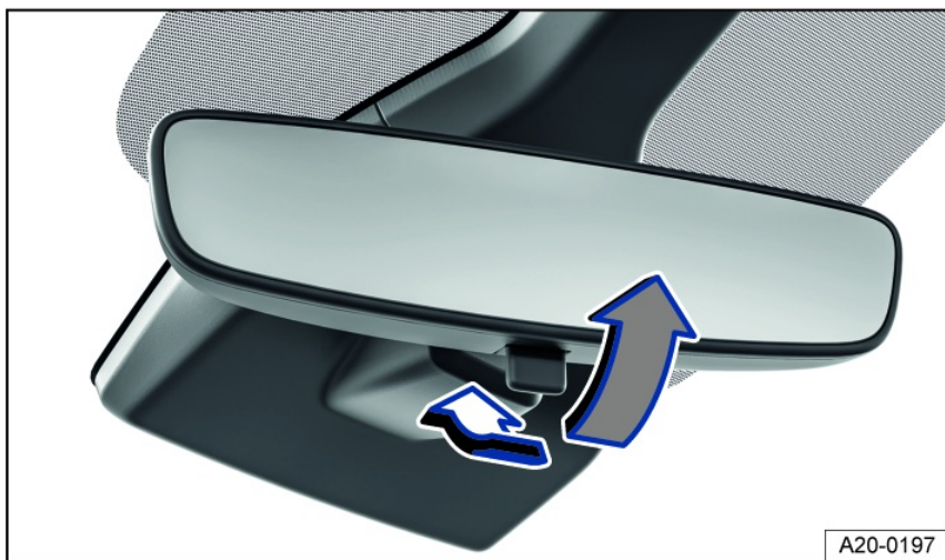
Fig. 85 On the windshield: manual dimming interior rearview mirror.
