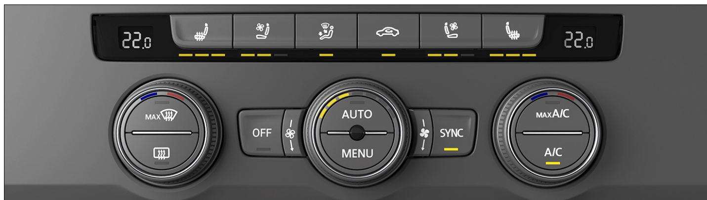
Fig. 88 In the upper section of the center console: Climate control bar for the Climatronic system.
