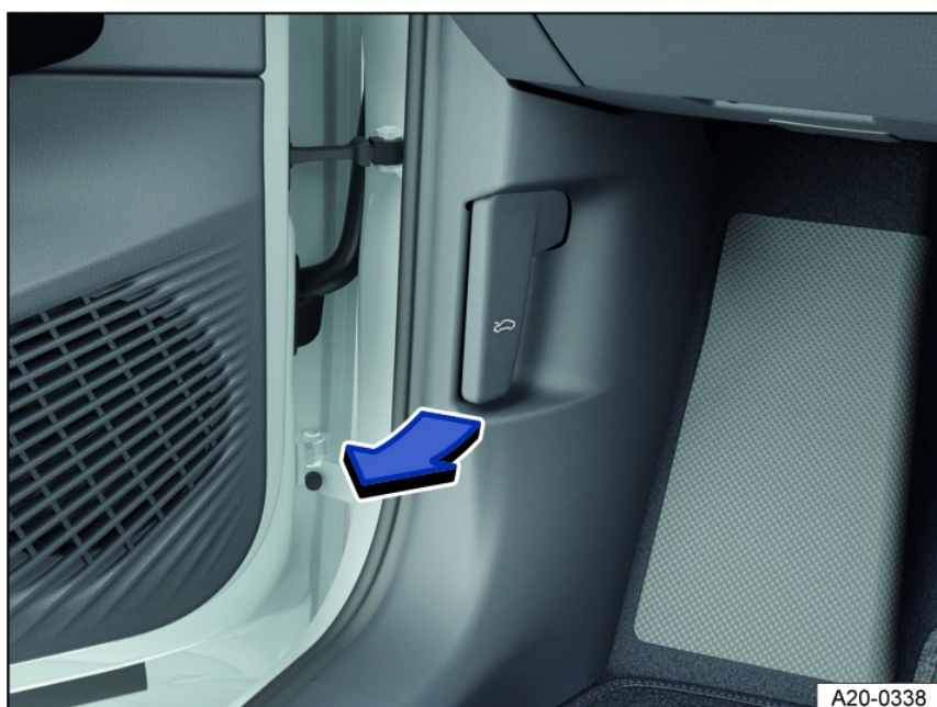
Fig. 156 In the driver's side footwell: Release lever for the hood (general example).
