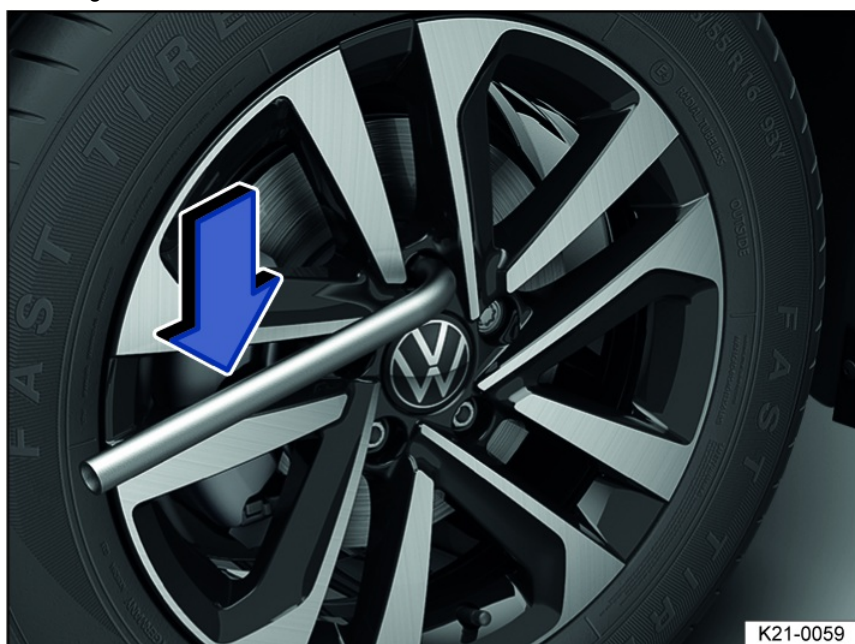
Fig. 182 Wheel change: removing wheel bolts with the lug wrench.
