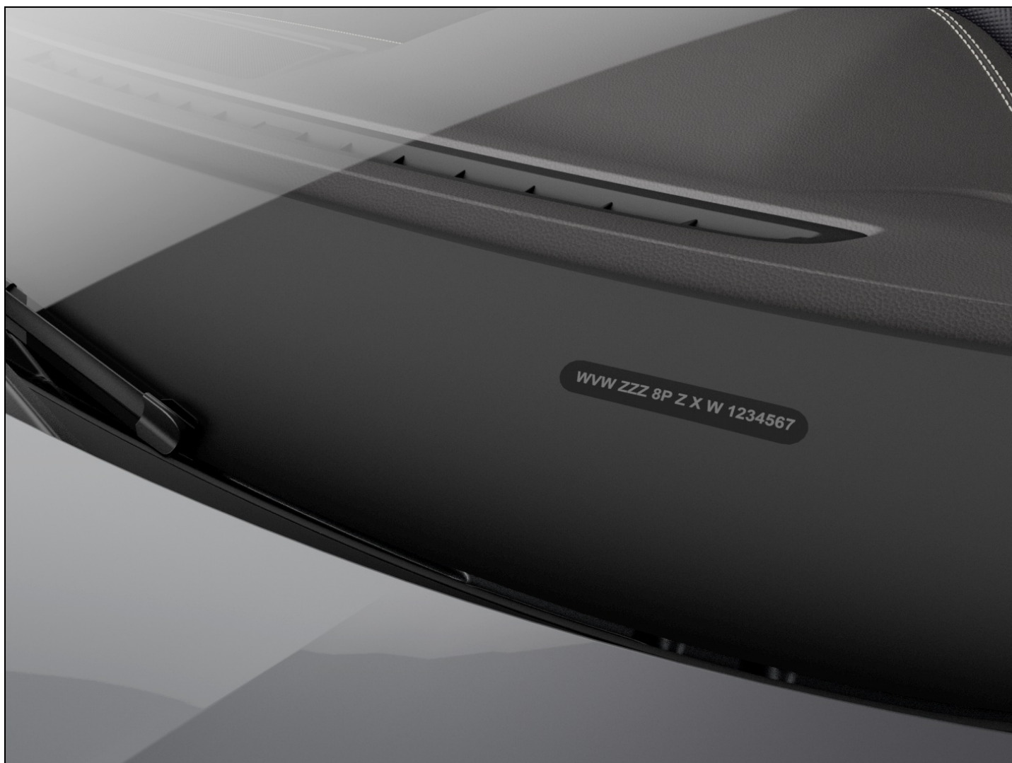
Fig. 191 In the windshield: vehicle identification number (VIN)
