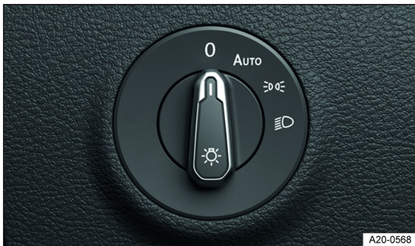
Fig. 80 Next to the steering wheel: light switch (one version).
