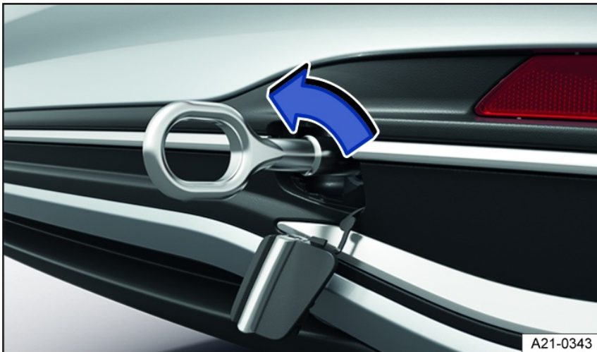
Fig. 153 In the right rear bumper: Screw in towing eye, variant 1.
