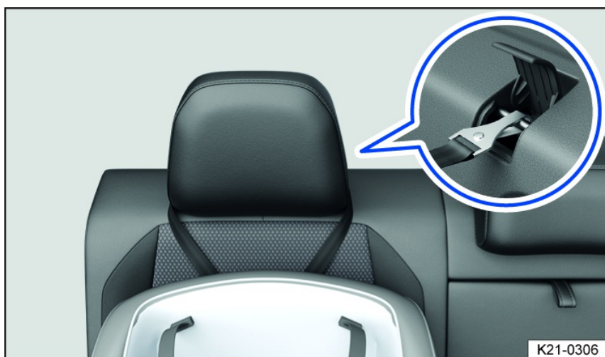
Fig. 40 On the rear seat backrest: Safety belt routing for non-adjustable head restraints with a V-shaped top tether safety belt.
