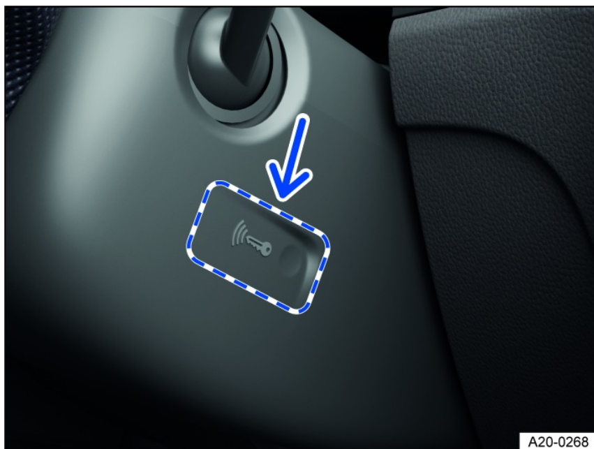
Fig. 95 On the right side of the steering column: emergency start function on vehicles with Keyless Access with push-button start.
