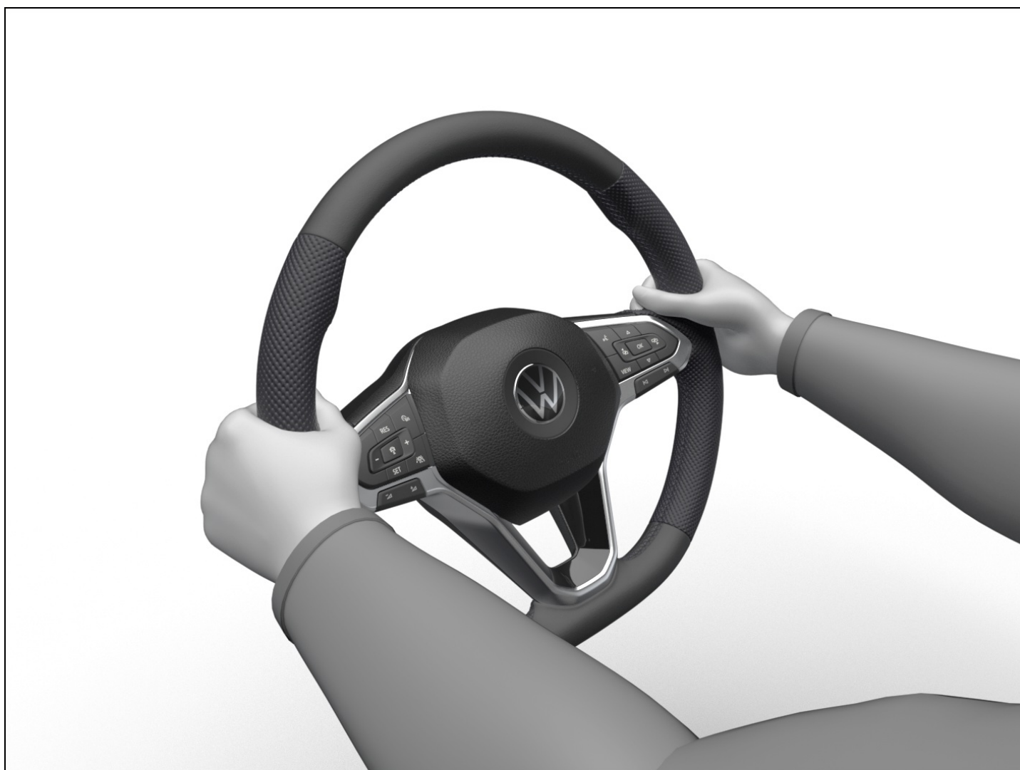
Fig. 65 On the steering wheel: nine o'clock and three o'clock position.
