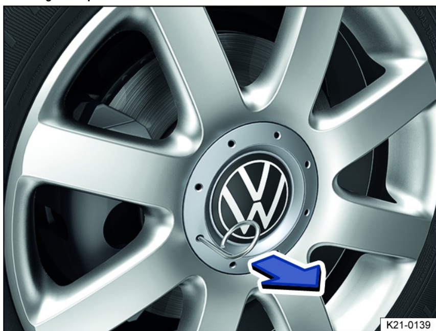
Fig. 172 Remove the hubcap.
