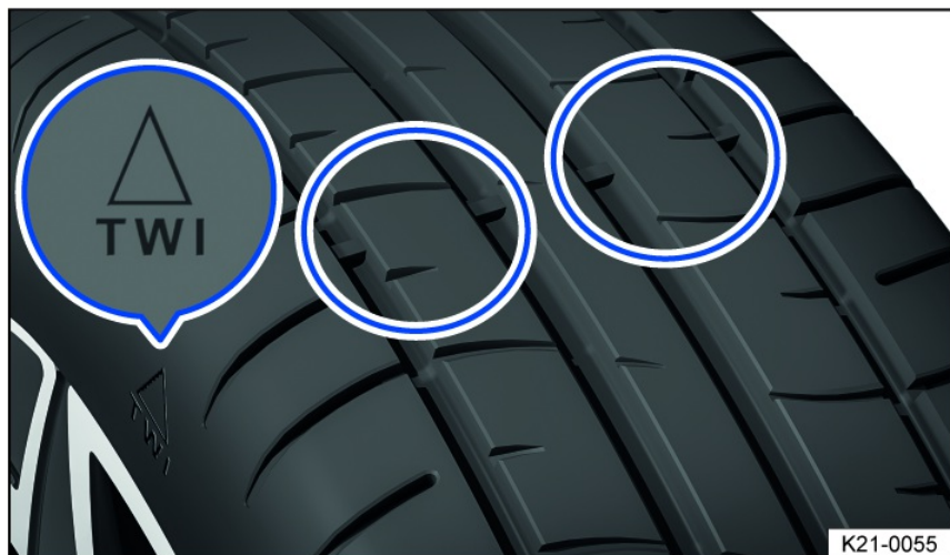
Fig. 169 Tire tread: tread wear indicator.
