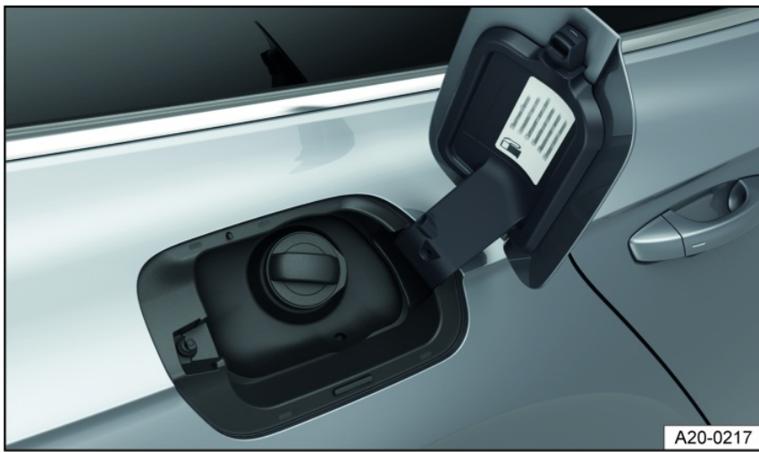
Fig. 134 Behind the fuel filler flap: fuel tank cap (general example)
