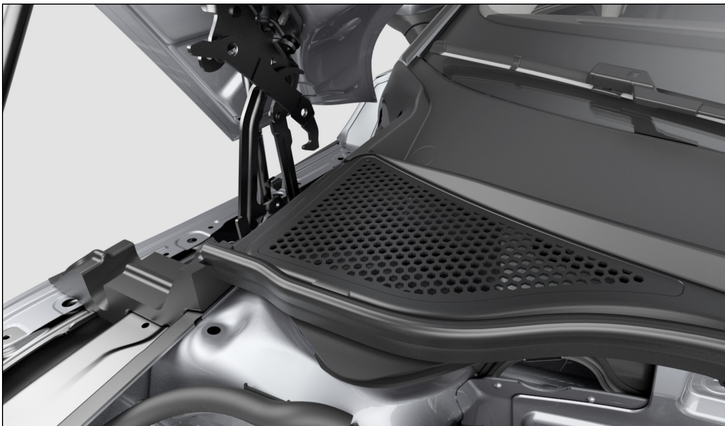
Fig. 186 Between the engine compartment and windshield: plenum chamber (general example).
