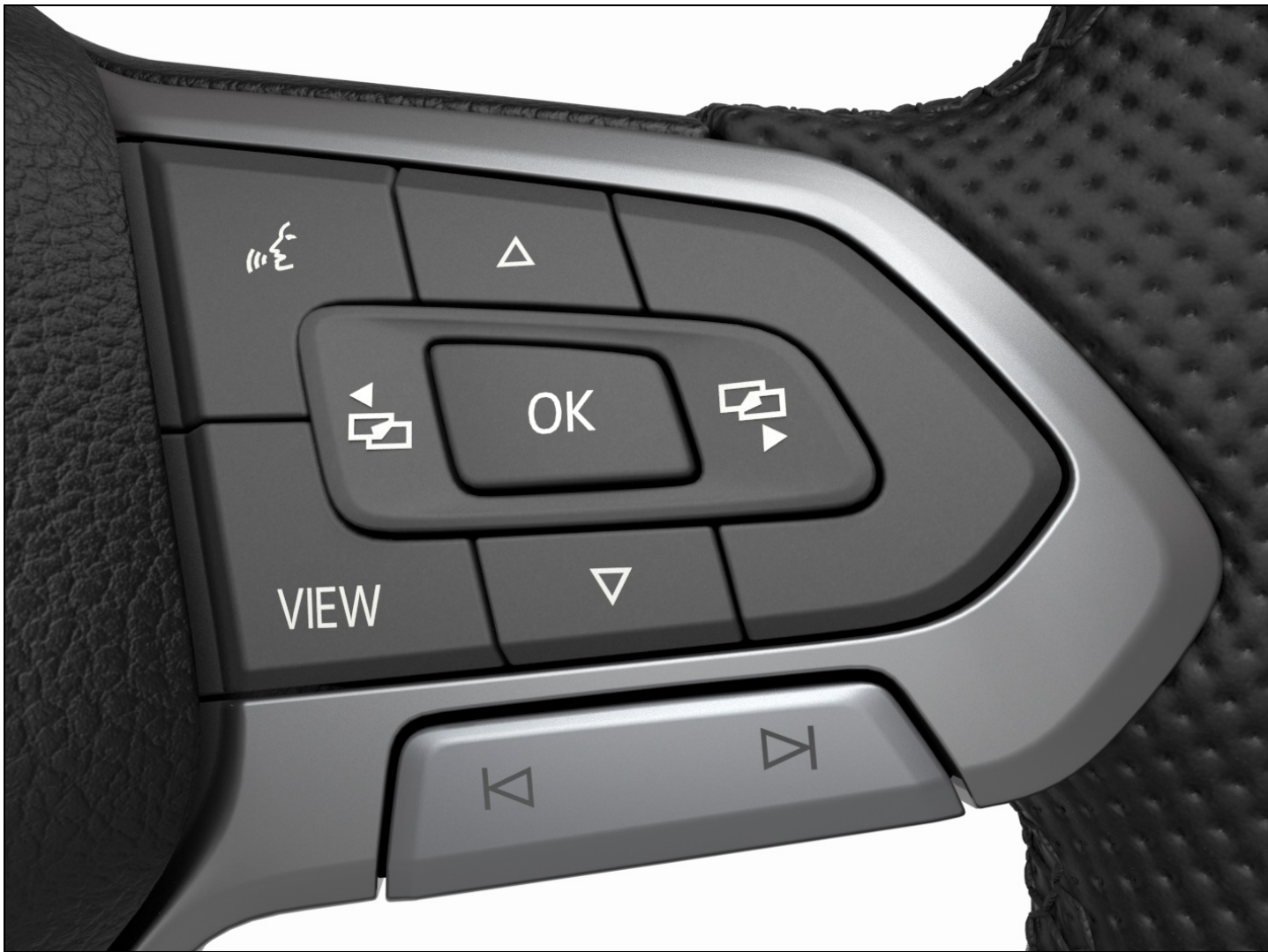
Fig. 13 Right side of the multi-function steering wheel: Operating the Volkswagen Digital Cockpit Basic (variant 1).
