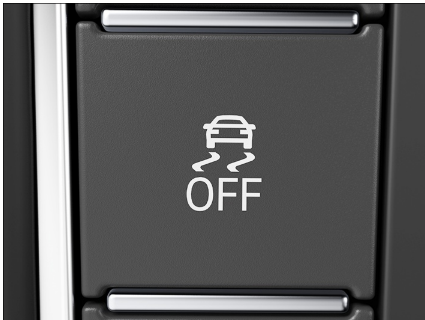
Fig. 125 Located on the center console: Button to manually switch ASR or ESC Sport on and off (depending on how your vehicle is equipped).
