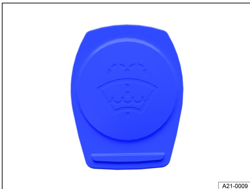
Fig. 160 In the engine compartment: Cap on the washer fluid reservoir (general example).
