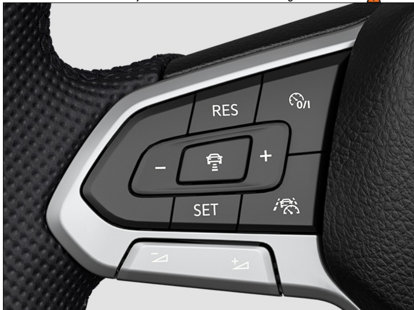
Fig. 118 Left side of the multi-function steering wheel (variant 1).
