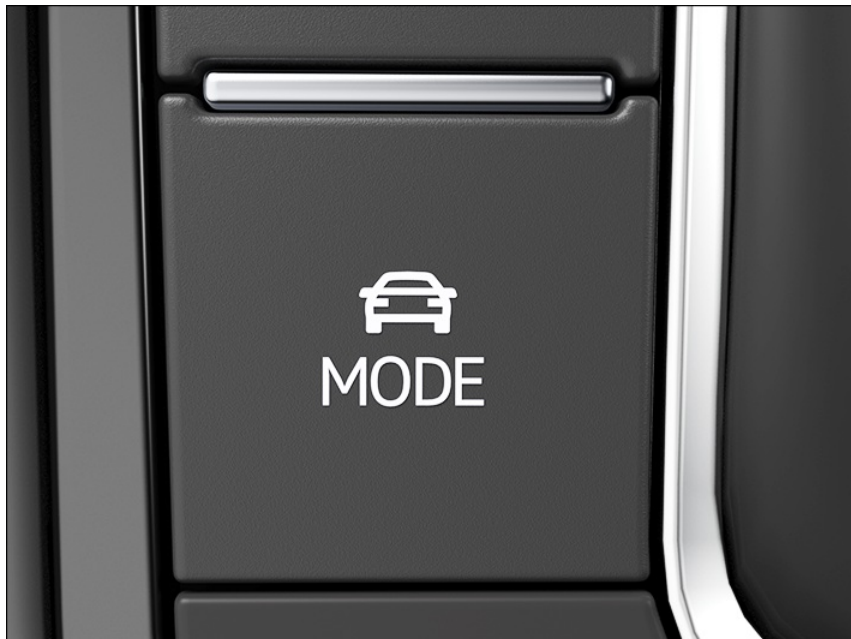
Fig. 105 In the center armrest: Driving Mode Selection MODE button.
