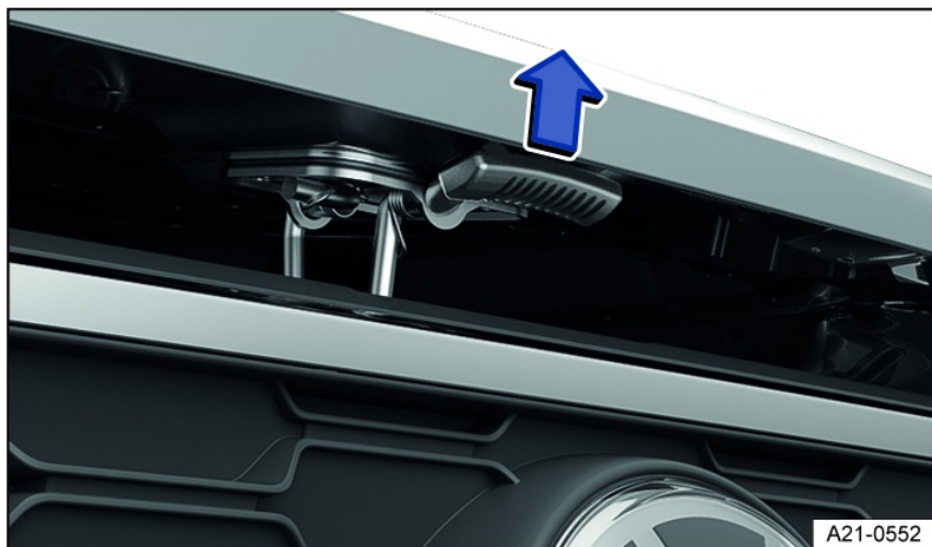
Fig. 157 Above the radiator grille: Opening lever for the hood (general example).
