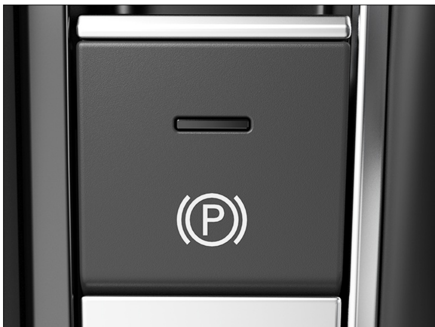
Fig. 121 In the center console: button for the electronic parking brake.
