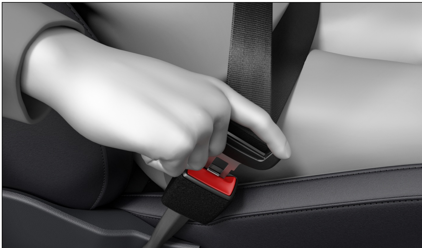
Fig. 24 Inserting the buckle tongue into the safety belt buckle.
