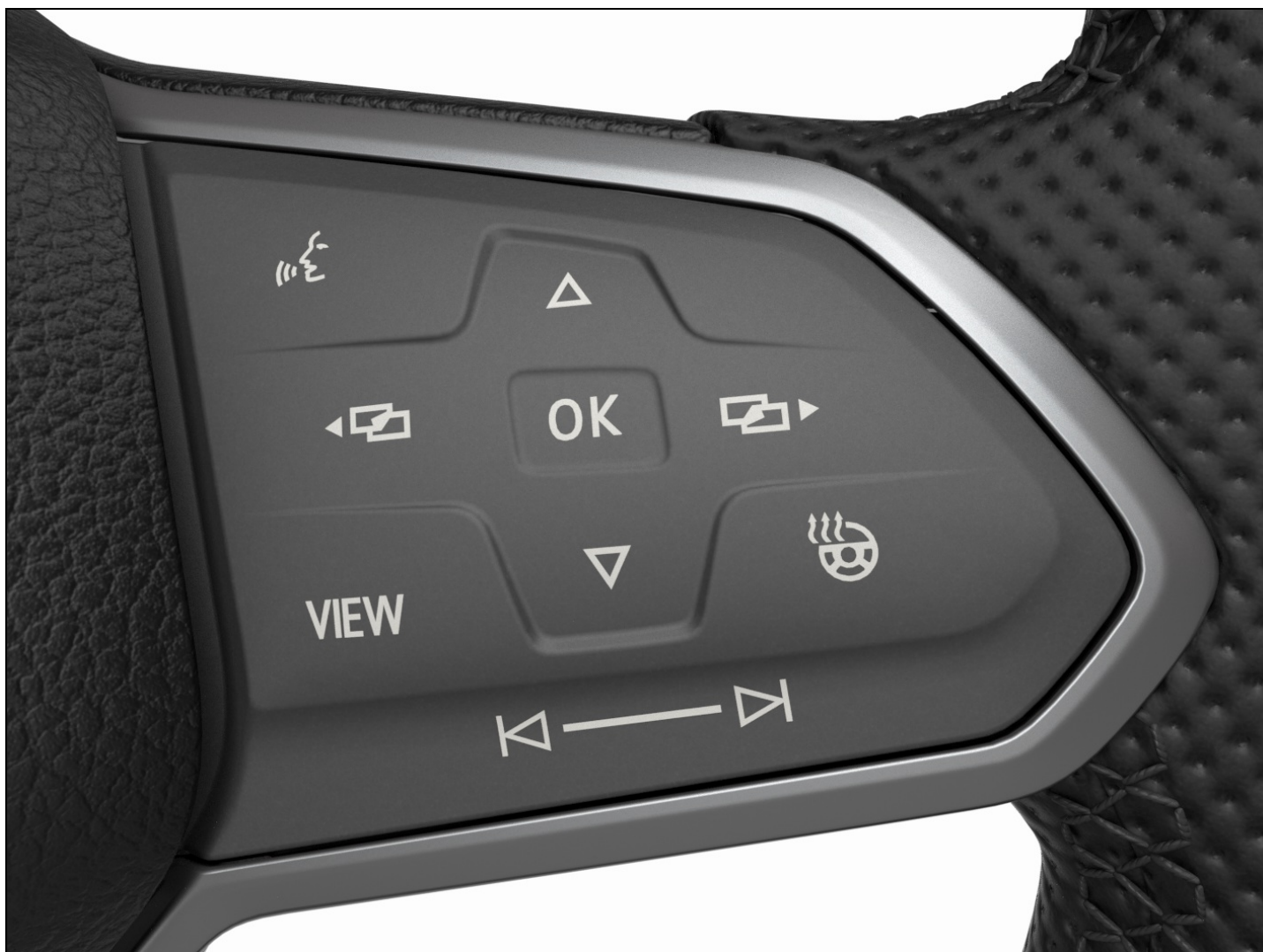
Fig. 14 Right side of the multi-function steering wheel: Operating the Volkswagen Digital Cockpit Basic (variant 2).
