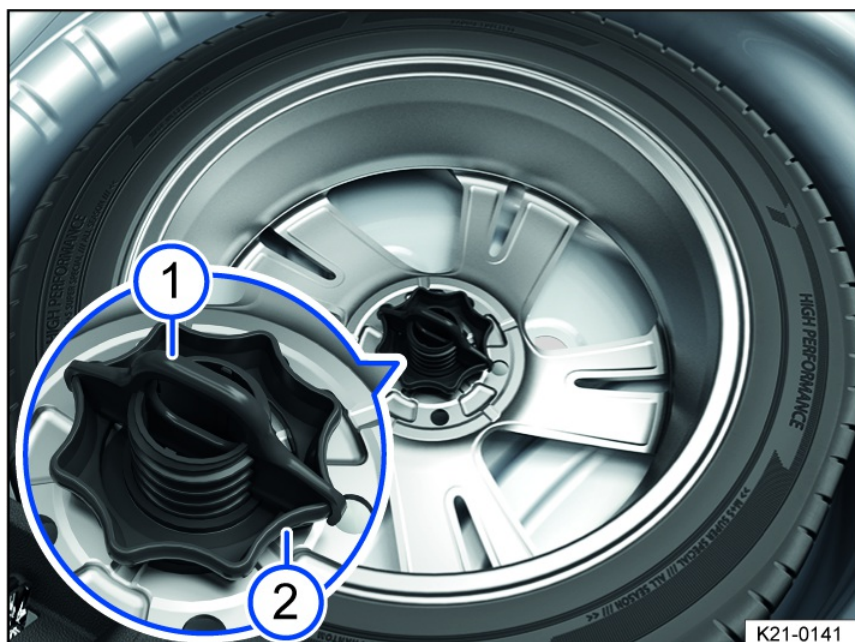
Fig. 171 In the luggage compartment: handle to secure the compact spare wheel.
