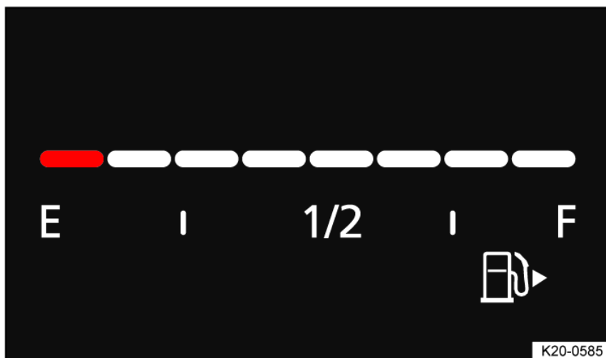
Fig. 16 Fuel gauge on the Volkswagen Digital Cockpit Basic (general example).
