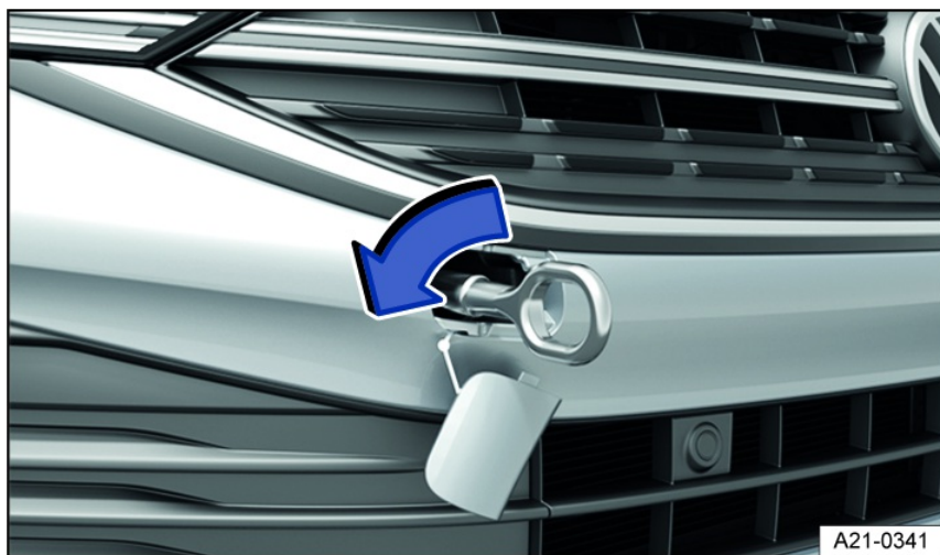
Fig. 150 In the right front bumper: Screw in the towing eye, variant 1.
