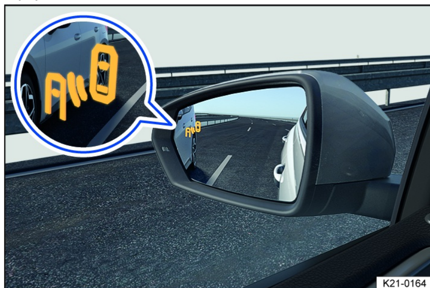
Fig. 120 In the mirror glass of the outside mirrors: Blind Spot Monitor indicator.
