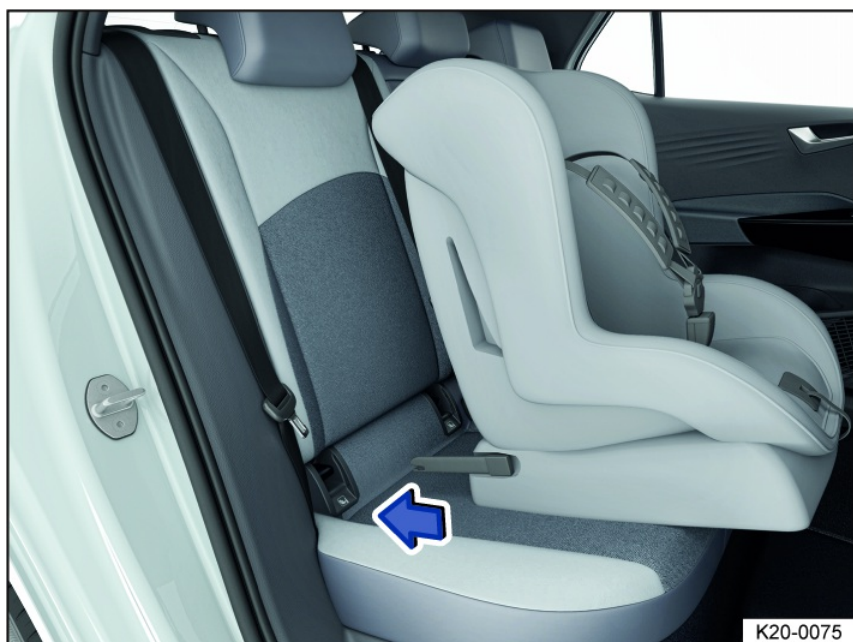
Fig. 37 General example: fitting a child restraint with attachment arms.
