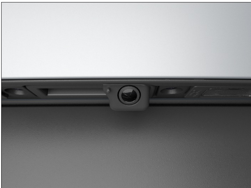
Fig. 187 In the rear of the vehicle: Rear View Camera system on the handle (general example).
