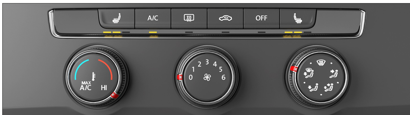
Fig. 89 In the upper section of the center console: Climate control bar for the manual climate control system.
