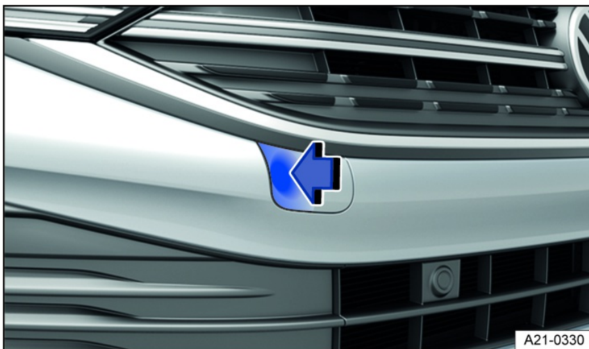
Fig. 148 In the right front bumper: Remove the cover, variant 1.
