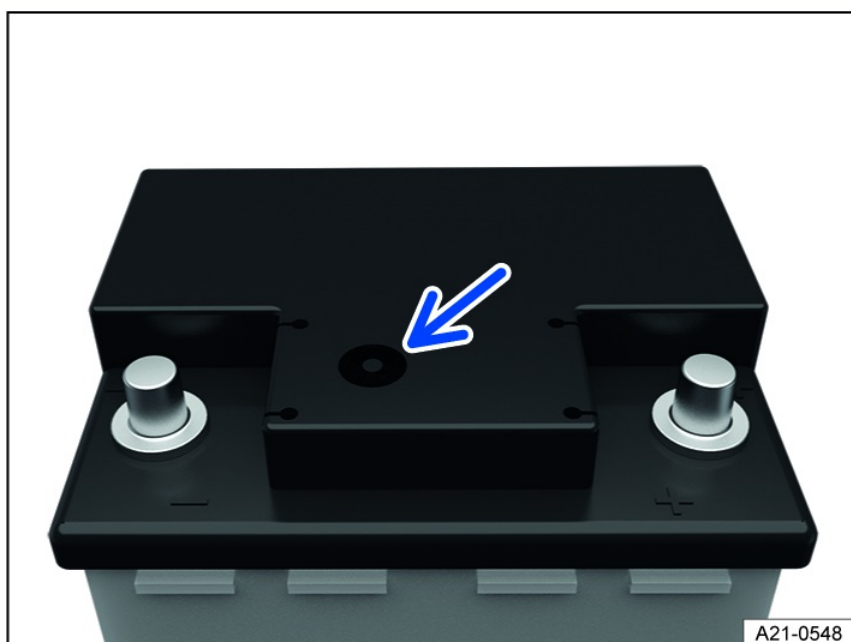
Fig. 166 On the top of the 12 V vehicle battery: Window (general example).
