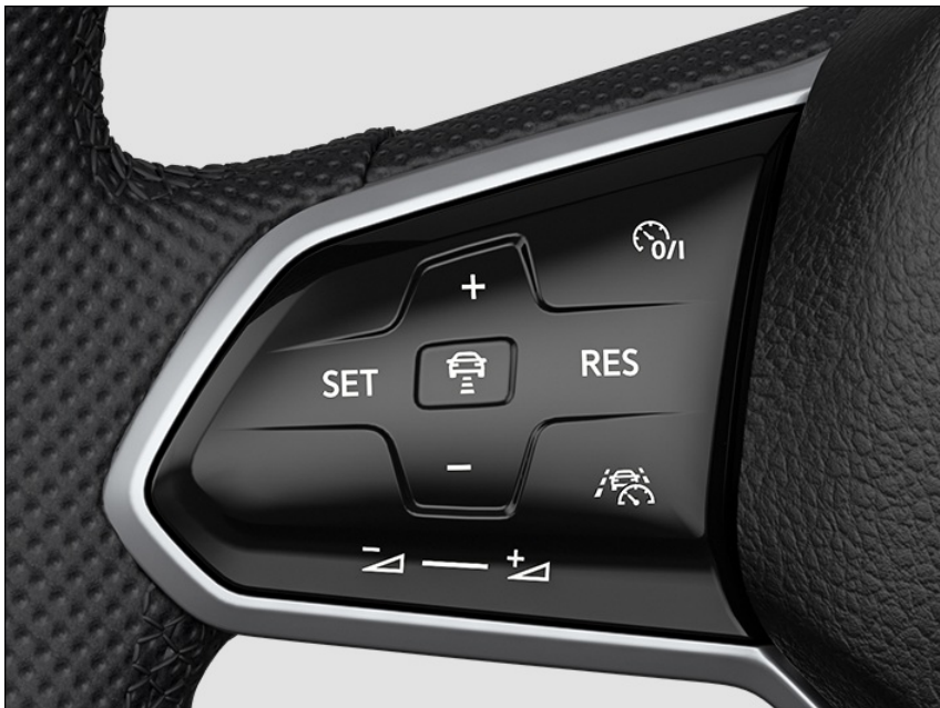
Fig. 111 Left side of the multi-function steering wheel (variant 2).
