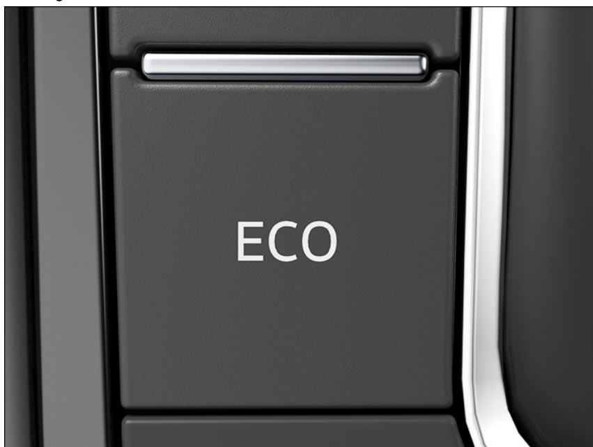
Fig. 106 In the center console: Button for the ECO mode.
