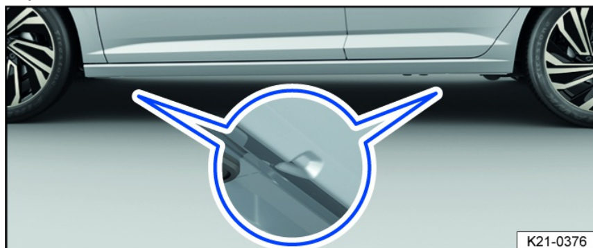
Fig. 176 Lift points for the vehicle jack (variant 1).
