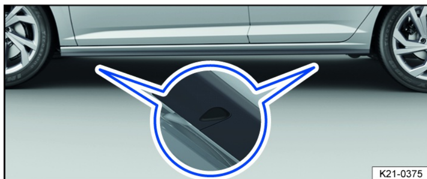
Fig. 177 Lift points for the vehicle jack (variant 2).
