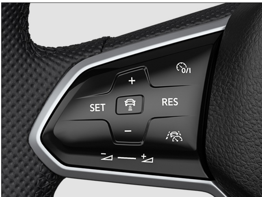
Fig. 114 Left side of the multi-function steering wheel (variant 2).
