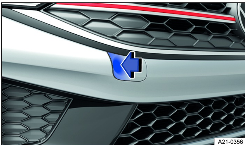
Fig. 149 In the right front bumper: Remove the cover, variant 2.
