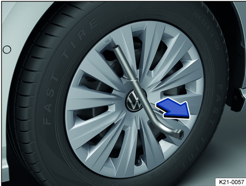
Fig. 173 Remove the wheel hub cover.
