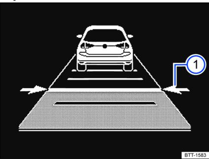
Fig. 116 In the instrument cluster display: set distance (1) (general example, ACC is regulating).
