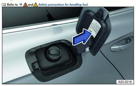
Fig. 134 On the inside of the fuel filler flap: fuel label (general example)
