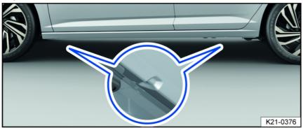
Fig. 179 Lift points for the vehicle jack (variant 1).
