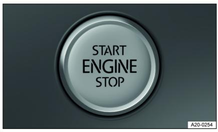
Fig. 96 In the lower area of the center console: starter button for starting the engine.
