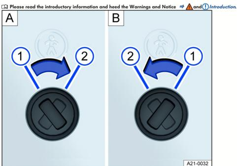
Fig. 57 Child safety lock: A left rear door, B right rear door.
