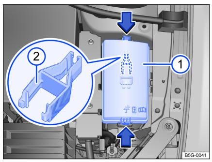
Fig. 140 In the engine compartment: Fuse box.
