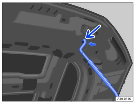
Fig. 159 On the engine hood: Hood support bracket.
