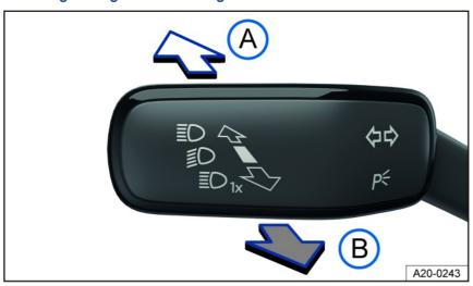
Fig. 81 On the left side of the steering column: turn signal and high beam lever.
