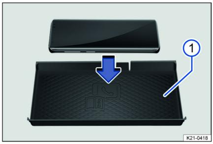
Fig. 131 Diagram: storage compartment with a liner pad for wireless charging.
