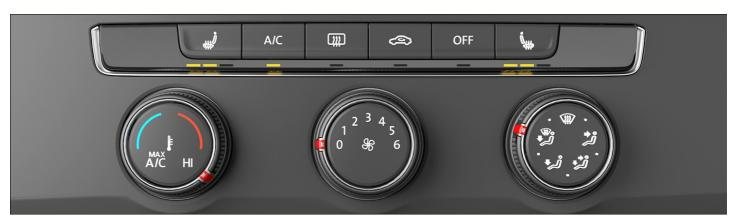
Fig. 89 In the upper section of the center console: Climate control bar for the manual climate control system.
