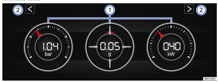
Fig. 21 On the Infotainment system screen: performance monitor.
