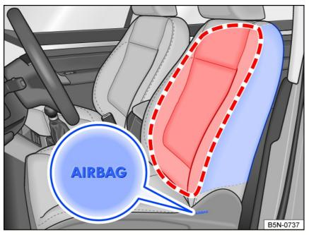
Fig. 33 On the side of the front seat: Side airbag installation location and deployment zone
