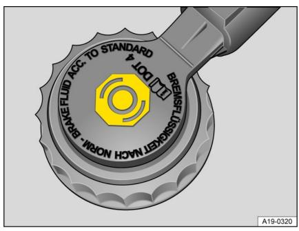
Fig. 166 In the engine compartment: cap on the brake fluid reservoir (version 1).
