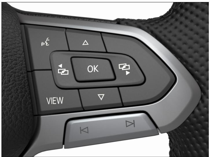
Fig. 10 Right side of the multi-function steering wheel: buttons for operating the menus and information displays in the Volkswagen Digital Cockpit Pro Version (version 1).
