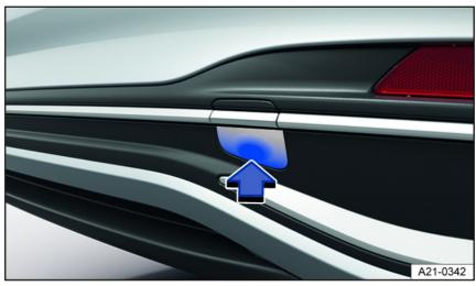
Fig. 152 In the right rear bumper: Remove the cover, variant 1.
