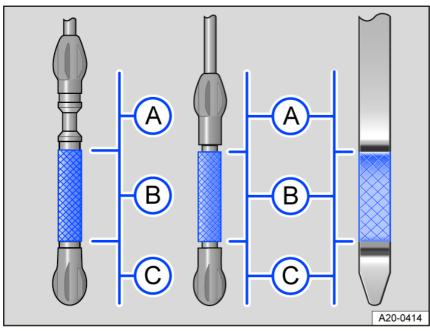
Fig. 163 Engine oil level markings on the oil dipstick (versions).
