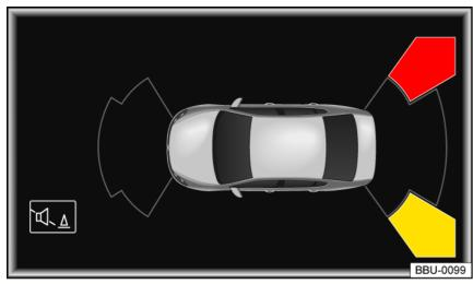
Fig. 125 Infotainment system: Rear Traffic Alert display (depending on the vehicle equipment).
