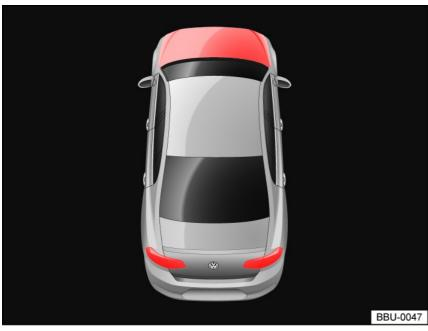
Fig. 160 In the instrument cluster display: the hood is open or not closed correctly (general example).
