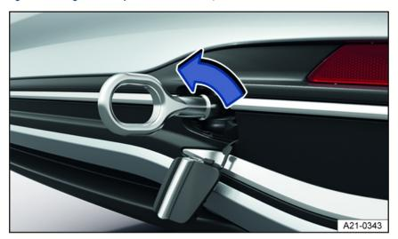
Fig. 153 In the right rear bumper: Screw in towing eye, variant 1.
