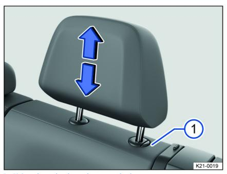
Fig. 72 General example: adjusting the rear center head restraint.
