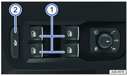
Fig. 62 In the driver door: Power window buttons.
