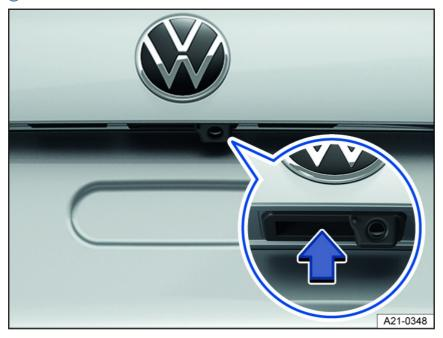
Fig. 59 In the trunk lid: button to open the trunk lid.
