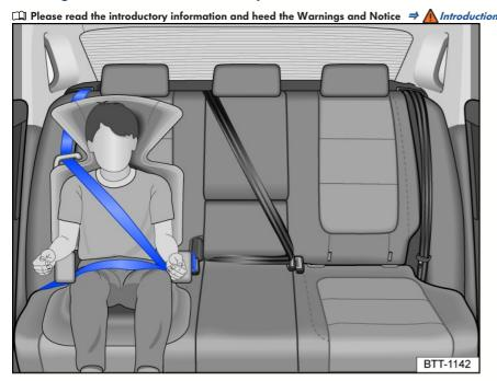
Fig. 42 Correctly fastened child on a booster seat.
