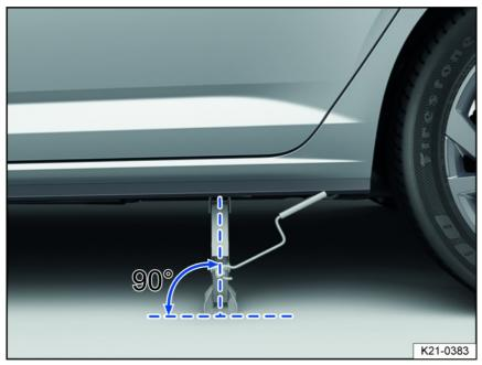
Fig. 181 Correct jack setup (variant 1).
