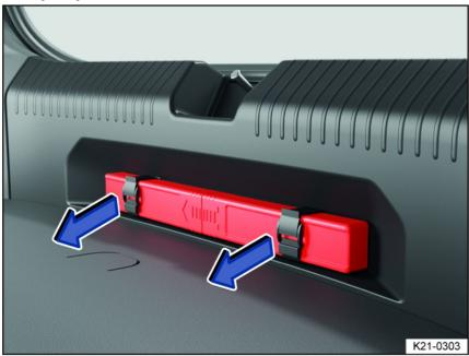
Fig. 43 Underneath the load sill: holder for the warning triangle.
