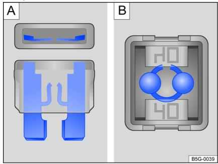
Fig. 144 Blown fuse (general example).
