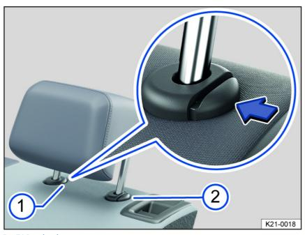
Fig. 74 Rear head restraint: removing.
