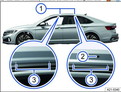
Fig. 133 Mounting points for base supports.
