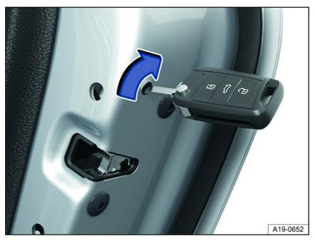
Fig. 56 On the front of the right rear door: emergency locking the vehicle with the vehicle key (general example).
