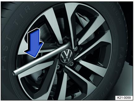
Fig. 185 Wheel change: removing wheel bolts with the lug wrench.
