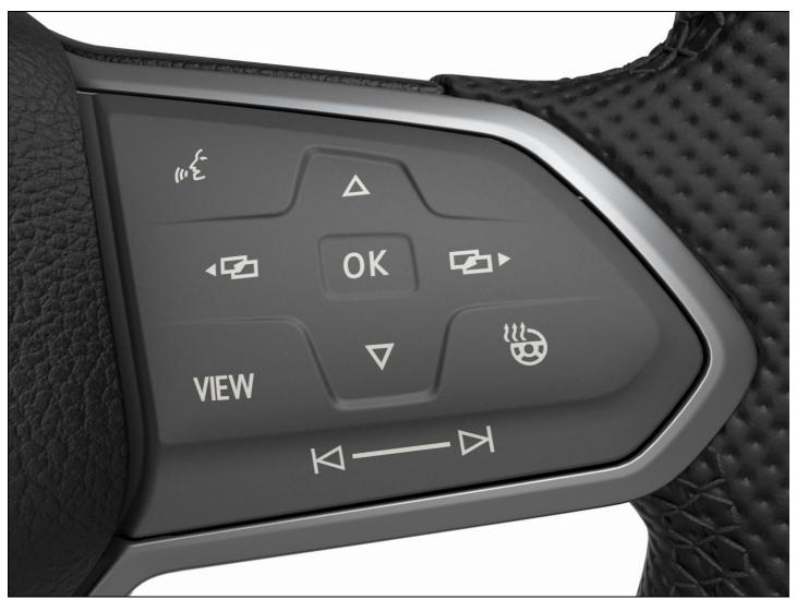
Fig. 11 Right side of the multi-function steering wheel: buttons for operating the menus and information displays in the Volkswagen Digital Cockpit Pro Version (version 2)
