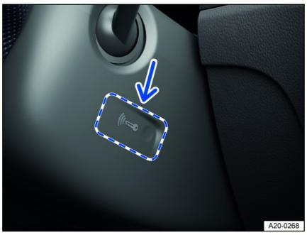
Fig. 98 On the right side of the steering column: emergency start function on vehicles with Keyless Access with push-button start.
