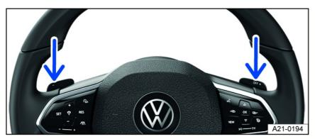
Fig. 103 Steering wheel with shift paddles for Tiptronic.
