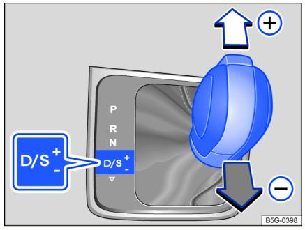
Fig. 102 Selector lever in Tiptronic position.
