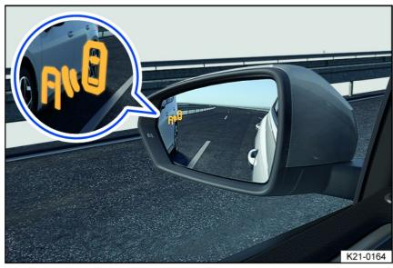
Fig. 121 In the outside mirrors: Blind Spot Monitor indicator.
