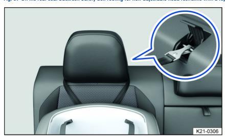
Fig. 40 On the rear seat backrest: Safety belt routing for non-adjustable head restraints with a V-shaped top tether safety belt.
