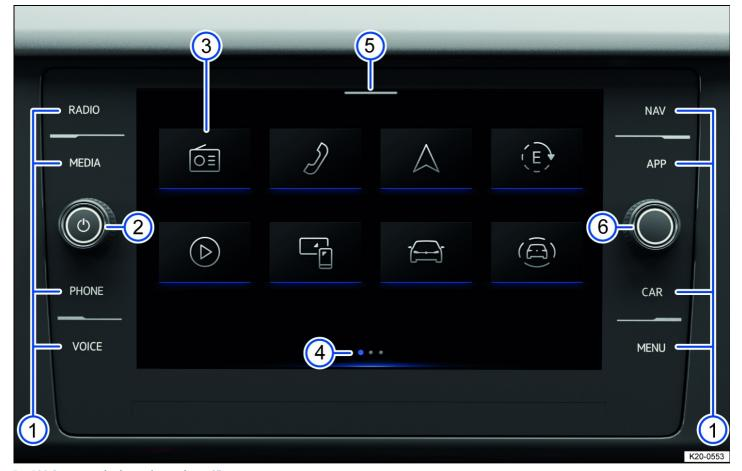
Fig. 129 Overview: display and control unit, 8" version.
