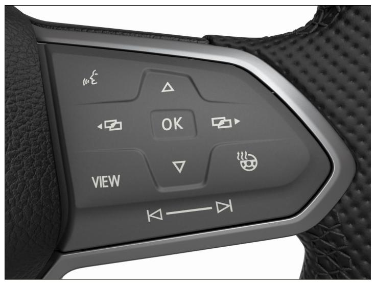
Fig. 14 Right side of the multi-function steering wheel: buttons for operating the menus and information displays in the Volkswagen Digital Cockpit Basic Version (version 2).
