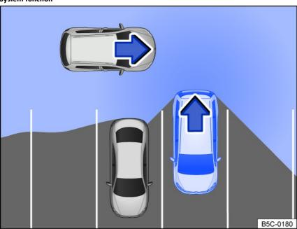
Fig. 124 Rear Traffic Alert, general example: monitored area around the vehicle that is exiting a parking space.
