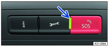
Fig. 44 In the roof console: controls for call services.
