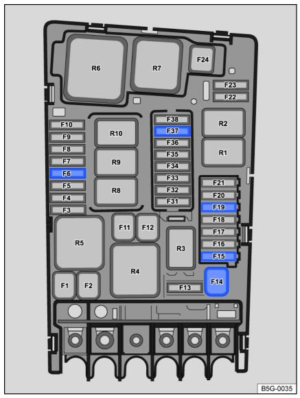
Fig. 141 Fuse locations in the engine compartment.
