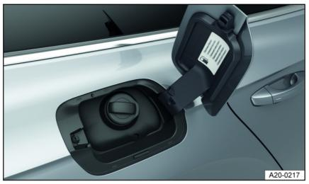
Fig. 135 Behind the fuel filler flap: fuel tank cap (general example)
