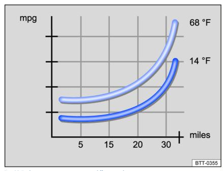
Fig. 93 Fuel consumption in mpg at two different ambient temperatures.
