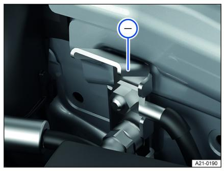
Fig. 146 In the engine compartment: jump-start point (negative terminal).
