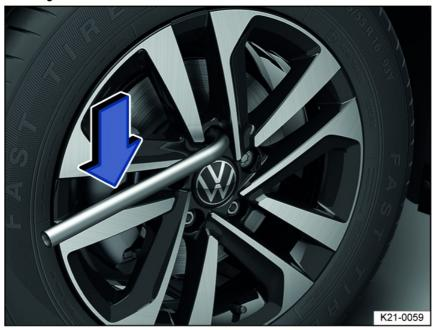
Fig. 176 Changing a tire: loosening the wheel bolts.
