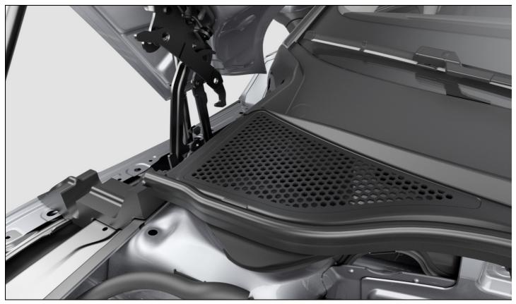
Fig. 187 Between the engine compartment and windshield: plenum chamber (general example).
