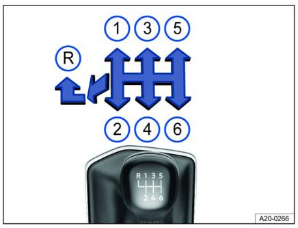
Fig. 100 Gear shift pattern for 6-speed manual transmission. Your vehicle may be equipped with a 5-speed manual transmission.
