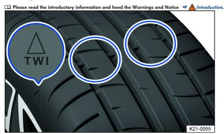
Fig. 171 Tire tread: tread wear indicator.
