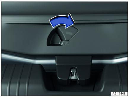
Fig. 61 In the luggage compartment: mechanically unlocking the trunk lid using the emergency release.
