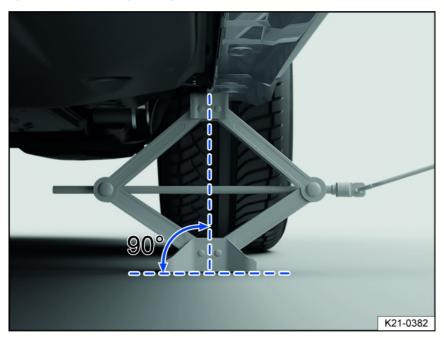
Fig. 182 Jack positioned on the left side of the vehicle at the rear (variant 1).
