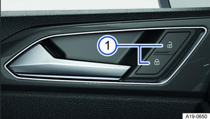
Fig. 54 In the driver's door: central locking button.
