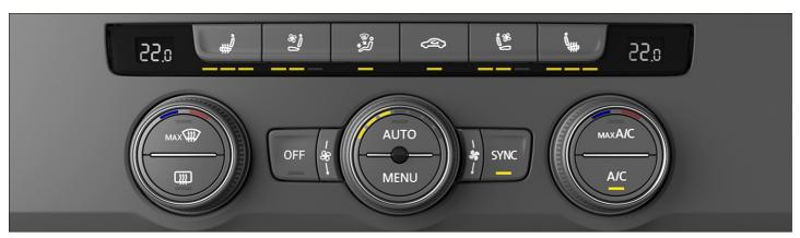
Fig. 88 In the upper section of the center console: Climate control bar for the Climatronic system.
