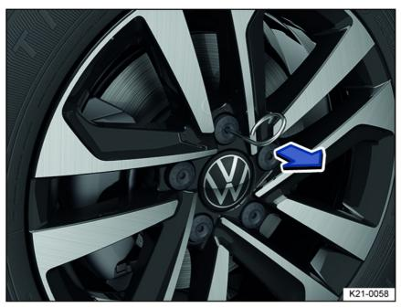
Fig. 175 Remove the caps from the wheel bolts.
