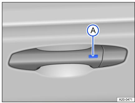
Fig. 53 In door handle: Button to unlock or lock.
