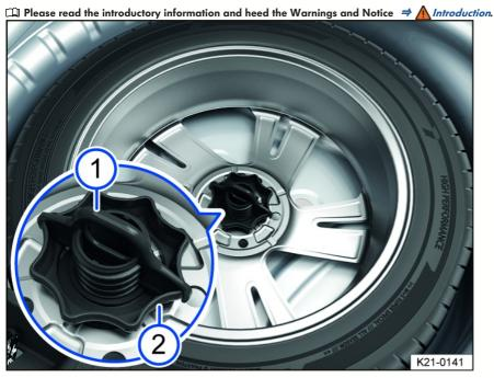
Fig. 178 In the luggage compartment: handle to secure the compact spare wheel.
