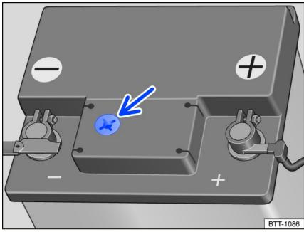
Fig. 168 Window on the top of the 12 V vehicle battery (general example).
