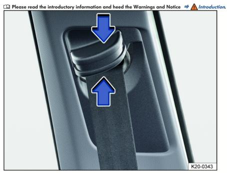
Fig. 28 Next to the front seats: safety belt height adjuster.
