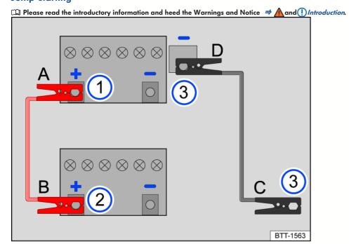
Fig. 147 Diagram for connecting the jumper cables.
