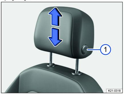
Fig. 71 General example: adjusting the front head restraint.
