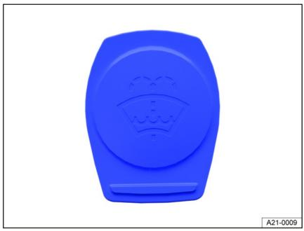
Fig. 161 In the engine compartment: Cap on the washer fluid reservoir (general example).
