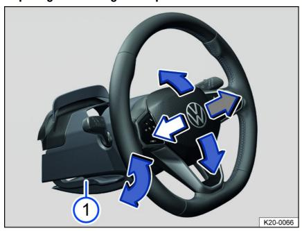
Fig. 64 Under the steering wheel in the steering column trim panel: lever to adjust the steering wheel position manually (general example).
