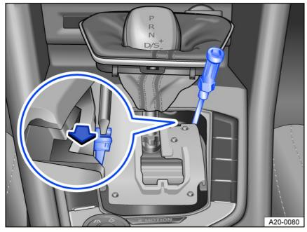
Fig. 105 Manually release the Automatic Shift Lock (ASL) (variant 2).
