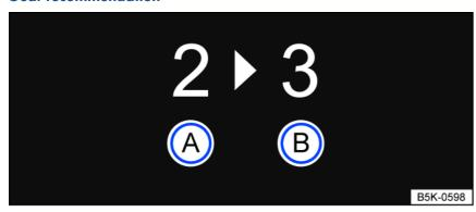
Fig. 92 Gear recommendation on the instrument cluster display.
