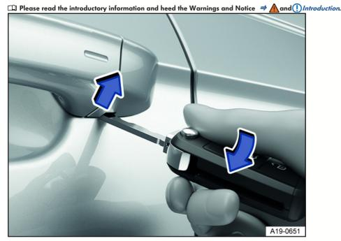
Fig. 55 Driver's door handle: prying off the cap.
