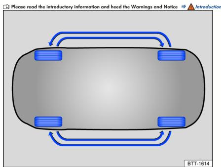
Fig. 169 General example: Diagram for rotating the wheels.
