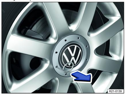
Fig. 173 Remove the hubcap.
