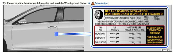
Fig. 170 On the driver door pillar: tire pressure sticker
