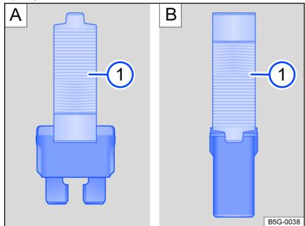
Fig. 145 Remove or install a fuse with the plastic pliers (general example).
