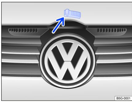
Fig. 157 Above the radiator grille: Opening lever for the hood (general example).
