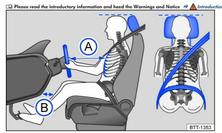
Fig. 22 General example: correct distance between the driver and the steering wheel, correct safety belt routing and correct head restraint adjustment.
