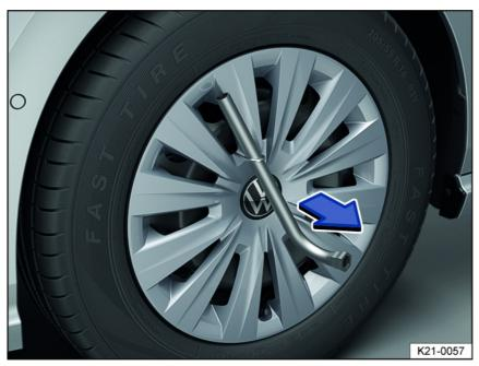
Fig. 174 Remove the wheel hub cover.
