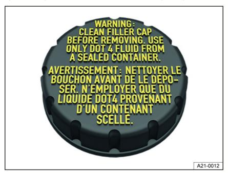
Fig. 167 In the engine compartment: cap on the brake fluid reservoir (version 2).
