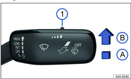
Fig. 83 On the right side of the steering column: windshield wiper lever.
