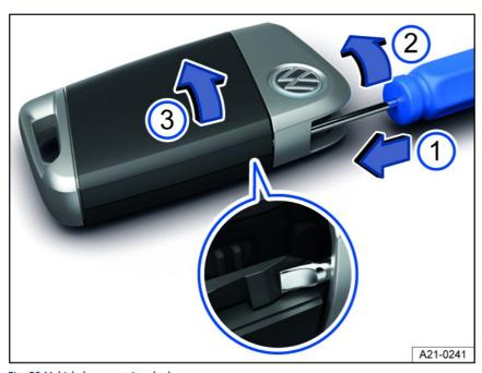
Fig. 50 Vehicle key: opening the battery compartment cover.
