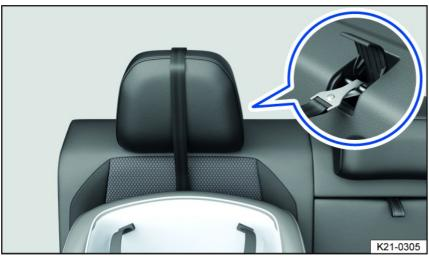
Fig. 39 On the rear seat backrest: Safety belt routing for non-adjustable head restraints with a top tether individual belt.
