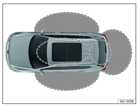
Fig. 52 Keyless Access: Sensor ranges (general example).
