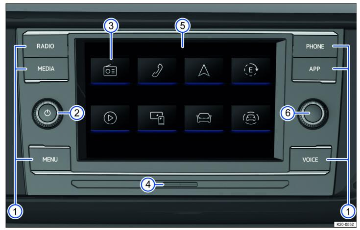
Fig. 130 Overview: display and control unit, 6.5" version.
