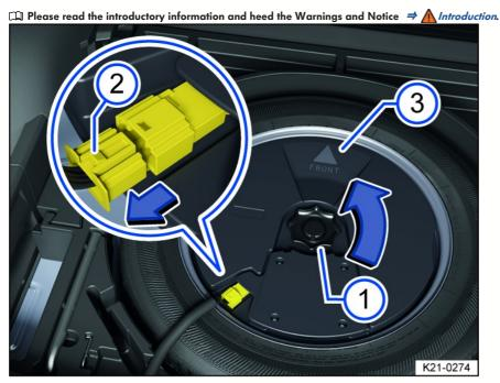
Fig. 177 In the luggage compartment: Removing the subwoofer.
