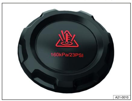
Fig. 164 In the engine compartment: cap on the engine coolant expansion tank.
