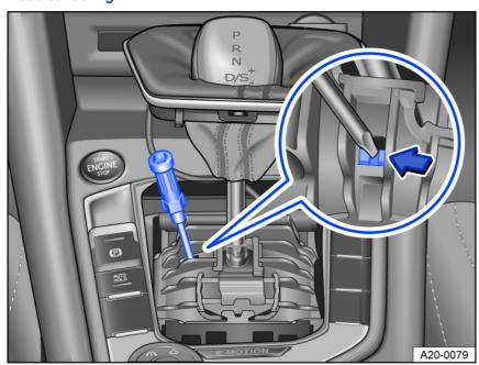
Fig. 104 Manually release the Automatic Shift Lock (ASL) (variant 1).
