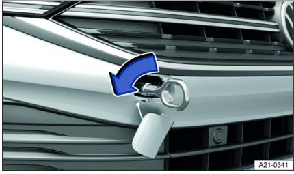
Fig. 150 In the right front bumper: Screw in the towing eye, variant 1.
