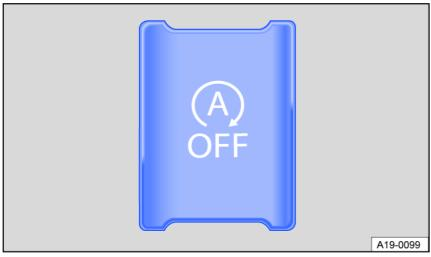
Fig. 99 In the lower section of the center console: Button for the start-stop system.
