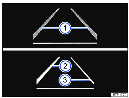
Fig. 117 In the instrument cluster display: Lane Assist indicators.
