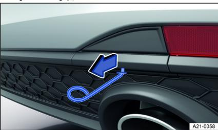
Fig. 154 In the right rear bumper: Remove the cover, variant 2.
