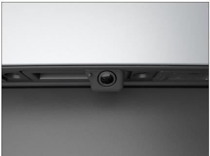
Fig. 188 In the rear of the vehicle: Rear View Camera system on the handle (general example).
