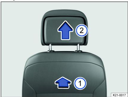
Fig. 73 Front head restraint: removing.
