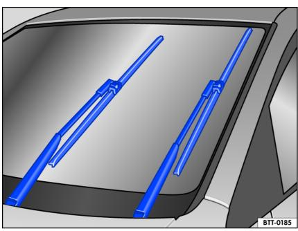
Fig. 137 Windshield wipers in service position (general example).
