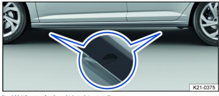
Fig. 180 Lift points for the vehicle jack (variant 2).
