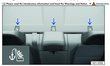
Fig. 38 In the storage compartment behind the rear bench seat: Top tether anchorages for the top tether safety belt.
