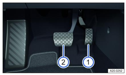
Fig. 91 In the footwell: Pedals in vehicles with an automatic gearbox.
