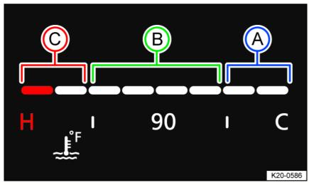
Fig. 18 Coolant temperature gauge in the Volkswagen Digital Cockpit Basic version (general example).
