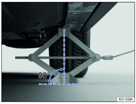
Fig. 184 Jack positioned on the left side of the vehicle at the rear (variant 2).
