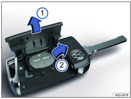
Fig. 49 Vehicle key: Replacing the button cell battery (general example).
