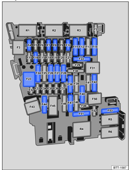
Fig. 143 Fuse assignment in the instrument panel.
