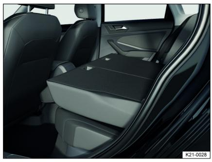
Fig. 70 Rear bench seat: Rear seat backrest folded forwards.
