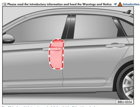
Fig. 32 In the vehicle interior on the left-hand side: Side airbag deployment zone.
