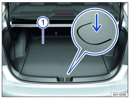
Fig. 132 In the luggage compartment: opening the luggage compartment floor.
